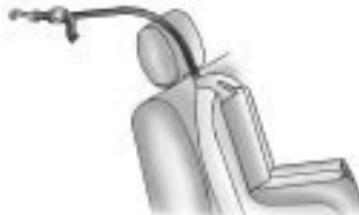
If the position you are using has a fixed headrest or head restraint and you are using a single tether, route the tether over the headrest or head restraint.
