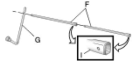
1. Assemble the two jack handle extensions (F) and wheel wrench (G).
