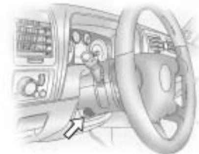
The tilt lever is located on the left side of the steering column.
