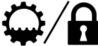
The automatic transmission dipstick handle with this symbol on it is located in the engine compartment on the passenger side of the vehicle.
