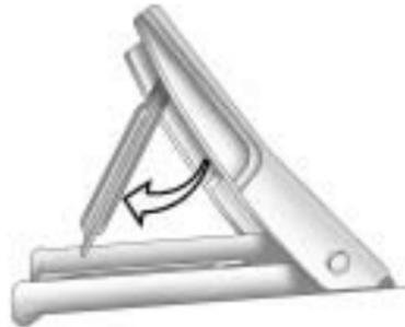
To use the wheel blocks, lift the wheel block and lock it into place.
