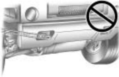
If the vehicle has a brush guard, never tow or apply any loads onto the brush guard.
