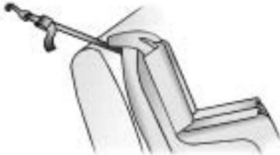
If the position you are using does not have a headrest or head restraint and you are using a single tether, route the tether over the seatback.
