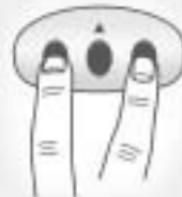
1. Press and hold down the two outside buttons until the indicator light begins to flash, after 20 seconds.
