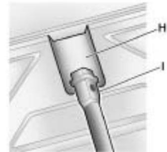
2. Insert the hoist end of the extension tool (I) through the hoist shaft access ramp (H).
