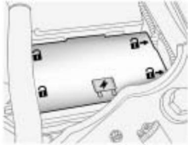
The engine compartment fuse block is located on the driver side of the engine compartment. See *Engine Compartment Overview* on page 5-10 for more information on location.
