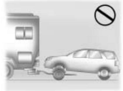
**Notice:** Dolly towing the vehicle will damage drivetrain components. Do not dolly tow the vehicle.
