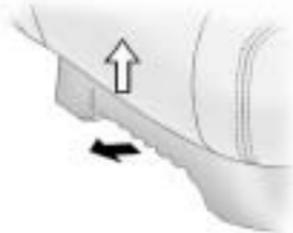
1. Reach under the front of the seat and lift the cushion up while moving it forward.
