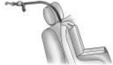
If the position you are using has a fixed headrest or head restraint and you are using a single tether, route the tether over the headrest or head restraint.
