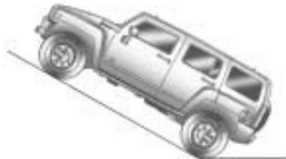
Design specifications required a minimum gradeability of 60% (31 degrees) slope, with the vehicle fully loaded, on high friction surfaces with maximum vehicle speed not to exceed 6 mph (9.7 km/h). The vehicle is expected to traverse this grade only for short durations. Never stop and idle the vehicle or park it on this grade.
