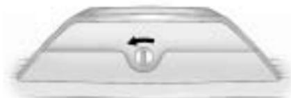
1. Turn the crossrail key counterclockwise to unlock the crossrail end cap.
