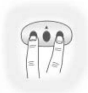
1. From inside the vehicle, press and hold down the two outside buttons at the same time, releasing only when the Universal Home Remote indicator light begins to flash, after 20 seconds. This step erases the factory settings or all previously programmed buttons.
