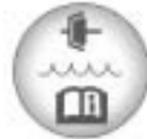
The hydraulic clutch fluid reservoir cap has this symbol on it. See *Engine Compartment Overview on page 5-10* for reservoir location.
