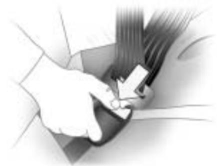
To unlatch the belt, push the button on the buckle. The belt should return to its stowed position. Slide the latch plate up the safety belt webbing when the safety belt is not in use. The latch plate should rest on the stitching on the safety belt, near the guide loop on the side wall.
