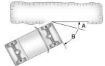
If you encounter a large dip in the terrain, do not enter straight on; enter at an angle — 15° minimum approach (A), 75° maximum approach angle (B).
