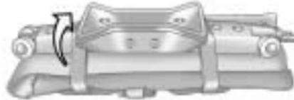
2. Secure the tool bag to the jack by securely wrapping the straps around the jack. Then, slide the straps through the rings on the bag and secure.
