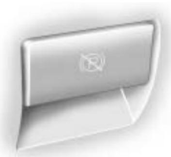
To release the parking brake, hold the regular brake pedal down. Pull the park brake release lever, located above the parking brake pedal.
