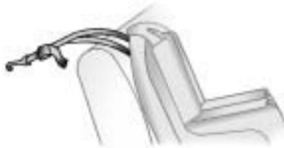
If the position you are using does not have a headrest or head restraint and you are using a dual tether, route the tether over the seatback.
