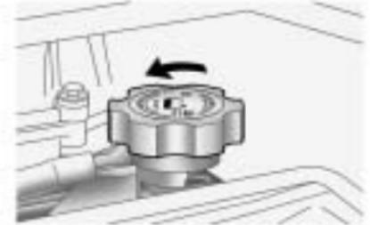
1. Remove the radiator pressure cap when the cooling system, including the upper radiator hose, is no longer hot. Turn the pressure cap slowly counterclockwise about one full turn.
