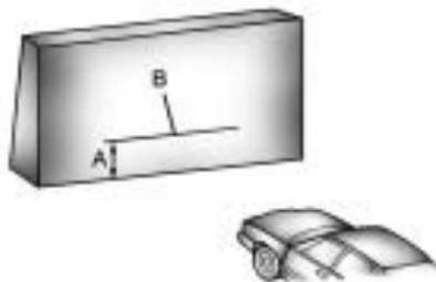
3. At a wall, measure from the ground upward the recorded distance from Step 2 and mark it.
