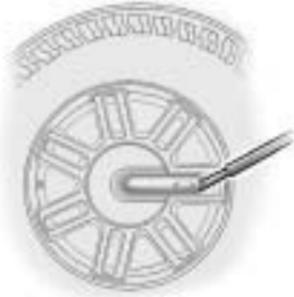
Remove the center cap, if equipped, by placing the flat end of the wheel wrench in the slot on the wheel and gently pry the center cap out.
