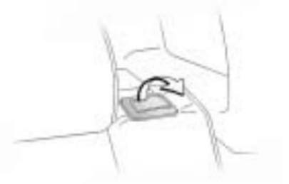
3. Lift the latch on top of the seatback and pull the seatback forward. Fold the seatback down until it is nearly flat.
