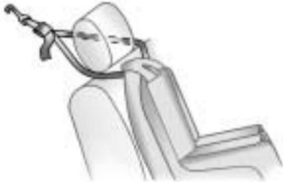
If the position you are using has a fixed headrest or head restraint and you are using a dual tether, route the tether around the headrest or head restraint.
