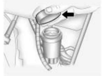
Refer to the Maintenance Schedule to determine how often to check the fluid level in the clutch master cylinder reservoir and for the proper fluid. See *Recommended Fluids and Lubricants on page 6-12*.
