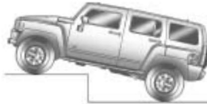
The vehicle can climb a 16 inch (40.6 cm) vertical step. Step climbing is best done by approaching the step at an angle rather than straight on.
