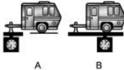
The trailer tongue weight (A) should be 10 percent to 15 percent of the total loaded trailer weight (B), up to a maximum of 500 lbs (227 kg) with a weight carrying hitch or a weight distributing hitch.
