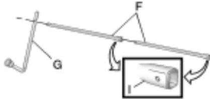
4. Assemble the two jack handle extensions (F) and wheel wrench (G).
