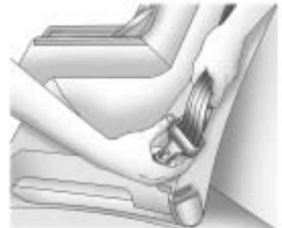
3. For H3T models, tilt the latch plate to adjust the belt if needed.
