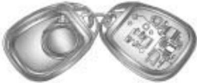
1. Separate the transmitter with a flat, thin object inserted into the notch on the side.
