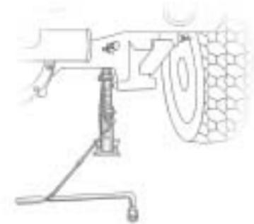
**Rear Tire Flat:** Use the jack handle and both jack handle extensions. Attach the wheel wrench to the jack extensions. Attach the jack handle to the jack. From the rear of the vehicle align the jack under the rear axle. Turn the wheel wrench clockwise to raise the vehicle. Raise the vehicle far enough off the ground so there is enough room for the spare tire to clear the ground.
