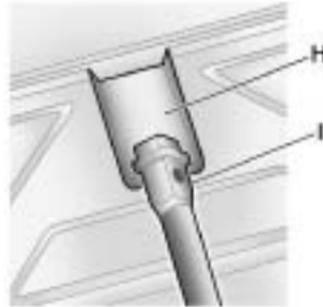
5. Insert the hoist end of the extension tool (I) through the hoist shaft access ramp (H).
