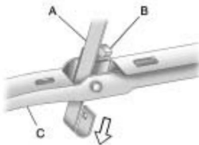
2. Push the release lever (B) to disengage the hook and push the wiper arm (A) out of the blade (C).
