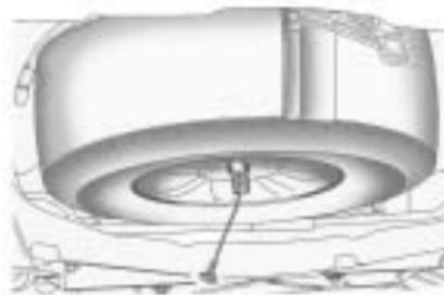
2. Turn the lug wrench counterclockwise until approximately 6 inches (15 cm) of cable is exposed.
