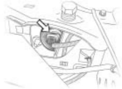
2. Turn the bulb socket counterclockwise to remove it from the headlamp assembly and pull it straight out.
