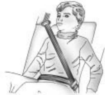
4. Buckle, position, and release the safety belt as described previously in this section. Make sure that the shoulder belt crosses the shoulder.
