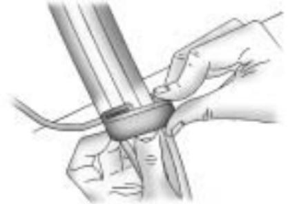
2. Place the guide over the belt and insert the two edges of the belt into the slots of the guide.
