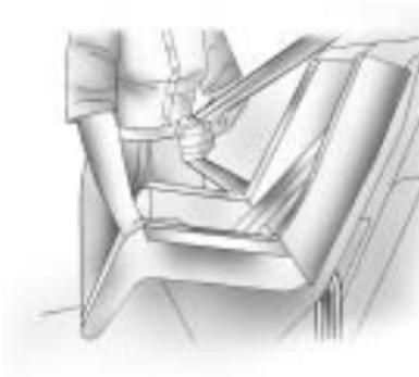
5. For H3 models, pull the rest of the shoulder belt all the way out of the retractor to set the lock.
