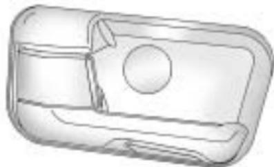
From the inside, use the manual lock levers or power door lock switch.
