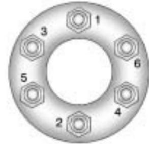
13. Tighten the nuts firmly in a crisscross sequence as shown by turning the wheel wrench clockwise.
