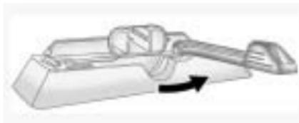
3. Pull the lever labeled "PULL" from left to right to loosen the crossrail.
