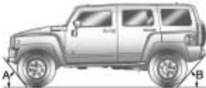
The H3 has an approximate approach angle (A) of 37.4 degrees and a departure angle (B) of 34.7 degrees, depending on suspension packages.
