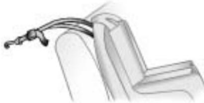
If the position you are using does not have a headrest or head restraint and you are using a dual tether, route the tether over the seatback.
