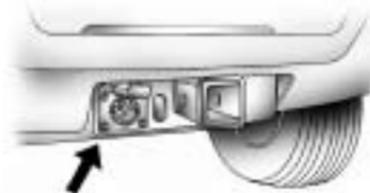
Connect the adapter to the seven-pin universal heavy-duty trailer connector attached to the bracket on the hitch platform. The flip cap on the vehicle's harness locks onto the tab and helps hold the adapter in place. Plug the four-way pin connector onto the adapter.
