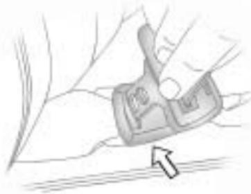
1. Disconnect the rear center safety belt latch from the mini buckle by inserting the tip of the safety belt into the slot on the buckle. Let the belt retract.
