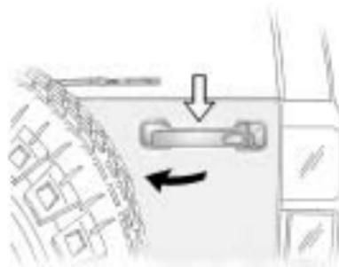
To open the swing-gate, use the door handle to pull the swing-gate rearward slightly so it opens automatically.
