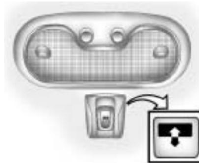
The switch used to operate the sunroof is located in the headliner.
