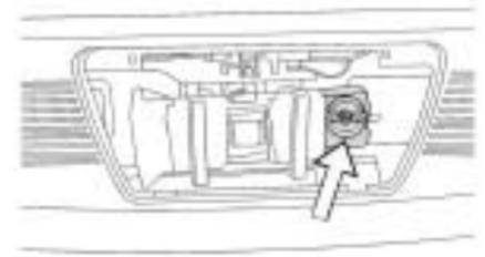
4. Reinstall the wing nut retainer to fasten the jack and tool bag in the storage compartment.
