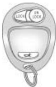
**LOCK:** Press to lock all the doors. The parking lamps may flash and the horn may chirp.
