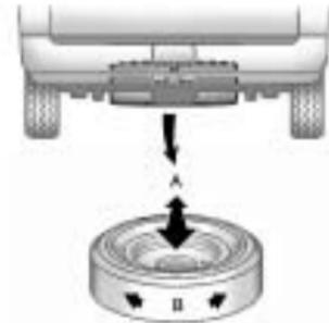
8. Push, pull (A) and then try to turn (B) the tire. If the tire moves, use the wheel wrench to tighten the cable.
