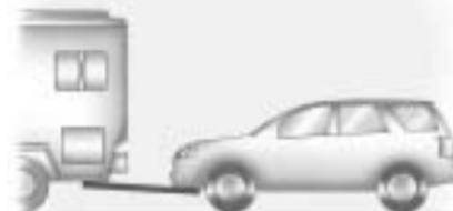
This full-time four-wheel-drive vehicle can be dinghy towed from the front. These vehicles can also be towed by placing them on a platform trailer with all four wheels off the ground. These vehicles cannot be towed using a dolly.
