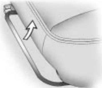
1. Lift the bar to unlock the seat.
