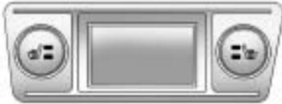
If the controls are located on the center console, press the button to turn the heated seat and seatback on or off.
