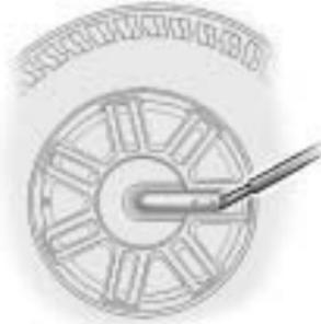
2. Remove the center cap by placing the flat end of the wheel wrench in the slot on the wheel and gently pry the center cap out.
