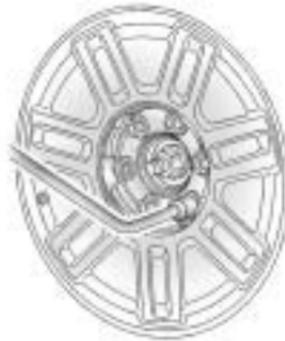
3. Turn the wheel wrench counterclockwise to loosen the wheel nuts. Do not remove them yet.
