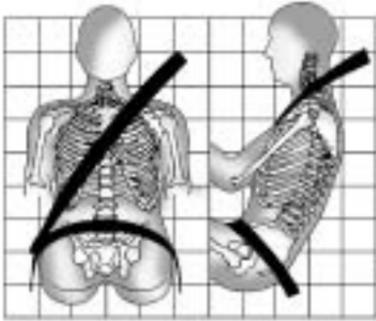
Sit up straight and always keep your feet on the floor in front of you. The lap part of the belt should be worn low and snug on the hips, just
