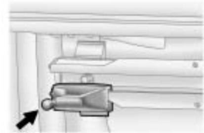
To adjust a tie-down, pull the locator pin out and move the tie-down to another location making sure the locator pin lines up with a locator hole on the rail. The tie-down pin may not be installed correctly if the pin does not line up, turn it over and reinstall. The tie-down will not move when the pin is completely installed. The maximum load for each rail is 500 lbs (227 kg).
