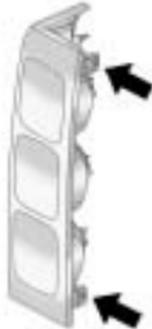
2. Remove the two screws from the taillamp assembly.
