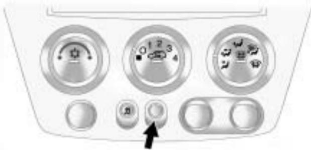
The off-road lamps button is located on the instrument panel below the climate controls.
