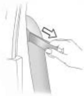
2. Pull the loop, located on the outboard side of the seatback, forward until you hear a click.
