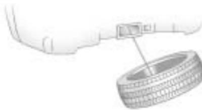
6. Tilt the tire, with slack in the cable, to access the tire/wheel retainer (B).
