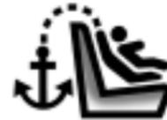
For H3T models, the top tether anchor symbol is located near the top tether anchors to assist you in locating the top tether anchors.
