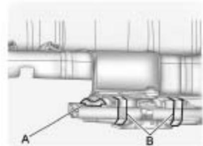
1. Turn the wing nut (A) counterclockwise to release the jack and tools.
