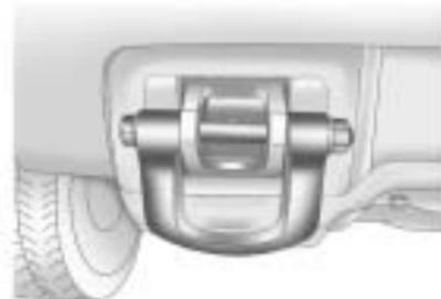
The vehicle has two recovery loops at the front of the vehicle and one at the rear of the vehicle.
