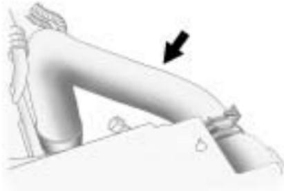
6. Start the engine and let it run until you can feel the upper radiator hose getting hot. Watch out for the engine cooling fan.
