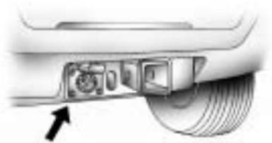
If the vehicle has a trailer towing package, the rear bumper harness will have a seven-pin universal heavy-duty trailer connector attached to a bracket on the hitch platform.
