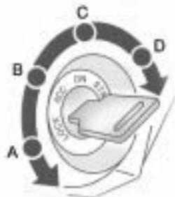
The ignition switch has four different positions.
