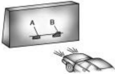
7. Turn the vertical aiming screw until the headlamp beam is aimed to the horizontal tape line. Turn it clockwise or counterclockwise to raise or lower the beam.
