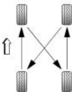
When rotating the vehicle's tires, always use the correct rotation pattern shown here. Do not include the spare tire in the tire rotation.
