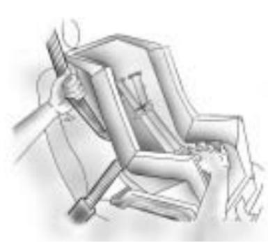
6. To tighten the belt, push down on the child restraint, pull the shoulder portion of the belt and feed the lap portion of the belt into the retractor. When installing a forward-facing child restraint, it may be helpful to use your knee to push down on the child restraint as you tighten the belt.
