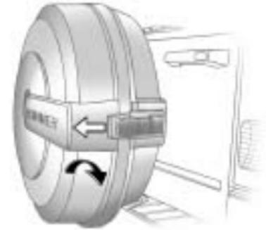
1. If the vehicle has a spare tire cover release the latch by pulling the latch straight back and turning it away from the cover at the same time.
