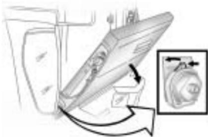
1. Open the tailgate fully and remove the retainer clip from the driver's side hinge.
