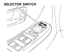
Adjust the outside mirrors with the adjustment switch on the driver's door armrest:
