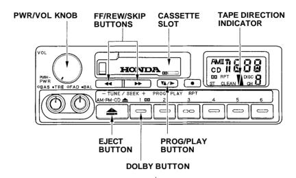
Dolby® noise reduction turns on when you insert a cassette. If the tape was not recorded with Dolby "B" noise reduction, turn it off by pressing the DID button.
