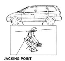
10. Find the jacking point nearest the wheel you are removing. Place the jack under the jacking point. Turn the end bracket clockwise until the top of the jack contacts the jacking point. Make sure the jacking point tab is resting in the jack notch.
