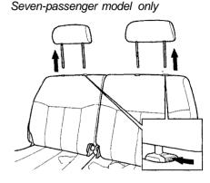
You can recline the seat-backs on the second seat so they are level with the seat cushion of the third seat, making a large, cushioned area. To do this:
