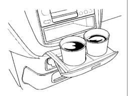
Use the beverage holder only when the car is parked. If you place cups in the holder while driving, the liquid may spill when you go over bumps or around corners.
