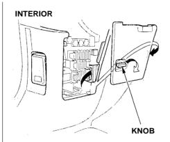
The interior fuse box is underneath the dashboard on the driver's side. To open, turn the knob as shown.
