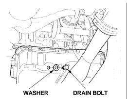
2. Open the hood and remove the engine oil fill cap. Remove the oil drain bolt from the bottom of the engine. Drain the oil into an appropriate container.
