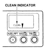
The cassette drive picks up dirt and oxides whenever you play a tape. This builds up over time and causes the sound quality to degrade. To prevent this, you should clean the cassette drive after every 30 hours of use. Your dealer has a cleaning kit available for this purpose.
