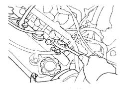
5. Torque the spark plug. (If you do not have a torque wrench, tighten the spark plug 2/3 turn after it contacts the cylinder head.) Tightening torque: 18 N m (1.8 kg-m, 13 lb-ft)
