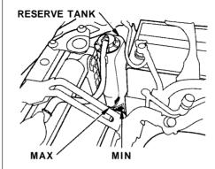
Look at the coolant level in the radiator reserve tank. Make sure it is between the MAX and MIN lines. If it is below the MIN line, see **Adding Engine Coolant** on page 151 for information on adding the proper coolant.
