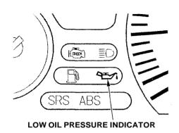
The low oil pressure indicator should never come on when the engine is running. If this light flashes or stays on with the engine running, take immediate action.
