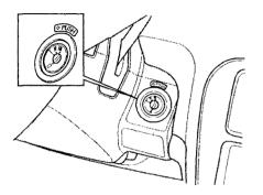
The ignition switch is on the right side of the steering column. It has tour positions: LOCK (0), ACCESSORY (I), ON(II), and START (III).
