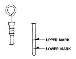
Pull it out again and look at the oil level at the end of the dipstick. If it is between the upper and lower marks, the level is correct. Add oil if the level is at or below the lower mark.
