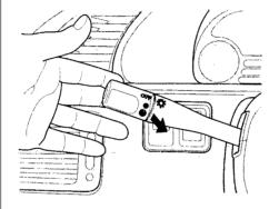
To change between low beams and high beams, pull back on the turn signal lever until you hear a click, then let go. The blue high beam indicator will light (see page 38).
