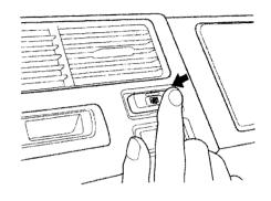
The rear window defogger will clear fog, frost, and thin ice from the window. Push the defogger button to turn it on and off. The light in the button lights to show the defogger is on. If you do not turn it off, the defogger will shut itself off after about 25 minutes. It also shuts off when you turn off the ignition. You have to turn it on again when you restart the car.
