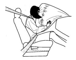
If you ever have a severe frontal collision, the passenger's airbag will inflate at the same time as the driver's airbag.
