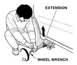
11.Use the extension and wheel wrench as shown to raise the car. until the flat tire is off the ground.
