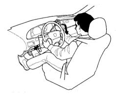
Reverse (R) — To shift to Reverse from Park, see the explanation under Park. To shift to Reverse from Neutral, come to a complete stop and then shift. Pull the shift lever towards you before shifting into Reverse from Neutral.
