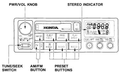
The TUNE function lets you find a desired frequency. Push the TUNE/ SEEK switch up to change to a higher frequency, and down to change to a lower frequency. To change the frequency up or down a single increment, push and release the TUNE/SEEK switch.
