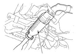
THREE WAY CATALYTIC CONVERTER
