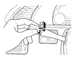
The rotating switch on the left lever controls the lights. Turning this switch to the first position "•" turns on the parking lights, taillights, instrument panel lights, side-marker lights, and rear license plate lights. Turning the switch to the second position "•" turns on the headlights.
