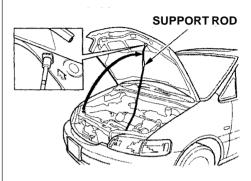
3. Pull the support rod out of its clip and insert the end into the hole on the left side of the hood.
