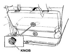
Unlock the seat-back by turning the knob. Push the seat-back forward.
