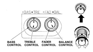
The illumination for the radio controls comes on with the instrument panel lights, even if the radio is off. You can use the Balance control to turn off the radio panel illumination even with the radio on. Push the control knob so it pops out, then pull it out slightly further. Check this control if the control panel lights do not come on with the instrument panel lights.
