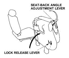
Pull the seat-back angle adjustment lever and tilt the seat-back forward. Then pull the lock release lever and pivot the seat forward.
