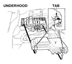
The underhood fuse box is located in the engine compartment on the passenger's side. To open, push the tab as shown.
