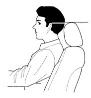
Head restraints can help protect you from whiplash and other injuries. For the best protection, adjust the top of the restraint so it is even with the tops of your ears, or as high as possible. For instructions on adjusting the head restraints, see page 58.
