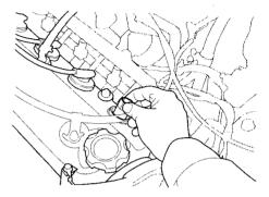
4. Put the new spark plug into the socket, then thread it into the hole. Screw it in by hand so you do not crossthread it.
