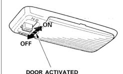
Your Honda has two ceiling lights. Each ceiling light has a three-position switch. In the OFF position, the lights do not come on. In the center position they come on when you open any door. In the ON position, they stay on continuously.
