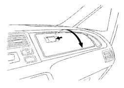
Open the dashboard compartment by squeezing the handle. Close it with a firm push.
