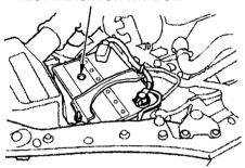
Check the battery condition by looking at the test indicator window on the battery:
