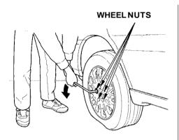
9. Loosen the four wheel nuts 1/2 turn with the wheel wrench.
