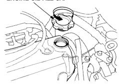
To add oil, unscrew and remove the engine oil fill cap on top of the valve cover. Pour in the oil, and replace the engine oil fill cap. Tighten it securely. Wait a few minutes and recheck the oil level. Do not fill above the upper mark; you could damage the engine.
