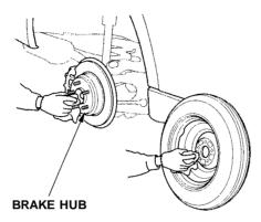
13. Before mounting the spare tire, wipe any dirt off the mounting surface of the wheel and hub with a cloth.
