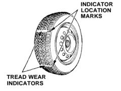
Your car's tires have wear indicators molded into the tread. When the tread wears down to that point, you will see a 12.7 mm (1/2 inch) wide band running across the tread. This shows there is less than 1.6 mm (1/16 inch) of tread left on the tire. A tire that is this worn gives very little traction on wet roads. You should replace the tire if you can see the tread wear indicator in three or more places around the tire.
