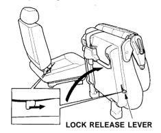
Pull the seat-back angle adjustment lever on the second row seat to tilt the seat-back forward. Pull the lock release lever and pivot the seat up out of the way. Move the second seat back into place by pivoting the seat down. Make sure it locks to the floor. Pull the seat-back angle adjustment lever forward and push the seat-back to the desired position, then release the lever. Make sure the seat is securely locked in place.
