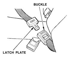
The lap belt has one manuallyadjusted belt that fits across the hips. It is similar to safety belts used in airplanes.
