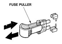
4. Check the smaller fuses in the underhood fuse box and all the fuses in the interior fuse box by pulling out each fuse with the fuse puller provided in the interior fuse box.
