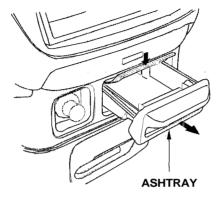
Open the front ashtray by pulling on the bottom edge. Push it in to close it. To remove the ashtray for emptying, push down on the metal plate inside, then pull the ashtray out completely.
