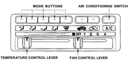
Air conditioning places an extra load on the engine. Watch the engine coolant temperature gauge (see page 40) when using the A/C in heavy traffic or driving up long hills. If it moves near the red zone, turn off the air conditioning until the gauge reads normally.
