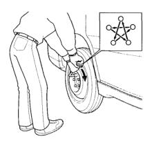
16.Tighten the wheel nuts securely in the same crisscross pattern. Have the wheel nut torque checked at the nearest automotive service facility.
