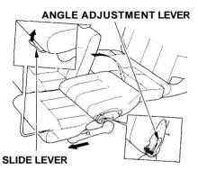
Lift the lever and slide the seat forward as far as it will go. Pull the seat-back angle adjustment lever and pivot the seat-back backward. Release the lever when the seatback is even with the cushion on the third seat.
