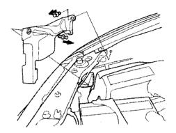
The air cleaner element is inside the box on the passenger's side of the engine compartment.
