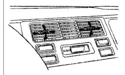
The direction of air flow from the vents in the center and each side of the dashboard is adjustable. Move the tab in the center of each vent upand-down and side-to-side.
