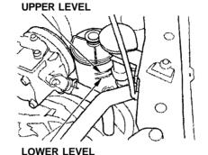
You should check the fluid level in the power steering reservoir monthly. Check the level when the engine is cold. Look at the side of the reservoir. The fluid should be between the UPPER LEVEL and LOWER LEVEL. If it is below the LOWER LEVEL, add power steering fluid to the UPPER LEVEL.
