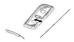
The tailgate light has a two position switch. In the OFF (down) position, the light does not come on. In the ON (up) position, the light comes on when you open the tailgate.
