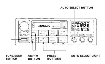
Once that station's frequency is stored, simply press and release the proper preset button to tune to it. If you want to change any preset button's selection, store another frequency as described. The frequencies you preset will be lost if your car's battery goes dead or is disconnected.
