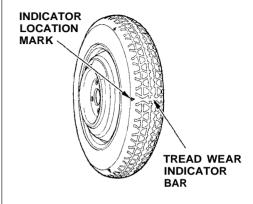
The compact spare tire has a shorter tread life than a regular tire. Replace it when you can see the tread wear indicator bars. The replacement should be the same size and design tire, mounted on the same wheel. The compact spare tire is not designed to be mounted on a regular wheel, and the compact wheel is not designed for mounting a regular tire. If you have a flat tire while driving, stop in a safe place to change it.
