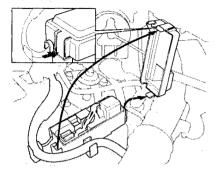
Cars equipped with ABS have a third fuse box for the ABS. It is in the engine compartment on the right side.
