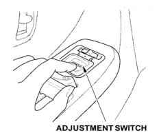
3. Push the appropriate edge of the adjustment switch to move the mirror right, left, up or down.
