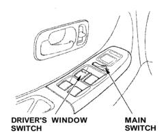
The driver's armrest has a master power window control panel. To open any of the passengers' windows, push down on the appropriate switch and hold it down until the window reaches the desired position. To close the window, pull back on the window switch. Release the switch when the window gets to the position you want.
