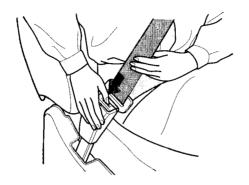
To unlatch the seat belt, push the red PRESS button on the buckle. Guide the belt across your body to the door pillar. If the belt doesn't retract easily, pull it out and check for twists or kinks.
