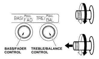
To adjust the Treble level, push on the TREBLE/BALANCE control knob to get it to pop out. Without pulling it out farther, turn the knob to adjust the treble level. Push the knob back in when you are done so you cannot change the setting by accidentally bumping it.
