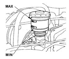
The fluid should be between the MIN and MAX marks on the side of the reservoir. If the level is at or below the MIN mark, it is an indication that your brake system needs attention. Have the brake system inspected for leaks or worn brake pads.
