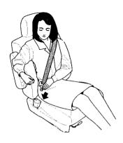
Pull the latch plate across your body and insert it into the buckle. Tug on the belt to make sure the latch is securely locked.
