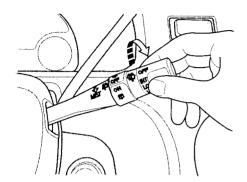
The right lever controls the windshield wipers and washers. The rotary switch at the end of the lever has three positions:
