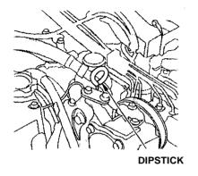
Check the engine oil level every time you fill the car with fuel. Wait at least two minutes after turning the engine off before you check the oil.
