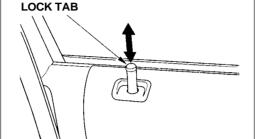
Each door also has a lock tab on the top. When you push down the lock tab on the driver's door, all the doors and the tailgate lock. Pulling up the lock tab on the driver's door unlocks only that door. The lock tab on each passenger's door locks and unlocks only that door.
