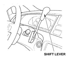
The shift lever has seven positions. It must be in Park or Neutral to start the engine. When you are stopped in D4, D3, 2, 1, N or R, press firmly on the brake pedal and keep your foot off the accelerator pedal.
