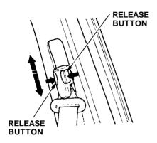
5. If you are sitting in one of the front seats and the shoulder belt crosses your neck, you should adjust the anchor height by squeezing the two buttons and sliding the anchor up or clown.
