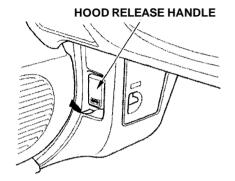
1. Shift to Park or Neutral and set the parking brake. Pull the hood release handle, located under the left lower corner of the dashboard. The hood will pop up slightly.
