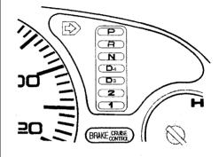
This indicator shows which shift position the shift lever is in. The "D<sub>4</sub>" indicator comes on for a few seconds when you turn the ignition switch ON (II). If it flashes while driving (in any shift position), it indicates a possible problem in the transmission. Avoid rapid acceleration and have the transmission checked by an authorized Honda dealer as soon as possible.
