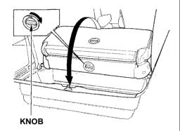
3. Turn the knob on the back of the seat cushion while you pull the entire seat towards you. Pivot the seat into the floor recess.
