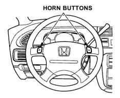
Press either of the buttons on the steering wheel spokes to sound the horn.
