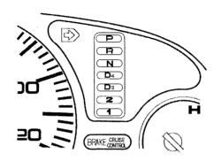
This display is on the instrument panel. It shows you the position of the shift lever. It also indicates a possible problem in the transmission if the "D4" indicator light flashes.
