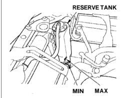
Check the level of the engine coolant by looking at the radiator reserve tank next to the battery. If the level is at or below the MIN line, add coolant to bring it up to the MAX line. Inspect the cooling system for leaks. This coolant should always be a mixture of 50% antifreeze and 50% water. Never add straight antifreeze or plain water.
