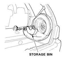
8. Unscrew the wing bolt. Remove the storage bin and spare tire.
