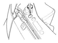
If you cannot get an indicator to align, have your Honda dealer inspect the car for body damage or suspension problems.
