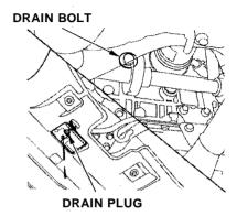
3. Loosen the drain plug on the bottom of the radiator. The coolant will drain through the splash guard. Remove the drain bolt from the engine block.
