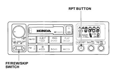
The SKIP and RPT functions use silent periods on the tape to find the end of a selection. These features may not work satisfactorily on tapes that have almost no gap between songs, a high noise level between songs, or silent periods in the middle of songs.
