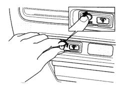
The knob on the dashboard to the left of the steering column controls the brightness of the instrument panel lights. Push the knob to get it to pop out. Turn the knob to adjust the brightness.
