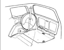
Your Honda has attachment points for a tether-style child seat to be installed on the second or third seat as shown.
