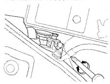
6. If either indicator is not aligned with its "0" mark as described above, an adjustment can be made using a Phillips-head screwdriver to realign it with the "0" mark. Please refer to the illustrations.
