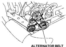
Check the condition of the two drive belts. Examine the edges of each belt for cracks or fraying.
