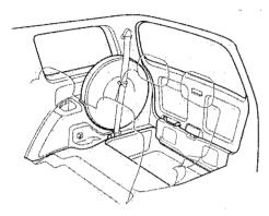
Your Honda has two attachment points on the tailgate sill that allow for a tether-style child seat to be installed in the third row seat.
