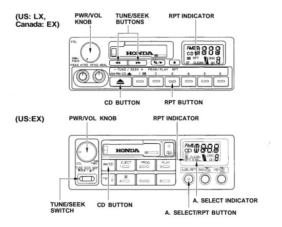
U.S. I.X and Canadian FX models You can use the TUNE/SEEK buttons while a disc is playing to select passages and change tracks. To move rapidly forward within a track, push and hold the button. Push and hold the dutton to move rapidly backward within a track. You will hear a beep a half second after you push the button. Keep pushing the button until you think the track has advanced or returned to the desired position. The disc will start playing when you release the button
