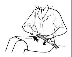
Position the belt as low as possible across your hips and pelvic bones, not across your stomach. Pull the loose end of the belt to adjust for a snug but comfortable fit.
