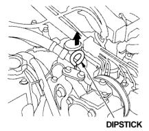
Check the engine oil a couple of minutes after shutting off the engine. This will allow the oil to drain down to the bottom of the engine. Make sure the car is parked on level ground.
