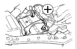
Connect one juniper cable to the positive (+) terminal on the booster battery. Connect the other end to the positive (+) terminal on your Honda's battery.
