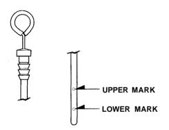
4. Remove it again and check the level. It should be between the upper and lower marks.
