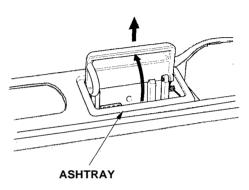
The rear ashtray is in the armrest on the left rear door. To use the rear ashtray, swing the lid open. To remove the rear ashtray, open the lid and pull it straight up.
