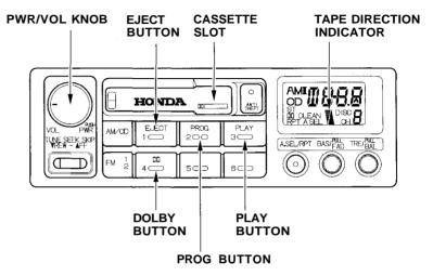
Dolby® noise reduction turns on when you insert a cassette. If the tape was not recorded with Dolby "B" noise reduction, turn it off by pressing the DD button.
