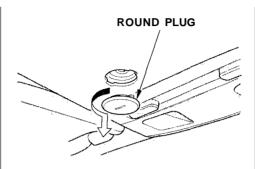
4. Use a screwdriver or coin to remove the round plug in the headliner between the sun visors.
