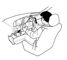
**Reverse (R)** — To shift to Reverse from Park, see the explanation under Park. To shift to Reverse from Neutral, come to a complete stop and then shift. Pull the shift lever towards you before shifting into Reverse from Neutral.
