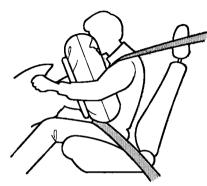
If you ever have a severe frontal collision, the sensors will detect rapid deceleration and signal the control unit to instantly inflate the airbags.
