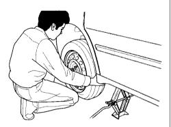
12.Remove the wheel nuts and flat tire. Temporarily place the flat tire on the ground with the outside surface of the wheel facing up. You could scratch the wheel if you put it face down.
