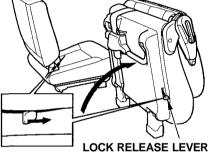
Pull the seat-back angle adjustment lever on the second row seat to tilt the seat-back forward. Pull the lock release lever and pivot the seat up out of the way. Move the second seat back into place by pivoting the seat down. Make sure it locks to the floor. Pull the seat-back angle adjustment lever forward and push the seat-back to the desired position, then release the lever. Make sure the seat is securely locked in place.
