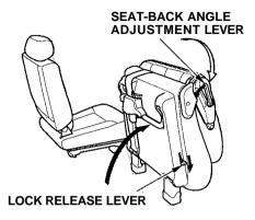
Pull the seat-back angle adjustment lever and tilt the seat-back forward. Then pull the lock release lever and pivot the seat forward.
