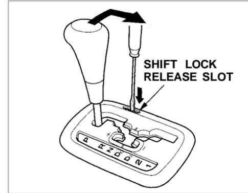
6. Remove the screwdriver from the shift lock release slot, then install a new cover.
