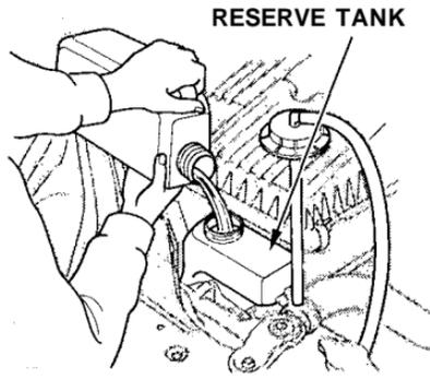
4. The coolant level should be up to the base of the filler neck. Add coolant if it is low.
