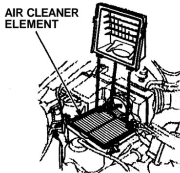
2. Remove the old air cleaner element. Carefully clean the inside of the air cleaner housing with a damp rag.
