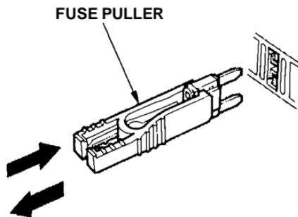
4. Check the smaller fuses in the under-hood fuse box and all the fuses in the interior fuse box by pulling out each fuse with the fuse puller provided in the interior fuse box.
