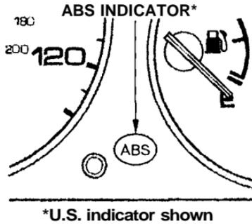
The ABS is self-checking. If anything goes wrong, the ABS indicator on the instrument panel comes on (see page 55 ). This means the anti-lock function of the braking system has shut down. The brakes still work like a conventional system without anti-lock, providing normal stopping ability. You should have the dealer inspect your car as soon as possible if this light stays on after you start the engine, or comes on while driving.
