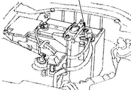
Check the battery condition by looking at the test indicator window on the battery. The label on the battery explains the test indicator's colors.
