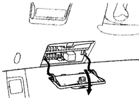
The interior fuse box is underneath the dashboard on the driver's side. Remove the fuse box lid by swinging the lid down and pulling it straight out of its hinges.
