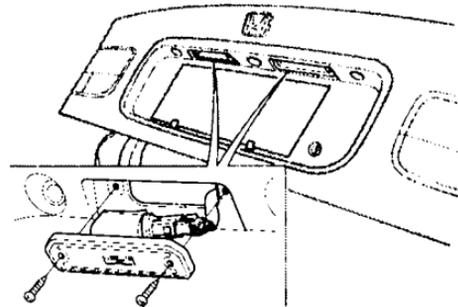
1. Remove the two screws and remove the license light assembly.
