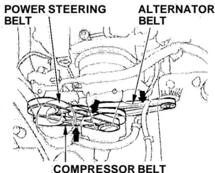
Check the condition of the two or three drive belts. Examine the edges of each belt for cracks or fraying. Check the tension of each belt by pushing on it with your thumb midway between the pulleys.
