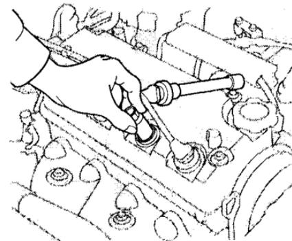
4. Put the new spark plug into the socket; then screw it into the hole. Screw it in by hand so you do not crossthread it.
