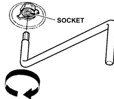
5. Insert the moonroof wrench into the socket behind this plug. Turn the wrench until the moonroof is fully closed.
