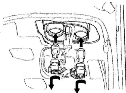
3. Determine which of the two bulbs is burned out: stop/taillight/side marker or back-up light.
