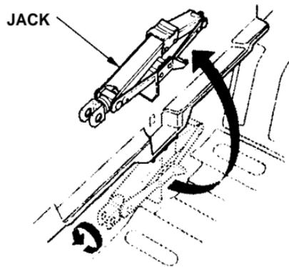
6. Turn the jack's end bracket counterclockwise to loosen it, then remove the jack.
