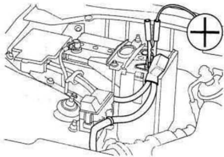
3. Connect one jumper cable to the positive (+) terminal on the booster battery. Connect the other end to the positive (+) terminal on your Honda's battery.
