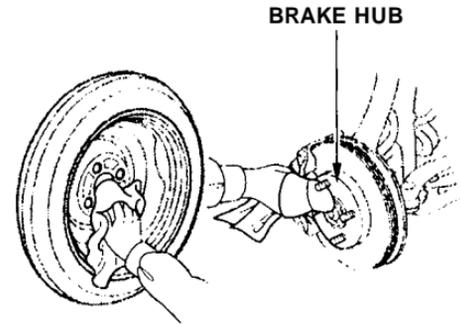
11. Before mounting the spare tire, wipe any dirt off the mounting surface of the wheel and hub with a clean cloth. Wipe the hub carefully, it may be hot from driving.
