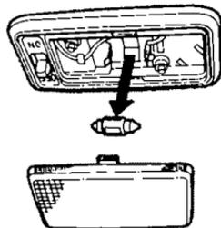
1. Remove the lens by carefully prying on the edge of the lens in the middle with a fingernail file or a small flat-tip screwdriver. Do not pry on the edge of the housing around the lens.
