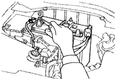
If the terminals are severely corroded, clean them with baking soda and water. Then use a wrench to loosen and remove the cables from the terminals. Always disconnect the negative ( — ) cable first and reconnect it last. Clean the battery terminals with a terminal cleaning tool or wire brush. Reconnect and tighten the cables, then coat the terminals with grease.
