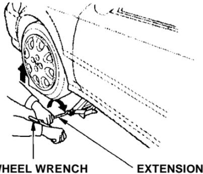
9. Use the extension and wheel wrench as shown to raise the vehicle until the flat tire is off the ground.
