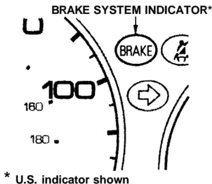
The Brake System indicator light should normally come on only when the parking brake is not fully released.
