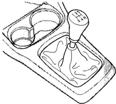
The manual transmission is synchronized in all forward gears for smooth operation. It has a lockout so you cannot shift directly from Fifth to Reverse. When shifting up or down, make sure you push the clutch pedal down all the way, shift to the next gear, and let the pedal up gradually. When you are not shifting, do not rest your foot on the clutch pedal. This can cause your clutch to wear out faster.
