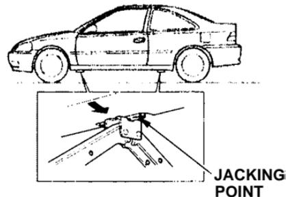
8. Locate the jacking point nearest the tire you need to change. It is pointed to by an arrow molded into the underside of the body. Place the jack under the jacking point. Turn the end bracket clockwise until the top of the jack contacts the jacking point. Make sure the jacking point tab is resting in the jack notch.
