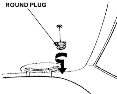
4. Use a screwdriver or coin to remove the round plug in the center of the headliner.
