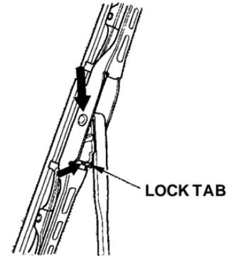
2. Disconnect the blade assembly from the wiper arm by pushing in the lock tab. Hold it in while you push the blade assembly toward the base of the arm.
