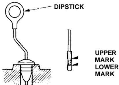
2. Remove the dipstick (yellow loop) from the transmission and wipe it with a clean cloth.
