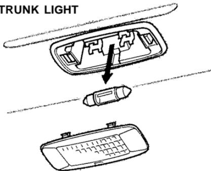
1. Remove the lens by carefully prying on the edge of the lens in the middle with a fingernail file or a small flat-tip screwdriver. Do not pry on the edge of the housing around the lens.
