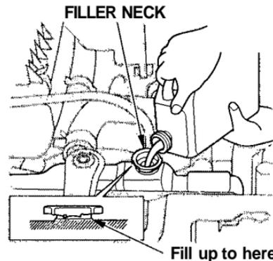
7. Pour coolant into the radiator up to the base of the filler neck. Start the engine and let it run for about 30 seconds. Then turn off the engine.
