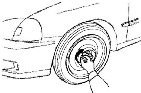
12. Put on the spare tire. Put the wheel nuts back on finger-tight, then tighten them in a crisscross pattern with the wheel wrench until the wheel is firmly against the hub. Do not try to tighten them fully.
