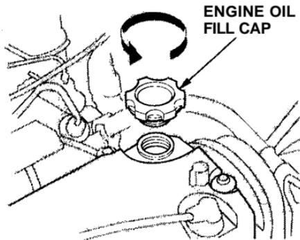
To add oil, unscrew and remove the engine oil fill cap on top of the valve cover. Pour in the oil, and reinstall the engine oil fill cap. Tighten it securely. Wait a few minutes and recheck the oil level. Do not fill above the upper mark; you could damage the engine.
