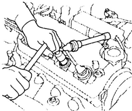
5. Torque the spark plug. (If you do not have a torque wrench, tighten the spark plug two-thirds of a turn after it contacts the cylinder head.)
