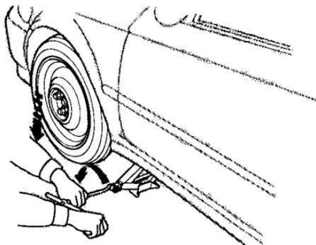
13. Lower the car to the ground and remove the jack.
