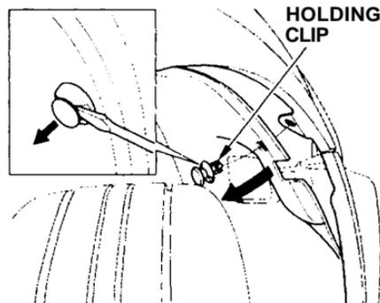
1. If you are changing the bulb on the driver's side, start the engine, turn the steering wheel all the way to the right, and turn off the engine. If you are changing the bulb on the passenger's side, turn the steering wheel to the left.
