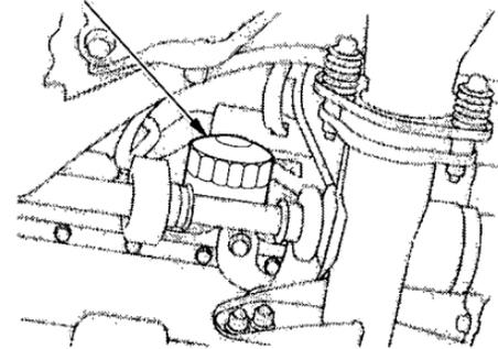
3. Remove the oil filter and let the remaining oil drain. A special wrench (available from your Honda dealer) is required to remove the filter.
