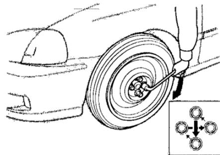
14. Tighten the wheel nuts securely in the same crisscross pattern. Have the wheel nut torque checked at the nearest automotive service facility.
