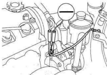
4. Connect the second jumper cable to the negative (-) terminal on the booster battery. Connect the other end to the grounding strap as shown. Do not connect this jumper cable to any other part of the engine.
