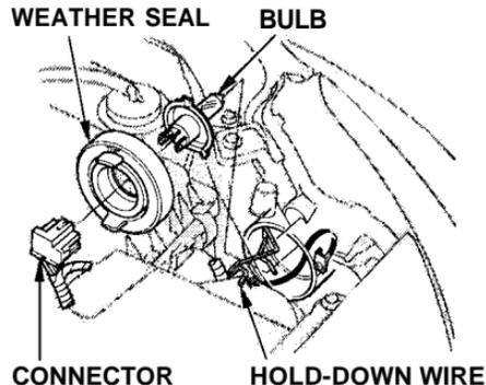
2. Remove the electrical connector from the bulb by squeezing the connector on both sides to unlock the tab. Pull the connector straight off.
