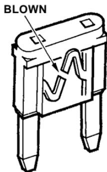
5. Look for a burned wire inside the fuse. If it is burned, replace it with one of the spare fuses of the same rating or lower.
