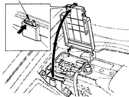
The under-hood fuse box is located in the engine compartment next to the battery. To open it, push the tab as shown.
