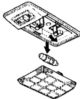
2. Remove the bulb by pulling it straight out of its metal tabs.
