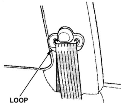
Dirt build-up in the loops of the seat belt anchors can cause the belts to retract slowly. Wipe the insides of the loops with a clean cloth dampened in mild soap and warm water or isopropyl alcohol.
