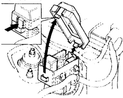
Vehicles equipped with ABS have a third fuse box for the ABS. It is in the engine compartment on the passenger's side.
