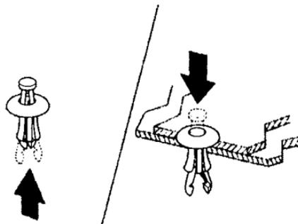
8. Reset the fastener by pushing on the pointed end until it pops back almost flush with the fingers on the housing.
