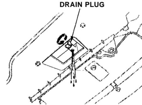
3. Loosen the drain plug on the bottom of the radiator. The coolant will come out through the hole in the splash cover.
