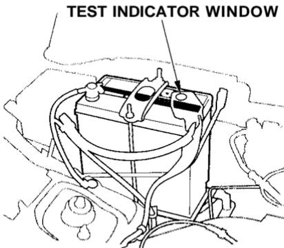
Check the battery condition by looking at the test indicator window on the battery. The label on the battery explains the test indicator's colors.
