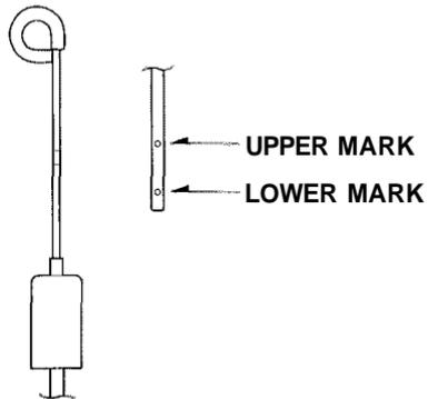
4. Remove the dipstick again and check the level. It should be between the upper and lower marks.
