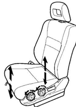
The height of your driver's seat is adjustable. Turn the front dial on the outside of the seat cushion to raise the front of the seat bottom and turn the rear dial to raise the rear.
