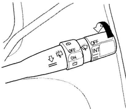
The right lever controls the windshield wipers and washers. The rotary switch at the end of the lever has three positions:
