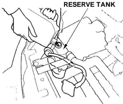
If the coolant level in the reserve tank is at or below the MIN line, add coolant to bring it up to the MAX line. Inspect the cooling system for leaks. This coolant should always be a mixture of 50 percent antifreeze and 50 percent water. Never add straight antifreeze or plain water.
