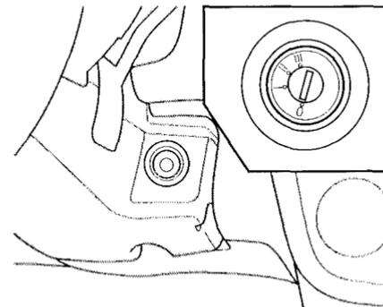
The ignition switch is on the right side of the steering column. It has four positions:
