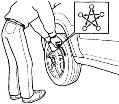
20. Tighten the wheel nuts securely in the same crisscross pattern. Have the wheel nut torque checked at the nearest automotive service facility.
