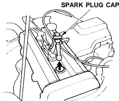
1. Clean up any dirt and oil around the spark plug caps.
