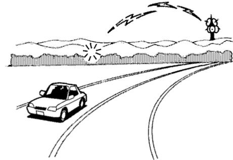
Driving very near the transmitter of a station that is broadcasting on a frequency close to the frequency of the station you are listening to can also affect your radio's reception. You may temporarily hear both stations, or hear only the station you are close to.
