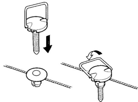
29. Replace the cargo storage bin. Secure it with the four clips. Push each clip down securely, and pivot the ring down flat.
