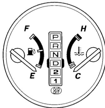
This indicator on the instrument panel shows which position the shift lever is in.
