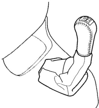
The manual transmission is synchronized in all forward gears for smooth operation. It has a lockout so you cannot shift directly from Fifth to Reverse. When shifting up or down, make sure you push the clutch pedal down all the way, shift to the next gear, and let the pedal up gradually. When you are not shifting, do not rest your foot on the clutch pedal. This can cause your clutch to wear out faster.
