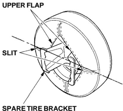
26. Pull the bottom of the cover over the tire, and make sure the two slits on the lower flaps of the cover are horizontal and the two upper flaps touch the spare tire bracket.
