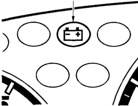
This indicator should come on when the ignition switch is ON (II), and go out after the engine starts. If it comes on brightly when the engine is running, it indicates that the charging system has stopped charging the battery.
