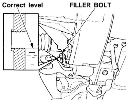
Check the fluid level with the transmission at normal operating temperature and the vehicle sitting on level ground. Remove the transmission filler bolt and carefully feel inside the bolt hole with your finger. The fluid level should be up to the edge of the bolt hole. If it is not, add Genuine Honda Manual Transmission Fluid (MTF) until it starts to run out of the hole. Reinstall the filler bolt and tighten it securely.
