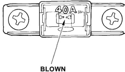
3. Check each of the large fuses in the under-hood fuse box by looking through the top at the wire inside. Removing these fuses requires a Phillips-head screwdriver.
