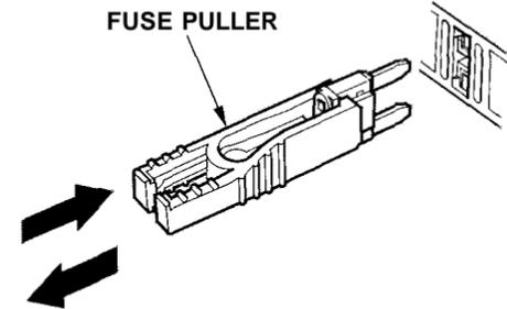
4. Check the smaller fuses in the under-hood fuse box and all the fuses in the interior fuse box by pulling out each fuse with the fuse puller provided in the door of the interior fuse box.
