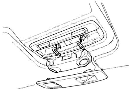
2. Remove the bulb by pulling it straight out of its metal tabs.
