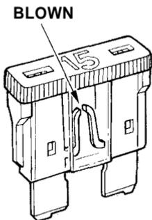
5. Look for a burned wire inside the fuse. If it is burned, replace it with one of the spare fuses of the same rating or lower.
