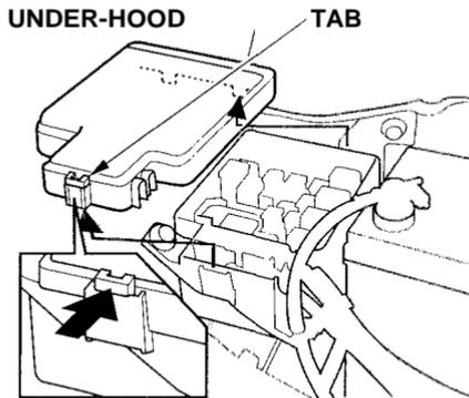
All the electrical circuits in your vehicle have fuses to protect them from a short circuit or overload. These fuses are located in two or three fuse boxes.
