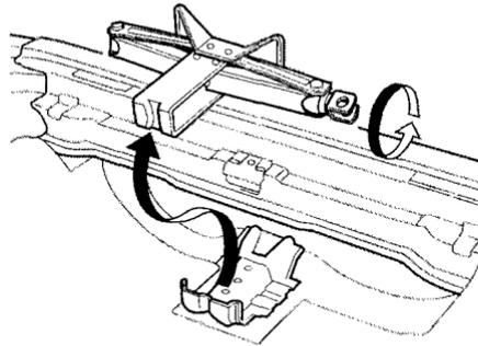
6. Turn the jack's end bracket counterclockwise to loosen it, then remove the jack by lifting it straight up.
