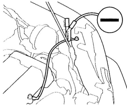
4. Connect the second jumper cable to the negative (-) terminal on the booster battery. Connect the other end to the ground wire on the right side of the engine as shown. Do not connect this jumper cable to any other part of the engine.
