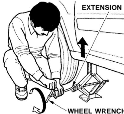
15. Use the extension and wheel wrench as shown to raise the vehicle until the flat tire is off the ground.
