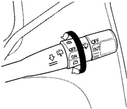
The rear window wiper switch is located next to the windshield wiper switch.
