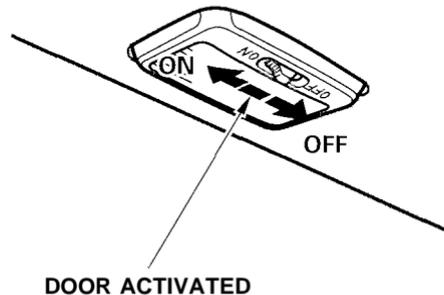
The cargo area light has a three-position switch. In the OFF position, the light does not come on. In the center position, the light comes on when you open the tailgate. In the ON position, the light stays on continuously.
