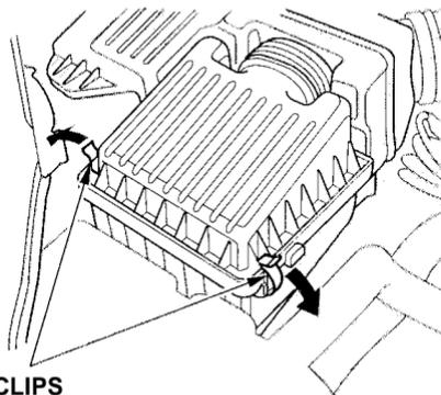
The air cleaner element is inside the air cleaner housing on the right side of the engine compartment.
