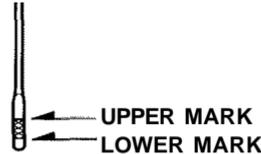
3. Insert the dipstick all the way into the transmission.
