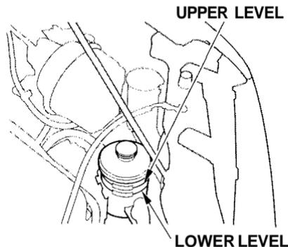
Check the level when the engine is cold. Look at the side of the reservoir. The fluid should be between the UPPER LEVEL and LOWER LEVEL. If it is below the LOWER LEVEL, add power steering fluid to the UPPER LEVEL.
