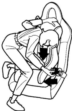
5. After confirming that the belt is locked, grab the shoulder part of the belt near the buckle and pull up to remove any slack from the lap part of the belt. Remember, if the lap part of the belt is not tight, the child seat will not be secure. It may help to put weight on the child seat, or push on the back of the seat, while pulling up on the belt.
