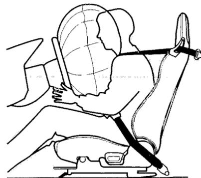
If you ever have a moderate to severe frontal collision, the sensors will detect rapid deceleration and signal the control unit to instantly inflate the airbags and activate the automatic seat belt tensioners.
