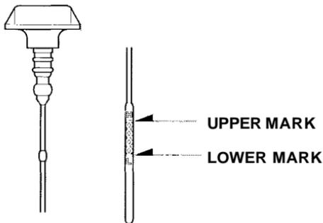
4. Remove the dipstick again and check the level. It should be between the upper and lower marks.
