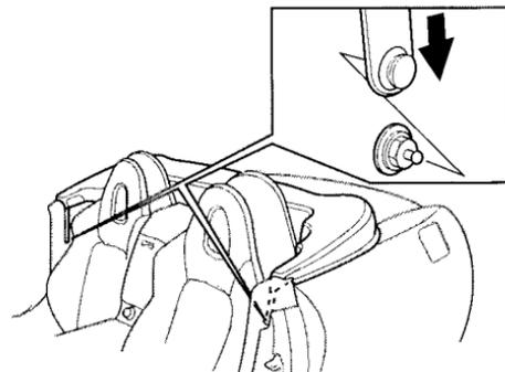
3. Hook the fastener string to the pin on each side wall of the passenger compartment.
