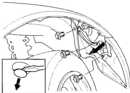
2. Use a flat-tipped screwdriver to remove the three holding clips from the inner fender.
