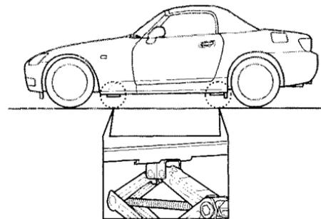
7. Locate the jacking point nearest the tire you need to change. It is pointed to by an arrow molded into the underside of the body. Place the jack under the jacking point. Turn the end bracket clockwise until the top of the jack contacts the jacking point. Make sure the jacking point tab is resting in the jack notch.
