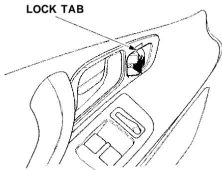
Each door has a lock tab next to the inside door handle. When you push in the lock tab on the driver's door, both doors lock. Pulling out the lock tab on the driver's door only unlocks that door. The lock tab on the passenger's door only locks and unlocks that door.
