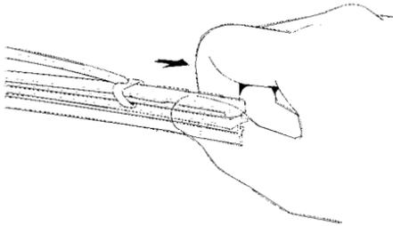
3. Remove the blade from its holder by grasping the tabbed end of the blade. Pull firmly until the tabs come out of the holder.
