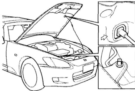
3. Pull the support rod out of its clip and insert the end into the hole on the front of the hood around the center.
