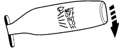
This lever controls the windshield wipers and washers. It has five positions;
