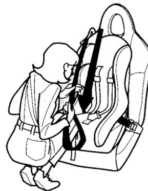
3. To activate the lockable retractor, slowly pull the shoulder part of the belt all the way out until it stops, then let the belt feed back into the retractor (you might hear a clicking noise as the belt retracts).
