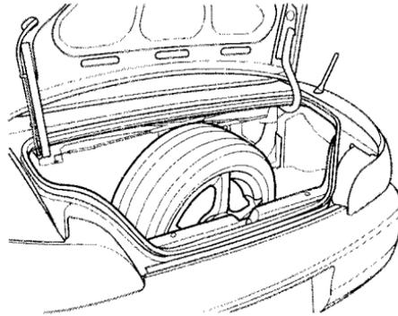
16. Replace the spare tire cover. Secure it with the three clips. Push each clip down securely, and pivot the ring down flat.
