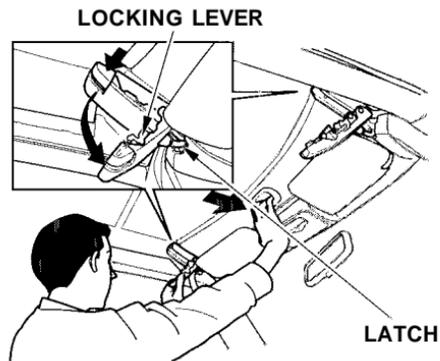
4. Push the top forward while you release the latches from the windshield header by pushing the locking levers forward.
