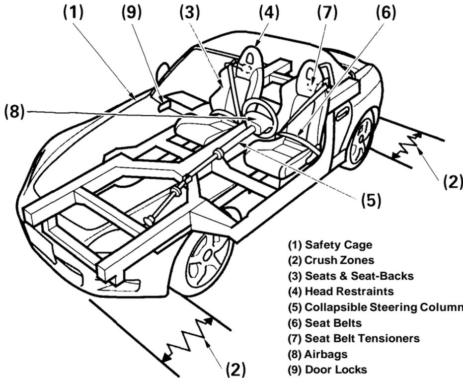
Your car is equipped with many features that work together to protect you and your passenger during a crash.
