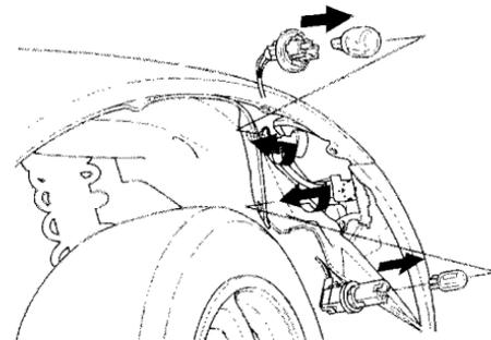
6. Install the new bulb in the socket.
