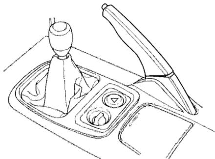
To apply the parking brake, pull the lever up fully. To release it, pull up slightly, push the button, and lower the lever. The parking brake light on the instrument panel should go out when the parking brake is fully released (see page 44). If you try to drive the vehicle without releasing the parking brake, the ABS indicator may come on, and the ABS may not work properly.
