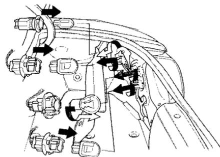
5. Remove the socket by turning it one-quarter turn counterclockwise.
