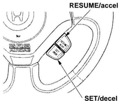
3. Press and release the SET/deccl button on the steering wheel. The CRUISE CONTROL light on the instrument panel comes on to show the system is now activated.
