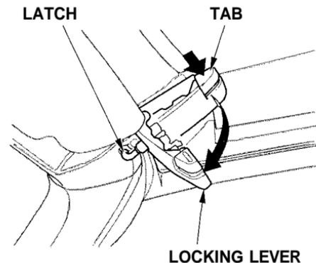
3. There is a latch on each side. Push in the tab and pull the locking lever down.
