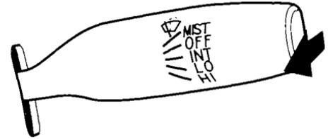
To clean the windshield, pull back on the wiper control lever. The washers spray until you release the lever.
