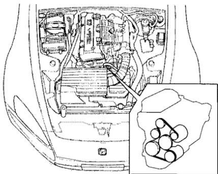
You should check the condition of the drive belt every 2 years. Examine the edges of belt for cracks or fraying.
