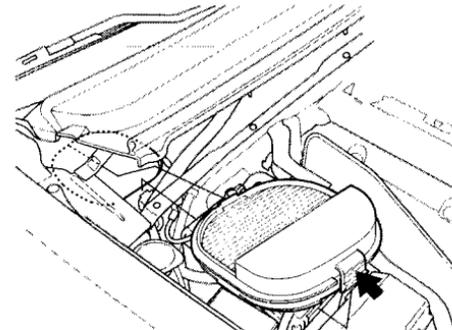
2. Push the tab on the air conditioning filter to unlock it from the holder.
