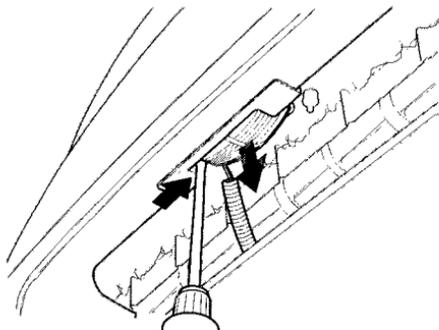
1. Insert a flat blade screwdriver between the left edge of the lens and the housing. The lens will come down.
