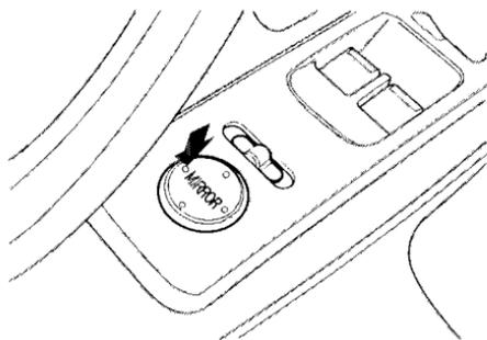
3. Push the appropriate edge of the adjustment switch to move the mirror right, left, up or down.
