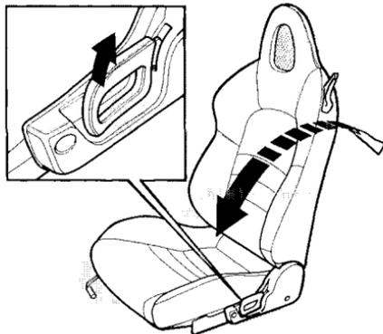
To change the angle of the seat-back, pull up on the lever on the outside of the seat bottom. Move the seat-back to the desired position and release the lever. Let the seat-back latch in the new position.
