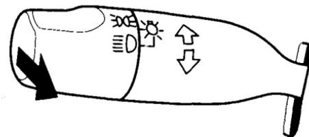
To flash the high beams, pull the turn signal lever back lightly, then release it. The high beams will come on and go off. The high beams will stay on for as long as you hold the lever back, no matter what position the headlight switch is in.
