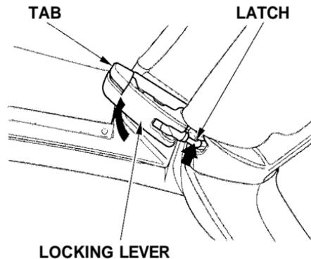
5. Push in the tab on each locking lever and pull the locking lever down.
