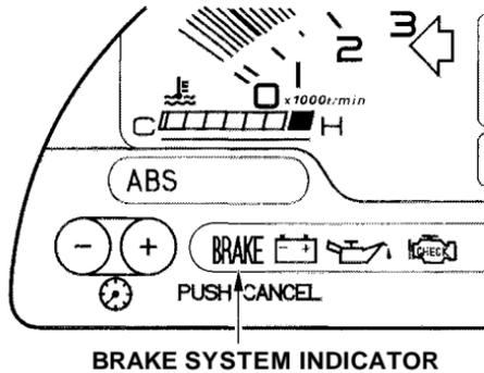
The Brake System Indicator light comes on when you turn the ignition ON (II). If the parking brake is not set, it goes off after you start the engine. If the parking brake is set, it goes off when you fully release the parking brake with the engine running.
