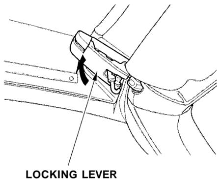
5. With the latches released, pull back on the locking levers and push them up until they latch.
