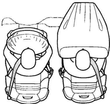
Your car has a Supplemental Restraint System (SRS) with frontal airbags to help protect the driver and a passenger.
