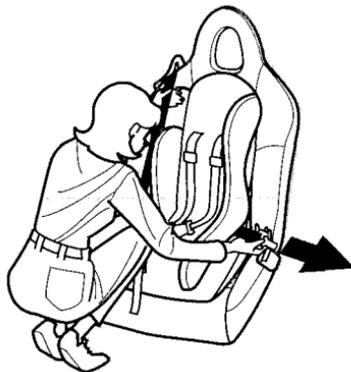
2. With the child seat in position, route the belt through the child seat according to the seat maker's instructions, then insert the latch plate into the buckle.
