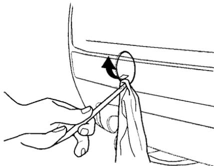
For very short distances, such as freeing the car, you can use the detachable towing hook that mounts on the anchors in the front and rear bumpers.
