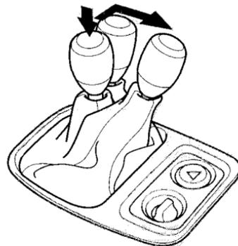
The 6-speed manual transmission has a lockout so you cannot accidentally shift from Fifth to Reverse instead of Sixth.
