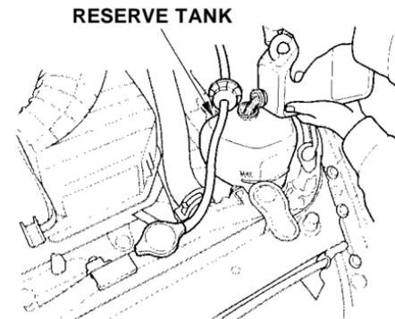
11. Fill the reserve tank to the MAX mark. Install the reserve tank cap.
