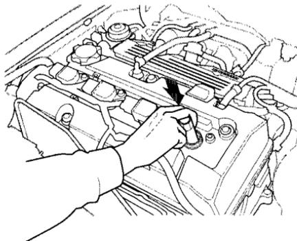
5. Put the new spark plug into the socket; then screw it into the hole. Screw it in by hand so you do not crosstread it.
