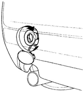
4. Screw the towing hook into the extension and tighten it securely by hand.
