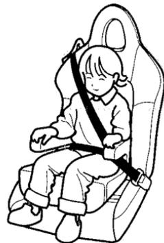
If a child needs a booster seat, we recommend choosing a style that allows the child to use the lap/shoulder belt directly, without a shield, as shown.
