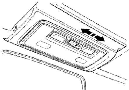
The interior light has a three-position switch. In the OFF position, the light does not come on. In the center position, the interior light comes on when you open either door. In the ON position, the interior light stays on continuously.
