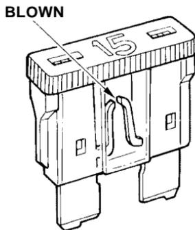
5. Look for a burned wire inside the fuse. If it is burned, replace it with one of the spare fuses of the same rating or lower.
