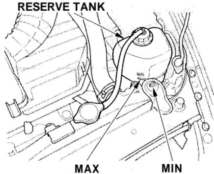
If the coolant level in the reserve tank is at or below the MIN line, add coolant to bring it up to the MAX line. Inspect the cooling system for leaks. This coolant should always be a mixture of 50 percent antifreeze and 50 percent water. Never add straight antifreeze or plain water.
