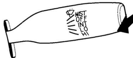
To clean the windshield, pull back on the wiper control lever. The washers spray until you release the lever.
