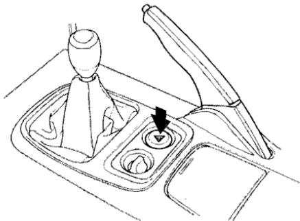
Push the red button next to the roof switch to turn on the hazard warning lights (four-way flashers). This causes all four outside turn signals and both indicators in the instrument panel to flash. Use the hazard warning lights if you need to park in a dangerous area near heavy traffic, or if your vehicle is disabled.
