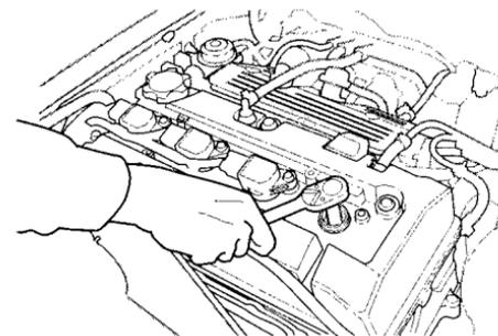
6. Torque the spark plug. (If you do not have a torque wrench, tighten the spark plug two-thirds of a turn after it contacts the cylinder head.) Tightening torque:
