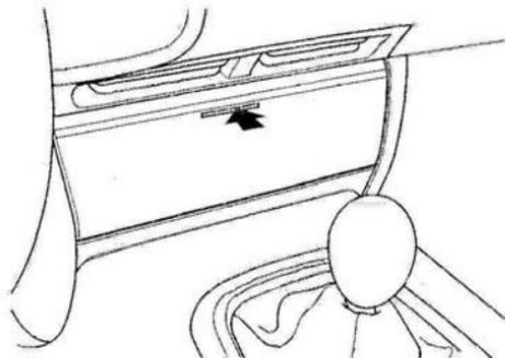
To open the audio panel, push on the top center and let the panel swing down. To close, pivot the panel up and push on it until it latches. Refer to page [94](#) for operation of the audio system.
