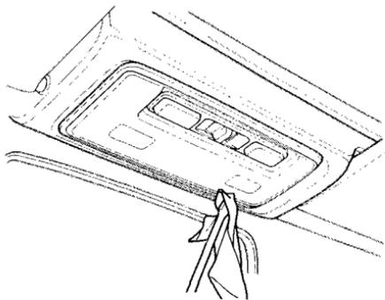
1. Remove the lens by carefully prying on the front edge of the lens near both sides.
