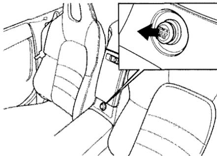
To use the accessory power socket, pull out on the cover. The ignition switch must be in ACCESSORY (I) or ON (II).
