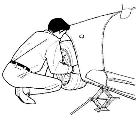
9. Remove the wheel nuts and flat tire. Temporarily place the flat tire on the ground with the outside surface of the wheel facing up. Placing the wheel face down could mar its finish.
