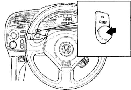
CRUISE CONTROL light comes on. The car will accelerate to the same cruising speed as before.
