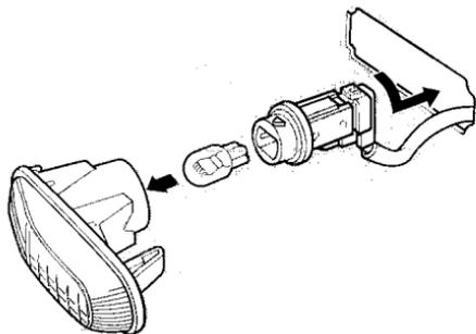
1. Push the side turn signal assembly forward until it pops out of the body.
