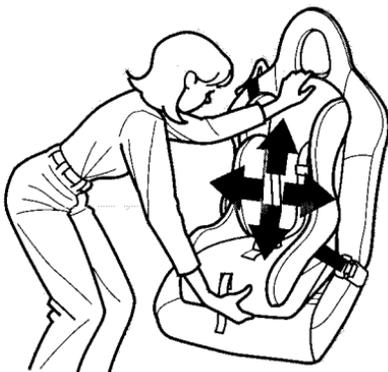
6. Push and pull the child seat forward and from side to side to verify that it is secure enough to stay upright during normal driving maneuvers. If the child seat is not secure, unlatch the belt, allow it to retract fully, then repeat these steps.
