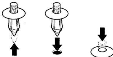
10. Install the trunk lining and secure it with the fasteners. To reinstall a fastener, reset the fastener by pushing on the pointed end until it pops back almost flush with the fingers on the housing. Put the fastener in the hole of the trunk lining and push on the center until it locks (the center is flush with the head).
