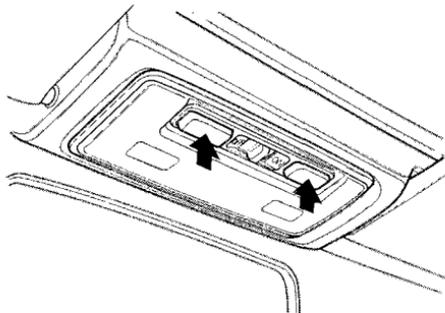
In addition, when the three position switch is in the center position with both doors closed, the two bulbs in the interior light can be turned on separately by the pushbutton switches next to them. Push the switch to turn the light on or off.
