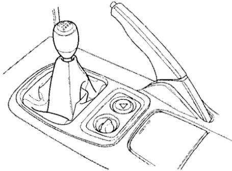
The manual transmission is synchronized in all forward gears for smooth operation. It has a lockout so you cannot shift directly from Fifth to Reverse instead of sixth (see page 134). When shifting up or down, make sure you push the clutch pedal down all the way, shift to the next gear, and let the pedal up gradually. When you are not shifting, do not rest your foot on the clutch pedal. This can cause your clutch to wear out faster.
