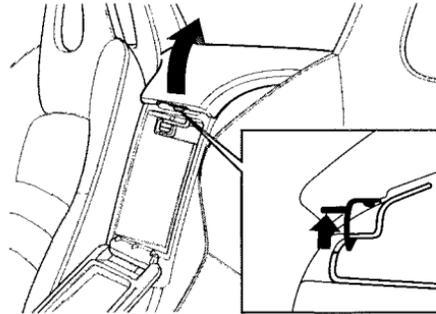
The lever to open the upper compartment is inside the lower compartment. Push up the lever and lift the lid. To close, lower the lid and push it down until it latches.
