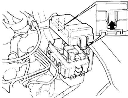
The auxiliary fuse box is located on the driver's side near the brake fluid reservoir. To open it, push the tab on each side and remove the lid.
