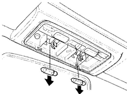
2. Remove the bulb by pulling it straight out of its metal tabs.
