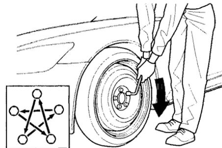
13. Tighten the wheel nuts securely in the same crisscross pattern. Have the wheel nut torque checked at the nearest automotive service facility.
