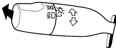
To change from low beams to high beams, push the turn signal lever forward until you hear a click. The blue high beam indicator will light (see page 46). To return to low beams, pull the turn signal lever back.
