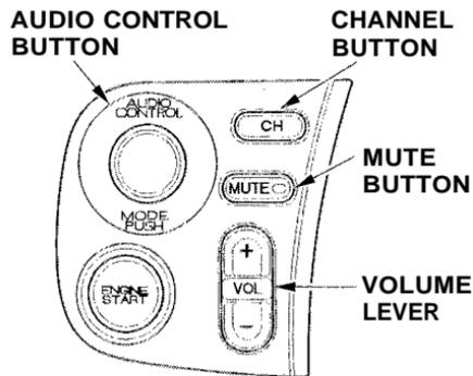
Four controls for the audio system are on the left side of the dashboard by the instrument panel. These let you control basic functions without distracting your attention from driving.
