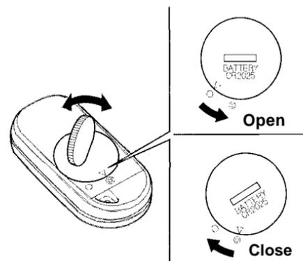
To replace the battery, remove the round cover on the back of the transmitter by turning it counterclockwise with a coin.
