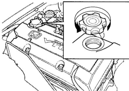
To add oil, unscrew and remove the engine oil fill cap on top of the left valve cover. Pour in the oil, and replace the engine oil fill cap. Tighten it securely. Wait a few minutes and recheck the oil level. Do not fill above the upper mark; you could damage the engine.
