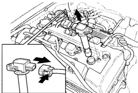
3. Remove the bolt holding the ignition coil and pull the ignition coil straight up slightly. Disconnect the ignition coil connector by pushing the tab and pulling the connector back. Pull the ignition coil all the way up.
