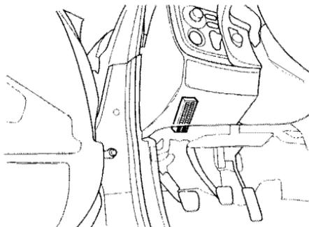
The interior fuse box is underneath the dashboard on the driver's side.
