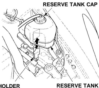
5. Remove the reserve tank from its holder by pulling it straight up. Drain the coolant, then put the tank back in its holder.
