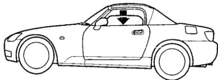
The windows will lower and the roof will fold back. Release the ROOF switch when the roof is retracted completely into the rear shelf.
