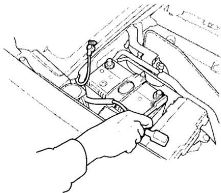
If the terminals are severely corroded, clean them with baking soda and water. Then use a wrench to loosen and remove the cables from the terminals. Always disconnect the negative (—) cable first and reconnect it last. Clean the battery terminals with a terminal cleaning tool or wire brush. Reconnect and tighten the cables, then coat the terminals with grease.
