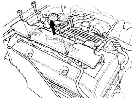
1. Remove the four hexagon socket head cap bolts holding the ignition coil cover.
