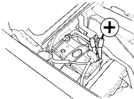
3. Connect one jumper cable to the positive (+) terminal on the booster battery. Connect the other end to the positive (+) terminal on your Honda's battery.
