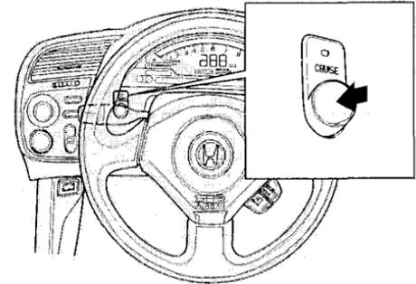
1. Push in the Cruise Control Master Switch on the dashboard beside the steering column. The indicator by the switch will light.
