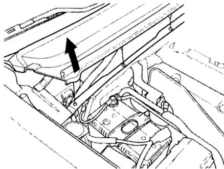
The air conditioning filter is located in the engine compartment on the passenger's side near the base of the windshield.
