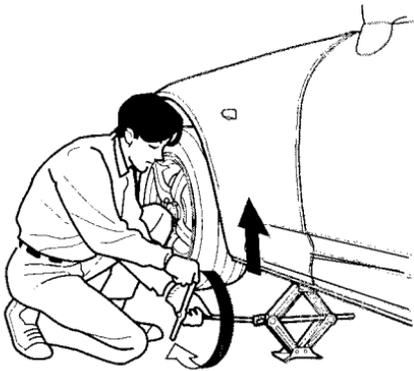
8. Use the extension and wheel wrench as shown to raise the car until the flat tire is off the ground.
