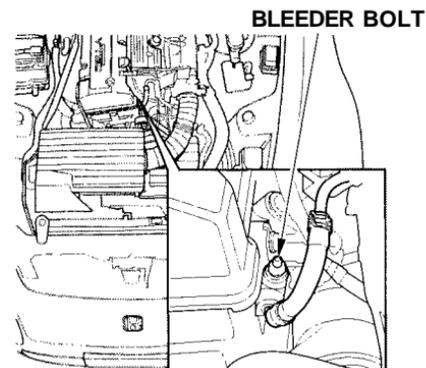
8. Loosen the bleeder bolt on top of the engine, and remove the bleeder cap near the engine oil fill cap. Pour coolant into the radiator up to the base of the filler neck. Tighten the bleeder bolt and reinstall the bleeder cap when coolant comes out in a steady stream with no bubbles.
