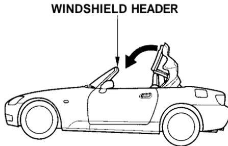
The convertible top will raise. Release the ROOF switch when the top reaches the windshield header.
