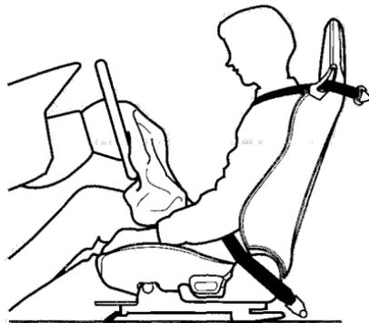
After inflating, the airbags immediately deflate, so they won't interfere with the driver's visibility, or the ability to steer or operate other controls.
