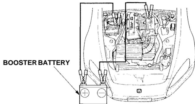
6. Start your car. If the starter motor still operates slowly, check the jumper cable connections to make sure they have good metal-to-metal contact.
