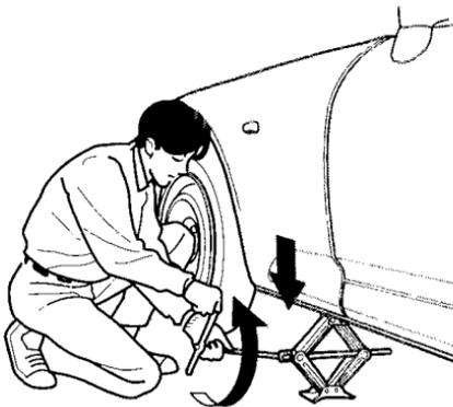
12. Lower the car to the ground and remove the jack.
