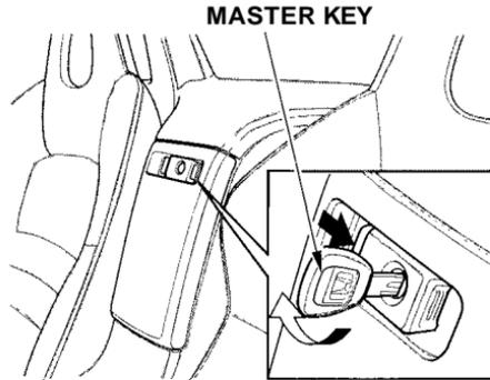
The area between the seats has two compartments. Open the lower compartment by squeezing the handle. Close it with a firm push. You can lock or unlock the lower compartment with the master key.
