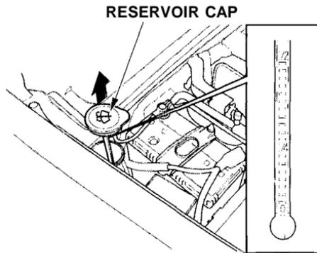
Check the reservoir's fluid level by removing the cap and looking at the level gauge attached to the cap.
