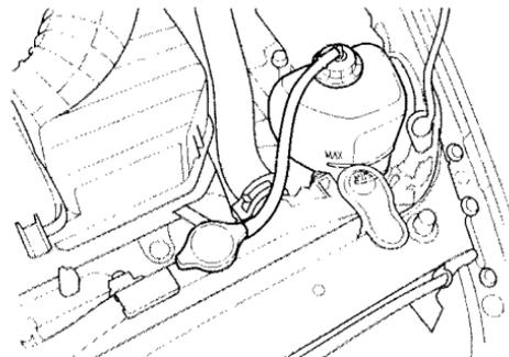
Look at the coolant level in the radiator reserve tank. Make sure it is between the MAX and MIN lines. If it is below the MIN line, see **Adding Engine Coolant** on page 161 for information on adding the proper coolant.
