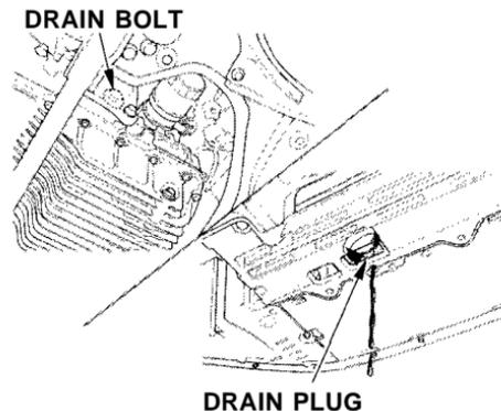
4. Loosen the drain plug on the bottom of the radiator. The coolant will drain through the splash guard. Remove the drain bolt and washer from the engine block.
