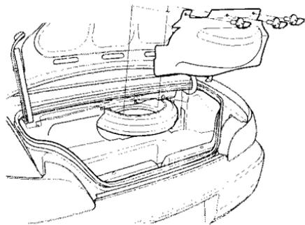
4. Remove the three clips holding the spare tire cover by pulling straight up on the rings. Remove the spare tire cover.
