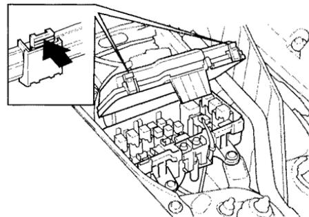
There are two under-hood fuse boxes in the engine compartment.
