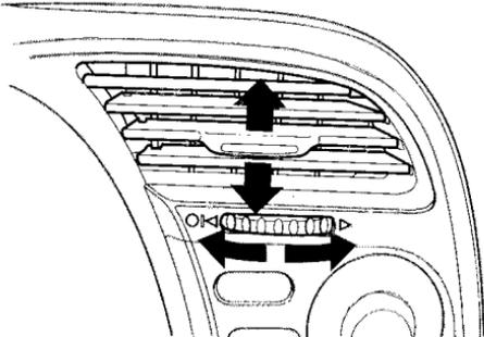
You can adjust the direction of the air coming from the vents on both sides of the instrument panel and at the corner of the dashboard on the passenger's side. To adjust the air flow up and down, move the tab in the center of each vent up and down. To adjust it left and right, turn the dial under each vent left and right.
