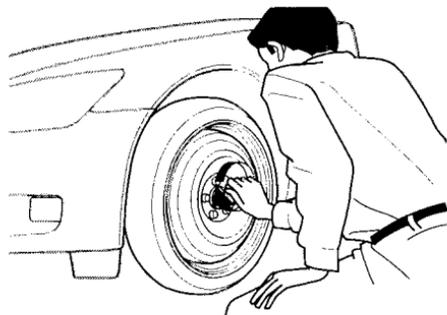
11. Put on the spare tire. Put the wheel nuts back on finger-tight, then tighten them in a crisscross pattern with the wheel wrench until the wheel is firmly against the hub. Do not try to tighten them fully.
