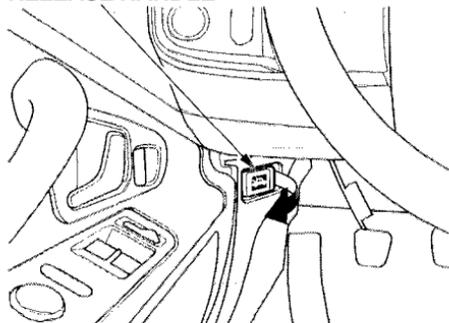
1. Shift to Neutral and set the parking brake. Pull the hood release handle located under the lower left corner of the dashboard. The hood will pop up slightly.
