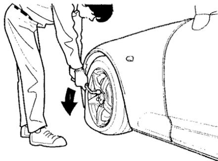
5. Unscrew the wing bolt and take the spare tire out of the spare tire shelf.
