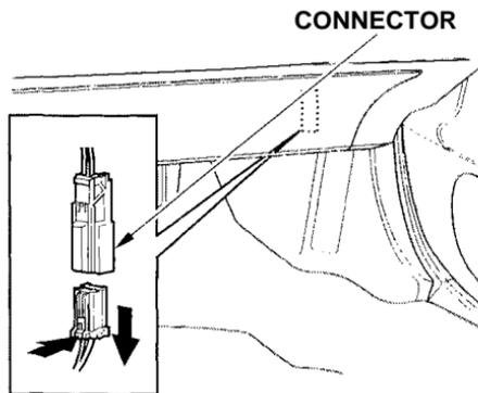
3. Locate the electrical connector for the convertible top motor. It is under the lower corner of the dashboard on the passenger's side. Disconnect the connector by pushing the tab and pulling the connector down.
