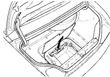
3. Open the trunk. Lift up the tool box lid and take the jack, wheel wrench and extension out of the tool box.
