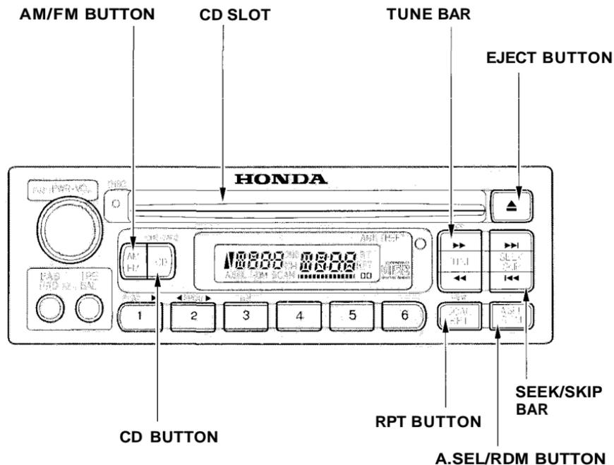
You can switch to the radio while a CD is playing by pressing the AM/FM button. Press the CD button to return to playing the CD. The CD will begin playing where it left off.
