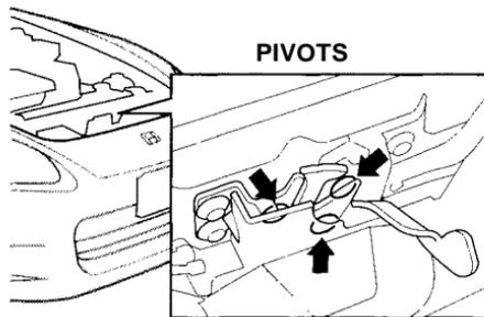
Clean the hood latch assembly with a mild cleaner, then lubricate it with a multipurpose grease. Lubricate all the moving parts, including the pivot. Follow the time and distance recommendations in the Maintenance Schedule. If you are not sure how to clean and grease the latch, contact your Honda dealer.
