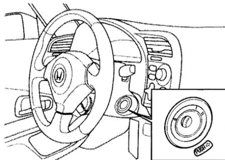
The ignition switch is on the right side of the steering column. It has three positions:
