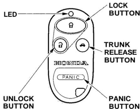
You can lock and unlock your car with the remote transmitter. When you push the LOCK button, both doors lock. The side marker lights and taillights flash once.
