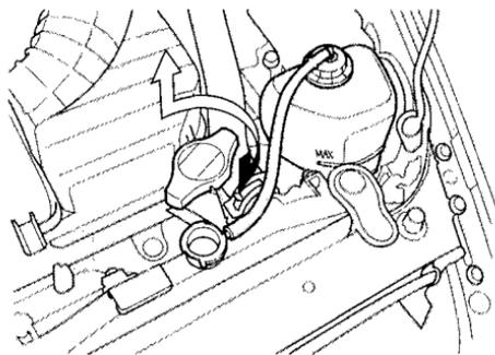
1. Turn the ignition ON (II). Turn the heater temperature control dial fully clockwise. Turn the ignition off.
