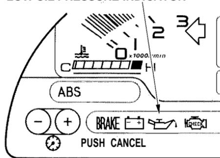
This indicator should light when the ignition switch is ON (II), and go out after the engine starts. It should never come on when the engine is running. If it starts flashing, it indicates that the oil pressure dropped very low for a moment, then recovered. If the indicator stays on with the engine running, it shows that the engine has lost oil pressure and serious engine damage is possible. In either case, you should take immediate action.
