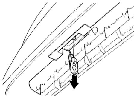
2. Pull the bulb straight out of its socket. Push the new bulb in until it bottoms in the socket.
