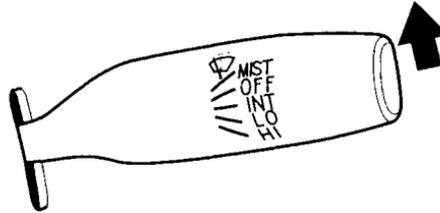
To operate the wipers in mist mode, push the control lever up from the OFF position. The wipers run at high speed until you release the lever. This gives you a quick way to clear the windshield.
