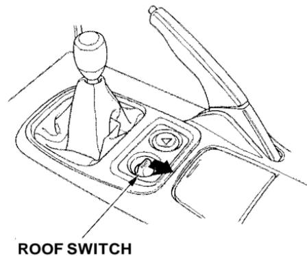
6. Pull back and hold the ROOF switch.
