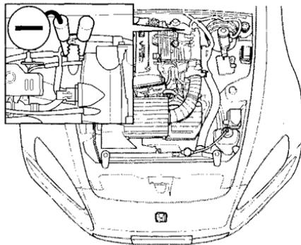
4. Connect the second jumper cable to the negative (—) terminal on the booster battery. Connect the other end to the metal projection near the intake manifold as shown in the illustration. Do not connect this jumper cable to any other part of the engine.
