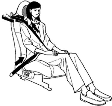
Your Honda has automatic seat belt tensioners for added protection during a moderate to severe frontal collision.
