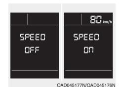
This message shows the speed of the vehicle (in km/h or mph).
