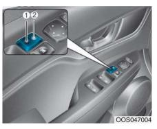
The driver side door armrest is equipped with a central door lock switch. The lock button is indicated by a  $(\widehat{r})$  symbol. The unlock button is indicated by a  $(\widehat{r})$  symbol.
