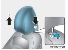
Adjusting the height up and down To raise the head restraint:
