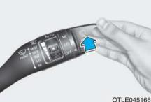
Push the lever away from you to sprav rear washer fluid and to run the rear wipers 1~3 cycles. The spray and wiper operation will continue until vou release the lever.
