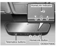
Your vehicle may be equipped with a Gentex Automatic-Dimming Mirror with a Z-Nav<sup>™</sup> Electronic Compass Integrated Display and an HomeLink® Wireless Control System. During nighttime driving, this feature will automatically detect and reduce rearview mirror glare while the compass indicates the direction the vehicle is traveling. The HomeLink<sup>®</sup> Universal Transceiver allows you to activate your garage door(s), electric gate, home lighting, etc.
