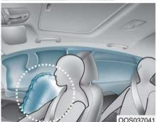
Your vehicle is equipped with a side air bag in each front seat. The purpose of the air bag is to provide the vehicle's driver and the front passenger with additional protection than that offered by the seat belt alone. The side air bags are designed to deploy during certain side impact collisions, depending on the crash severity.
