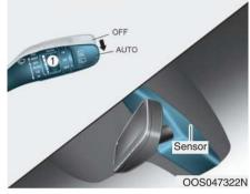
The rain sensor located on the upper end of the windshield glass senses the amount of rainfall and controls the wiping cycle for the proper interval.
