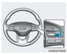
• Push the toggle switch up (RES+) and hold it, while monitoring the SET speed on the instrument cluster.
