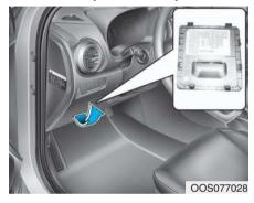
Inside the fuse/relay box cover, you can find the fuse/relay label describing fuse/relay names and ratings.
