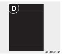
This indicator displays the gear position of the shift lever.
