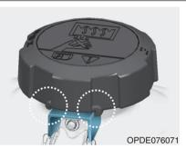
2. Make sure that the tiny protrusions inside the coolant cap is securely interlocked.
