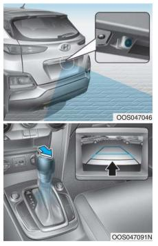
The rear view monitor will activate when the engine is running and the shift lever is in the R (Reverse) position. This is a supplemental system that helps provide a view of the area behind the vehicle through the audio display while the vehicle is in the R (Reverse) position.
