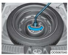
If it is hard to loosen the tire holddown wing bolt by hand, you can loosen it easily using the wheel nut wrench.
