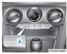
As a reminder to the front passenger, the front passenger's seat belt warning lights will illuminate for approximately 6 seconds each time you place the ignition switch to the ON position regardless of belt fastening.
