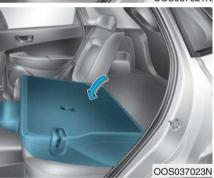
Put out the belt from guide (1) and pull up the seatback folding lever (2), then fold the seat toward the front of the vehicle.
