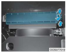
3. Remove the climate control air filter case while pressing the lock on the right side of the cover.
