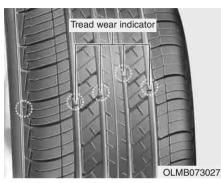
If the tire is worn evenly, a tread wear indicator will appear as a solid band across the tread. This shows there is less than 1.6 mm (2/32 inch) of tread left on the tire. Replace the tire when this happens.
