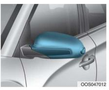
Make sure to adjust the side view mirrors to your desired position before you begin driving. Your vehicle is equipped with both left-hand and right-hand side view mirrors. The mirrors can be adjusted remotely with the remote switch. The side view mirrors can be folded to help prevent damage when going through an automatic car wash or when passing through a narrow street.
