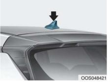
The shark fin antenna receives transmitted data. (for example: AM/FM, SXM, GPS, LTE)
