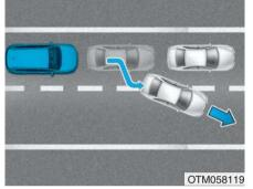
• When driving in stop-and-go traffic, and a vehicle in front of you merges out of the lane, the system may not immediately detect the new vehicle that is now in front of you. In this case, you must maintain a safe braking distance, and if necessary, depress the brake pedal to reduce your driving speed in order to maintain a safe distance.
