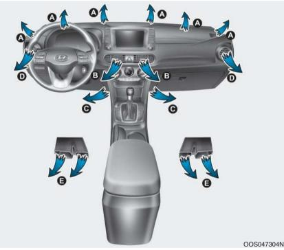
The mode selection knob controls the direction of the air flow through the ventilation system. Air can be directed to the floor, dashboard outlets, or windshield. Five symbols are used to represent Face, Bi-Level, Floor, Floor-Defrost and Defrost air position.
