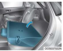
5. To use the rear seat, lift and unfold the seatback to the upright position. Push the seatback firmly until it clicks into place. Make sure the seatback is locked in place.
