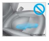
If large quantity of liquid has been spilled on the passenger seat, the air bag warning light may illuminate or malfunction.
