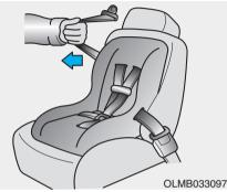
3. Pull the shoulder portion of the seat belt all the way out. When the shoulder portion of the seat belt is fully extended, it will shift the retractor to the "Automatic Locking" (child restraint) mode.
