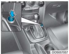
The All Wheel Drive (AWD) system delivers engine torque to both the front and rear wheels for extra traction. AWD is useful when maximum traction is required on slippery, muddy, wet, or snow-covered roads.
