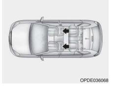
The vehicle's front and passenger's seats are equipped with adjustable head restraints for the passengers safety and comfort.
