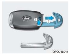
To remove the mechanical key from the smart key FOB, slide the release lever in the direction of the arrow (1) and then pull the mechanical key (2) outward.
