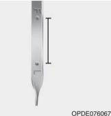
6. Pull the dipstick out again and check the level. The level should
