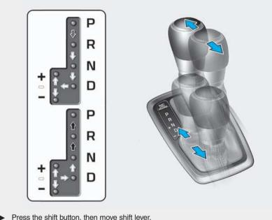
Depress the brake pedal, press the shift button, and then move shift lever. Move shift lever.
