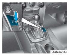
The Downhill Brake Control (DBC) feature assists the driver to descend down a steep hill without having to depress the brake pedal. The system automatically applies the brakes to maintain the vehicle speed below 8 km/h (5 mph) and allows the driver to concentrate on steering the vehicle down hill.
