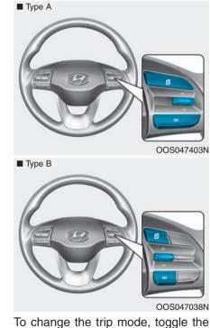
To change the trip mode, toggle the " $\land$ ,  $\checkmark$ " switch on the steering wheel.
