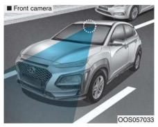
In order for the FCA system to operate properly, always make sure the camera is clean and free of dirt, snow, and debris. Dirt, snow, or foreign substances on the surface may adversely affect the sensing performance of the camera.
