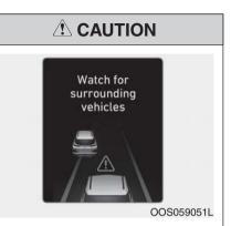
If the vehicle ahead (vehicle speed: less than 30 km/h (20 mph)) disappears to the next lane, the warning chime will sound and a message "Watch for surrounding vehicles" will appear. Adjust your vehicle speed for vehicles or objects that can suddenly appear in front of you by depressing the brake pedal.
