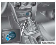
The power outlet is designed to provide power for mobile telephones or other devices designed to operate with vehicle electrical systems. The devices should draw less than 180 W with the engine running.
