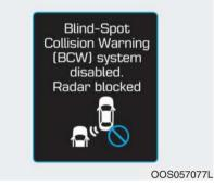
Blind-Spot Collision Warning (BCW) system disabled. Radar blocked
