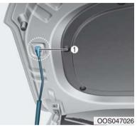
4. Pull out the support rod and hold the hood open with the support rod (1).
