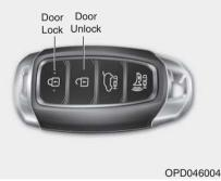
Press the button on the driver's outside door handle while carrying the Smart Key with you or press the Door Unlock button on the Smart Key, the driver's door will unlock.
