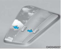
The sunshade can be opened and closed manually. However, the sunshade will open automatically with the sunroof glass when both the sunroof and sunshade are closed and the sunroof control lever is operated.
