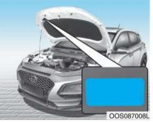
Air Conditioning refrigerant label You can find out which air conditioning refrigerant is applied to your vehicle on the label located inside of the hood.
