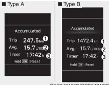
The accumulated driving information will continue to be counted while the engine is still running (for example, when the vehicle is in traffic or stopped at a stop light).
