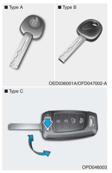
If the remote key does not operate normally, you can lock or unlock the driver's door by using the mechanical key.
