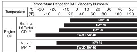
\*1 : For better fuel economy, it is recommended to use the engine oil of a viscosity grade 5W-30 (API Latest (ILSAC Latest) or ACEA A5 or above). However, if the engine oil is not available in your country, select the proper engine oil using the engine oil viscosity chart.
