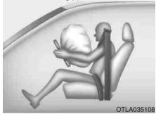
Upon deployment, tear seams molded directly into the pad covers will separate under pressure from the expansion of the air bags. Further opening of the covers allows full inflation of the air bags.
