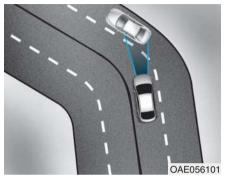
Forward Collision-Avoidance Assist system may recognize a vehicle or pedestrian in the next lane or outside the lane when driving on a curved road.
