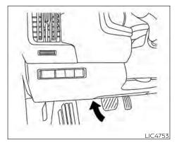
The extended storage switch is used when the vehicle is in transit from the factory. It is located above the brake pedal underneath the instrument panel. If any electrical equipment does not operate, ensure the extended storage switch is pushed fully in place, as shown.
