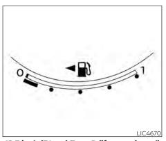
12.3 inch (31 cm) Type B (if so equipped) Refill the fuel tank before the gauge registers 0 (Empty).
