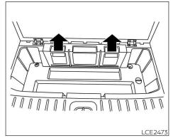
2. Remove the jack and tool kit cover by lifting up using the handles.
