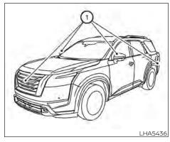
To display the multiple views, the Intelligent Around View Monitor system uses cameras located in the front grille, on the vehicle's outside mirrors and in the rear bumper 1).
