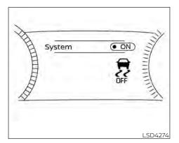
To turn off the VDC system, perform the following steps in the vehicle information display.
