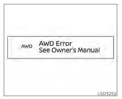
If any malfunction occurs in the I-4X4 system while the engine is running, messages are displayed in the meter.
