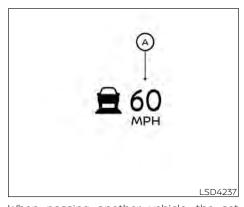
When passing another vehicle, the set speed indicator (A) flashes when the vehicle speed exceeds the set speed. The vehicle ahead detection indicator turns off when the area ahead of the vehicle is open. When the pedal is released, the vehicle returns to the previously set speed. Even though your vehicle speed is set in the ICC system, you can depress the accelerator pedal when it is necessary to accelerate vour vehicle rapidly.
