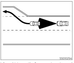
When driving on the freeway at a set speed and approaching a slower traveling vehicle ahead, the ICC system adjusts the speed to maintain the distance, selected by the driver, from the vehicle ahead. If the vehicle ahead changes lanes or exits the freeway, the ICC system accelerates and maintains the speed up to the set speed. Pay attention to the driving operation to maintain control of the vehicle as it accelerates to the set speed.
