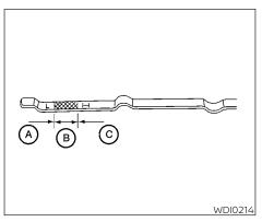
5. Remove the dipstick again and check the oil level. It should be between the H (High) and L (Low) marks (B). This is the normal operating oil level range. If the oil level is below the L (Low) mark (A), remove the oil filler cap and pour recommended oil through the opening. **Do not fill oil level above H (High) mark** (O).
