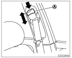
(A) Shoulder belt height adjust button Shoulder belt height adjustment (front seats)
