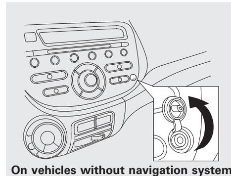
Your vehicle's audio system will disable itself if it is disconnected from electrical power for any reason. To make it work again, you must enter a specific digit code using the preset buttons. Because there are hundreds of number combinations possible from specific digits, making the system work without knowing the exact code is nearly impossible.
