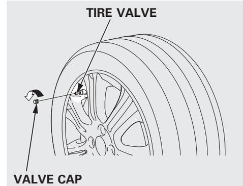
1. Park vehicle on a level surface in a safe place. Set shifter lever into PARK and engage the parking brake. Turn hazard light on. Remove valve cap from tire valve.
