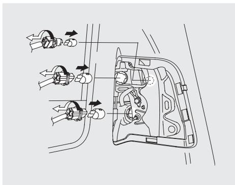
2. Determine which of the three bulbs is burned out: stop/taillight, back-up light, or turn signal light.
