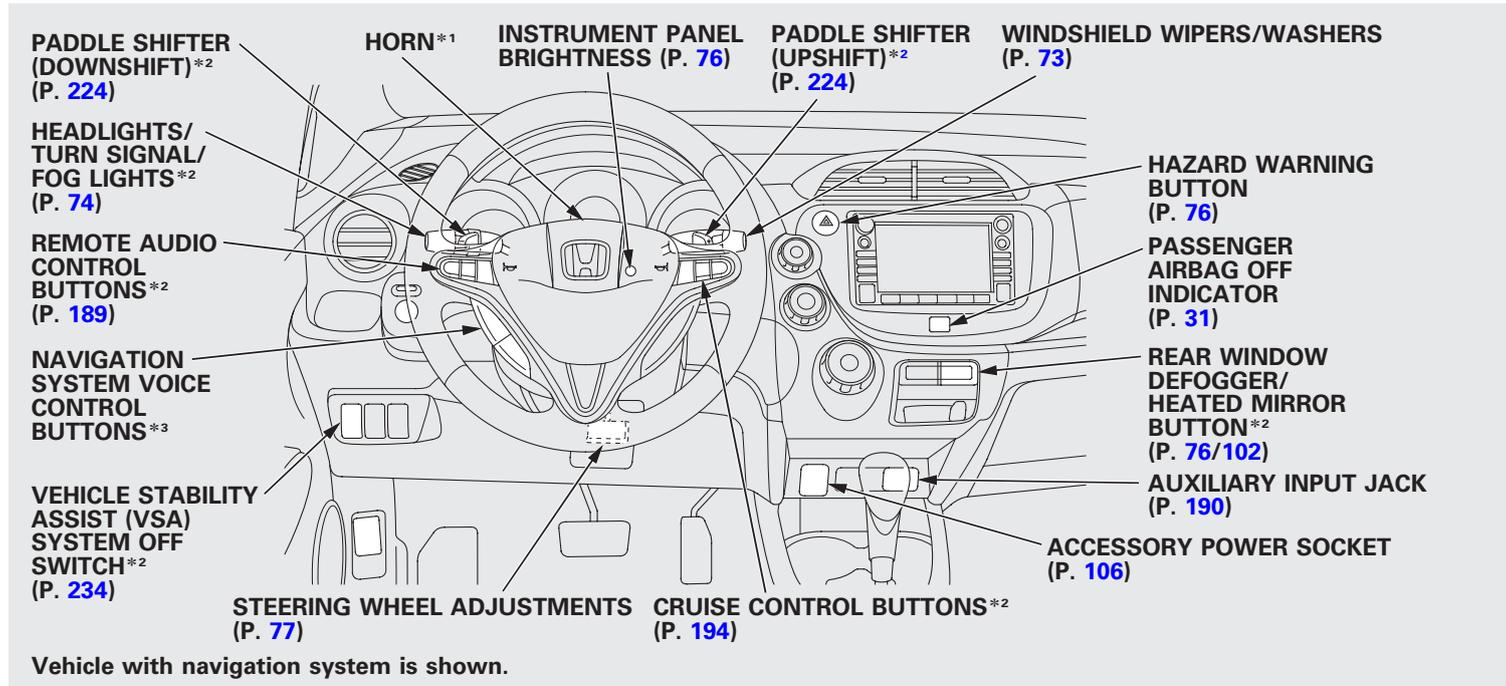
\*1: To use the horn, press the center pad of the steering wheel.
