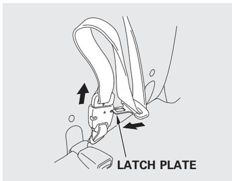
When you fold down the driver's side rear seat, use the latch plate to release the center seat belt from the detachable anchor (see page 99). Allow the seat belt to retract into the holder on the ceiling, and store the buckles in it.
