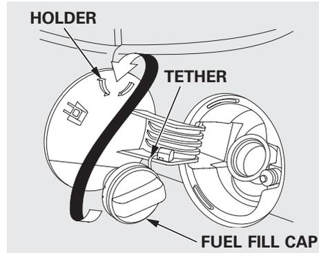
3. Remove the fuel fill cap slowly. You may hear a hissing sound as pressure inside the tank escapes. Place the fuel fill cap in the holder on the fuel fill door. To prevent the fuel fill cap from becoming lost, it is attached to the fuel filler with a tether.
