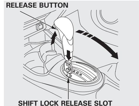
6. Remove the key from the shift lock release slot, then reinstall the cover. Make sure the notch on the cover is on the left side. Press the brake pedal, and restart the engine.
