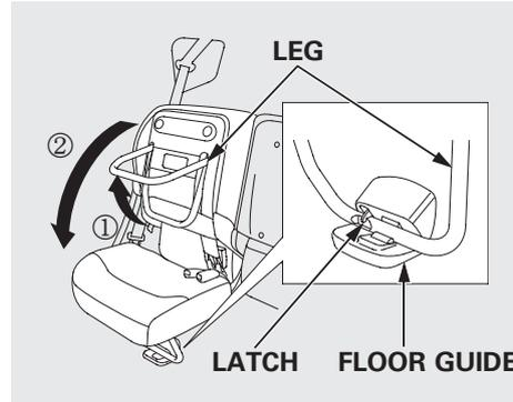
To return the seat cushion to its original position, first make sure there are no items on the floor, then pull up the seat leg fully, and push down the seat cushion slowly while holding it with your hands. Set the seat leg in the floor guide. A latch comes out when the leg is set properly.
