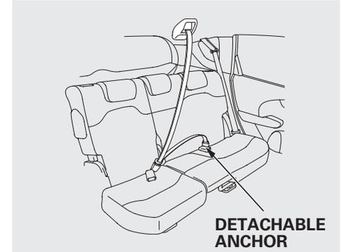
The lap/shoulder belt in the center seating position on the rear seat is equipped with a detachable seat belt that has two parts: a small latch plate and an anchor buckle.
