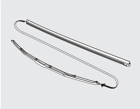
5. Place the top of the wiper blade on the end of the blade assembly, and slide the blade onto the assembly.
