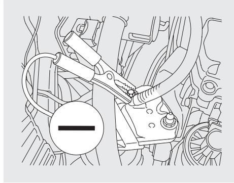
4. Connect the second jumper cable to the negative (-) terminal on the booster battery. Connect the other end to the ground strap as shown. Do not connect this jumper cable to any other part of the engine.
