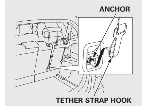
2. Attach the tether strap hook to the anchor, making sure the tether strap is not twisted.
