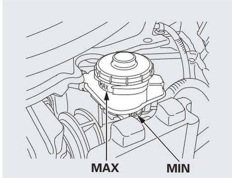
The fluid level should be between the MIN and MAX marks on the side of the reservoir. If the level is at or below the MIN mark, your brake system needs attention. Have the brake system inspected for leaks or worn brake pads/shoes.
