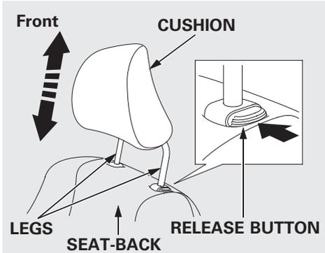
**Adjusting the Head Restraint**
