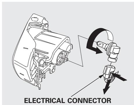
3. Remove the electrical connector from the bulb by squeezing the connector to unlock the tab, then slide the connector off the bulb.
