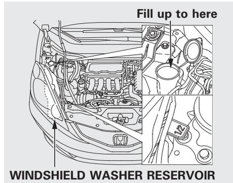
*On U.S. models:* To check the windshield washer fluid level, open the hood and look the windshield washer reservoir located behind the right headlight. You will see a “ 1/2 ” mark on the reservoir.
