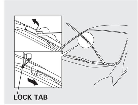
2. Disconnect the blade assembly from the wiper arm:
