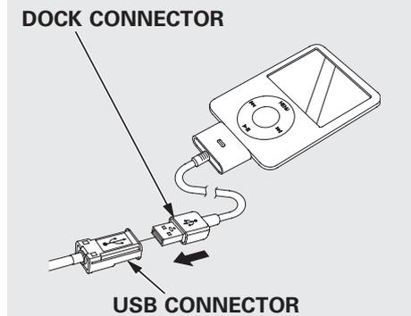
2. Connect your dock connector to the iPod correctly and securely.
