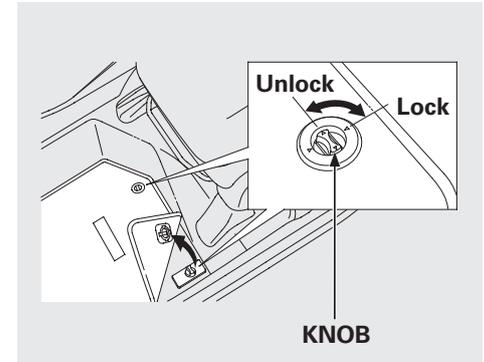
The driver's floor mat that came with your vehicle hooks over the floor mat anchors. To lock each hook, turn the knob clockwise. This keeps the floor mat from sliding forward and possibly interfering with the pedals.
