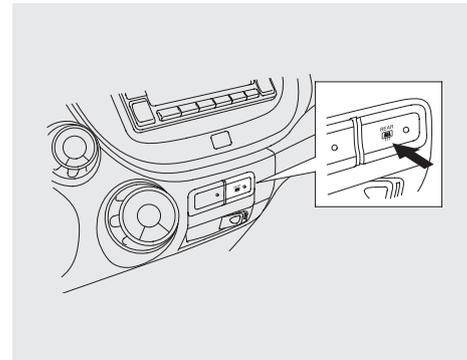
The rear window defogger will clear fog, frost, and thin ice from the window. Push the defogger button to turn it on and off. The indicator in the button comes on to show the defogger is on. You must manually shut off the rear window defogger when it is no longer needed.
