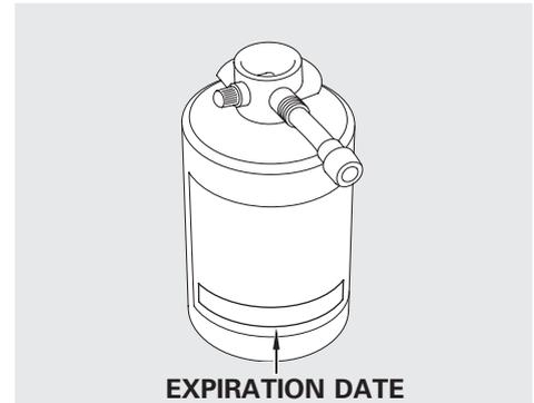
4. Remove the sealant bottle and check the expiration date on the label. If the date has expired, do not continue. Have your vehicle towed to the nearest Honda service center. In Canada or the continental U.S.A. simply call 1-800-465-PLUS (7587) for Honda Plus Roadside Assistance.
