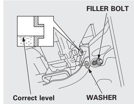
Check the fluid level with the transmission at normal operating temperature and the vehicle on level ground.
