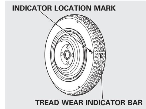
Replace the tire when you can see the tread wear indicator bars. The replacement should be the same size and design tire, mounted on the same wheel. The spare tire is not designed to be mounted on a regular wheel, and the spare wheel is not designed for mounting a regular tire.
