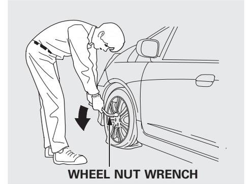
9. Loosen each wheel nut 1/2 turn with the wheel nut wrench.
