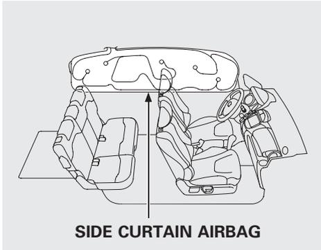
In a moderate to severe side impact, sensors will detect rapid acceleration and signal the control unit to instantly inflate the side curtain airbag and activate the seat belt tensioner on the driver's or the passenger's side of the vehicle.
