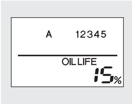
3. Press the select/reset knob for about 10 seconds. The engine oil life and the maintenance item code(s) will blink.
