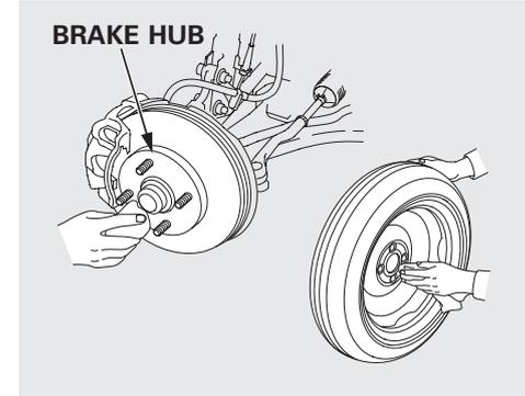
13. Before mounting the spare tire, wipe any dirt off the mounting surface of the wheel and hub with a clean cloth. Wipe the hub carefully; it may be hot from driving.
