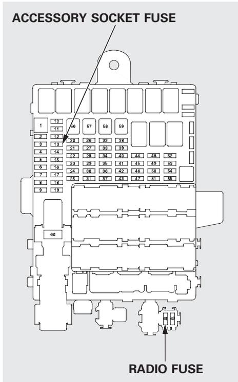
Only remove the fuses after you have performed the transmission shifting procedure, and the key is in the ACCESSORY (I) position. Store the fuses in an obvious location (center pocket, etc) as a reminder to re-install the fuses before driving the vehicle.
