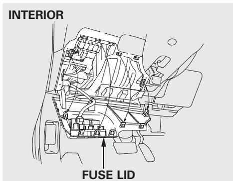
The vehicle's fuses are contained in two fuse boxes.
