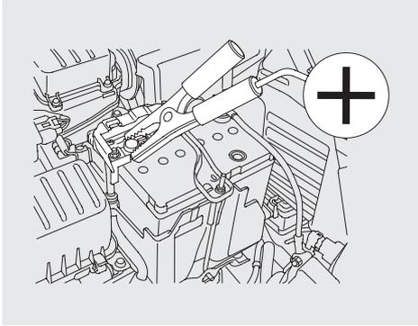
3. Remove the cover from the underhood fuse box (see page 306). Connect one jumper cable to the positive (+) terminal on your battery. Connect the other end to the positive (+) terminal on the booster battery.
