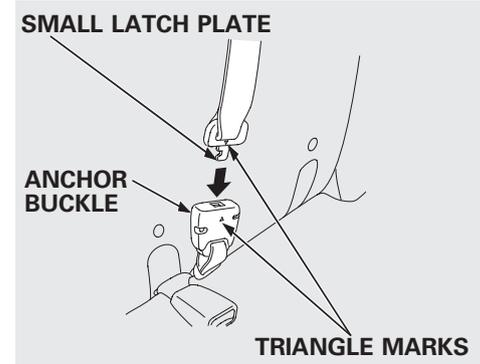
Line up the triangle marks on the small latch plate and anchor buckle when reattaching the belt and buckle.
