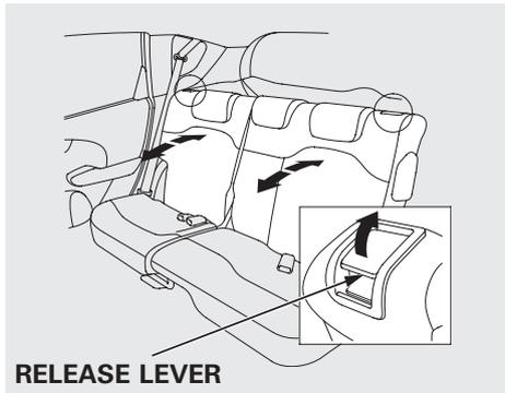
You can adjust the angle of the rear seat-backs separately. To change the seat-back angle, pull up the release lever on the outer side of the seat-back.
