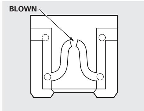
5. Look for a blown wire inside the fuse. If it is blown, replace it with one of the spare fuses of the same rating or lower.
