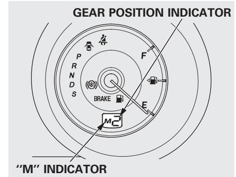
When you move the shift lever from "D" to the "S" position and pull either paddle shifter, the gear position indicator displays "M" along with the selected gear number.
