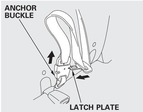
To unlatch the detachable anchor, insert the latch plate into the slot on the side of the anchor buckle. Store the detachable anchor and seat belt latch plates in the retractor housing.
