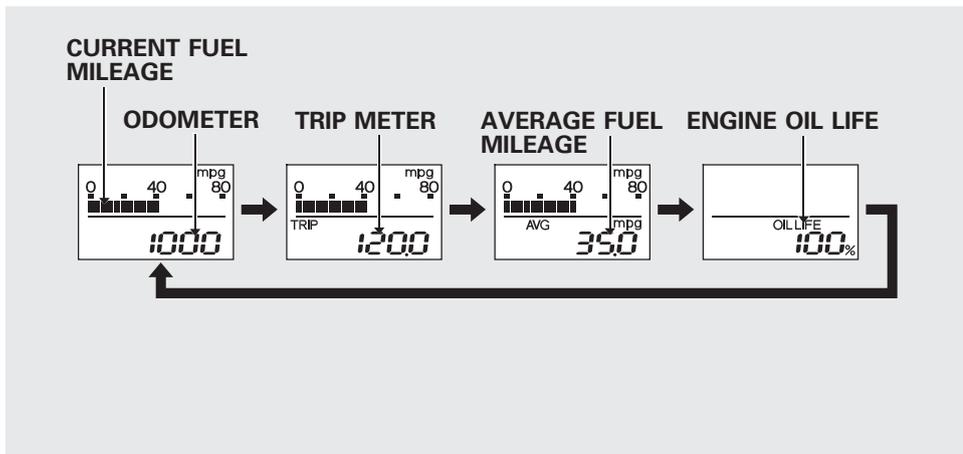
The information display consists of two segments. The upper segment displays current fuel mileage, maintenance item code(s), and the lower segment displays the trip meter, odometer, average fuel mileage, and engine oil life.
