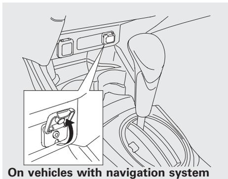
Your vehicle has the auxiliary input jack on the front panel. The system will accept auxiliary input from standard audio accessories.
