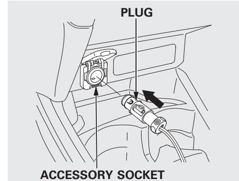
8. Route the power cord into the vehicle, and insert the plug into the accessory power socket.
