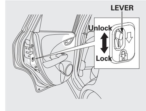
The childproof door locks are designed to prevent children seated in the rear from accidentally opening the rear doors. Each rear door has a lock lever near the edge. With the lever in the LOCK position (lever is down), the door cannot be opened from the inside regardless of the position of the lock tab. To open the door, pull the lock tab forward and use the outside door handle.
