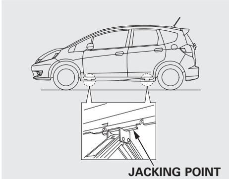
10. Place the jack under the jacking point nearest the tire you need to change. It is pointed to by a  $\triangle$  mark molded into the underside of the body (Sport model). Turn the end bracket clockwise until the top of the jack contacts the jacking point. Make sure the jacking point tab is resting in the jack notch.
