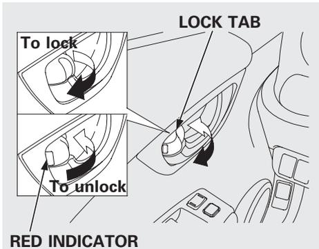
Each door has a lock tab next to the inside door handle. Pull the lock tab to lock the door, and push it forward to unlock the door.
