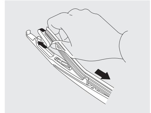
5. Slide the new blade into the holder. Make sure it is engaged in the slot along its full length.
