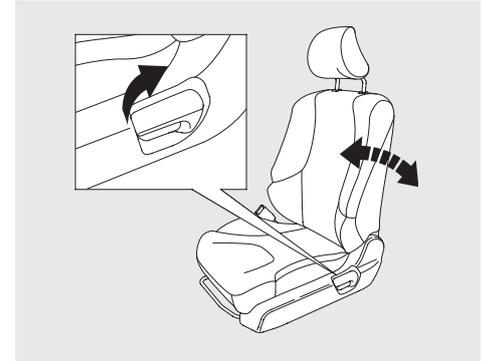
To change the seat-back angle, pull up the lever on the outside of the seat bottom.
