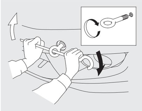
3. Screw the towing hook into the bolt hole behind the bumper, then tighten the hook securely with the extension.
