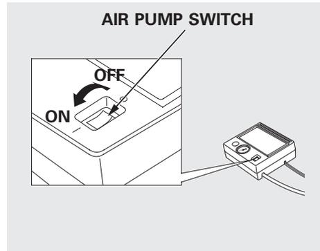
10. Turn the air pump on to inflate the tire. Do not run the air pump for more than 15 minutes or it may overheat. The air pressure gauge will show about 40 to 60 psi (275 to 415 kPa) for the first few minutes while the sealant is pumped into the tire, and then the pressure will go down to about 10 to 20 psi (70 to 140 kPa).
