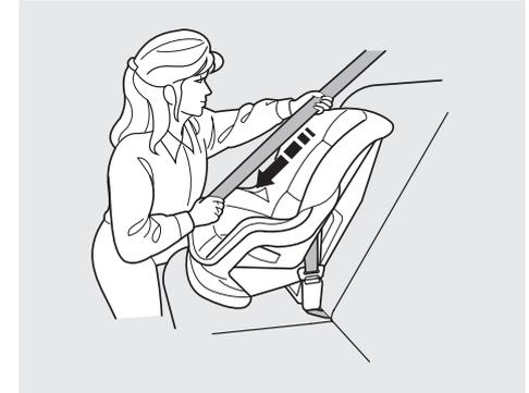
2. To activate the lockable retractor, slowly pull the shoulder part of the belt all the way out until it stops, then let the belt feed back into the retractor.
