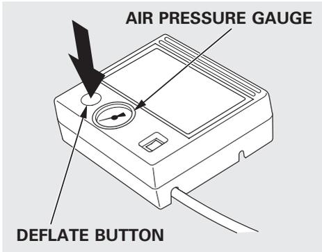
14. Push the deflate button on the air pump until the air pressure gauge shows 0 psi.
