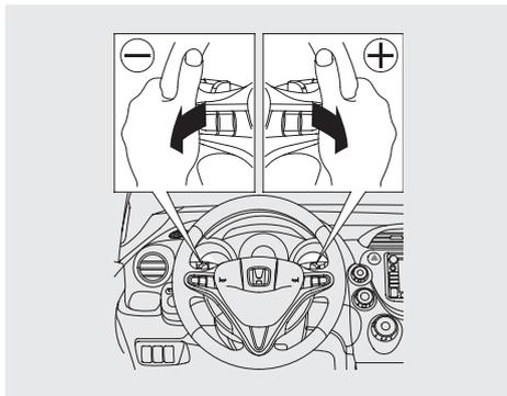
To shift up or down, use the + (right) or - (left) paddle shifter on each side of the steering wheel.
