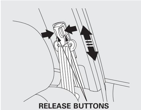
The front seats have adjustable seat belt anchors. To adjust the height of an anchor, squeeze the two release buttons, and slide the anchor up or down as needed (it has four positions).
