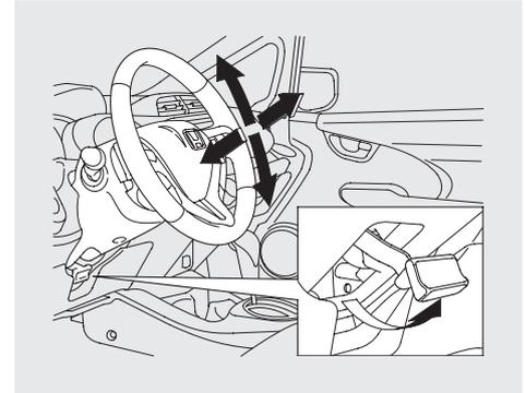
3. Push the lever forward fully to lock the steering wheel in position.
