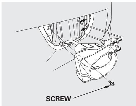
1. Use a Phillips-head screwdriver to remove the screw.
