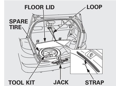
4. Open the tailgate. Raise the cargo area floor lid by lifting it up with the back of the strap. To keep the floor lid open, hook the looped side of the strap to the legs of the rear center head restraint.
