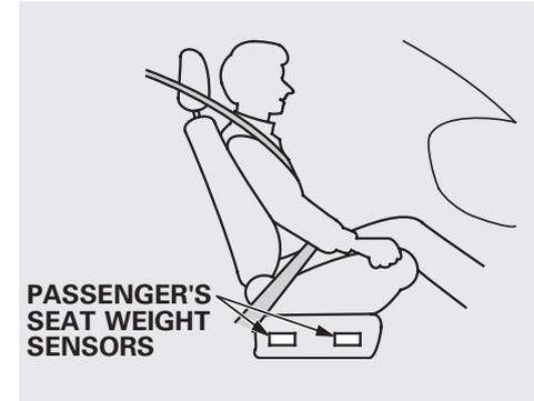
The passenger's advanced front airbag system has weight sensors under the seat. Although Honda does not encourage carrying an infant or small child in front, if the sensors detect the weight of an infant or small child (up to about 65 lbs or 29 kg), the system will automatically turn the passenger's front airbag off.
