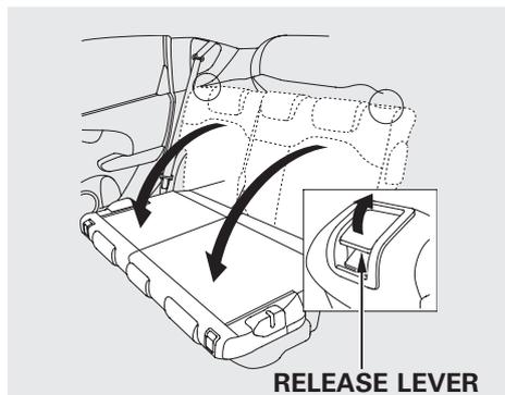
1. Lower the rear head restraints to its lowest position. If you fold down the driver's side seat-back, also adjust the rear center head restraint to its lowest position.
