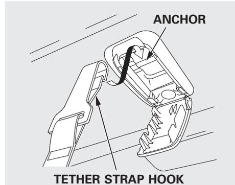
3. Route the tether strap over the head restraint, then attach the tether strap hook to the anchor, making sure the tether strap is not twisted.
