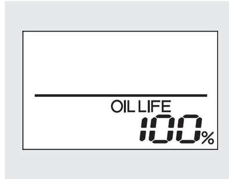
4. Press the select/reset knob for another 5 seconds. The maintenance item code(s) will disappear, and the engine oil life will reset to “100.”
