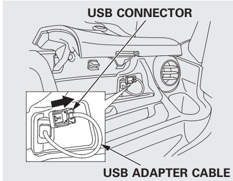
1. Open the upper glove box, and pull out the USB adapter cable.
