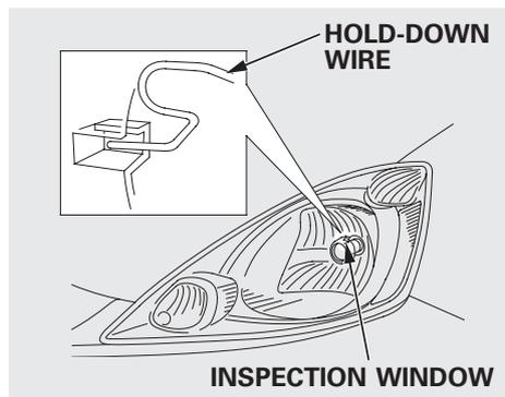
6. Make sure that the hold-down wire is installed properly and securely. You can check its installation from the inspection window on the headlight assembly.
