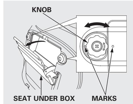
Pull up the driver's side rear seat cushion (see page 97). Open the seat under box by turning the knob. To close the seat under box, turn the knob and align the marks.
