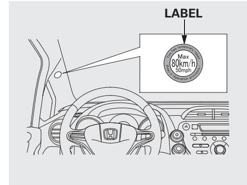
16. Remove the front pillar label from the repair kit and place it as shown above.
