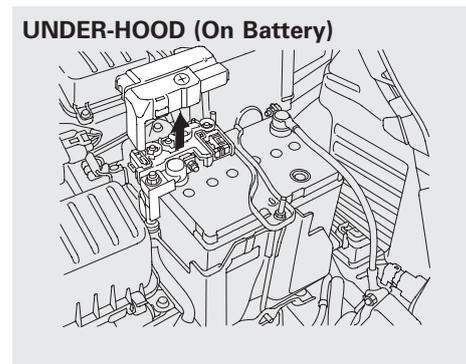
The under-hood fuse box is on the positive terminal of the battery.
