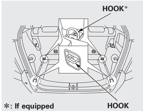
The two or four hooks on the floor can be used to install a net for securing items.
