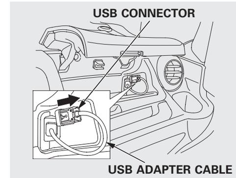
1. Open the upper glove box, and pull out the USB adapter cable.
