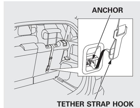
6. Attach the tether strap hook to the anchor, then tighten the strap as instructed by the child seat maker.
