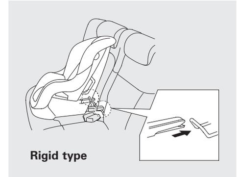
3. Place the child seat on the vehicle seat, then attach the seat to the lower anchors according to the child seat maker's instructions.
