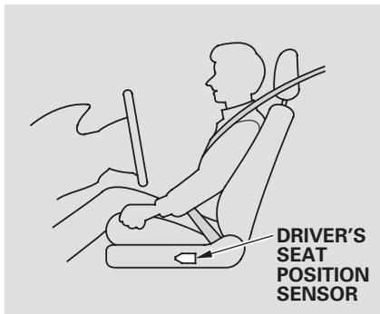
The driver's advanced front airbag system includes a seat position sensor under the seat. If the seat is too far forward, the airbag will inflate with less force, regardless of the severity of the impact.
