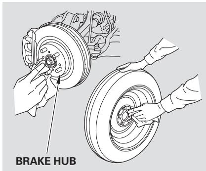
17. Before mounting the spare tire, wipe any dirt off the mounting surface of the wheel and hub with a clean cloth. Wipe the hub carefully; it may be hot from driving.
