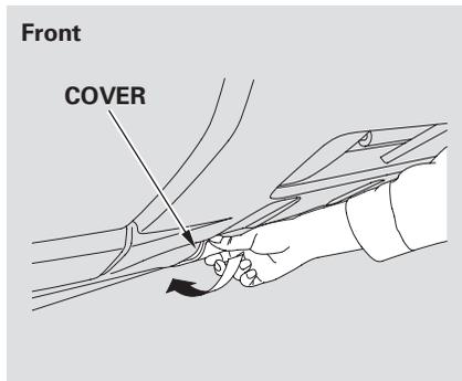
1. Remove the cover, put cloth on the edge of the cover and carefully pry with a small flat-tip screwdriver or a metal fingernail file.
