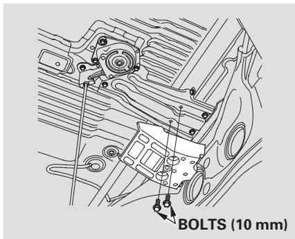
To remove the spacer, loosen the two bolts.
