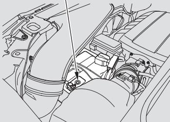
Check the condition of the battery monthly by looking at the test indicator window. The label on the battery explains the test indicator's colors.
