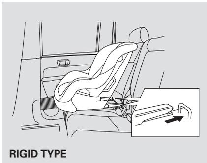
3. Place the child seat on the vehicle seat, then attach the seat to the lower anchors according to the child seat maker's instructions.
