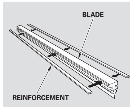
3. Examine the new wiper blades. If they have no plastic or metal reinforcement along the back edge, remove the metal reinforcement strips from the old wiper blade, and install them in the slots along the edge of the new blade.
