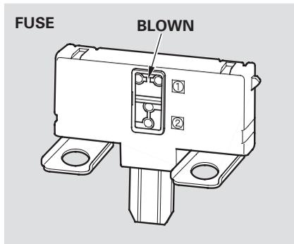
3. Check each of the large fuses in the under-hood fuse boxes by looking through the top at the wire inside. Removing these fuses requires a Phillips-head screwdriver.
