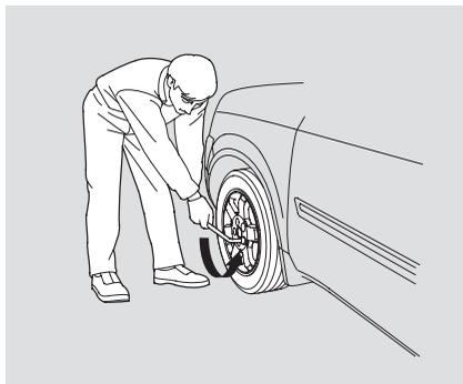
11. Loosen each wheel nut 1/2 turn with the wheel nut wrench.
