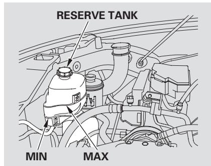
Look at the coolant level in the radiator reserve tank. Make sure it is between the MAX and MIN lines. If it is below the MIN line, see **Adding Engine Coolant** on page [479](#) for information on adding the proper coolant.
