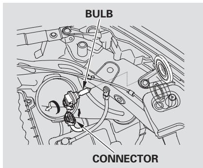
4. Insert the new bulb into the hole, and turn it one-quarter turn clockwise to lock it in place.
