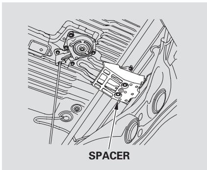
If you store a full size tire on the hoist, remove the spacer. Otherwise the hoist will not fully return to its original position.
