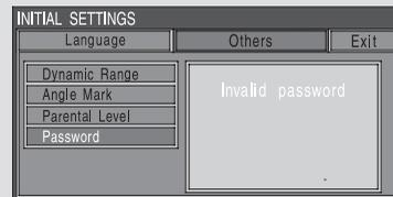
If the system does not recognize the password you entered, you will see the above display. Repeat the password setting steps until you enter the correct password.
