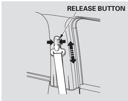
The front seats and second row seats have adjustable seat belt anchors. To adjust the height of an anchor, squeeze the two release buttons, and slide the anchor up or down as needed (it has four positions).
