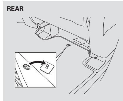
If you use a non-Honda floor mat, make sure it fits properly and that it can be used with the floor mat anchors. Do not put additional floor mats on top of the anchored mats.
