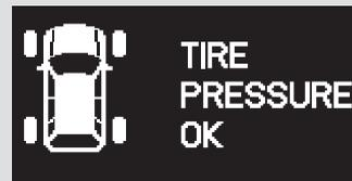
To select the tire pressure monitor, press the INFO button several times with the ignition switch in the ON (II) position.
