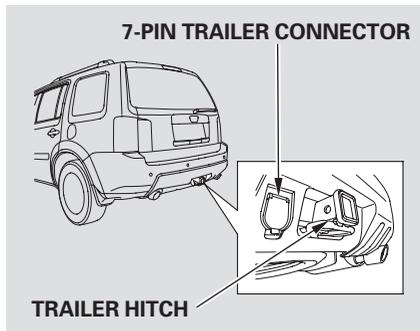
Your vehicle has a class 3 trailer hitch as standard equipment.
