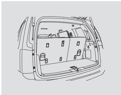
Each third row seat has a tether anchorage point behind the seat-back.
