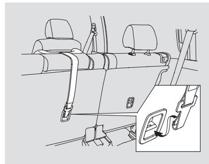
For the center seat, lower the head restraint, then route the tether strap over the head restraint and seat-back.
