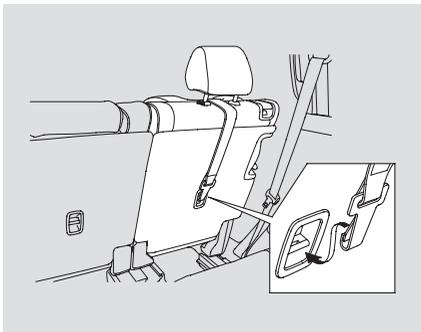
2. Attach the tether strap hook to the anchor, making sure the tether strap is not twisted.
