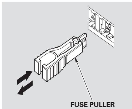
4. Check the smaller fuses in the under-hood fuse boxes and rear fuse box, and all the fuses in the interior and rear fuse boxes by pulling out each one with the fuse puller provided in the primary under-hood fuse box.
