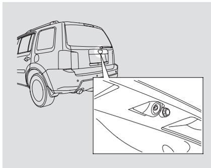
Whenever you shift to reverse (R) with the ignition switch in the ON (II) position, the rear view is shown on the navigation system screen. On vehicle without navigation system, the rear view is shown on the left side of the inside mirror.
