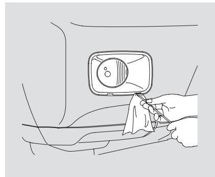
1. Place a cloth on the edge of the cover. Remove the covers by carefully prying on the edge with a small flat-tipped screwdriver.
