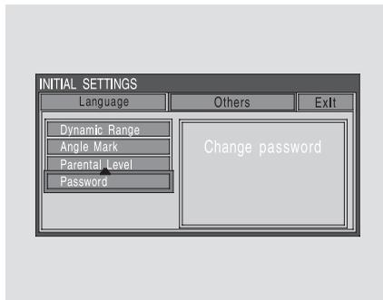
If you forget the password, select "Password," and press the ▲ button 10 times.
