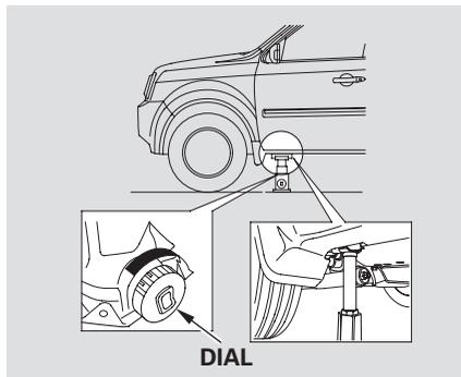
13. Turn the dial at the bottom of the jack clockwise until the top of the jack contacts the jacking point. Make sure the jacking point tab is resting in the jack notch.
