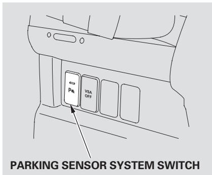
To activate the system, push the switch on the dashboard with the ignition in the ON (II) position. The indicator in the switch comes on when the system is on. To turn the system off, push the switch again.
