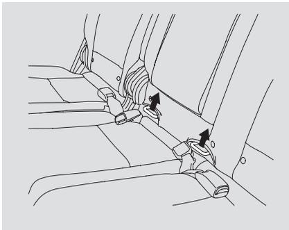
To install a LATCH-compatible child seat in the center seating position on the second row seat, use the center lower anchors as shown above.
