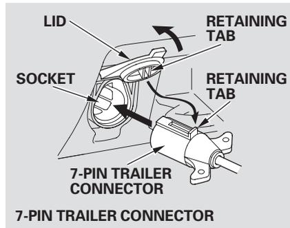
The 7-pin trailer connector is needed for the trailer lights. To connect the connector, do this:
