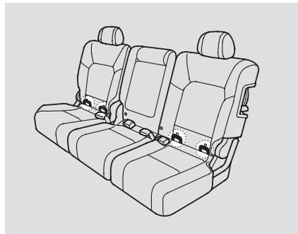
To install a LATCH-compatible child seat in either outer second row seat:
