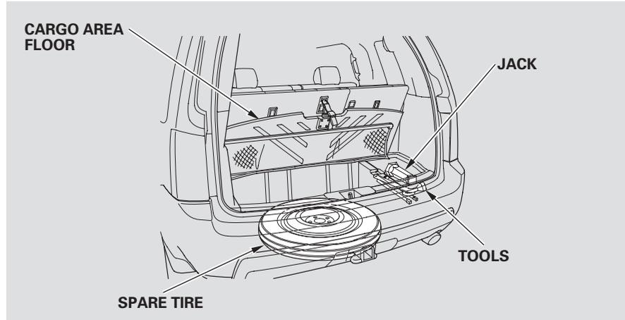
2. Turn on the hazard warning lights, and turn the ignition switch to the LOCK (0) position. Have all passengers get out of the vehicle while you change the tire.
