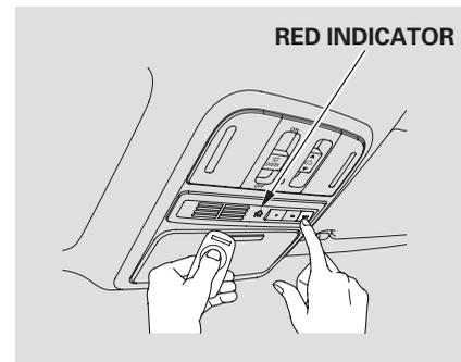
2. Press and hold the remote transmitter button and one of the HomeLink buttons at the same time.
