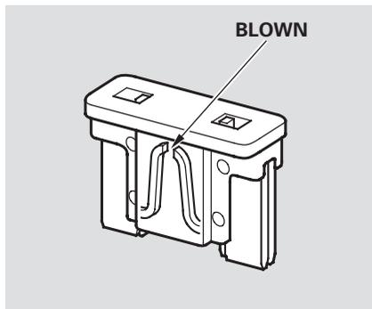
5. Look for a burned wire inside the fuse. If it is burned out, replace it with one of the spare fuses of the same rating or lower.
