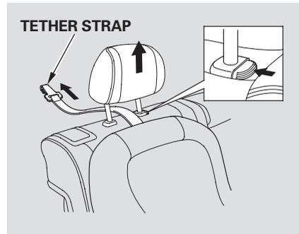
5. Lift the head restraint (see page [155](#)), then route the tether strap through the legs of the head restraint and over the seat-back, making sure the strap is not twisted.
