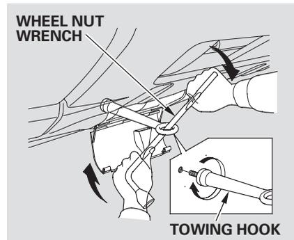
2. Remove the towing hook and wheel nut wrench placed behind a cover under the cargo area.
