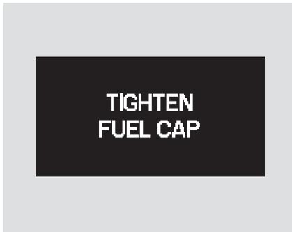
Your vehicle’s on board diagnostic system will detect a loose or missing fuel fill cap as an evaporative system leak. The first time a leak is detected a “TIGHTEN FUEL CAP” message appears on the multi-information display. Turn the engine off, and confirm the fuel fill cap is installed. If it is, loosen it, then retighten it until it clicks at least once. The message should go off after several days of
