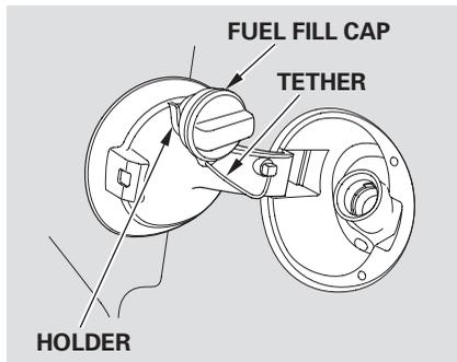
3. Remove the fuel fill cap slowly. You may hear a hissing sound as pressure inside the tank escapes. Place the cap in the holder on the fuel fill door.
