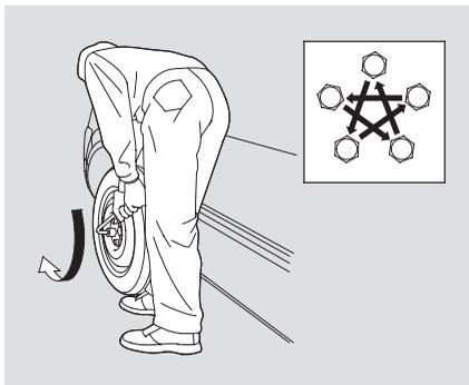
20. Tighten the wheel nuts securely in the same crisscross pattern. Have the wheel nut torque checked at the nearest automotive service facility.
