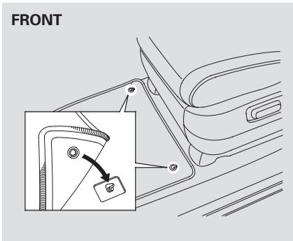
The floor mats that came with your vehicle hook over the floor mat anchors. This keeps the floor mats from sliding forward, possibly interfering with the pedals, or backwards, making the front passenger's weight sensors ineffective.
