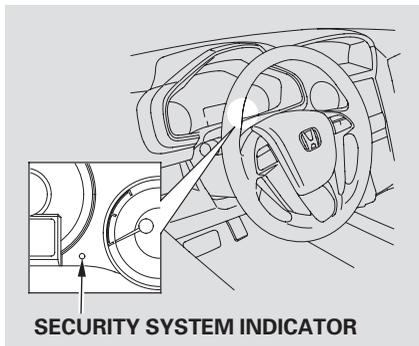
Once the security system is set, opening any door, the tailgate, the glass hatch, or the hood without using the key or the remote transmitter will cause the alarm to sound. It will also sound if the radio is removed from the dashboard or the wiring is cut.
