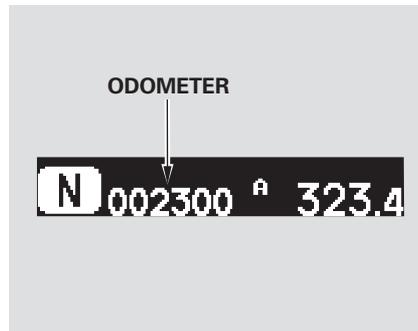
The odometer shows the total distance your vehicle has been driven. It measures miles in U.S. models and kilometers in Canadian models. It is illegal under U.S. federal law and Canadian provincial regulations to disconnect, reset, or alter the odometer with the intent to change the number of miles or kilometers indicated.
