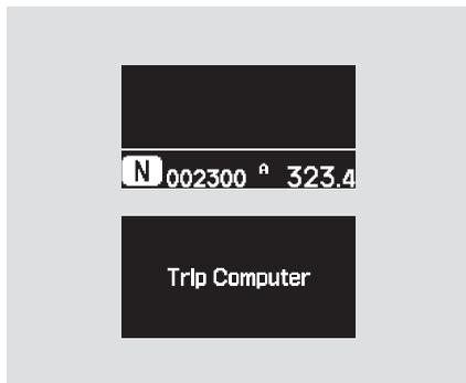
When the main menu is blank or Trip Computer, pressing the SEL/RESET button changes the display to “odometer/trip meter” “outside temperature/trip meter” and “engine oil life.”
