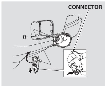
2. Remove the front fog light assembly from the bumper.
