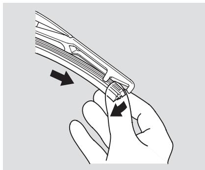
2. Slide the blade out of the wiper arm.
