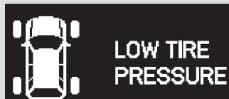
If any of the tires has low pressure, the tire pressure monitor also shows the above message to warn you about the low tire pressure when you select the display by pressing the INFO button several times. Following this display, press the SEL/RESET button to see each tire pressure. When you continue driving after installing the spare tire, you will also see this message on the multi-information display.
