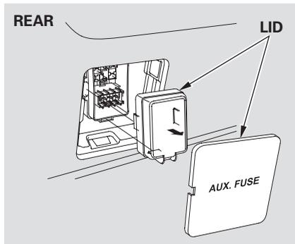
The rear fuse box is located at the left side of cargo area.
