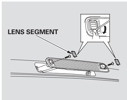
1. Place a cloth on the edge of the lens segment. Remove each lens segment by carefully prying on its edge with a small flat-tipped screwdriver.
