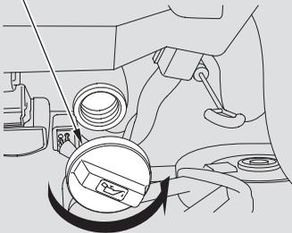
Unscrew and remove the engine oil fill cap on top of the valve cover. Pour in the oil slowly and carefully so you do not spill any. Clean up any spills immediately. Spilled oil could damage components in the engine compartment. Reinstall the engine oil fill cap, and tighten it securely. Wait a few minutes, and recheck the oil level on the engine oil dipstick. Do not fill above the upper mark; you could damage the engine.
