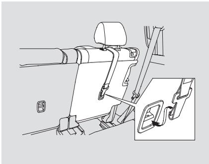
6. Attach the tether strap hook to the tether anchor, then tighten the strap as instructed by the child seat maker.
