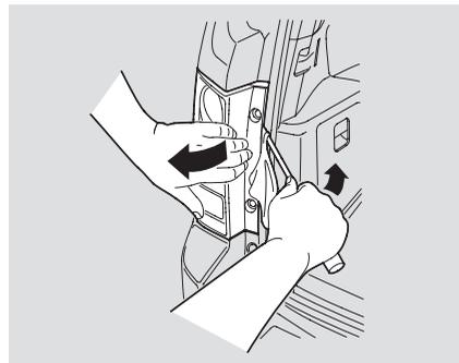
3. Place a cloth on the inner edge of the assembly. Loosen the assembly by carefully prying on the top and side edges with a small flat-tipped screwdriver. Use your fingers to further pull it loose.
