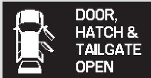
When the glass hatch, tailgate, and one or more doors are not tightly closed, the “DOOR, HATCH & TAILGATE OPEN” message will come on.
