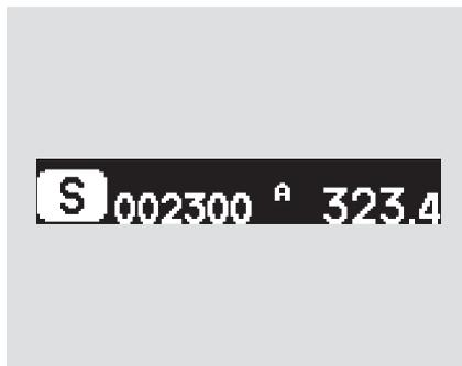
In the left corner of the lower segment, a compass indicates which direction your vehicle is pointed.
