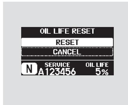
3. Press and hold the SEL/RESET button on the steering wheel for more than 10 seconds. The remaining engine oil life reset mode will be shown on the multi-information display.
