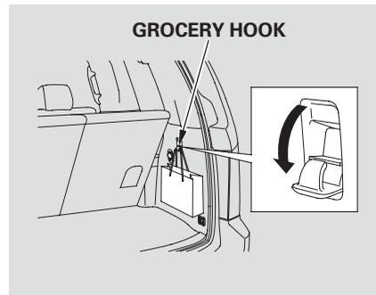
Your vehicle also has grocery hook(s) on the side panels and on the back of the third row seats in the cargo area. They are designed to hold light items. Heavy objects may damage the hook.
