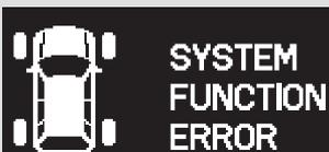
If there is a problem with the TPMS, the tire pressure monitor shows a "SYSTEM FUNCTION ERROR" message and the tire pressure readings are not displayed. If this happens, you will first see a system warning message "CHECK TPMS SYSTEM" on the multi-information display.
