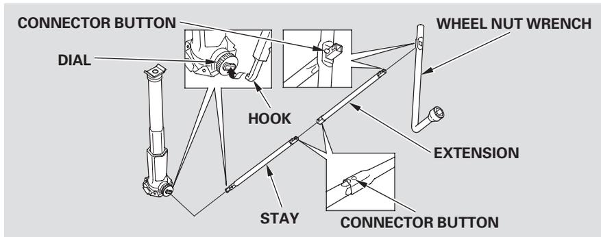
14. Attach the stay to the extension, then attach the wheel nut wrench to the end of the extension. Make sure the stay, the extension, and the wheel nut wrench are securely attached.
