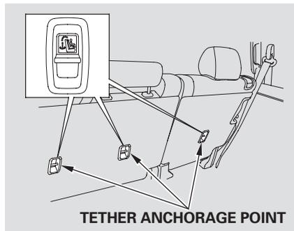
Each second row seat has a tether anchorage point behind the seat-back.
