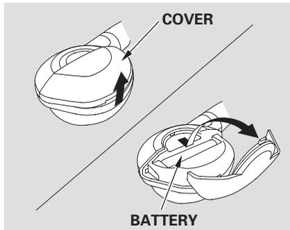
Remove the battery. Install the new battery in the earpiece as shown in the diagram next to the battery slot. Slide the cover back into place on the earpiece, then press down on the back edge to lock it in place.
