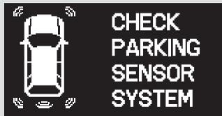
If the system develops a problem, you will see a “CHECK PARKING SENSOR SYSTEM” message on the multi-information display, and a beeper sounds continuously. Very often, a sensor covered with mud, ice, snow, etc. is the cause of this message. Check the sensors first. If the message stays on or the beeper does not stop, have the system checked by your dealer.
