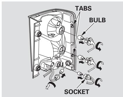
5. Determine which of the four bulbs is burned out: stop/taillight, back-up light, side marker light, or turn signal light.
