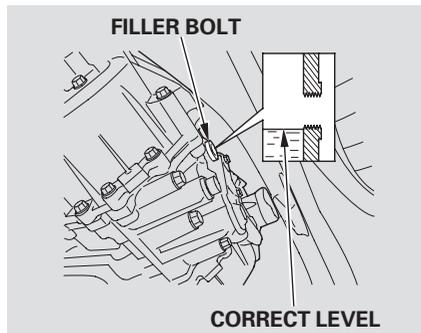
The rear differential should be drained and refilled with new fluid when this service is indicated by a maintenance message on the information display or multi-information display. This service may be needed more often under certain driving conditions (see page [473](#)).
