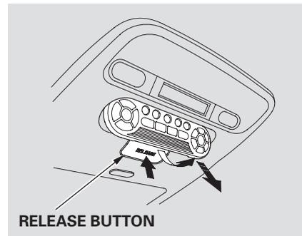
The rear control panel can be detached from the ceiling unit and used as a remote control. To remove it from the ceiling unit, press the release button. The control panel will swing down partway. Pivot it down further past the detent until it detaches from the hinge. To reinstall it, reverse the procedure.
