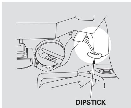
2. Remove the dipstick (yellow loop) from the transmission, and wipe it with a clean cloth.
