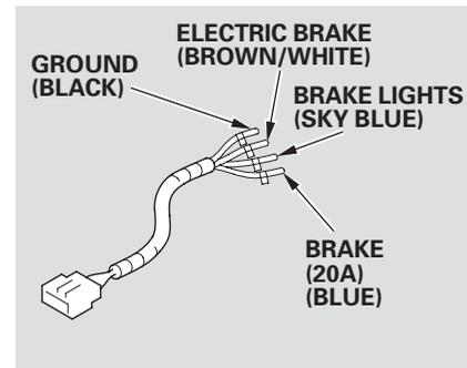
The trailer jumper harness is used to install the controller for the electric trailer brakes. For more information, see **Trailer Brakes** on page [445](#).
