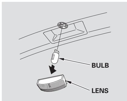
3. Turn on the parking lights and check that the new bulb is working.
