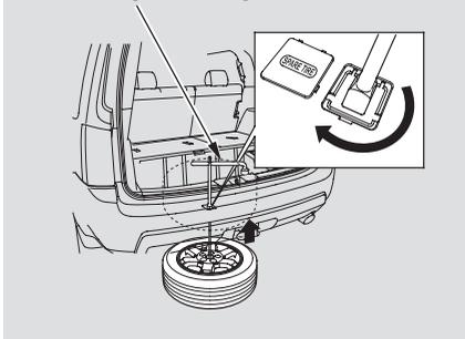
23. Slowly turn the extension with the wheel nut wrench clockwise to take up the slack of the hoist cable. Make sure the bracket is seated in the center hole of the flat tire.
