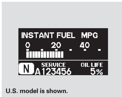
To cancel the system message, press and release the INFO (▲/▼) button on the steering wheel. At this time, the system message indicator will **not** be turned off. Then the display will change to the engine oil life display. You will see the engine oil life blinking and a “SERVICE” message along with the maintenance item code(s) on the multi-information display.
