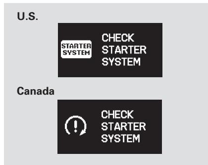
If there is a problem with the starter system, you will see a “CHECK STARTER SYSTEM” message on the multi-information display when the ignition switch is turned to the ON (II) position. You will also see this message when the auto control mode of the starter system has a problem.
