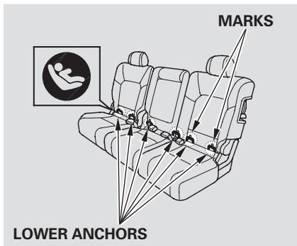
When you install a child seat in the second row seating position, use the lower anchors as shown in the illustration. You can install up to three child seats at a time with LATCH.
