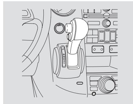
To shift from any position, press firmly on the brake pedal and press the release button on the side of the shift lever. You cannot shift out of Park when the ignition switch is in the LOCK (0) or ACCESSORY (I) position.
