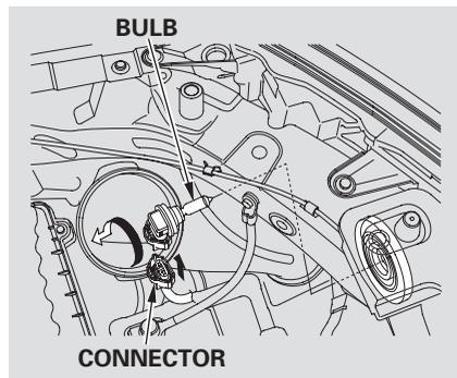
The high beam headlight bulb, the low beam headlight bulb, and daytime running light bulb are replaced the same way.
