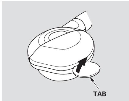
Each headphone uses one AAA battery. The battery is under the cover on the left earpiece. To remove the cover, insert a coin in the slot and twist it slightly to pry the cover away from the earpiece. Pull the cover outward, and pivot it out of the way.
