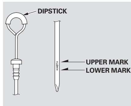
3. Insert the dipstick all the way into the transmission securely as shown in the illustration.
