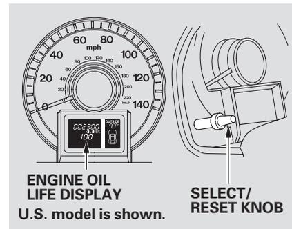
To see the current engine oil life, turn the ignition switch to the ON (II) position, and press the select/reset knob repeatedly until the engine oil life display appears (see page 81).
