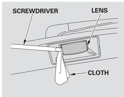
1. Place a cloth on the edge of the lens segment to prevent scratching. Insert a small flat-tip screwdriver between the left edge of the lens and the housing. The lens will come down.
