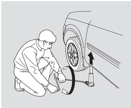
16. Turn the jack dial (wheel nut wrench) clockwise as shown to raise the vehicle until the flat tire is off the ground.
