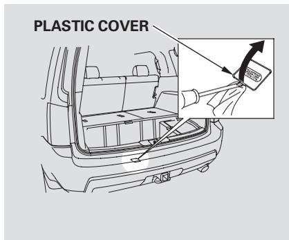
6. The spare tire is stored underneath the rear cargo area. Remove the plastic cover and the rubber cap on the cargo area lining to access the shaft for the spare tire hoist.
