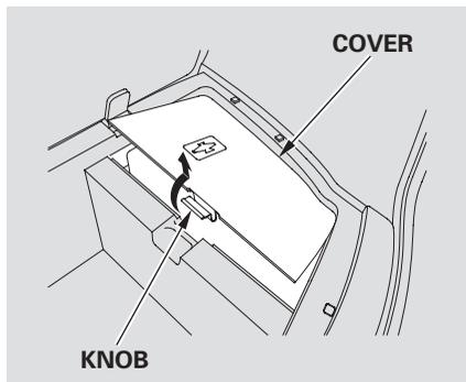
5. The tools and jack are under the cargo area behind a cover on the passenger's side. Remove the cover and take the jack out of the tool kit case.
