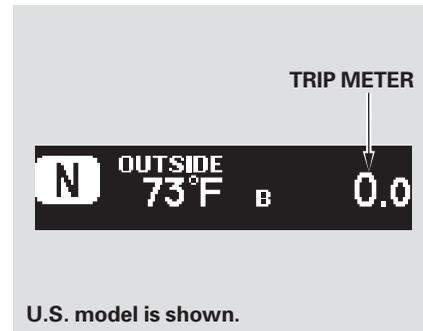
This meter shows the number of miles (U.S.) or kilometers (Canada) driven since you last reset it. There are two trip meters: Trip A and Trip B. Each trip meter works independently, so you can keep track of two different distances.
