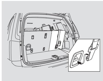
2. Route the tether strap over the head restraint, then attach the tether strap hook to the anchor, making sure the strap is not twisted.
