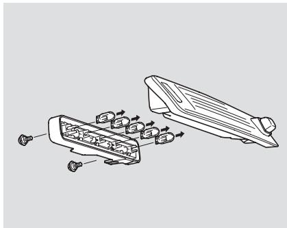
4. Remove the two mounting screws from the light assembly.
