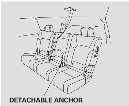
The lap/shoulder belts in the center seat of the second row and both of the third row seats are equipped with a detachable anchor that has two parts: a small latch plate and a buckle.
