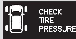
Each tire has its own pressure sensor. If the air pressure of a tire becomes significantly low, the sensor in that tire immediately sends a signal that causes the low tire pressure/TPMS indicator in the instrument panel to come on. If this happens, you will see which tire is losing pressure on the multi-information display along with a "CHECK TIRE PRESSURE" message.
