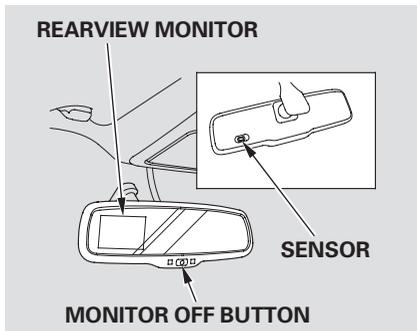
You can turn the monitor on and off by pressing the monitor off button when the shift lever is in reverse. The monitor turns on everytime you shift to reverse, even if you turned it off the last time.
