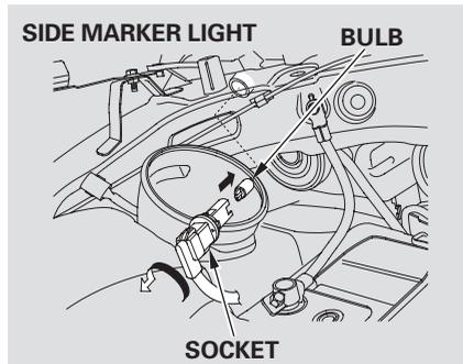
4. Push the new bulb straight into the socket until it bottoms.
