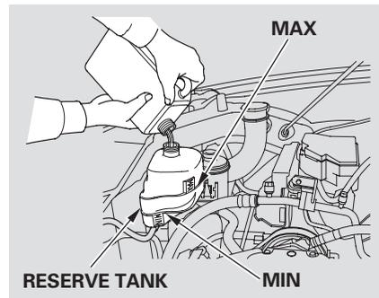
6. Pour coolant into the reserve tank. Fill it to halfway between the MAX and MIN marks. Put the cap back on the reserve tank.
