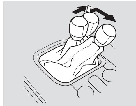
The manual transmission has a lockout so you cannot accidentally shift from fifth to reverse instead of sixth while the vehicle is moving.
