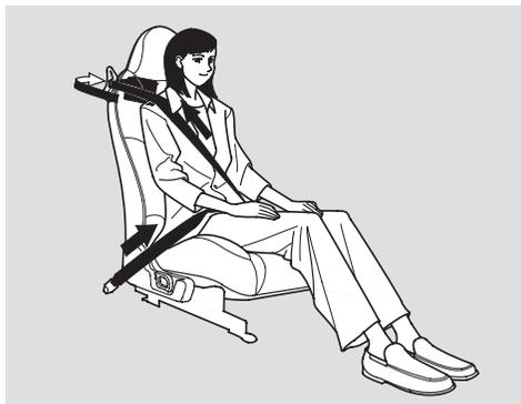
For added protection, the seat belts are equipped with automatic seat belt tensioners. When activated, the tensioners immediately tighten the belts to help hold the driver and a passenger in place.
