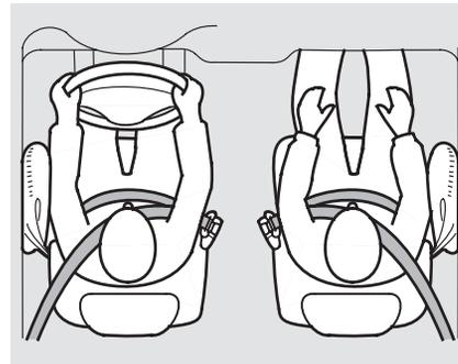
Your vehicle also has side airbags to help protect the upper torso of the driver or a front seat passenger during a moderate to severe side impact (see page [28](#) for more information on how your side airbags work).
