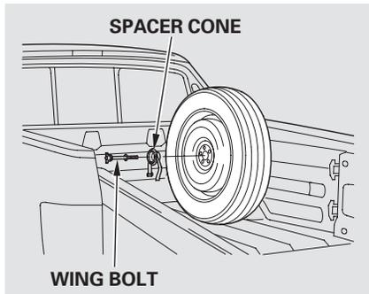
3. Place the spare tire on the pickup bed as shown.
