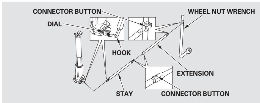
11. Attach the stay to the extension, then attach the wheel nut wrench to the end of the extension.
