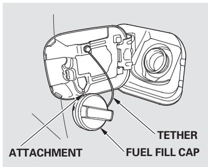
3. Remove the fuel fill cap slowly. You may hear a hissing sound as pressure inside the tank escapes. The fuel fill cap is attached to the fuel filler with a tether. Insert the attachment on the fuel fill cap into the slit on the fuel fill door.
