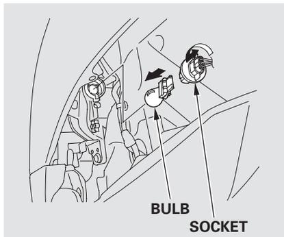
3. Remove the socket from the headlight assembly by turning it one-quarter turn counterclockwise.
