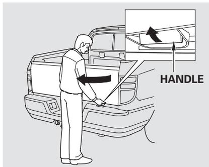
To swing open the tailgate, first make sure it is fully closed, then pull up the right lower handle, and swing the tailgate to the left.
