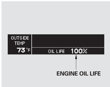
This shows the remaining life of the engine oil. It shows 100% after the engine oil is replaced and the display is reset. The engine oil life is calculated based on engine operating conditions and accumulated engine revolutions. For more information, see page [313](#).
