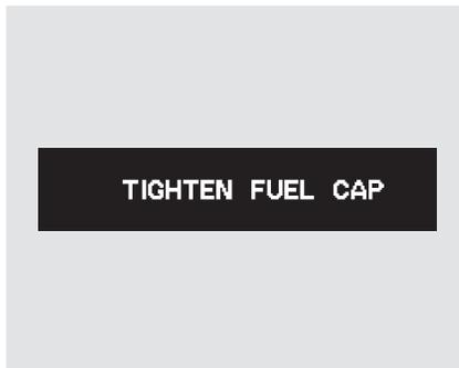
Your vehicle's on board diagnostic system will detect a loose or missing fuel fill cap as an evaporative system leak. The first time a leak is detected a “TIGHTEN FUEL CAP” message appears on the multi-information display. Turn the engine off, and confirm the fuel fill cap is installed. If it is, loosen it, then retighten it until it clicks at least once. The message should go off after several days of
