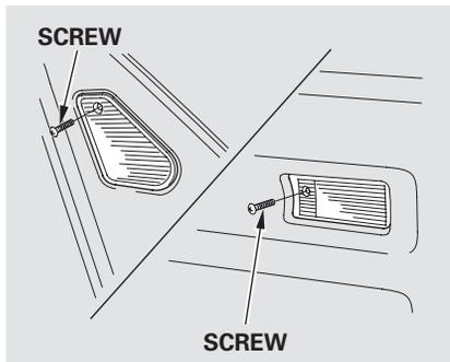
1. Remove the mounting screw from the bed light assembly.
