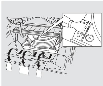
5. Pull out the tire tray with the handle, and hook the rear of the tire tray to the guides on the back edge of the In-Bed Trunk.
