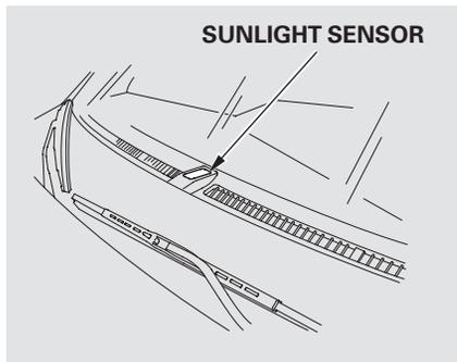
The climate control system has two sensors. A sunlight sensor is in the top of the dashboard, and a temperature sensor is under the steering column. Do not cover the sensors or spill any liquid on them.
