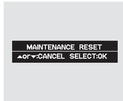
3. Press and hold the SEL/RESET button for 10 seconds. The multi-information display will ask for a confirmation.
