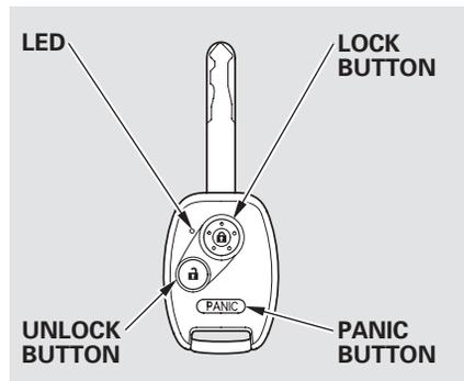
**LOCK** – Press this button once to lock all doors and the In-Bed Trunk. Some exterior and interior lights will flash once. When you push LOCK twice within 5 seconds, you will hear a beep to verify that the doors and In-Bed Trunk are locked and the security system (if equipped) has set. This button does not work if any door is not fully closed or the key is in the ignition switch.
