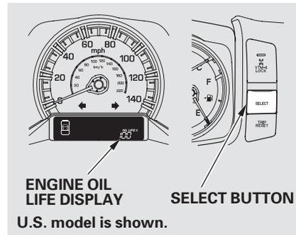
To see the current engine oil life, turn the ignition switch to the ON (II) position, and press the SELECT button repeatedly until the engine oil life display appears (see page 78).
