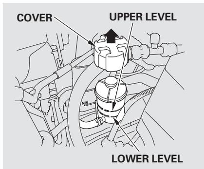
Remove the cover, then check the level on the side of the reservoir when the engine is cold. The fluid should be between the UPPER LEVEL and LOWER LEVEL. If not, add power steering fluid to the UPPER LEVEL mark, and put the cover back in place.
