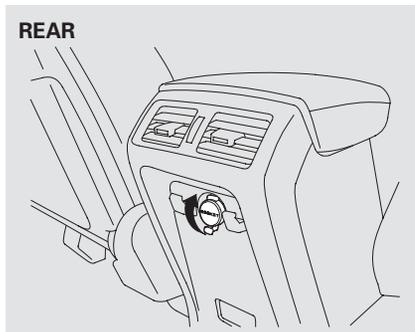
These sockets are intended to supply power for 12 volt DC accessories that are rated 120 watts or less (10 amps).
