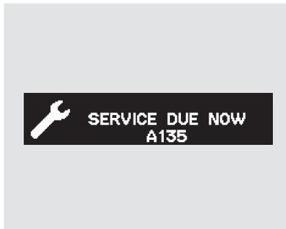
When the remaining engine oil life is less than 5 percent, you will see the above display. The display then changes to “SERVICE DUE NOW.” Have the indicated maintenance done as soon as possible.
