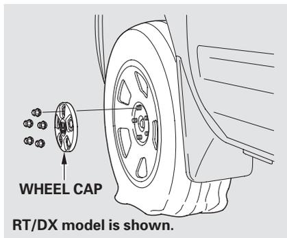
14. Remove the wheel nuts and the wheel cap (on RT and Canadian DX models) then remove the flat tire. Handle the wheel nuts carefully; they may be hot from driving. Place the flat tire on the ground with the outside surface facing up.
