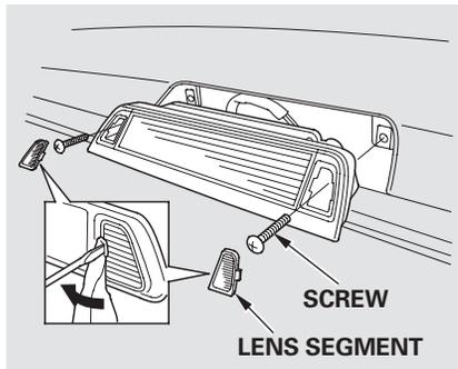
1. Place a cloth on the edge of the lens segment to prevent scratches. Remove each lens segment by carefully prying on its edge with a small flat-tip screwdriver.
