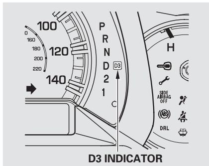
When D3 is on, the transmission selects only the first three gears. Use D3 for engine braking when going down a steep hill.
