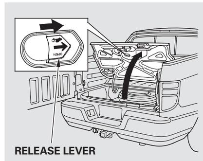
As a safety feature, your vehicle has a release lever on the latch of the In-Bed Trunk lid so it can be opened from the inside. To open the In-Bed Trunk, push the release lever in the direction of the arrow.
