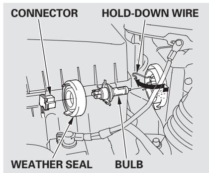
1. Remove the electrical connector from the bulb by pulling the connector straight back.
