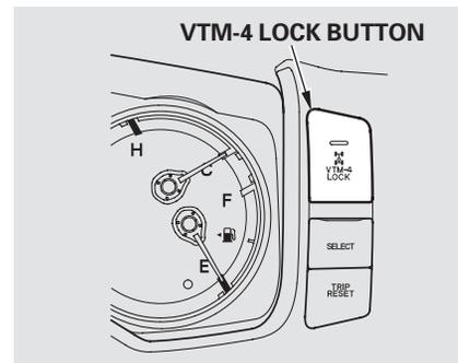
Your vehicle is equipped with a Variable Torque Management® 4-wheel-drive system (VTM-4®) that distributes engine torque to the appropriate drive axle depending on the available traction conditions. The system is completely automatic, always active, and does not require any driver interaction.
