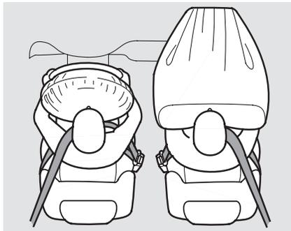
Your vehicle has a supplemental restraint system (SRS) with front airbags to help protect the heads and chests of the driver and a front seat passenger during a moderate to severe frontal collision (see page [25](#) for more information on how your front airbags work).
