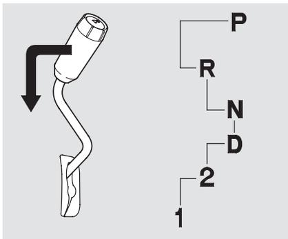
**Park (P)** – This position mechanically locks the transmission. Use Park whenever you are turning off or starting the engine. To shift out of Park, you must press on the brake pedal and have your foot off the accelerator pedal. Pull the shift lever towards you, then move it out of Park.
