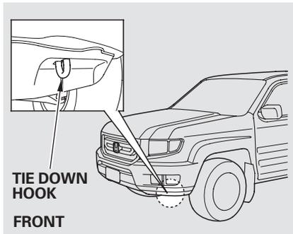
For very short distances, such as freeing the vehicle, you can use the tie down hooks on the lower of the front and rear bumpers.
