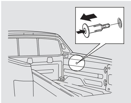
As a temporary mounting location, you can secure a spare tire on the pickup bed, if needed.
