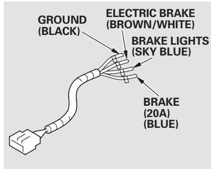
The trailer jumper harness is used to install the controller for the electric trailer brakes. For more information, see *Trailer Brakes* on page [298](#).
