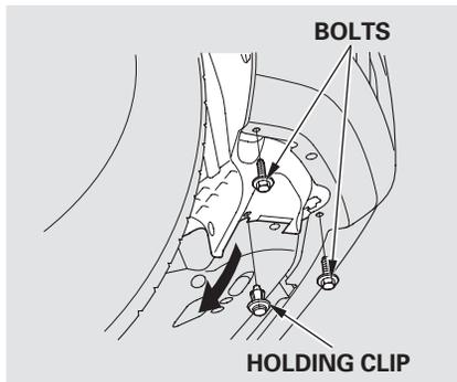
1. Remove the bolts and use the flat-tip screwdriver to remove the holding clip located under the front bumper.
