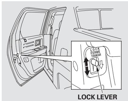
The childproof door locks are designed to prevent children seated in the rear from accidentally opening the rear doors. Each rear door has a lock lever near the edge. With the lever in the LOCK position, the door cannot be opened from inside regardless of the position of the lock tab. To open the door, pull the lock tab up, and use the outside door handle.
