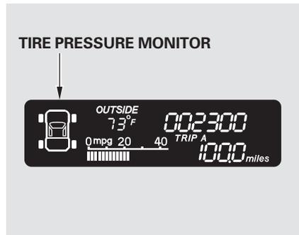
The appropriate tire indicator will come on along with the low tire pressure indicator if a tire is significantly underinflated or has suddenly lost pressure. See **Low Tire Pressure Indicator** for what to do if this indicator comes on.
