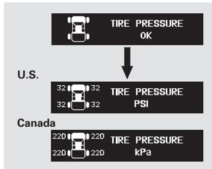
When the tire pressure monitor is shown on the multi-information display, press the SEL/RESET button. The display changes as shown. You can see the pressure of each tire in this monitor. If one or more tires are low, inflate them to the correct pressure. For more information, see page [282](#).
