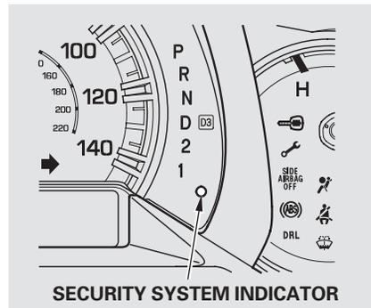
Once the security system is set, opening any door (without using the key or the remote transmitter), the hood, or the In-Bed Trunk, will cause it to alarm. It also alarms if the radio and navigation components are removed from the dashboard or the wiring is cut.
