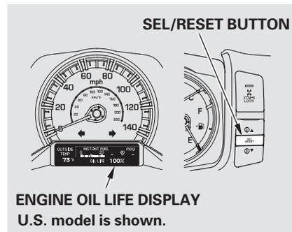
To see the current engine oil life, turn the ignition switch to the ON (II) position, and push and release the SEL/RESET button on the dashboard repeatedly, until the engine oil life is displayed (see page 83).
