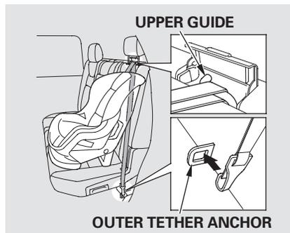
1. After properly securing the child seat (see page 46), lift the head restraint, then route the tether strap over the seat-back and through the head restraint legs.
