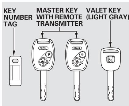
The master key fits all the locks on your vehicle. The valet key works only in the ignition and the driver's door lock. You can keep the glove box locked when you leave your vehicle and the valet key at a parking facility.
