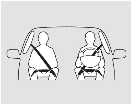
In addition, your vehicle has side curtain airbags to help protect the heads of the driver, front passenger, and passengers in the outer rear seating positions during a moderate to severe side impact or rollover (see page 30 for more information on how your side curtain airbags work).
