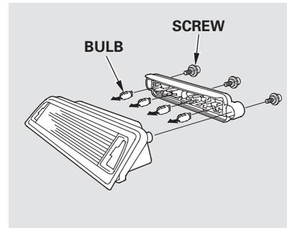
4. Remove the three mounting screws from the light assembly.
