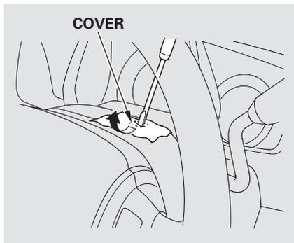
4. Insert the built-in key into the shift lock release slot.
