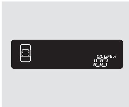
4. Press the TRIP/RESET button for another 5 seconds. The maintenance item code(s) will disappear, and the engine oil life will reset to "100."
