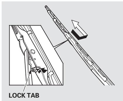
3. Disconnect the blade assembly from the wiper arm:
