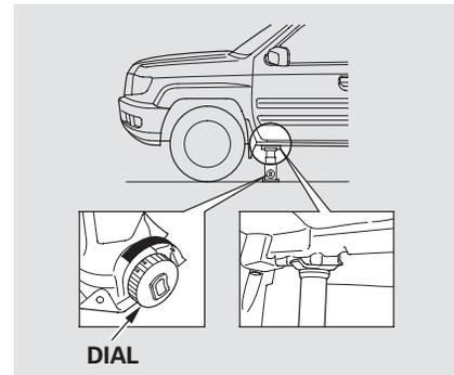
10. Turn the dial at the bottom of the jack clockwise until the top of the jack contacts the jacking point. Make sure the jacking point tab is resting in the jack notch.
