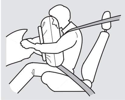
If you ever have a moderate to severe frontal collision, sensors will detect the vehicle's rapid deceleration.
