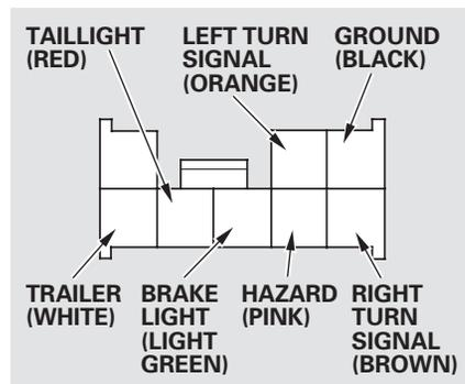
Your vehicle has a trailer lighting connector located behind the left side panel in the cargo area. Refer to the drawing above for the wiring color code and purpose of each pin.
