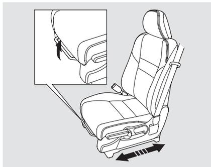
To adjust the seat forward or backward, pull up on the bar under the seat cushion's front edge. Move the seat to the desired position, and release the bar. Try to move the seat
