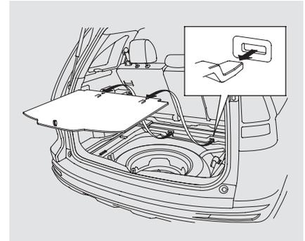
3. Open the tailgate. Raise the cargo area floor lid by lifting up with the strap, and remove it from cargo area by disengaging the tabs.
