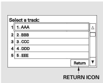
To scroll through the display, touch the ▲ or ▼ icon on the side of the screen. To go back to the previous display, touch the Return icon.
