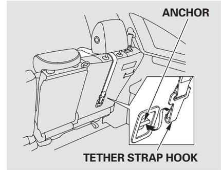
3. Attach the tether strap hook to the anchor, making sure the tether strap is not twisted.
