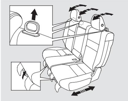
To adjust the seats forward and backward, pull up on the lever under the seat cushion. After moving the seat, make sure it is locked into position.
