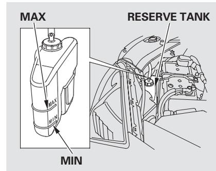
Look at the coolant level in the radiator reserve tank. Make sure it is between the MAX and MIN lines. If it is below the MIN line, see **Adding Engine Coolant** on page 352 for information on adding the proper coolant.
