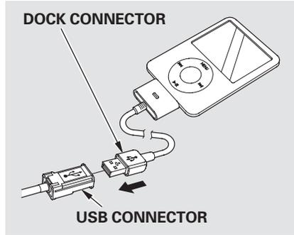
4. Install the dock connector to the USB adapter cable securely.
