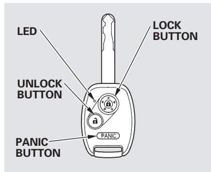
**LOCK** — Press this button once to lock all doors and the tailgate. Some exterior lights will flash once. When you push **LOCK** twice within 5 seconds, you will hear a beep to verify that the doors and the tailgate are locked and the security system (if equipped) has set. You cannot lock the doors and the tailgate if any door or the tailgate is not fully closed or the key is in the ignition switch.
