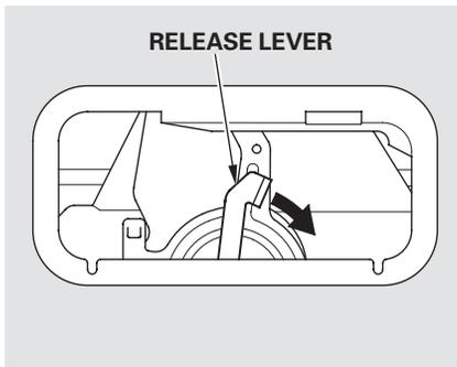
Push the release lever to the lower right as shown.
