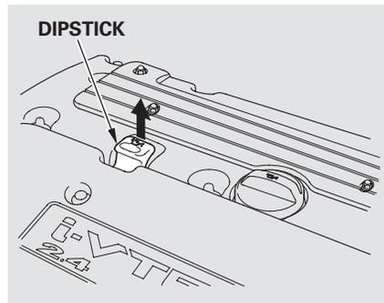
Wait a few minutes after turning the engine off before you check the oil.
