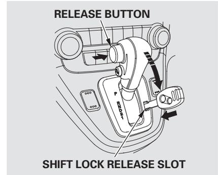
6. Remove the key from the shift lock release slot, then reinstall the cover. Make sure the notch on the cover is on the right side. Insert the key into the ignition switch, press the brake pedal, and restart the engine.
