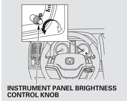
You can change the instrument panel brightness only when the light switch is on. Turn the knob on the lower part of the instrument panel to adjust the brightness. You will hear a beep when maximum or minimum brightness is reached.
