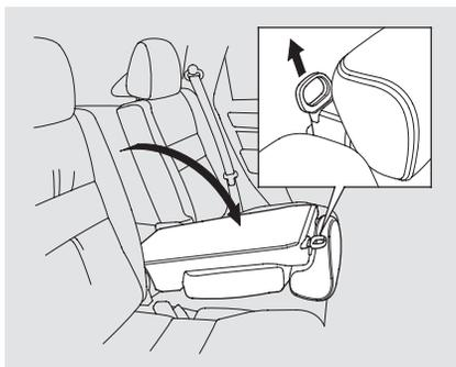
The rear center seat-back has a cargo area pass-through. To use the cargo area pass-through, pull up the release on top of the center seat-back and fold it down.
