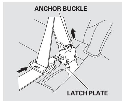
To unlatch the detachable anchor, insert the latch plate into the slot on the side of the anchor buckle. Store the detachable anchor and seat belt latch plates in the retractor housing.
