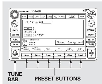
You can use the preset buttons while a disc is playing to select passages and change tracks. Each preset button function is shown on the bottom of the screen.
