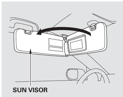
To use the sun visor, pull it down. When using the sun visor for the side window, remove the support rod from the clip, and swing it out.
