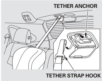
4. Route the tether strap over the seat-back, then attach the tether strap hook to the tether anchor in the ceiling, making sure the strap is not twisted. Tighten the strap according to the seat maker's instructions.
