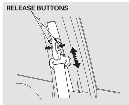
The front seats have adjustable seat belt anchors. To adjust the height of an anchor, press and hold the release buttons, and slide the anchor up or down as needed (it has four positions).
