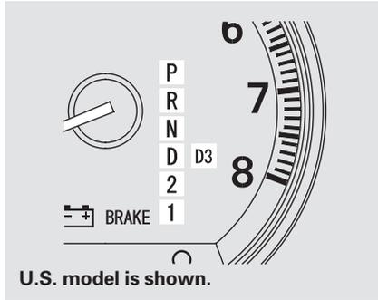
These indicators on the instrument panel show which position the shift lever is in.
