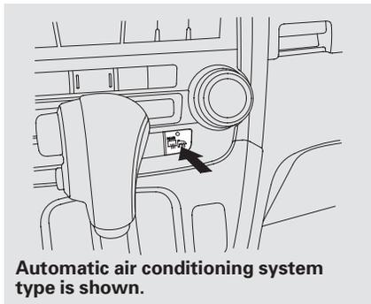
The rear window defogger will clear fog, frost, and thin ice from the window. Push the defogger button to turn it on and off. The indicator in the button comes on to show the defogger is on. It also shuts off when you turn off the ignition switch. You have to turn the defogger on again when you restart the vehicle.
