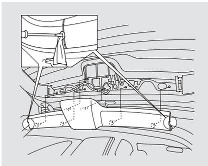
2. Place a cloth on the side edge of the cover to prevent scratches. Remove the cover by carefully prying on the edge with a small flat-tip screwdriver and pulling the cover off.
