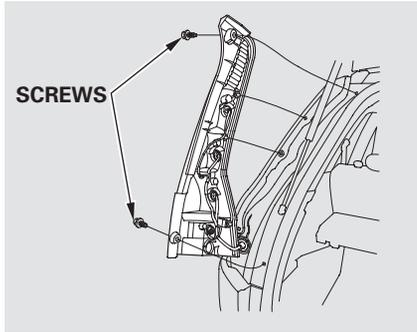
2. Use a Phillips-head screwdriver to remove the taillight assembly mounting screw under each cover.
