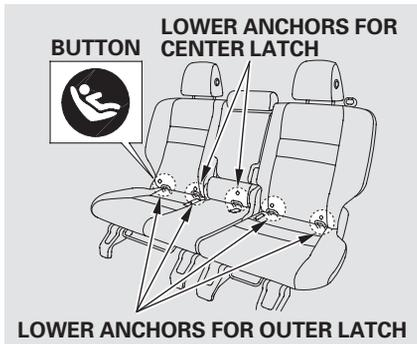
When you install a child seat in the rear center seating position, use the center lower anchors as shown in the illustration. To install a child seat in either outer seating position, use the outer lower anchors. You can install up to two child seats at a time using the outer lower anchors.
