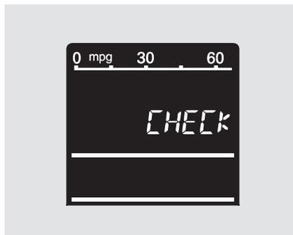
Your vehicle's onboard diagnostic system will detect a loose or missing fuel fill cap as an evaporative system leak. The first time a leak is detected a “CHECK FUEL CAP” message appears on the information display.
