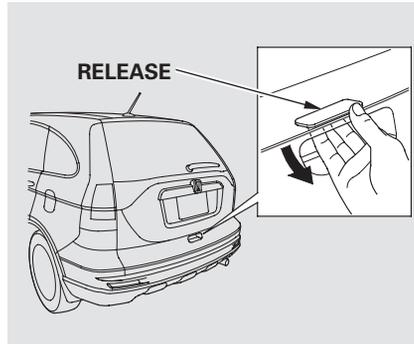
To open the tailgate, push the release, and lift up. To close the tailgate, use the tailgate handle to lower it, then press down on the back edge.
