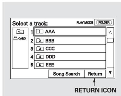
To scroll through the display, touch the ▲ or ▼ icon on the side of the screen. To go back to the previous display, touch the Return icon.
