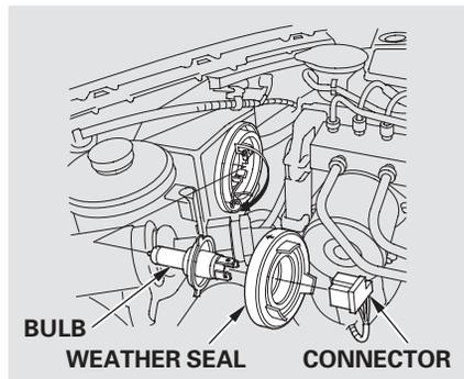
2. Remove the electrical connector from the bulb by pulling the connector straight back.
