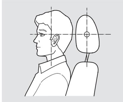
They are most effective when you adjust them so the center of the back of the occupant's head rests against the center of the restraint.
