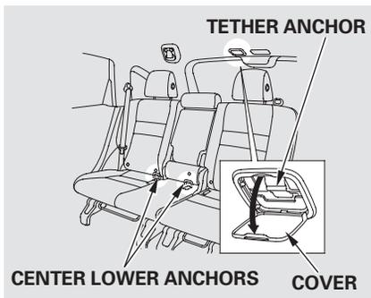
To install a LATCH-compatible child seat in the rear center seating position, use the center lower anchors as shown above.
