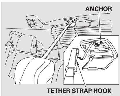
3. Route the tether strap over the seat-back, then attach the tether strap hook to the anchor, making sure the tether strap is not twisted.
