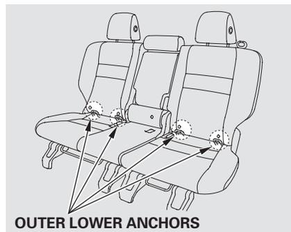
To install a LATCH-compatible child seat in either of the rear outer seats:
