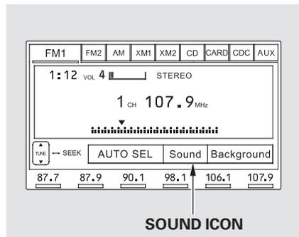
You can adjust the sound on the navigation screen. To adjust the sound, push the AUDIO button, then enter the sound grid by touching the SOUND icon on the display.
