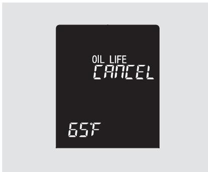
To adjust the outside temperature display, press and hold the select/reset knob for 10 seconds. The display changes as shown above. Select the outside temperature indicator by turning the select/reset knob. The display begins to blink. Push the same knob to enter this setting, then turn it to adjust the temperature. The following sequence will appear for each: 0, 1, 2, 3, 4, 5, -5, -4, -3, -2, -1, 0 (U.S.) or 0, 1, 2, 3, -3, -2, -1, 0 (Canada).
