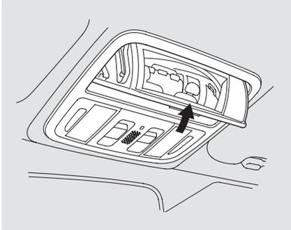
The sunglasses holder uses a convex mirror for its bottom panel. You can see all the vehicle passengers in this mirror. To use the mirror, open the sunglasses holder fully, push it to the first detent, and release it.
