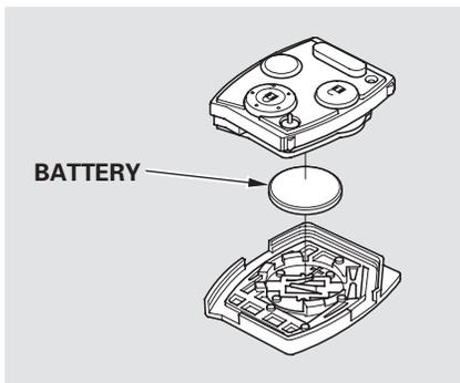
4. Remove the old battery and note the polarity. Make sure the polarity of the new battery is the same (+ side facing down), then insert it in the keypad.
