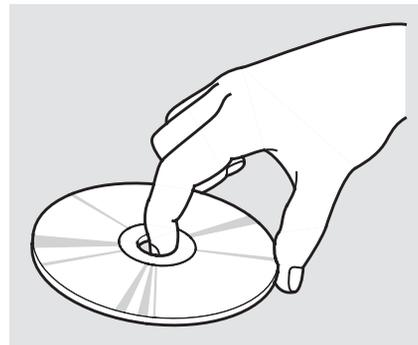
Handle a disc by its edges; never touch either surface. Do not place stabilizer rings or labels on the disc. These, along with contamination from fingerprints, liquids, and felt-tip pens, can cause the disc to not play properly, or possibly jam in the drive.
