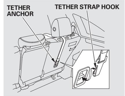
6. Route the tether strap over the seat-back and through the legs of the head restraint, then attach the tether strap hook to the anchor, making sure the tether strap is not twisted.
