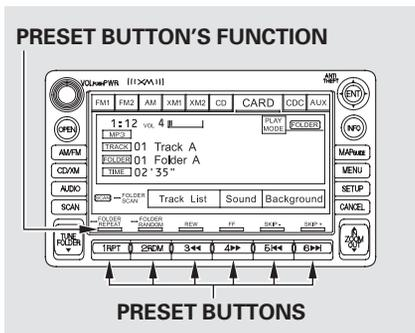
You can use the preset buttons while a card is playing to select or change files. Each preset button's function is shown on the bottom of the screen.
