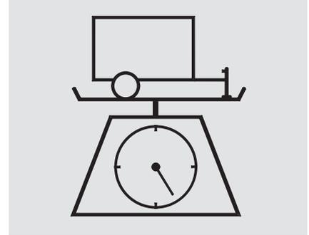
**Total Trailer Weight:** The maximum allowable weight of the trailer and everything in or on it must not exceed 1,500 lbs (680 kg). Towing a load that is too heavy can seriously affect your vehicle's handling and performance. It can also damage the engine and drivetrain.
