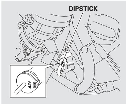
Check the fluid level with the engine at normal operating temperature.
