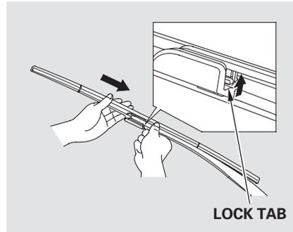
2. Disconnect the blade assembly from the wiper arm:
