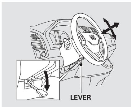
3. Push the lever up to lock the steering wheel in position.
