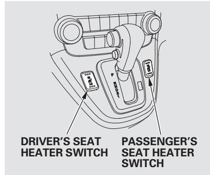
The ignition switch must be in the ON (II) position to use the heaters. Push the top of the switch, HI, to rapidly heat up the seat. After the seat reaches a comfortable temperature, select LO by pushing the bottom of the switch. This will keep the seat warm.
