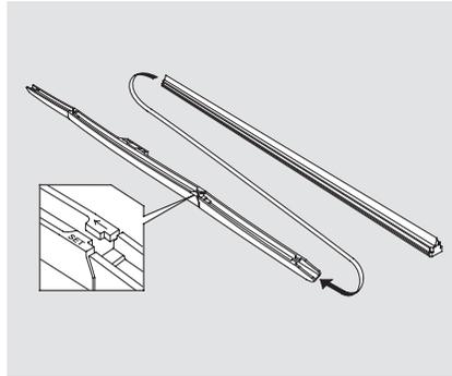
5. Place the top of the wiper blade on the end of the blade assembly, and slide the blade onto the assembly in the direction pointed to by the arrow. Make sure the blade is completely installed.
