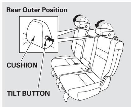
To pivot the outer head restraint down for better visibility, press the tilt button on the side of the head restraint. It folds down forward. To raise the head restraint, pivot it up by hand. Make sure the head restraint locks in position.
