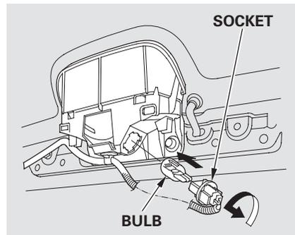
4. Pull the bulb straight out of its socket. Push the new bulb straight into the socket until it bottoms.
