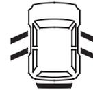
The appropriate indicator comes on in this display if the tailgate or any door is not closed tightly.
