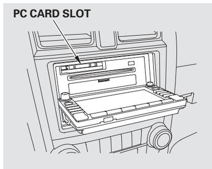
The PC card slot is behind the navigation screen. To use the PC card player, press the OPEN button beside the screen. The screen folds back, and the PC card slot appears.
