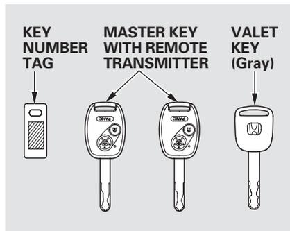
The master key fits all the locks on your vehicle. The valet key works only in the ignition and the driver's door lock. You can keep the glove box locked when you leave your vehicle and the valet key at a parking facility.
