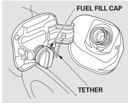
3. Remove the fuel fill cap slowly. You may hear a hissing sound as pressure inside the tank equalizes. The fuel fill cap is attached to the fuel filler with a tether. Place the cap in the holder on the fuel fill door.
