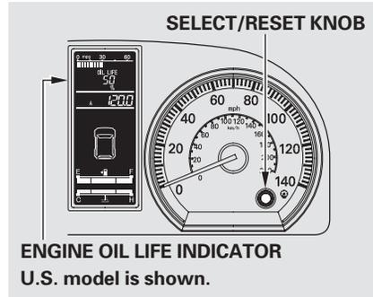
To see the current engine oil life, turn the ignition switch to the ON (II) position, then press and release the select/reset knob repeatedly until the engine oil life indicator appears (see page 69).
