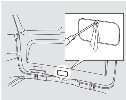
If the power door lock system cannot unlock the tailgate, unlock it manually.
