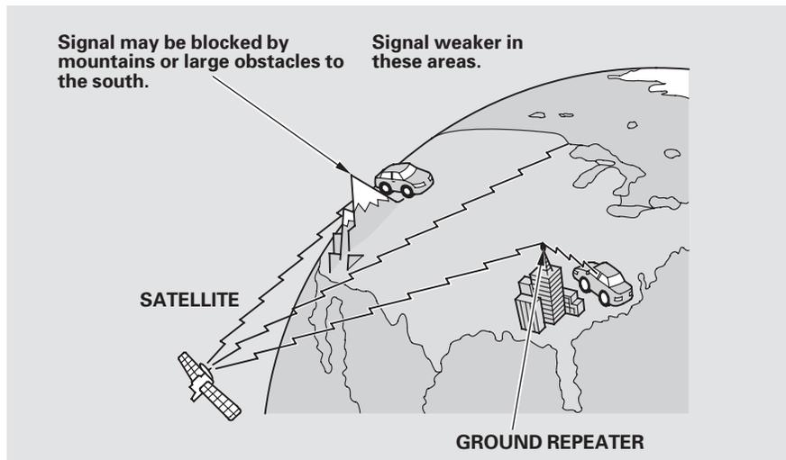
The XM satellites are in orbit over the equator; therefore, objects south of the vehicle may cause satellite reception interruptions. To help compensate for this, ground-based repeaters are placed in major metropolitan areas.
