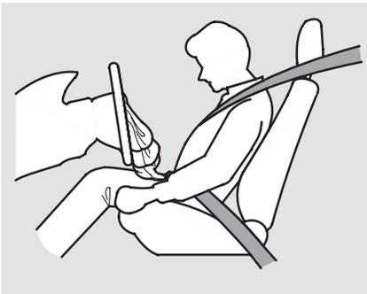
After inflating, the front airbags immediately deflate, so they won't interfere with the driver's visibility, or the ability to steer or operate other controls.
