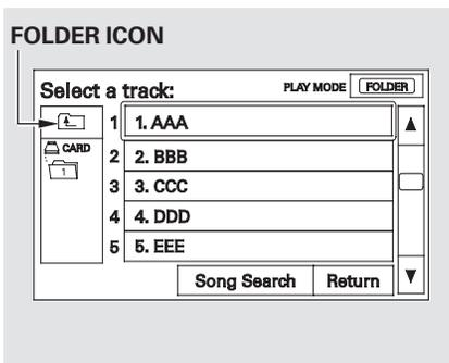
To select a folder, touch its icon on the screen. The display changes to the file list. Then, select and touch a desired file. In folder mode, touch the folder icon on the upper left of the screen to move to the parent folder.
