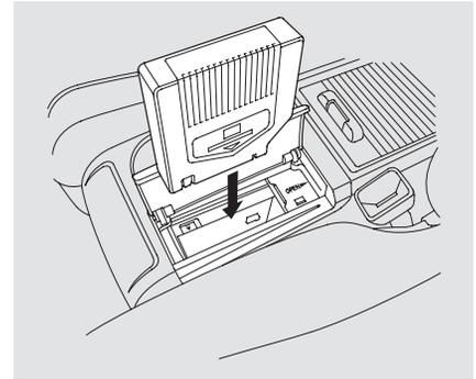
6. Store all six trays in the magazine, and reinstall the magazine in the CD changer as shown.
