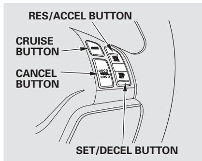
1. Push the CRUISE button on the steering wheel. The CRUISE MAIN indicator on the instrument panel comes on.
