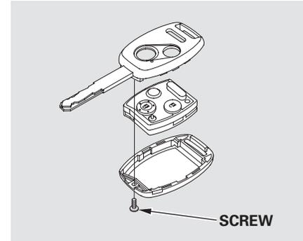
1. Remove the screw at the base of the transmitter with a small Phillips-head screwdriver.
