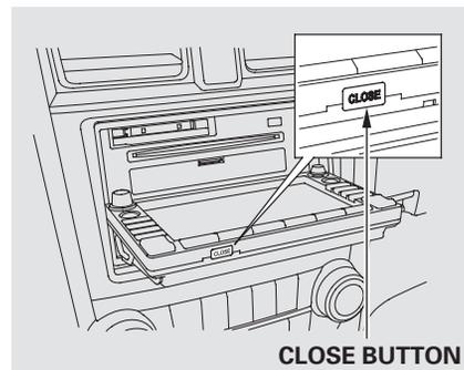
To return the screen to the upright position, press the CLOSE button on the edge of the screen panel. Do not use the folded down screen as a tray. If you put a cup, for example, on the screen, the liquid inside the cup may spill on the screen when you go over a bump.
