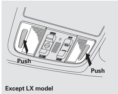
The spotlights (with the switch in the DOOR position) also come on when you unlock the door with the key or the remote transmitter, and when you remove the key from the ignition switch.
