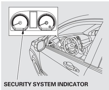
Once the security system is set, opening any door without using the key or the remote transmitter, the hood, or the tailgate will cause the system to alarm.
