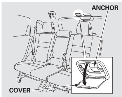
1. Remove the rear center head restraint, and store it in the cargo area.
