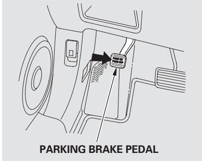
To apply the parking brake, push the pedal down with your foot. To release it, push on the pedal again. The parking brake indicator on the instrument panel should go out when the parking brake is fully released (see page 62).
