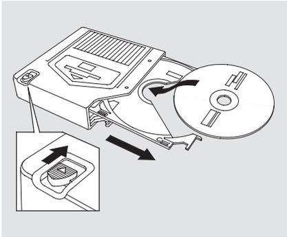
3. To install a CD into the magazine, push the button while pulling out on the tab.
