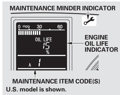
If the remaining engine oil life is 15 to 6 percent, you will see the engine oil life indicator every time you turn the ignition switch to the ON (II) position. The Maintenance Minder indicator will also come on, and the maintenance item code(s) for other scheduled maintenance items needing service will be displayed below the engine oil life indicator.
