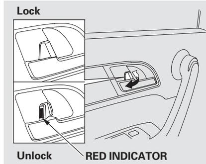
The lock tab on any passenger's door locks and unlocks that door.
