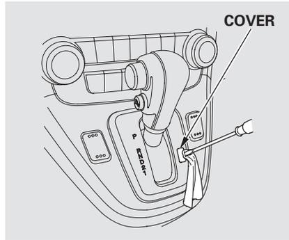
4. Insert the key in the shift lock release slot.
