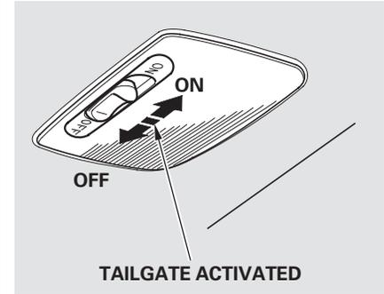
The cargo area light has a three-position switch. In the OFF position, the light does not come on. In the center position, it comes on when you open the tailgate. In the ON position, it stays on continuously.
