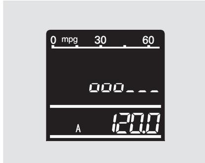
To reduce glare at night, the instrument panel illumination dims when you turn the light switch to  $\Rightarrow \odot \Leftarrow$  or  $\equiv \odot$ . Turning the select/reset knob fully to the right until you hear a beep will cancel the reduced brightness.
