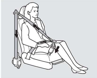
For added protection, the front seat belts are equipped with automatic seat belt tensioners. When activated, the tensioners immediately tighten the belts to help hold the driver and a front passenger in position.
