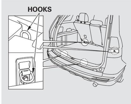
The four hooks on the floor can be used to install a net for securing items.
