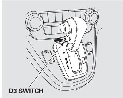
Press the D3 switch on the side of the shift lever to turn this mode on or off; the D3 mode indicator comes on whenever the D3 mode is selected.
