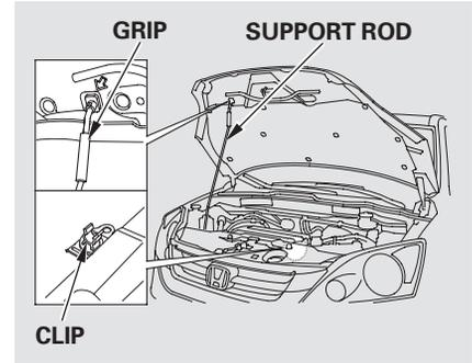
3. Holding the grip, pull the support rod out of its clip. Insert the end into the hole in the hood designated by an arrow.
