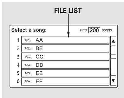
After the system searches for a song, a file list is displayed. To scroll through the list, touch the ▲ or ▼ icon on the side of the screen. Select the desired file by touching the appropriate icon, or moving the joystick and pressing ENT.
