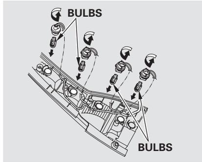
4. Determine which of the four bulbs is burned out: stop/taillight, back-up light, turn signal, or side marker.
