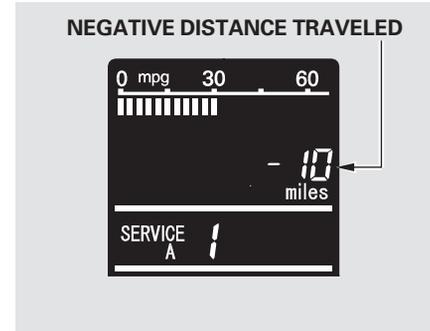
If you do not perform the indicated maintenance, negative distance traveled is displayed and begins to blink after the vehicle has been driven 10 miles (10 km) or more.
