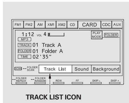
You can also select a file directly from the folder and track lists on the audio display. Press the AUDIO button to show the audio display, then touch the Track List icon. The folder list menu appears on the display.
