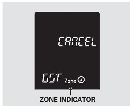
2. Select the zone indicator by turning the select/reset knob. The display begins to blink. Push the same knob to enter this setting.
