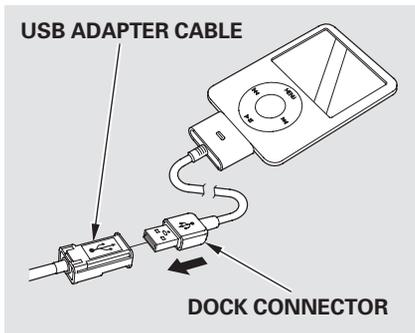
3. Connect your dock connector to the iPod correctly and securely.
