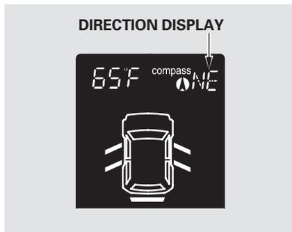
Next to the outside temperature indicator of the information display, a compass indicates which direction your vehicle is pointed. It indicates eight directions.
