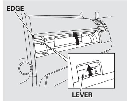
Open the upper glove box by pushing up the lever. Close it by pulling down on the edge under the lever.
