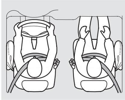
Your vehicle also has side airbags to help protect the upper torso of the driver or a front seat passenger during a moderate to severe side impact (see page 29 for more information on how your side airbags work).
