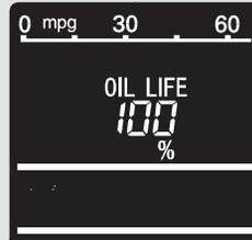
5. The engine oil life and the maintenance item code(s) will begin to blink. Press the select/reset knob for another 5 seconds.
