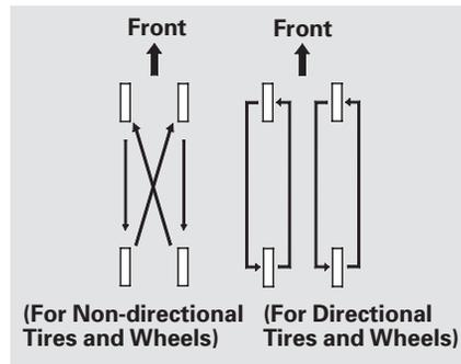
To help increase tire life and distribute wear more evenly, rotate the tires according to the maintenance messages displayed on the information display. Move the tires to the positions shown in the diagram each time they are rotated. If you purchase directional tires, rotate only front-to-back. When the tires are rotated, make sure the air pressures are checked.
