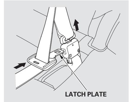
When you are folding the rear center seat-back, use the latch plate to release the center seat belt from the detachable anchor (see page 109). Allow the seat belt to retract into the holder on the ceiling and store the buckles in it.
