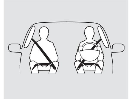
In addition, your vehicle has side curtain airbags to help protect the heads of the driver, front passenger, and passengers in the outer rear seating positions during a moderate to severe side impact or rollover (see page 31 for more information on how your side curtain airbags work).
