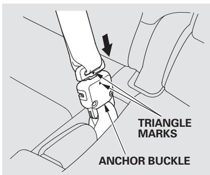
Line up the triangle marks on the small latch plate and anchor buckle when reattaching the belt and buckle.
