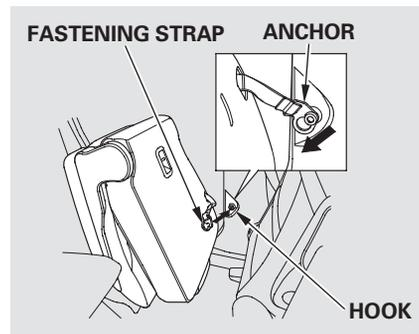
5. Pull down on the anchor to engage the upper part of the anchor securely on the hook, and make sure the seat is secure.
