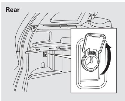
Make sure to put the socket cover back in place to prevent any small foreign objects from getting into the socket.
