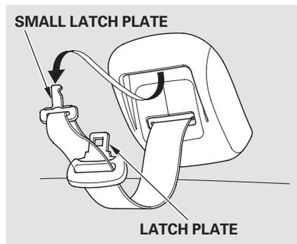
Pull out the small latch plate and the latch plate from each holding slot in the ceiling, and pull out the seat belt to extend it.
