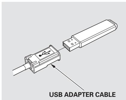
3. Connect the USB flash memory device to the USB connector correctly and securely.
