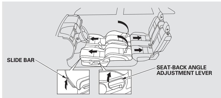
You can recline the seat-backs on the front seats so they are level with the rear seat cushions, making a large cushioned area. To do this:
