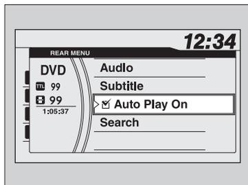
Press the **REAR SOURCE** button on the front panel while a DVD is playing and display **REAR MENU** in front. Rotate to select DVD Setup, then press .
