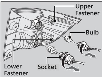
3. Slowly pull out the assembly to release the lower fastener from the grommet, using your fingers.
