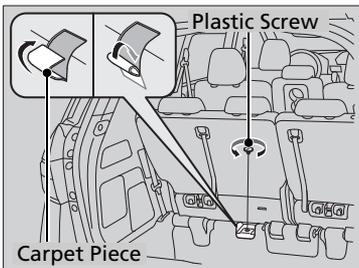
2. Pull down the U-shaped carpet piece, fold it, and tuck the end under the carpet.
