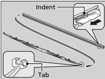
**5.** Slide the new wiper blade onto the holder from the bottom end.
