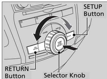
Press the SETUP button, and rotate
