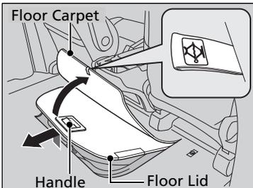
1. Remove the floor mat under the second row seat.
