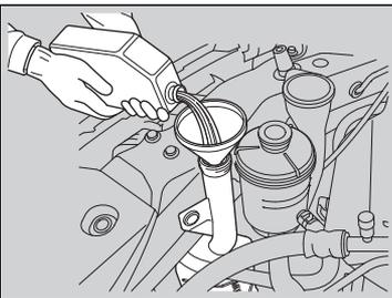
2. If the coolant level is below the MIN mark, add the specified coolant until it reaches the MAX mark.
