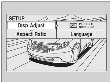
Press the SETUP button while the DVD is playing to see the available options. Use the ▲, ▼, ▶, and ◀ buttons to highlight the option and then press the ENTER button.
