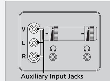
The system also allows for auxiliary inputs from standard video games. The jacks are above the third row seat armrest on the driver's side.
