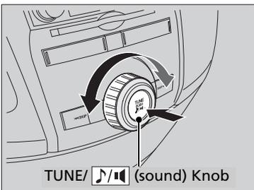
Press and rotate to adjust the setting.
