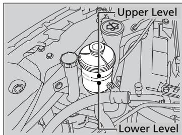
1. Look at the side of the reservoir. The fluid should be between the UPPER LEVEL and LOWER LEVEL.
