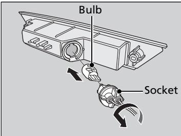
2. Turn the socket to the left and remove it.
