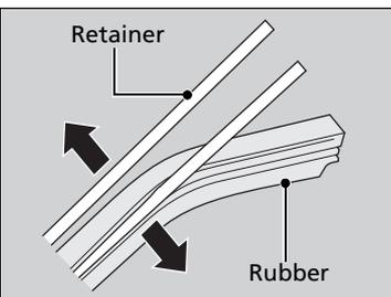
4. Remove the retainers from wiper blade and mount it to a new rubber blade.
