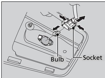
2. Remove the license plate light assembly by squeezing the tabs on both sides of the socket.
