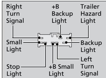
Your trailer lighting connector is located behind the left side panel in the cargo area. Each pin's purpose and wiring color code are shown in the image.
