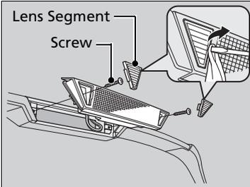
1. Remove the lens segment by prying on the edge using a flat-tip screwdriver.
