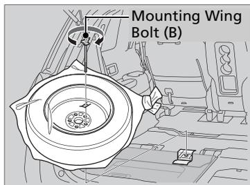
3. Place the flat tire face down on the attachment point.
