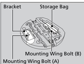
The storage bag, bracket, mounting wing bolt (A) and mounting wing bolt (B) are in the tool case.
