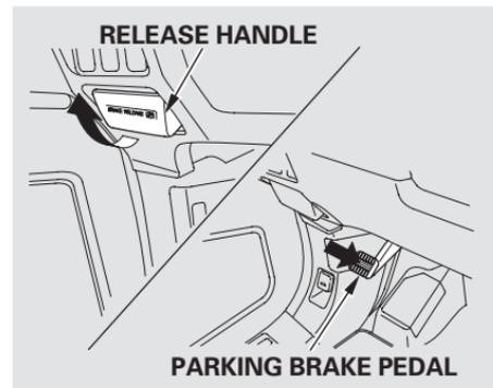
To apply the parking brake, push the pedal down with your foot. To release it, pull the release handle fully. The parking brake indicator on the instrument panel should go out when the parking brake is fully released (see page 65).
