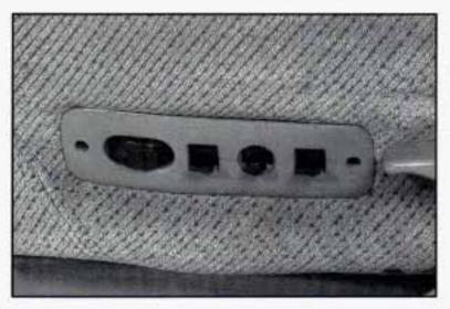
If your vehicle has a power seat on the driver's side, you can adjust it with this switch at the outside edge of the seat.
