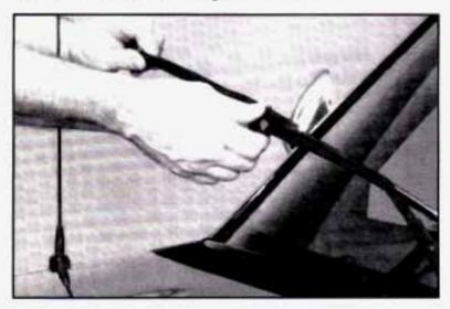
To replace the windshield wiper blade insert, lift the wiper arm and rotate the blade until it is facing away from the windshield.
