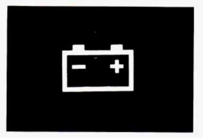
The red Charging System Warning light should come on briefly when you turn on the ignition, before starting the engine, as a check to show you it is working. After the engine starts, the light should go out. If it stays on or comes on while you are driving, you may have a problem with your charging system. It could indicate a problem with the alternator drive belt, or some other charging system problem. Have it checked right away. Driving while this light is on could drain your battery.
