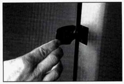
To open a rear swing-out window, just flip the latch open and swing the glass out.
