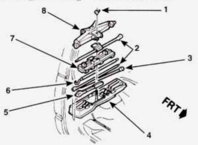
1. Nut5. Ratchet2. Jack Handle Extension6. Jack Handle3. Wheel Wrench7. Tool Retainer4. Jack and Tool Storage Box8. Jack
