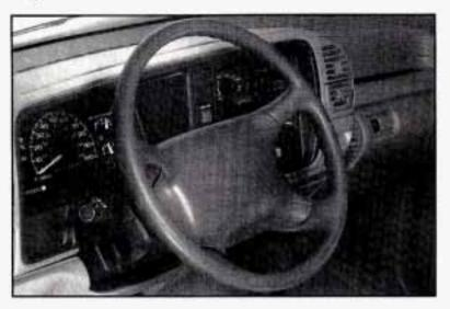
Your vehicle may have an air bag for the driver. If it does, it will say Supplemental Inflatable Restraint on the middle part of the steering wheel.
