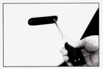
Remove the screws and take the fender marker assembly out of the fender.
