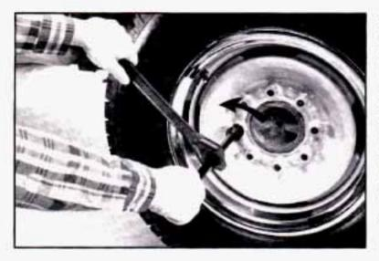
Now, use the ratchet and wheel wrench to loosen all the wheel nuts. Turn the wheel wrench counterclockwise, with DOWN facing you, to loosen the wheel nuts.
