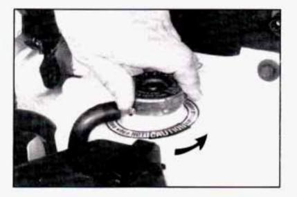
You can remove the coolant surge tank pressure cap when the cooling system, including the coolant surge tank pressure cap and upper radiator hose, is no longer hot. Turn the pressure cap slowly to the left until it first stops. (Don't press down while turning the pressure cap.)
