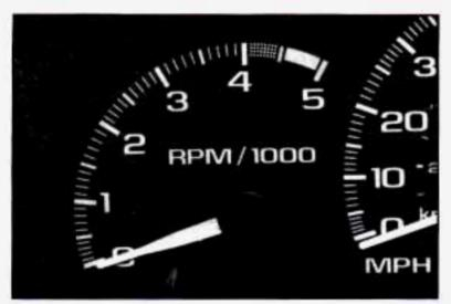
Your tachometer displays the engine speed in revolutions per minute (rpm).
