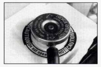
The surge tank pressure cap must be tightly installed with the arrows on the cap lined up with the top tube of the coolant surge tank.
