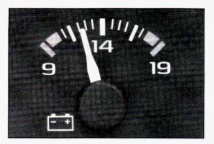
When your engine is not running, but the ignition is in the RUN position, this gage shows your battery's state of charge in DC volts.
