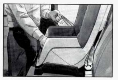
Pull the rest of the lap belt all the way out of the retractor to set the lock.
