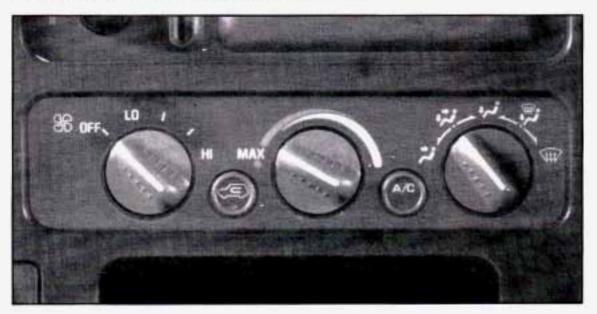
If your vehicle has air conditioning, your heater/air conditioning controls will look like this. Before using your vehicle's air conditioning, open the windows to clear the vehicle of hot air.
