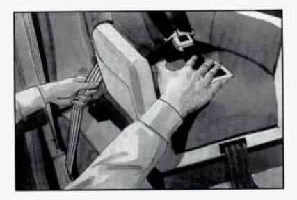
To tighten the belt, feed the lap belt back into the retractor while you push down on the child restraint.
