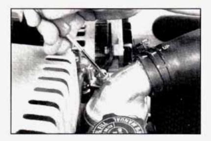
After the engine cools, open the air bleed valve on the thermostat housing.
