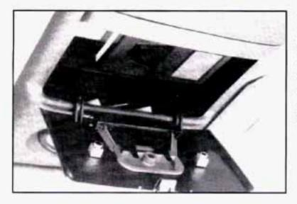
The pegs inside the compartment door are used to make sure the button on the compartment door will contact the control button on the garage door opener.
