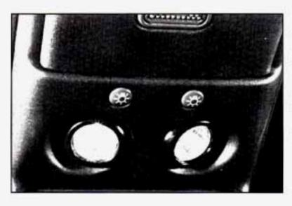
If your vehicle has an overhead console with reading lamps, press the button next to the lamp to turn the lamp on.
