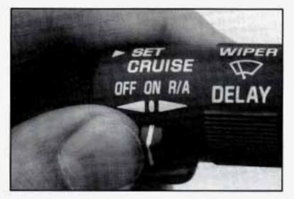
Move the Cruise Control switch to ON.
