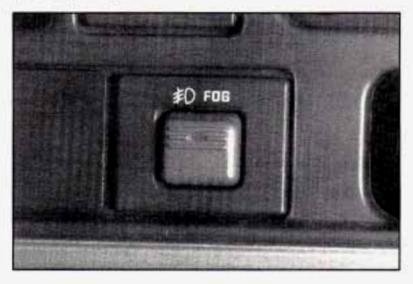
The fog lamp switch is on the lower edge of your instrument panel.
