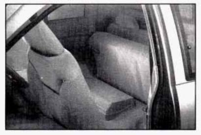
To use the seat, pull the entire seat forward until it is flat. Then, pull forward on the RELEASE lever at the side of the seat cushion, located behind the passenger side front seat. Push the seatback rearward until it latches.
