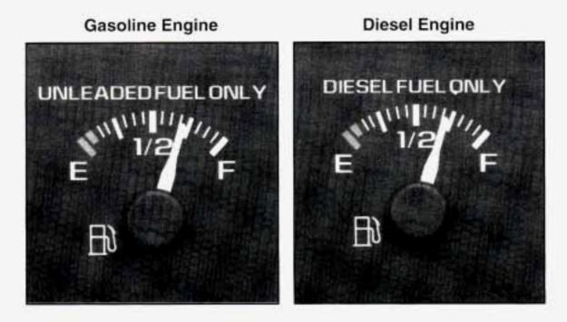
The fuel gage, when the ignition is on, tells you about how much fuel you have left in your tank. The gage will first indicate empty before you are out of fuel, and you should get more fuel as soon as possible.
