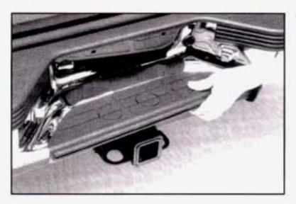
To remove the pad, lift the edge of the pad from the rear of the bumper and swing it forward. When the pad releases from the bumper holes, lift the pad off.
