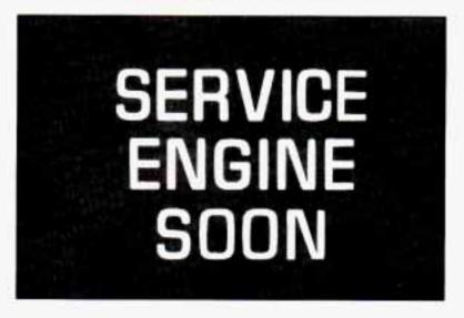
A computer monitors the operation of your fuel, ignition and emission control systems. This orange light should come on when the ignition is on but the engine is not running, as a check to show you it's working. If it does not come on at all, have it fixed right away. If it stays on, or comes on while you are driving, the computer is indicating that you have a problem. You should take your vehicle in for service soon.
