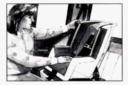
To tighten the belt, pull up on the shoulder belt while you push down on the child restraint.
