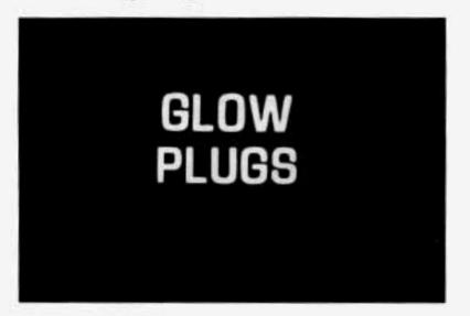
If you have a diesel engine, it has a special starting system. An orange instrument panel Glow Plugs light shows that the system is functioning properly and tells you when the engine is ready to be started. For more details, see "Starting Your Diesel Engine" in the Index.
