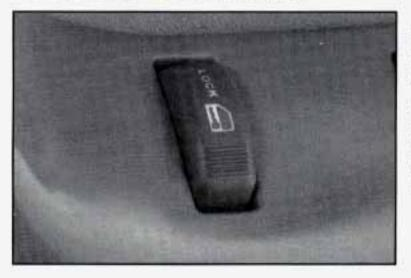
Press the side of the power door lock switch, marked LOCK, on either front door to lock all the doors at once. Press the ribbed side of the switch to unlock all the doors at once.
