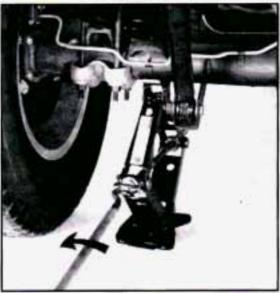
Lower the vehicle by rotating the ratchet and wheel wrench counterclockwise. Lower the jack completely.
