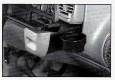
To use the cup holder, pull the handle and slide the cup holder tray open.
