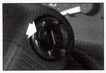
The ignition key cannot be removed from the ignition of manual transmission vehicles unless the key release button is used.
