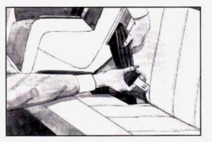
3. Pick up the latch plate, and run the lap and shoulder portions of the vehicle's safety belt through or around the restraint. The child restraint instructions will show you how. Tilt the latch plate to adjust the belt if needed. If the shoulder belt goes in front of the child's face or neck, put it behind the child restraint.
