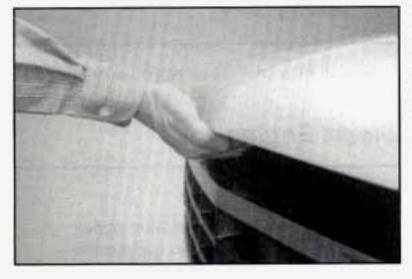
Then go to the front of the vehicle and pull up on the secondary hood release, located just to the passenger side of the center of the grill.
