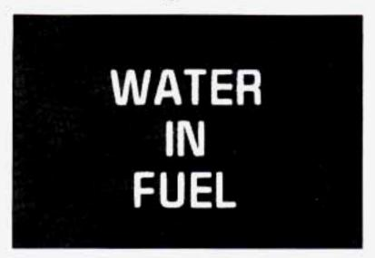
This red light will come on to warn you if there is water in the diesel fuel system. For more information on how this light works, see "Diesel Fuel Requirements and Fuel System" in the Index.
