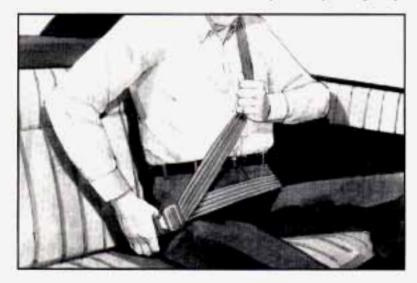
To make the lap part tight, pull down on the buckle end of the belt as you pull up on the shoulder part.
