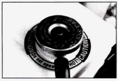
Then replace the pressure cap. Be sure the arrows on the pressure cap line up like this.
