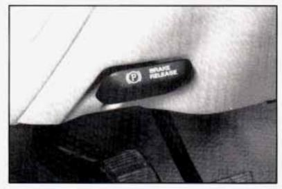
Hold the regular brake pedal down. Pull the lever, located just above the parking brake pedal, marked BRAKE RELEASE, to release the parking brake.
