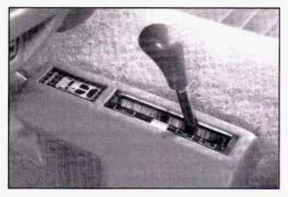
The transfer case shift lever is on the floor to the right of the driver. Use this lever to shift into and out of four-wheel drive.
