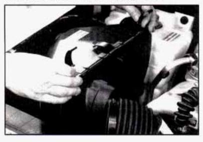
Then, unhook the cover retaining clips and push the rear of the cover toward the engine.
