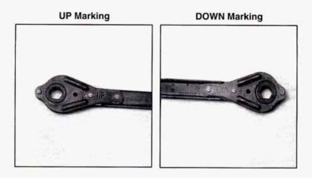
One side of the ratchet has an UP marking. The other side has a DOWN marking.
