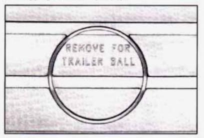
If you will be using the bumper to tow a trailer, you must remove the center cutout circle to install the trailer ball. You must also remove both outer cutouts to attach the trailer safety chains.
