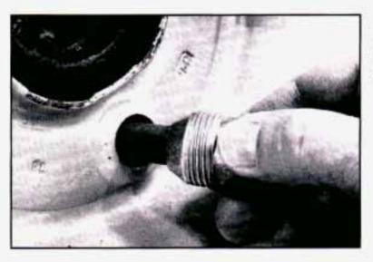
Replace the wheel nuts with the rounded end of the nuts toward the wheel.
