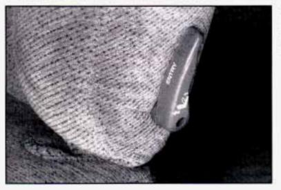
To fold a seatback forward, pull this lever forward and fold the seatback forward.
