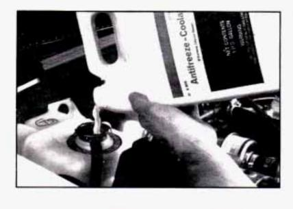
Then fill the coolant surge tank with the proper mix. up to the COLD mark.
