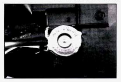
Then replace the pressure cap. At any time during this procedure if coolant begins to flow out of the filler neck, reinstall the pressure cap. Be sure the arrows on the pressure cap line up like this.
