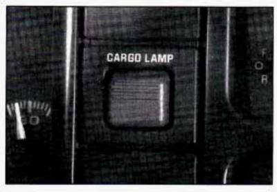
Press the top, ribbed part of the switch to turn the cargo lamp on, and press the bottom of the switch to turn it off.
