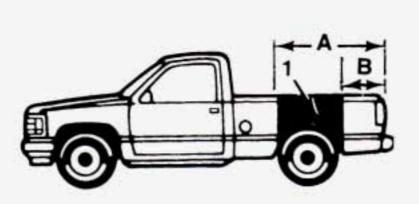
Recommended location for cargo center of gravity for cargo weight rating (Pickup Truck).
