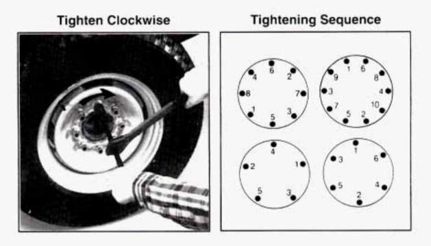
Tighten the nuts firmly in a criss-cross sequence as shown. Rotate the wheel wrench clockwise.
