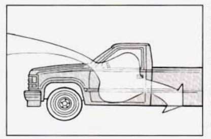
Your vehicle's ventilation system supplies outside air to the inside of your vehicle when it is moving. With the side windows closed, air will flow into the front air inlet grilles, through the vehicle, and out the rear air exhaust valve.
