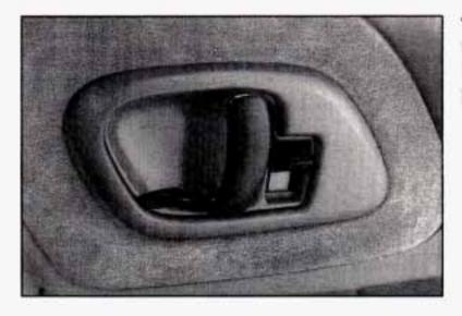
To open the door from the inside, pull the lever toward you and push the door open.
