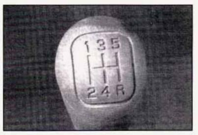
If you have a five speed manual transmission with low gear (RPO MW3), this is your shift pattern. Here's how to operate your transmission:
