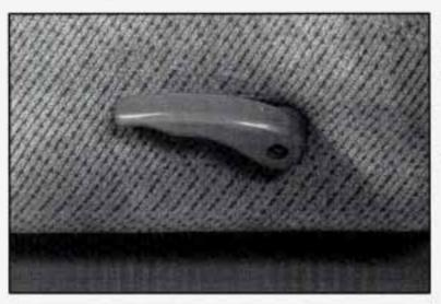
To adjust the seatback, lift the front of this lever.
