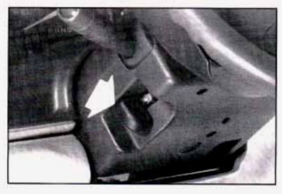
A tilt steering wheel allows you to adjust the steering wheel BEFORE you drive.
