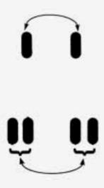
If your vehicle has dual rear wheels and the load range or tread design for your front tires is different from your rear tires, always use the correct rotation pattern shown here when rotating your tires. The dual tires are rotated as a pair, and the inside rear tires become the outside rear tires.
