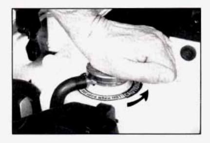
Then keep turning the cap, but now push down as you turn it. Remove the pressure cap.
