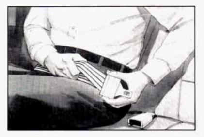
When you sit in a center seating position, you have a lap safety belt, which has no retractor. To make the belt longer, tilt the latch plate and pull it along the belt.
