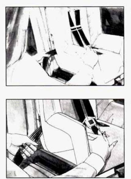
Pull the rest of the lap belt all the way out of the retractor to set the lock.
