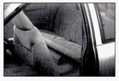
To store the seat, pull forward on the RELEASE lever at the side of the seat cushion, behind the passenger side front seat. Fold the seatback forward until it latches with the seat cushion. Lift the entire seat and push it rearward into place.
