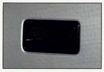
You can open the tailgate by lifting up on its handle while pulling the tailgate toward you.
