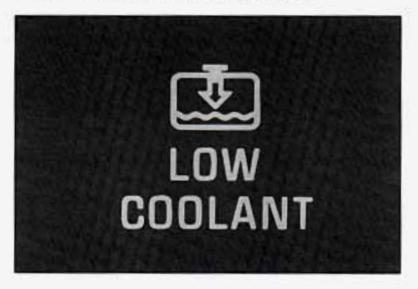
If you have a diesel engine, you have a low coolant light. As a check to show you it's working, this orange light comes on for a few seconds after the ignition is turned on. If this light comes on anytime the engine is running, your system is low on coolant and the engine may overheat. See "Engine Coolant" in the Index and have your vehicle serviced as soon as you can.
