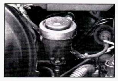
Refer to the Maintenance Schedule to determine how often you should check the fluid level in your clutch master cylinder reservoir and for the proper fluid.
