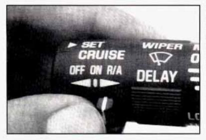
Once you're going about 25 mph (40 km/h) or more, you can move the Cruise Control switch from ON to R/A (Resume/Accelerate) for about half a second.
