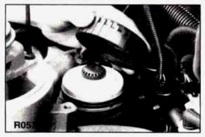
Unscrew and remove the ring nut from the top of the filter head.
