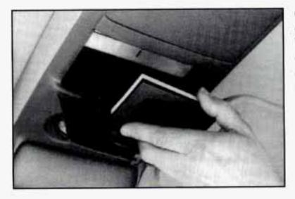
Center the garage door opener activation button over the console door button, and press the opener firmly into place.
