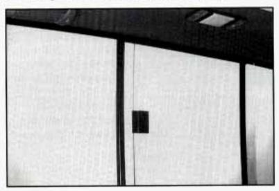
To open the sliding rear window, unlock the latch lever by moving the lever toward the driver's side. Release the lever from the latch plate and slide the window toward the driver's side of the vehicle.
