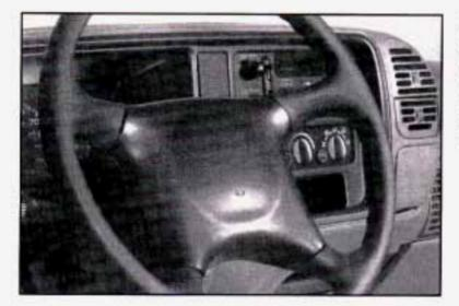
On vehicles not equipped with an air bag, press the pad in the center of the steering wheel to sound the horn.
