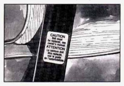
If belts are cut or damaged, replace them. Collision damage also may mean you will need to have safety belt or seat parts repaired or replaced. New parts and repairs may be necessary even if the belt wasn't being used at the time of the collision.
