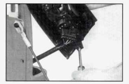
Remove the screws from the bulb retainer and take it off the lamp assembly.
