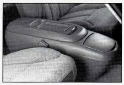
To open it, lift the latch handle and swing the door open.
