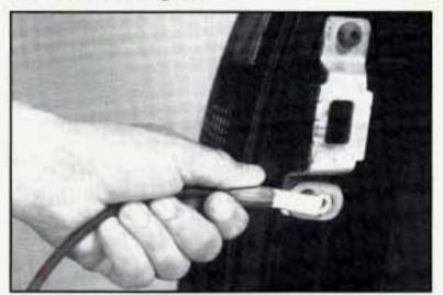
Raise the tailgate slightly and release both retaining cable clips. To release the cable clips, lift the cable so it points straight out and push the cable clips forward.
