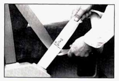
The model number on the replacement belt may be listed on the safety belt you want to replace. Pull the lap belt all the way out to see this label. If there is no model number listed on the safety belt, see your dealer to make sure you get the correct part number for the replacement belt.
