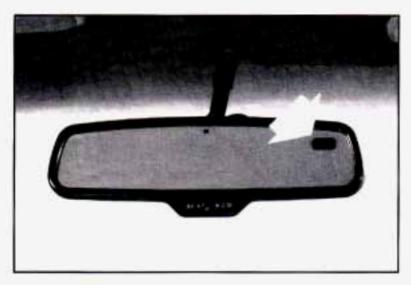
Your vehicle may have an optional electrochromic inside rearview mirror. An electrochromic inside rearview mirror, when on, automatically dims to the proper level to minimize glare from lights behind you after dark.
