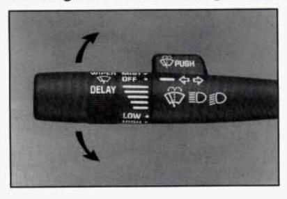
The turn signal has two upward (for right signal) and two downward (for left signal) positions. These positions allow you to signal a turn or a lane change. To signal a turn, move the lever all the way up or down. When the turn is finished, the lever will return automatically.
