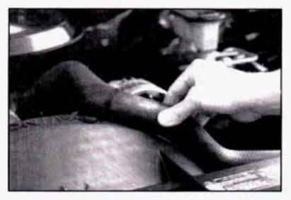
With the coolant surge tank pressure cap off, start the engine and let it run until you can feel the upper radiator hose getting hot. Watch out for the engine fan(s).
