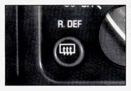
To turn on the rear window defogger, press the rear defog button next to the fan control knob.
