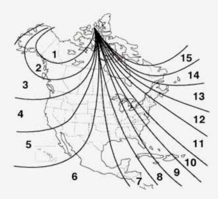
Press and hold the CAL switch until the new zone number appears in the display. After you release the switch, the display will show a compass direction within a few seconds.
