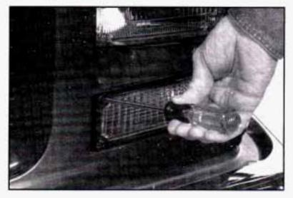
Remove the two screws at the inside edge of the parking/turn signal lamp assembly.
