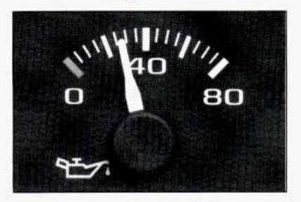
The oil pressure gage shows the engine oil pressure in psi (pounds per square inch) when the engine is running. Canadian vehicles indicate pressure in kPa (kilopascals). Oil pressure may vary with engine speed, outside temperature and oil viscosity, but readings above the low pressure zone indicate the normal operating range.
