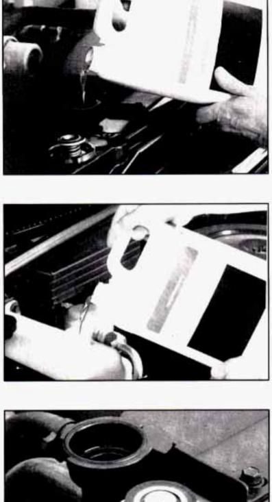
Fill the radiator with the proper mix, up to the base of the filler neck.
