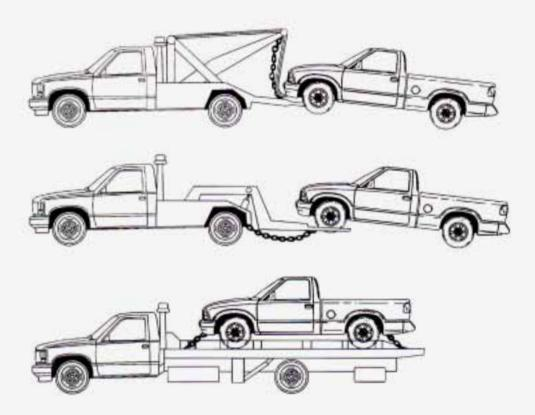
If you have a two-wheel drive vehicle, don't have your vehicle towed on the rear wheels, unless you must. If the vehicle must be towed on the rear wheels, don't go more than 35 mph (56 km/h) or farther than 50 miles (80 km) or your transmission will be damaged. If these limits must be exceeded, then the rear wheels have to be supported on a dolly.
