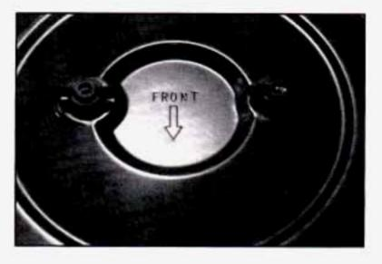
To avoid the possibility of un-filtered air being drawn into the engine, make sure the air cleaner cover is on straight and the wing nuts are properly tightened. If there is an arrow on the air cleaner cover, it should point to the front of the engine.
