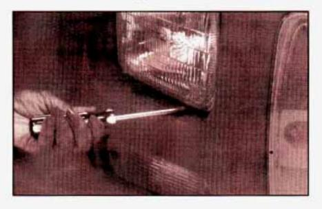
Remove the four screws from the headlamp retainer.
