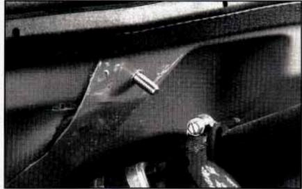
Make your last connection away from the battery, to the engine block, frame or other unpainted metal parts of your vehicle. A ground location has been provided through a stud attached to the body surface.
