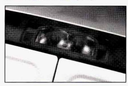
Your vehicle's center high-mounted stoplamp is located above the rear doors at the center of the vehicle.
