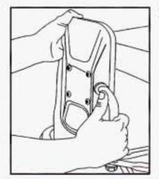
To adjust the mirrors when towing a trailer, rotate the mirror by pushing the mirror head toward the front of the vehicle.
