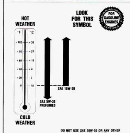
As shown in the chart, SAE 5W-30 is best for your vehicle. However, you can use SAE 10W-30 if it's going to be 0°F (-18°C) or above. These numbers on an oil container show its viscosity, or thickness. Do not use other viscosity oils, such as SAE 20W-50.
