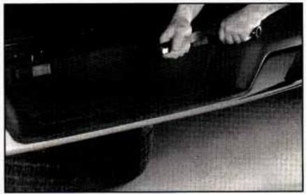
Put the flat end of the extension on an angle through the hole in the rear door frame, above the bumper.
