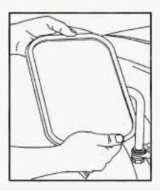
Rotate the mirror head, so that the mirror surface faces the rear of the vehicle.
