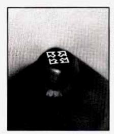
Select the mirror you want to move by rotating the switch to the right to adjust the passenger side mirror and to the left to adjust the driver side mirror. The center position is neutral.
