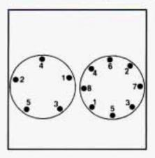
Tighten the nuts firmly in a crisscross sequence as shown.
