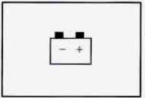
This light should come on briefly when you turn on the ignition, before starting the engine, as a check to show you it is working.
