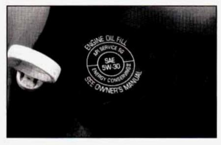
The engine oil filler cap is located between the coolant recovery tank and the air cleaner.
