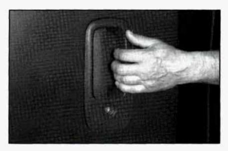
To close the sliding side door from outside, use the outside door handle to slide the door toward the front of the vehicle.
