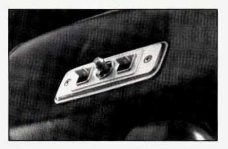
If your vehicle has a power seat on the driver's or passenger's side, you can adjust it with this switch at the front center cushion of the seat.
