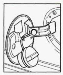
While refueling your vehicle, hang the cap by the tether from the hook on the filler door.
