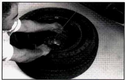
Pull the wheel toward the rear of the vehicle keeping the cable tight.
