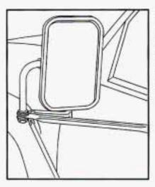
If your vehicle is equipped with the camper-type mirrors, they can be adjusted so you can have a clear view of objects behind you.
