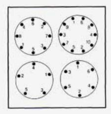
Tighten the nuts firmly in a crisscross sequence as shown by rotating the wheel wrench to the right.
