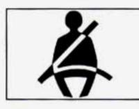
The safety belt light will also come on and stay on for about 20 seconds, then it will flash for about 55 seconds. If the driver's belt is already buckled, neither the tone nor the light will come on.
