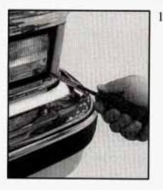
Remove the four screws and take out the parking/turn signal lamp assembly.
