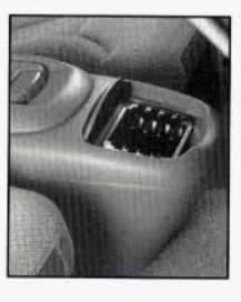
Your vehicle may have a cassette/compact disc holder at the front of the console. The holder will store up to four compact disc cases, up to four cassette tape cases, or any combination of these items that adds up to four.
