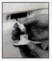
Turn the bulb socket to the left and remove it from the lens assembly.
