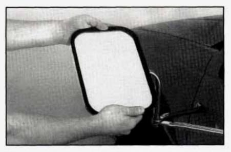
Rotate the mirror head, so that the mirror surface faces the rear of the vehicle.
