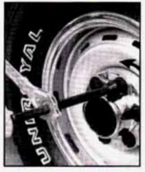
If your vehicle has wheel nut caps, use the wheel wrench and ratchet to remove them. Turn the wheel wrench to the left, with DOWN facing you, to remove the wheel nut caps.
