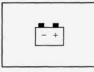
This light should come on briefly when you turn on the ignition, before starting the engine, as a check to show you it is working. After the engine starts, the light should go out. If it stays on or comes on while you are driving, you may have a problem with your charging system. It could indicate a problem with the generator drive belt, or some other charging system problem. Have it checked right away. Driving while this light is on could drain your battery.
