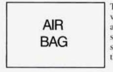
This light will come on when you start your engine, and it will flash for a few seconds. Then the light should go out. This means the system is ready.
