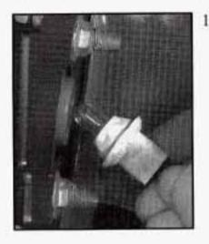
Remove the four screws and pull out the parking/turn signal lamp assembly.
