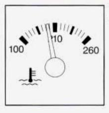
This gage shows the engine coolant temperature.
