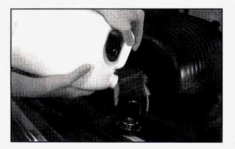
Fill the radiator with the proper DEX-COOL<sup>®</sup> coolant mixture, up to the base of the filler neck. (See "Engine Coolant" in the Index for more information about the proper mixture.)
