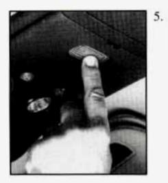
Now, with the compartment door closed, press the button marked PUSH again to make sure the garage door opener operates properly.
