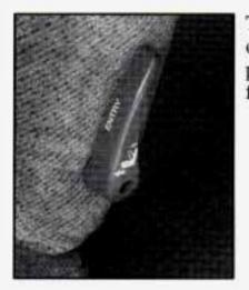
To fold a front split bench or bucket seatback forward, pull this lever forward and fold the seatback forward.
