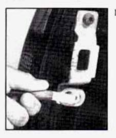
Raise the tailgate slightly and release both retaining cable clips. To release the retaining cable clips, pull the retaining cable clip away from the cable end. Lift the cable so it points straight out and push the cable clips forward.
