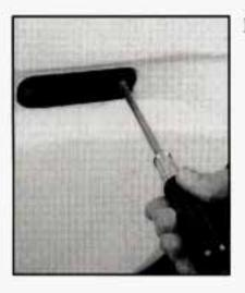
Remove the screws and take the fender marker assembly out of the fender.
