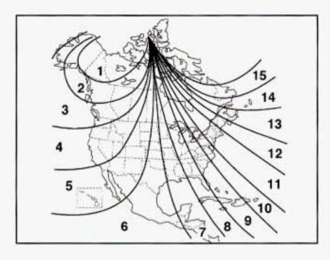
Press the COMP button on the bottom of the mirror until the new zone number appears in the display. After you stop pressing the button in, the display will show a compass direction within a few seconds.
