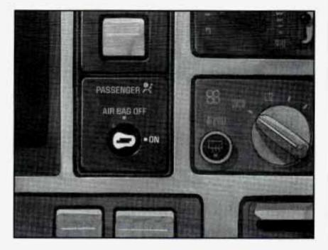
If your vehicle has air bags, there is a switch on the instrument panel that you can use to turn off the right front passenger's air bag. But use this switch only when you want to secure a rear-facing child restraint at the right front passenger's position.
