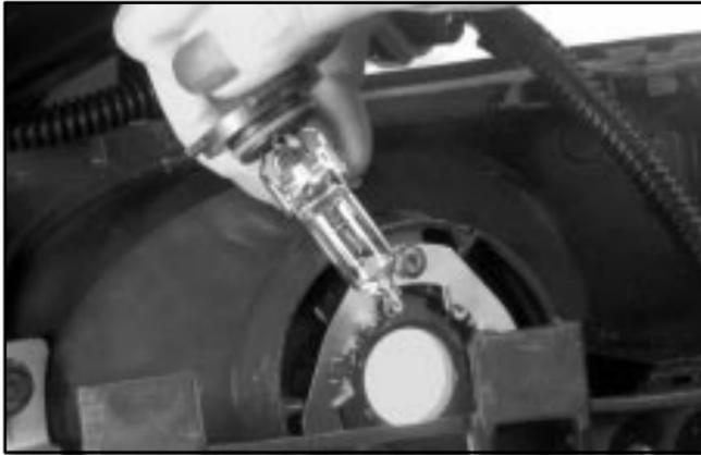
5. Turn the bulb assembly counterclockwise to remove it.
