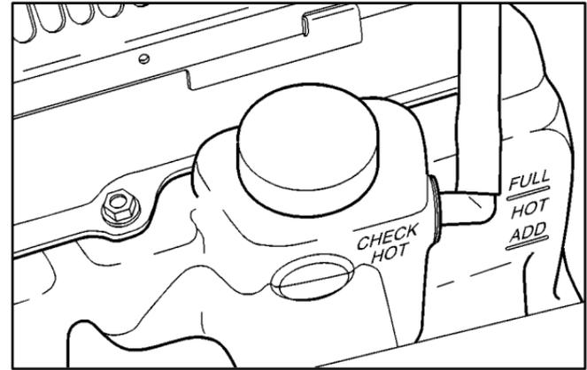
When the engine is cold, the coolant level should be at least up to the ADD mark. If it isn't, you may have a leak in the radiator hoses, heater hoses, radiator, water pump or somewhere else in the cooling system.
