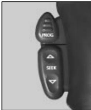
**PROG:** Press this button to play a station you have programmed on the radio preset buttons on the selected band.
