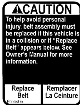
If you ever see a label on the driver's or the right front passenger's safety belt that says to replace the belt, be sure to do so. Then the new belt will be there to help protect you in a collision. You would see this label on the belt near the door opening.
