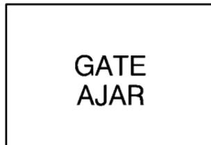
If this light comes on, your liftgate or liftglass is ajar. Try closing the liftgate or liftglass again. Never drive with the liftgate or liftglass even partially open.
