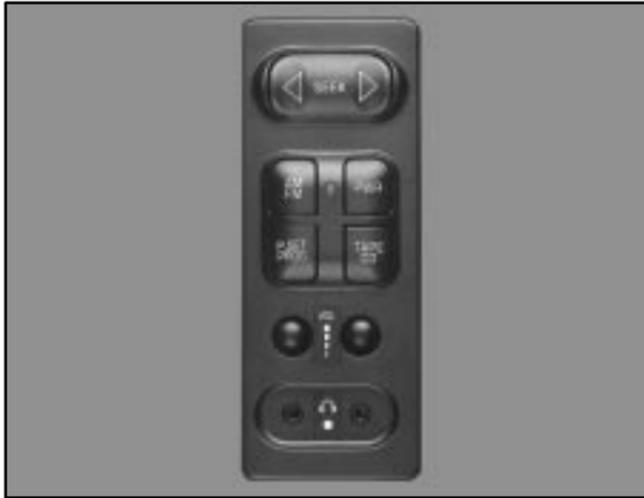
This feature allows rear seat passengers to listen to and control any of the music sources, including AM-FM, cassette tapes and CDs, through the Rear Seat Audio (RSA) controller. However, the rear seat passengers can only control the music sources that the front seat passengers are not listening to. For example, rear seat passengers may listen to a cassette tape through
