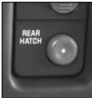
This button to the right of the steering wheel on the instrument panel allows you to release the liftglass from inside the vehicle.
