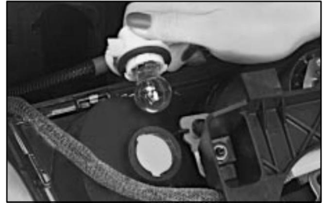
2. Twist the bulb socket to remove it from the headlamp assembly.
