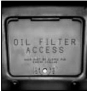
The access door for the remote oil filter is in the steering linkage shield assembly located under the radiator support. Twist the screw to unlock or lock the door. If you open the door, make sure it is securely closed when you are finished.
