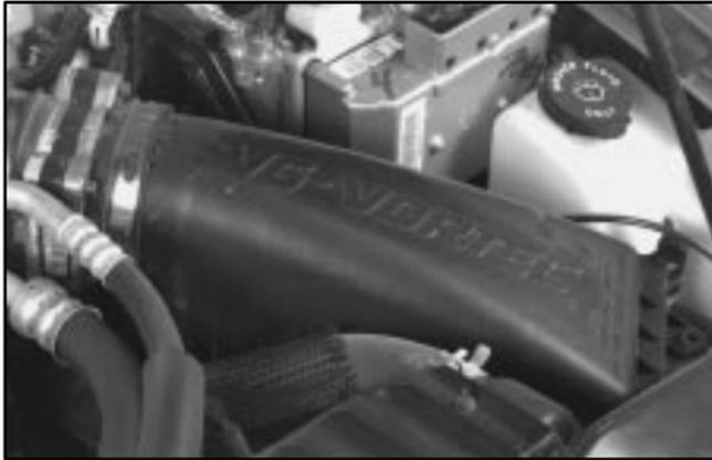
1. To remove the air cleaner filter, remove the fasteners that hold the cover on.
