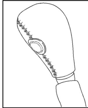
Your vehicle is equipped with a tow/haul selector switch. This switch is located on the shift knob.
