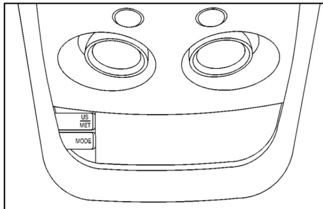
This system displays the outside air temperature, compass direction and trip information in the overhead console.
