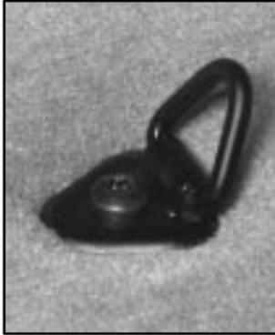
There are four cargo tie downs in the rear of the vehicle that allow you to strap cargo in and keep it from moving.
