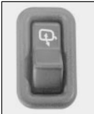
Your vehicle is equipped with power folding mirrors. This feature can be helpful when taking your vehicle through a car wash or through narrow spaces.
