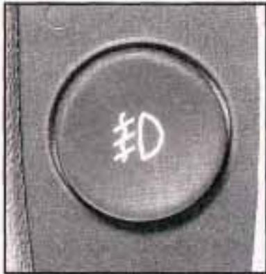
The fog lamp button is located on the instrument panel to the right of the exterior lamps knob.
