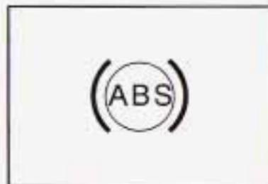
If there's a problem with the anti-lock brake system, this warning light will stay on. See *Anti-Lock Brake System Warning Light* on page 3-40.
