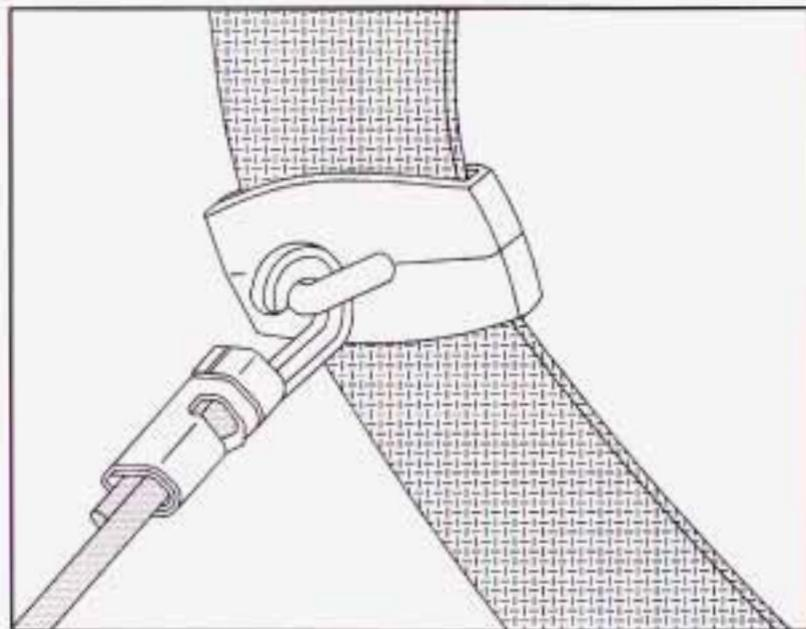
2. Align the sliding comfort guide, located on the shoulder belt, with the hook. Attach the hook to the loop on the sliding comfort guide.
