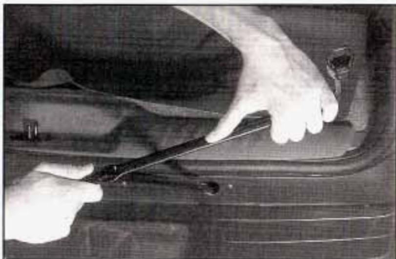
If the spare tire is hanging from the cable, insert the jack handle, extension and wheel wrench into the hoist shaft hole in the bumper, on an angle, and turn the wheel wrench counterclockwise to lower the spare the rest of the way.
