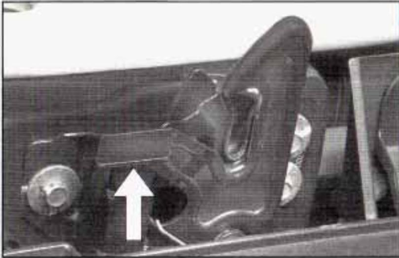
2. Then go to the front of the vehicle and release the secondary hood release.
