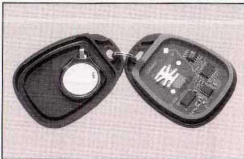
1. Insert a thin coin in the slot between the covers of the transmitter housing. Gently pry the transmitter apart.
