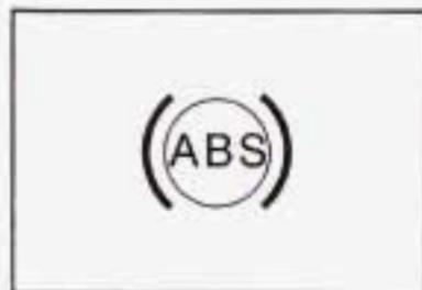
With the anti-lock brake system, this light will come on when you start your engine and may stay on for several seconds. That's normal. A chime may also sound when the light comes on.
