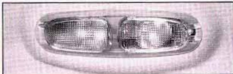
Press the lens on the lamp located above the doors to turn the reading lamps on and off.
