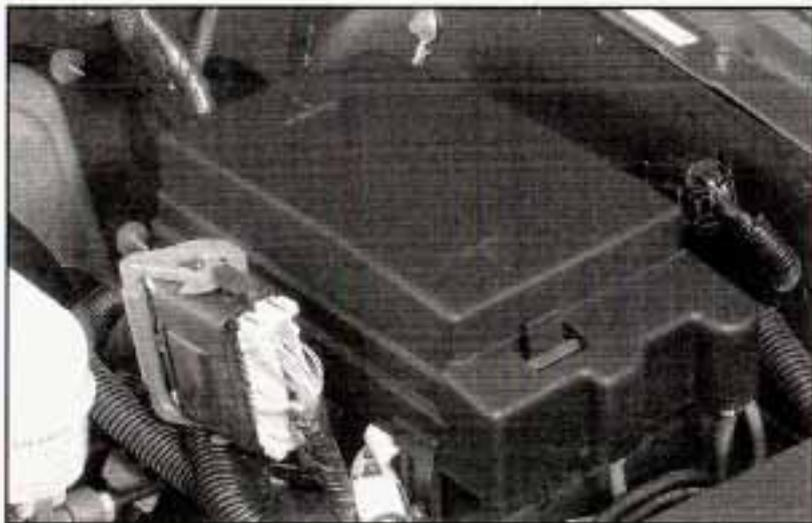
The fuse block is located under the hood in the engine compartment on the driver's side of the vehicle. See *Engine Compartment Overview on page 5-12* for more information on location.
