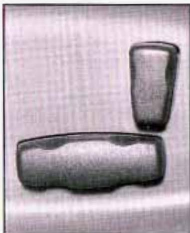
Your vehicle may have this feature. The power seat controls are located on the outboard side of the front seat cushions. The horizontal control adjusts the seat cushion and the vertical control adjusts the seatback.
