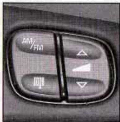
If your vehicle has this feature, certain radio functions can be operated by using the controls on your steering wheel.
