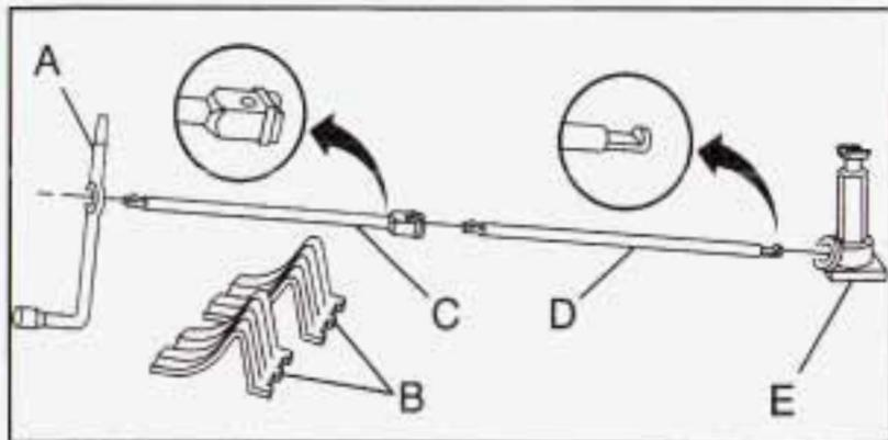
The tools you'll be using include the wheel wrench (A), tire blocks (B), extension(s) (socket end) (C), handle (jack end) (D), and jack (E). The Envoy XL will include an additional extension.
