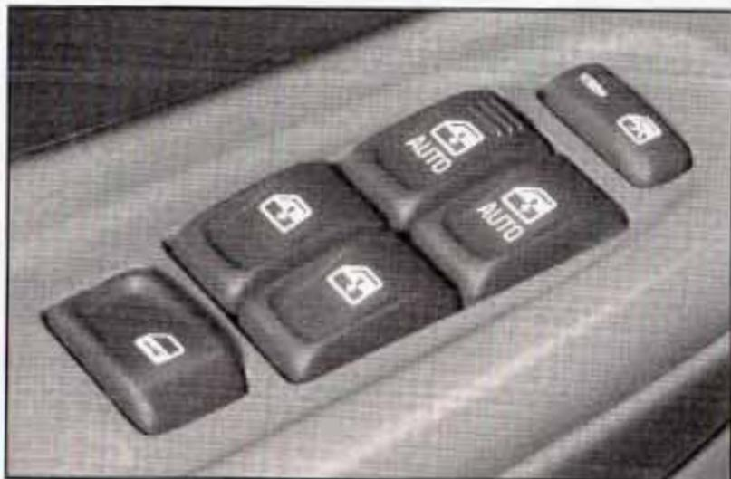
The controls for the power windows are located on the armrest on each of the side doors. With power windows, the switches operate the windows when the ignition is in RUN, ACCESSORY or when Retained Accessory Power (RAP) is active. The driver's door has a switch for each of the passenger's windows as well.
