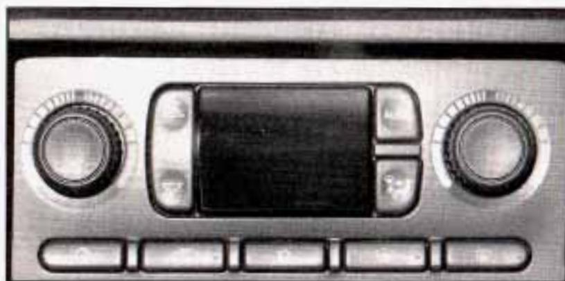
When your vehicle is first started, the display will show the driver's temperature setting and air delivery mode for five seconds. Then it will show the outside temperature.
