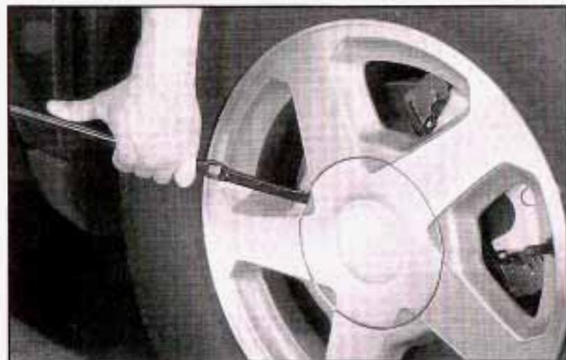
4. Use the chisel end of the wheel wrench to pry off the center cap.
