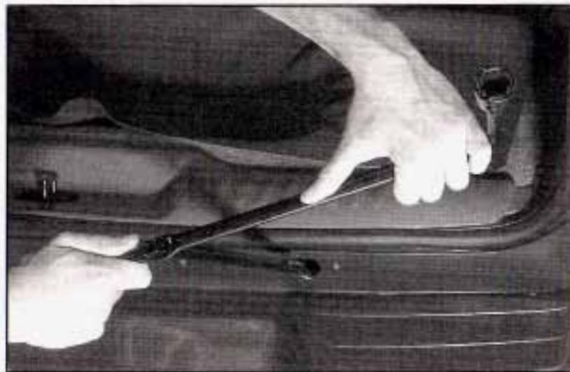
1. To remove the underbody-mounted spare, insert the socket end of the extension on a 45° angle downward into the hoist drive shaft hole. It is exposed when the rear gate is open and is just above the rear bumper. Be sure the socket end of the extension connects into the hoist shaft.
