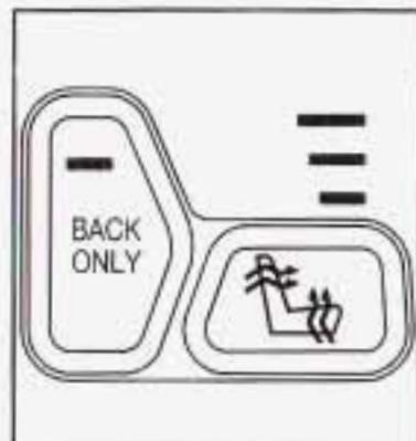
Your vehicle may have heated front seats. The buttons used to control this feature are located on the front door armrests. The engine must be running for the heated seat feature to work.
