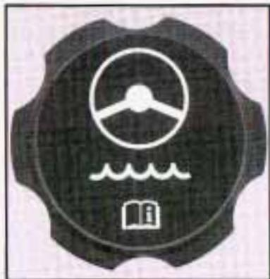
The power steering fluid reservoir is located in the engine compartment. It is on the passenger's side of vehicles with the L6 engine and is on the driver's side of vehicles with the V8 engine.
