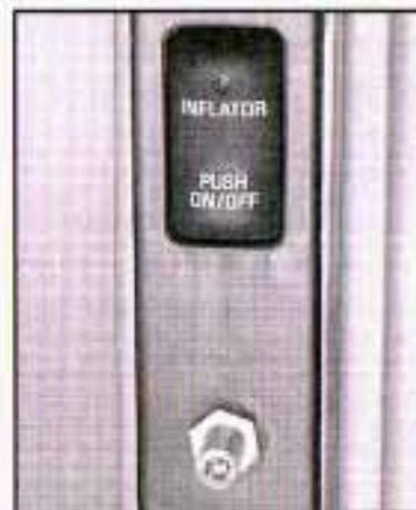
The air inflator is often located in the rear compartment on the passenger's side of the vehicle behind an access cover.
