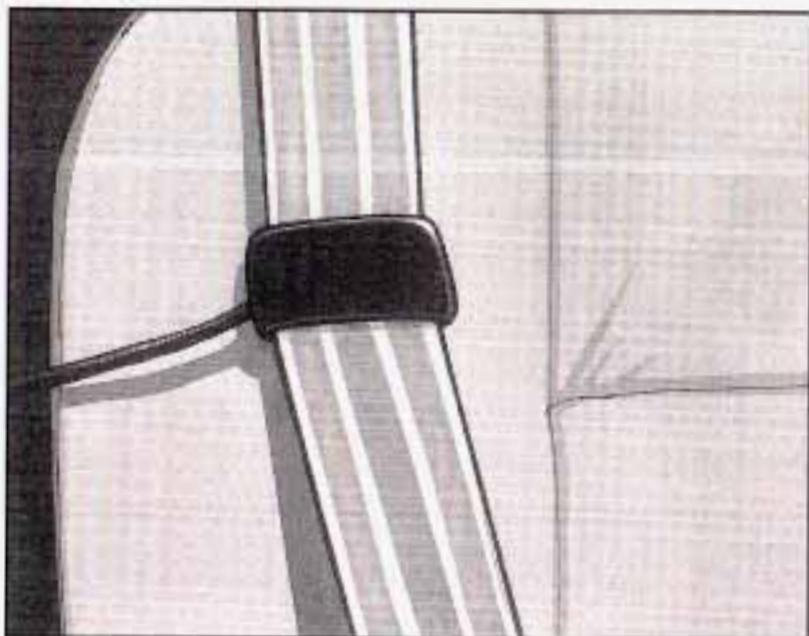
To remove and store the comfort guides, remove the hook from the loop. Slide the guide back into its storage pocket located on the side of the seatback.
