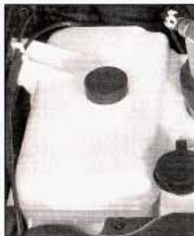
The engine coolant recovery tank is in the engine compartment on the passenger's side of the vehicle. See *Engine Compartment Overview* on page 5-12 for more information on location.
