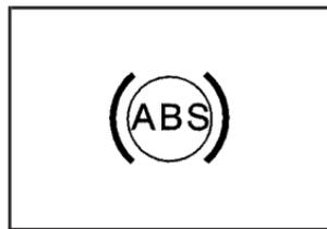
If there is a problem with the anti-lock brake system, this warning light will stay on. See *Anti-Lock Brake System Warning Light on page 3-29*.
