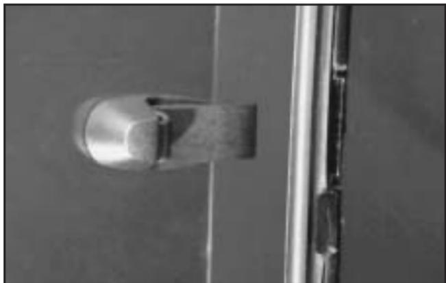
If your vehicle has this feature, squeeze the latch in the center of the window and slide the glass to open it. When you close the window, be sure the latch is engaged.
