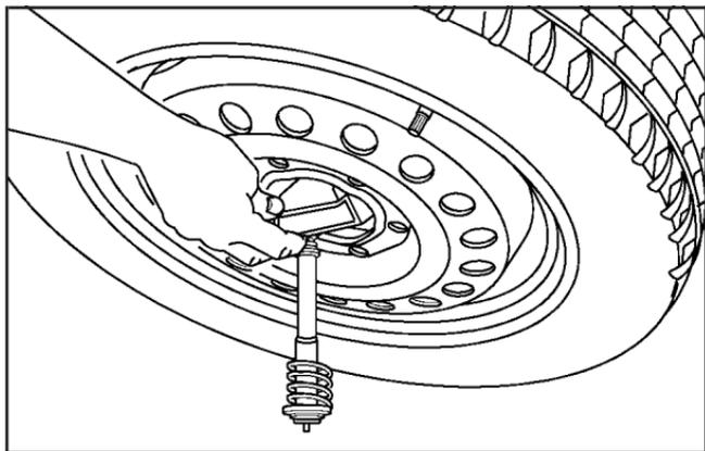
2. Tilt the retainer downward and through the wheel opening. Make sure the retainer is fully seated across the underside of the wheel.
