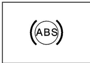
With the anti-lock brake system, this light will come on briefly when you start your engine to show it is working. Then it will turn off. This is normal.
