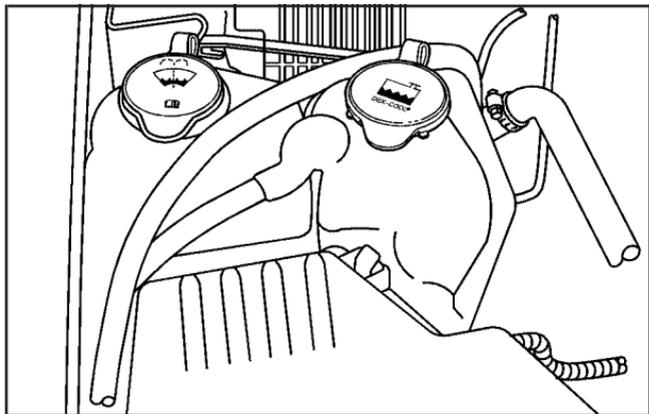
When the engine is cold, the coolant level should be at least up to the FULL COLD mark. If it isn't, you may have a leak at the pressure cap or in the radiator hoses, heater hoses, radiator, water pump or somewhere else in the cooling system.
