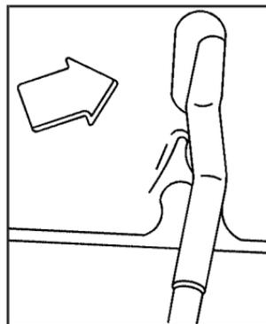
4. Release the hood prop from its retainer and put the hood prop into the slot in the hood.
