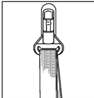
To move it up or down, squeeze the release buttons together and move the height adjuster to the desired position. After you move the adjuster to where you want it, try to move it down without squeezing the release buttons to make sure it has locked into position.
