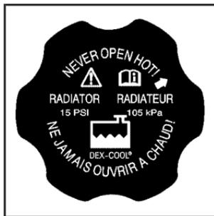
You can remove the radiator pressure cap when the cooling system, including the upper radiator hose, is no longer hot.
