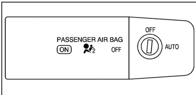
If your vehicle is a regular cab model or an extended cab model without rear seats, it has a switch on the instrument panel that you can use to turn off the right front passenger's frontal air bag.
