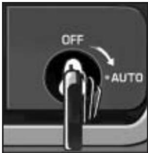
To turn the right front passenger's frontal air bag on again, insert your ignition key into the switch, push in, and move the switch to the auto position.
