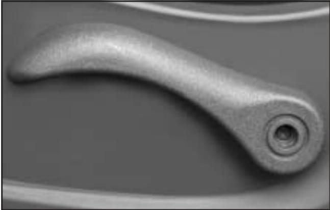
To manually recline your seatback, lift the lever on the outboard side of the seat.
