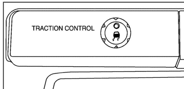
The TCS button is located on your instrument panel. Press this button to turn the TCS off and on.
