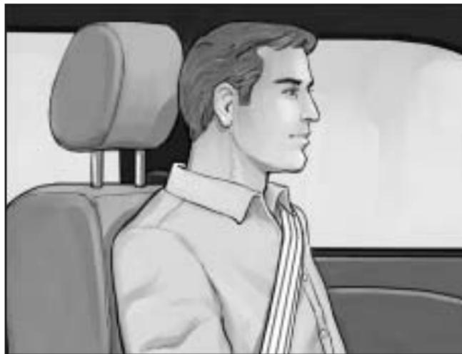
If your vehicle is equipped with adjustable head restraints, adjust your head restraint so that the top of the restraint is closest to the top of your head. This position reduces the chance of a neck injury in a crash.
