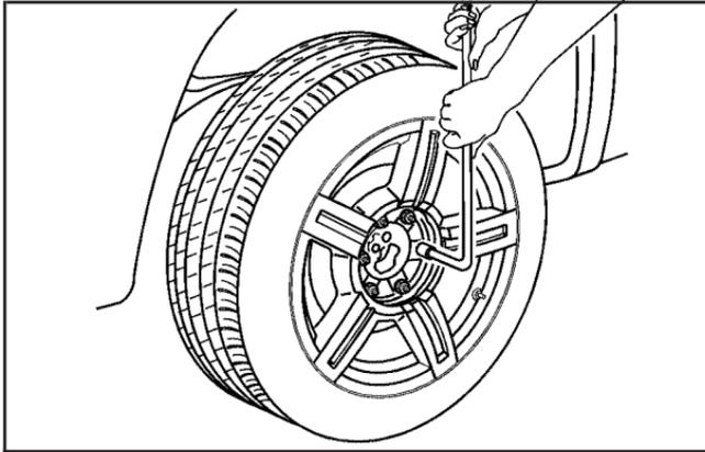
2. Use the wheel wrench to loosen all the wheel nuts. Turn the wheel wrench counterclockwise to loosen the wheel nuts. Do not remove the wheel nuts yet.
