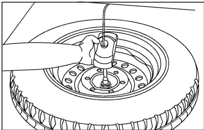
14. Tilt the tire retainer at the end of the cable and pull it through the wheel opening. Pull the tire out from under the vehicle.
