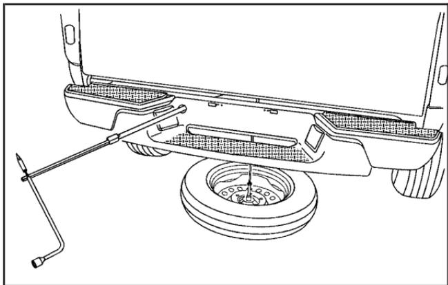
4. Insert the hoist end through the hole in the rear bumper and into the funnel-shaped guide.
