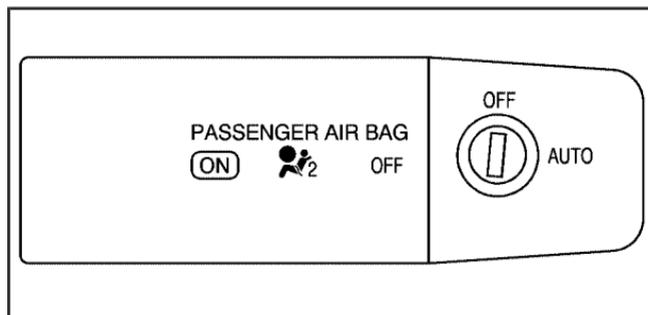
Unless the right front passenger's frontal air bag has been turned off, *never* put a rear-facing child restraint in this vehicle. Here is why:
