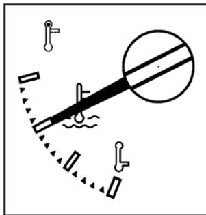
This gage shows the engine coolant temperature.
