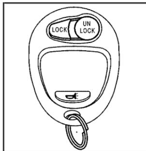
**UNLOCK:** Press this button to unlock the driver's door and turn on the interior lights. The parking lamps may also flash, and the horn may chirp, when this button is pressed.
