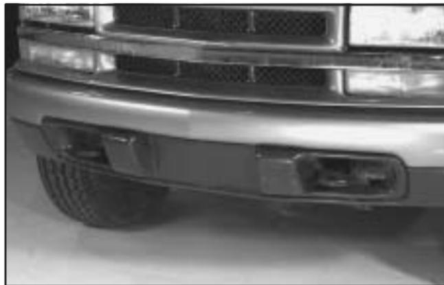
Your vehicle may be equipped with recovery hooks. The hooks are provided at the front of your vehicle. You may need to use them if you are stuck off-road and need to be pulled to some place where you can continue driving.
