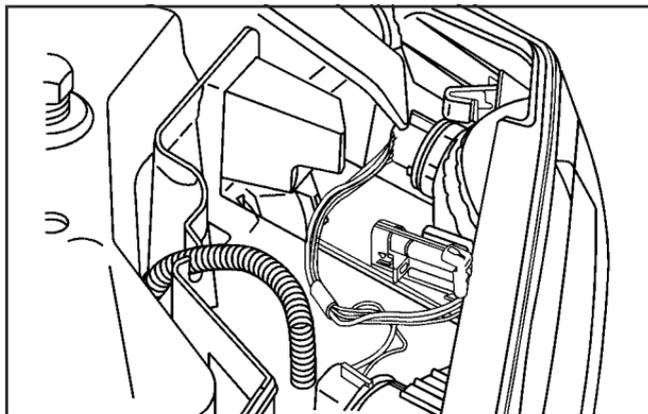
1. Remove the turn signal/parking lamp/daytime running lamp (DRL) assembly by pressing on the release clip on the outboard side of the housing and pulling the outboard end of the lamp toward you.
