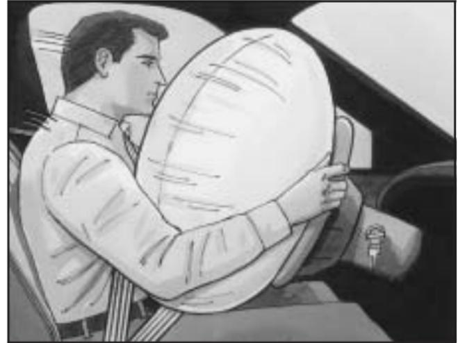
The driver's air bag is in the middle of the steering wheel.
