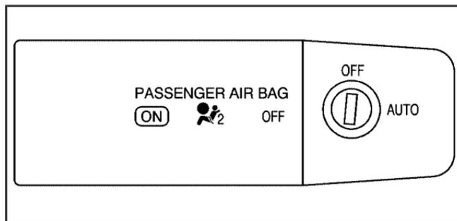
Unless the right front passenger's frontal air bag has been turned off, never put a rear facing child restraint in the right front passenger's seat. Here is why:
