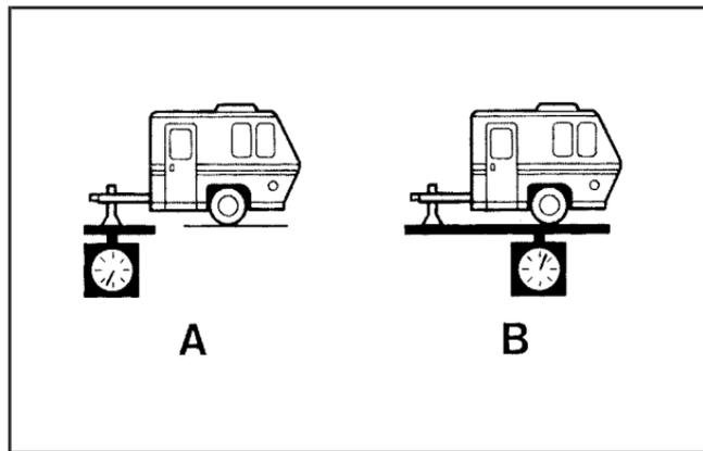
The trailer tongue weight (A) should be 10 percent to 15 percent of the total loaded trailer weight, up to a maximum of 500 lbs (226 kg) with a weight carrying hitch.
