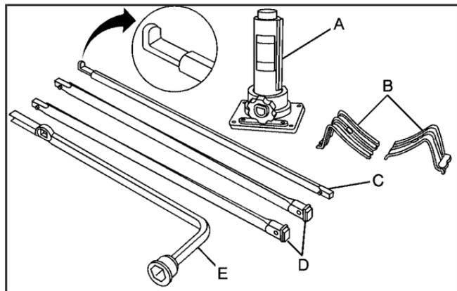
The tools you will be using include the bottle jack (A), the wheel blocks (B), the extension tool (C), the jack handle extensions (D), and the wheel wrench (E).
