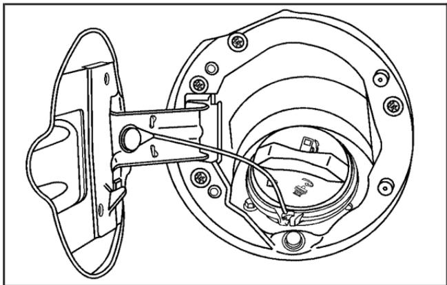
The tethered fuel cap is located behind a hinged door on the driver's side of your vehicle.
