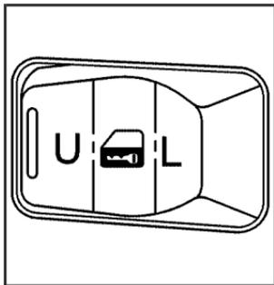
If your vehicle has power door locks, the switches are located on the driver's and the front passenger's armrests.
