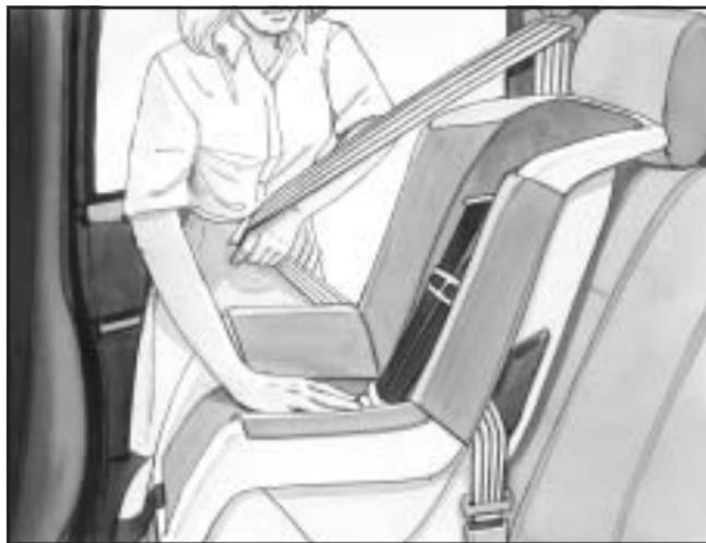
4. Pull the rest of the shoulder belt all the way out of the retractor to set the lock (crew cab only).
