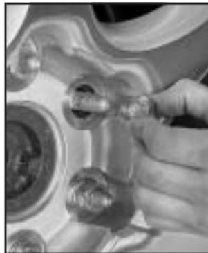
8. After mounting the spare, put the wheel nuts back on with the rounded end of the nuts toward the wheel. Tighten each wheel nut by hand. Then use the wheel wrench to tighten the nuts until the wheel is held against the hub.
