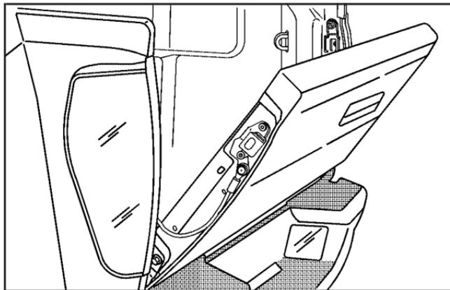
You can open the tailgate by pulling up on the handle while pulling the tailgate down.
