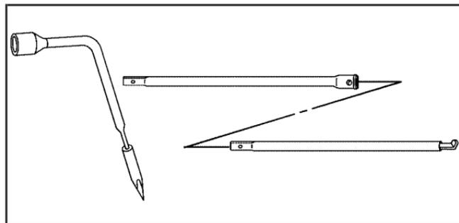
3. Attach the wheel wrench and extensions together.
