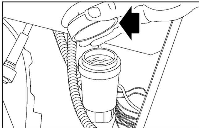
Refer to the Maintenance Schedule to determine how often you should check the fluid level in your clutch master cylinder reservoir and for the proper fluid. See *Owner Checks and Services* on page 6-9 and *Recommended Fluids and Lubricants* on page 6-13.
