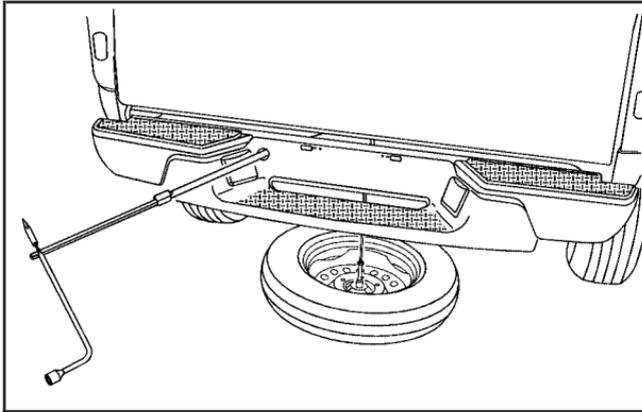
2. Insert the hoist end (chiseled end) of the extension tool through the hole in the rear bumper and into the funnel-shaped guide. The chiseled end of the extension is used to lower the spare tire.
