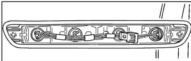
1. Remove the screws and lift off the lamp assembly.
