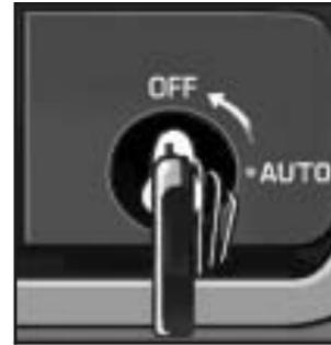
To turn off the right front passenger's frontal air bag, insert your ignition key into the switch, push in, and move the switch to the off position.
