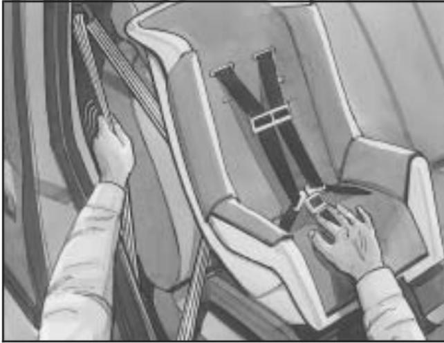
6. To tighten the belt, push down on the child restraint, pull the shoulder portion of the belt to tighten the lap portion of the belt and feed the shoulder belt back into the retractor. If you are using a forward-facing child restraint, you may find it helpful to use your knee to push down on the child restraint as you tighten the belt.
