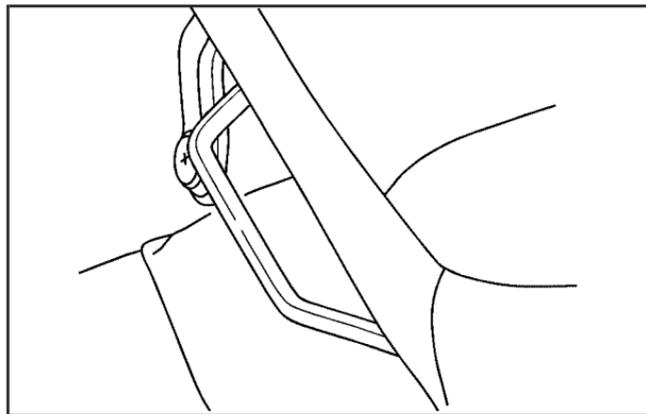
Move the lever located under the front of a manual seat up to unlock it. Slide the seat to where you want it and release the lever. Try to move the seat with your body to make sure the seat is locked into place.
