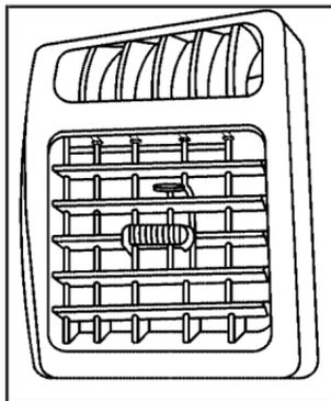
Use the thumbwheel on the outlets to change the direction of the air flow.
