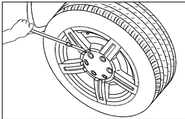
1. Remove the center cap by placing the chisel end of the wheel wrench (E) in the slot on the wheel and gently prying the cap out.
