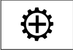
This light appears when you need to shift to the next higher gear on a manual transmission vehicle.
