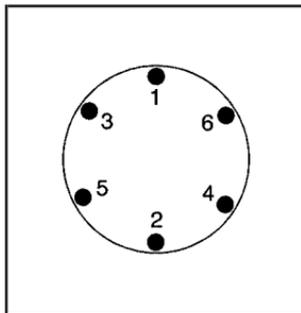
10. Tighten the wheel nuts firmly in a crisscross sequence as shown by turning the wheel wrench clockwise.
