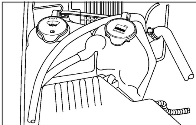
The coolant recovery tank is located toward the rear of the engine compartment on the passenger's side. See *Engine Compartment Overview* on page 5-12 for more information on location.
