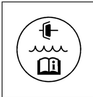
The hydraulic clutch fluid reservoir cap has this symbol on it.
