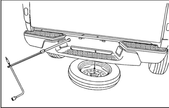
11. Remove the jack handle and insert the hoist end of the extension through the hole in the rear bumper. Turn the wheel counterclockwise one turn or until the wheel retainer assembly falls out.
