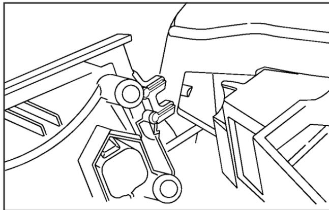
7. Place the inboard end of the turn signal/parking lamp/DRL housing over the small post in the grille.
