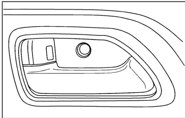
To lock a door from the inside, rotate the manual lever on your door forward. To unlock a door from the inside, rotate the lever on the door rearward.
