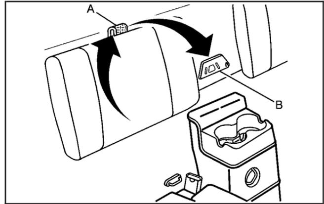
Anchor points for the top strap in a regular or extended cab vehicle are located behind the front seat on the back wall of the passenger compartment. You must route the top strap through the loop (A) at the top of the seatback to attach the strap to the anchor (B) as shown.
