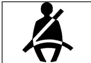
The safety belt light will also come on and stay on for several seconds, then it will flash until the driver’s safety belt is buckled.
