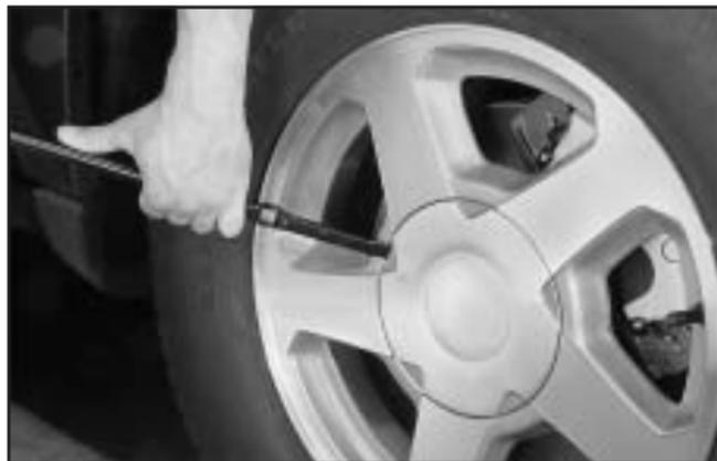
4. Position the chisel end of your wheel wrench in the notch of the center cap and pry off the center cap.
