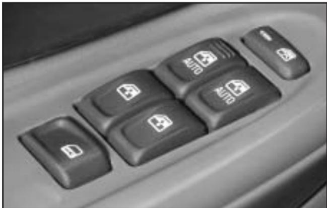
The controls for the power windows are located on the armrest on each of the side doors. With power windows, the switches operate the windows when the ignition is in RUN, ACCESSORY or when Retained Accessory Power (RAP) is active. See “Retained Accessory Power (RAP)” under *Ignition Positions on page 2-20*. The driver's door has a switch for each of the passenger's windows as well.
