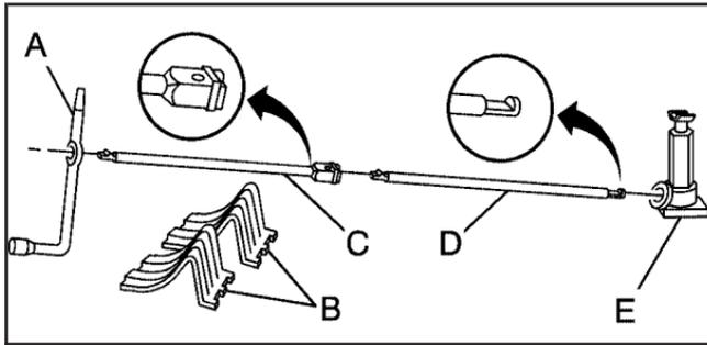
The tools you'll be using include the wheel wrench (A), wheel blocks (B), extension(s) (socket end) (C), handle (jack end) (D), and jack (E).
