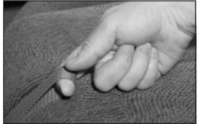
Pull up on the loop located where the seat cushion meets the seatback to fold the seat cushion up and out of the way. This will allow the seatback to fold flat and increase the cargo area.
