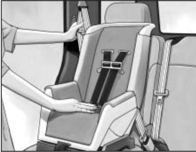
5. To tighten the belt, push down on the child restraint, pull the shoulder portion of the belt to tighten the lap portion of the belt and feed the shoulder belt back into the retractor. If you are using a forward-facing child restraint, you may find it helpful to use your knee to push down on the child restraint as you tighten the belt.
