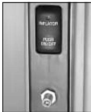
The air inflator is located in the rear compartment on the passenger's side of the vehicle behind an access cover.
