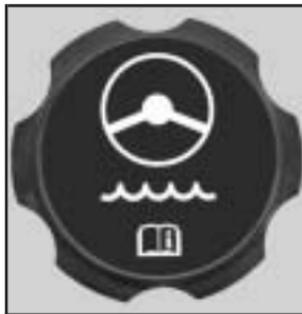
The power steering fluid reservoir is located in the engine compartment. It is on the passenger's side of vehicles with the L6 engine and is on the driver's side of vehicles with the V8 engine. See *Engine Compartment Overview* on page 5-12 for reservoir location.
