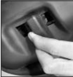
You should adjust the steering wheel before you drive. The tilt lever is located to the left of the steering column, under the turn signal lever.
