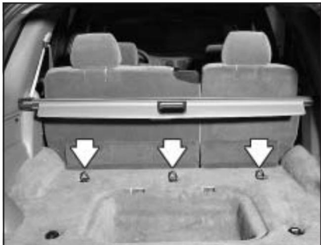
Anchor brackets for the rear seat positions are located on the floor in the cargo area of your vehicle (Envoy only). Do not use the rear tie-down brackets near the liftgate for top strap tethers.
