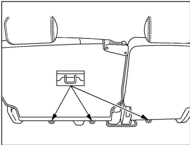
An anchor bracket for a top strap is located at the bottom rear of the seat cushion for each seating position in the second row (Envoy XL only).
