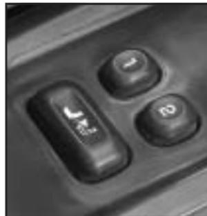
Your vehicle may have this feature. The controls are located on the driver's door, and are used to program and recall memory settings for the driver's seating positions, outside mirror positions and adjustable pedals (if equipped).
