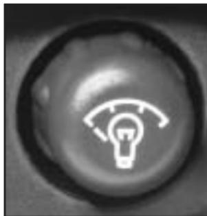
Press the knob located next to the exterior lamps knob to extend it.
