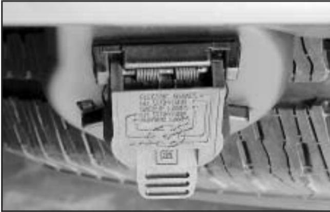
Your vehicle may be equipped with the seven-wire trailer towing harness. This harness has a seven-pin universal heavy-duty trailer connector that is attached to a bracket on the hitch platform. The seven-wire harness contains the following trailer circuits:
