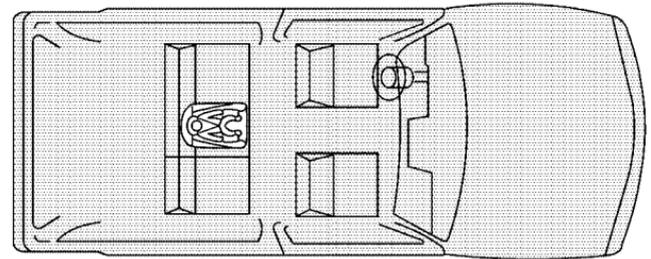
Many child restraints are too wide to be correctly secured in the center rear seat, although some of them will fit there. If the center seat position is too narrow for your child restraint, secure it in a rear outside seat position.
