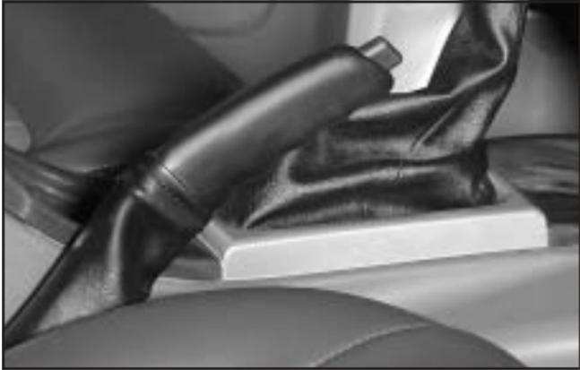
To release the parking brake, hold the regular brake pedal down. Pull the parking brake lever up until you can press in the button at the end of the lever. Hold the button in as you move the parking brake lever all the way down.
