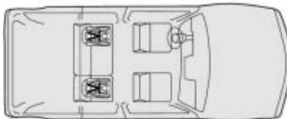
Your vehicle has the LATCH system. You will find anchors in the rear outside seat positions.
