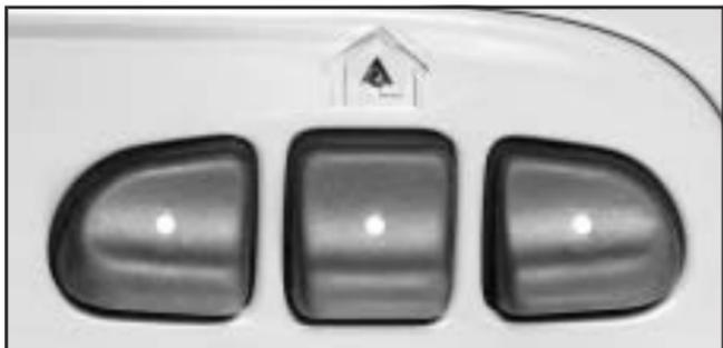
HomeLink<sup>®</sup>, a combined universal transmitter and receiver, provides a way to replace up to three hand-held transmitters used to activate devices such as gate operators, garage door openers, entry door locks, security systems and home lighting. Additional HomeLink<sup>®</sup> information can be found on the internet at [www.homelink.com](http://www.homelink.com) or by calling 1-800-355-3515.
