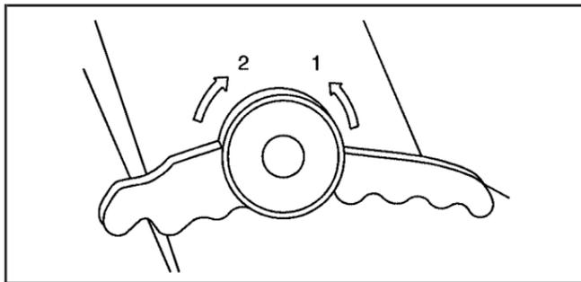
3. Release the rear set of seat hooks from the floor pins by pulling up on the rear part of the lever (indicated as 2 on the handle side cover). This enables the seat to be tumbled forward.
