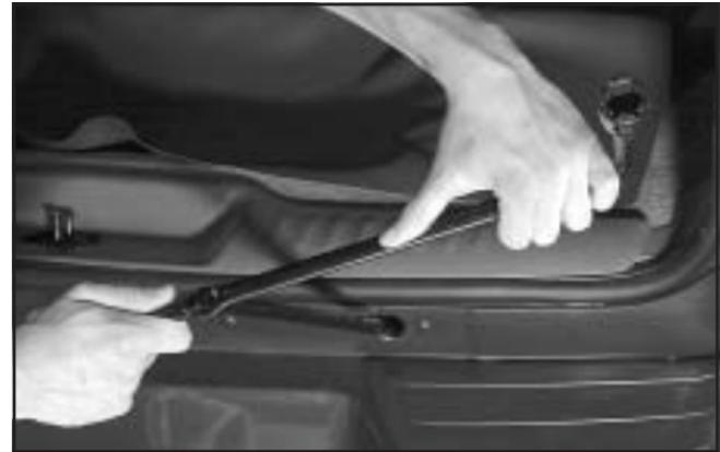
1. To remove the underbody-mounted spare, insert the socket end of the extension on a 45° angle downward into the hoist drive shaft hole. It is exposed when the rear gate is open and is just above the rear bumper. Be sure the socket end of the extension connects to the hoist shaft.
