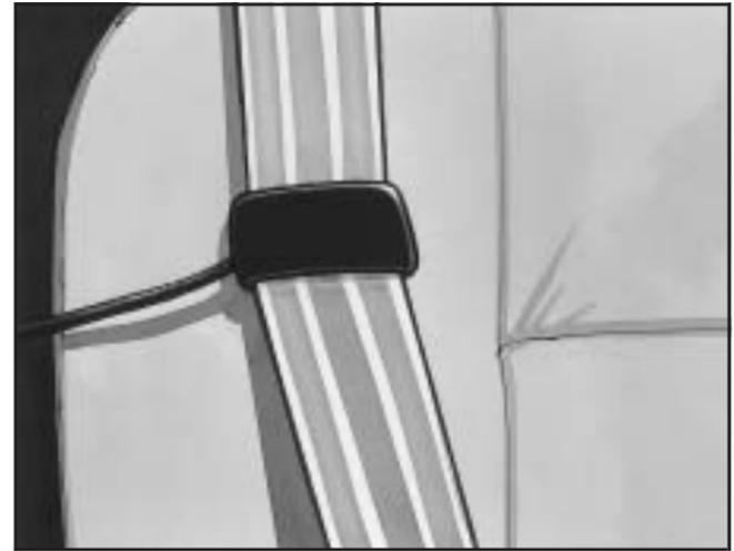
4. Be sure that the belt is not twisted and it lies flat. The elastic cord must be under the belt and the guide on top.
