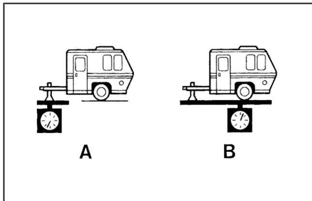
The trailer tongue weight (A) should be 10 percent to 15 percent of the total loaded trailer weight (B), up to a maximum of 400 lbs. (181 kg) with a weight carrying hitch. The trailer tongue weight (A) should be 10 percent to 15 percent of the total loaded trailer weight (A), up to a maximum of 900 lbs. (408 kg) for a weight distributing hitch.
