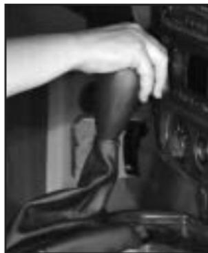
3. Press the button in on the side of the lever.
