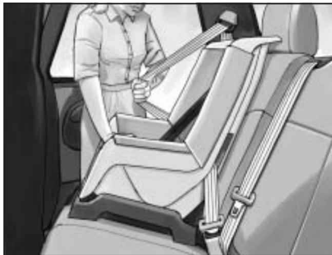
4. Pull the rest of the shoulder belt all the way out of the retractor to set the lock.
