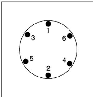
12. Use the wrench to tighten the wheel nuts firmly in a crisscross sequence as shown.
