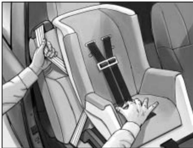
6. To tighten the belt, push down on the child restraint, pull the shoulder portion of the belt to tighten the lap portion of the belt and feed the shoulder belt back into the retractor. You may find it helpful to use your knee to push down on the child restraint as you tighten the belt.
