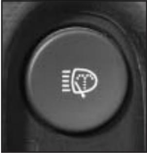
Your vehicle may be equipped with a headlamp washer system. The button to operate this feature is located on the instrument panel and functions separately from your other washer systems.
