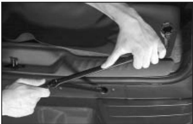
If the spare tire is hanging from the cable, insert the socket end of the extension connected to the wheel wrench into the hoist shaft hole in the bumper on an angle. Turn the wheel wrench counterclockwise to lower the spare the rest of the way.
