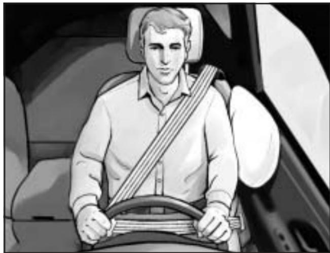
If your vehicle has a driver's side impact air bag it is located in the side of the driver's seatback closest to the door.
