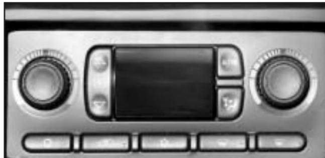
When your vehicle is first started and the climate control system is on, or if the climate control system has been turned on, the display will show the driver's temperature setting for five seconds. Then it will show the outside temperature.
