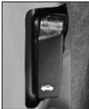
1. To open the hood, first pull the handle located inside the vehicle on the lower driver's side of the instrument panel.
