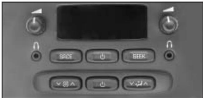
**⏻ (Power):** Press this button to turn the system on or off. The rear speakers will be muted when the power is turned on unless you have a Bose® equipped vehicle.
