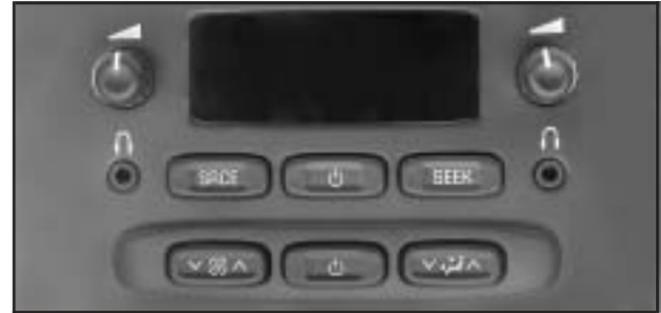
If your vehicle has the rear seat audio system, the lower buttons are used to adjust the rear seat climate controls. The temperature of the air coming through the rear outlets is determined by the front passenger's temperature setting.
