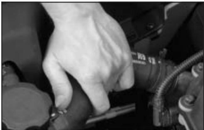
6. Start the engine and let it run until you can feel the upper radiator hose getting hot. Watch out for the engine cooling fan.
