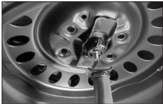
6. Attach the jack handle, extension and the wheel wrench to the jack and place it under the vehicle towards the front of the rear bumper. Position the center lift point of the jack under the center of the spare tire.
