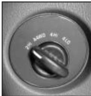
If your vehicle is equipped with four-wheel drive, the transfer case knob is located to the right of the steering wheel on the instrument panel. Use this knob to shift into and out of four-wheel drive.
