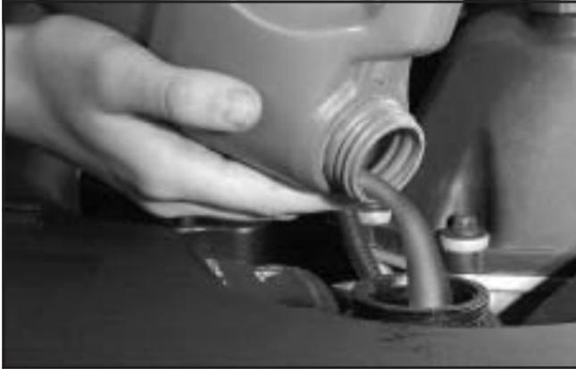
3. Fill the radiator with the proper DEX-COOL<sup>®</sup> coolant mixture, up to the base of the filler neck. See *Engine Coolant* on page 5-24 for more information about the proper coolant mixture.
