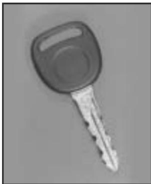
This vehicle has one double-sided key for the ignition and door lock. It will fit with either side up.
