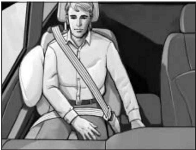
If your vehicle has a right front passenger's side impact air bag it is located in the side of the passenger's seatback closest to the door.
