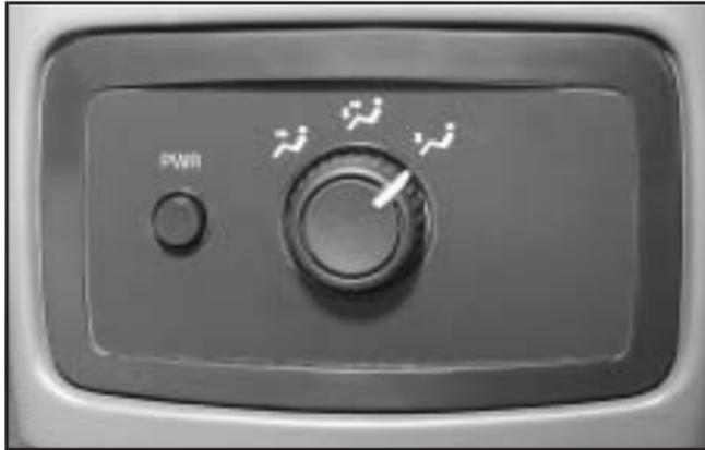
The temperature of the air coming through the rear outlets is determined by the front passenger's temperature setting. Press the PWR button to turn the rear climate controls on and off. Use the mode knob to change the direction of airflow (upper, bi-level or floor) to the rear seat area.
