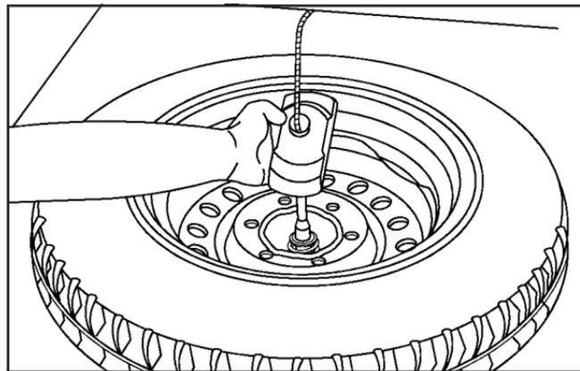
4. When the tire has been lowered, pull the tire toward you so you can reach the tire retainer and pull it up through the wheel opening.
