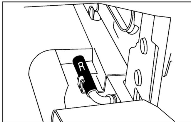
4. Push the pin with the black cap marked "R" down until it is in the retaining clip.
