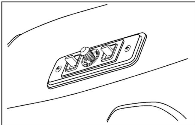
If your vehicle has front power seat(s), you can adjust them with these controls located at the front center of the seat cushion.
