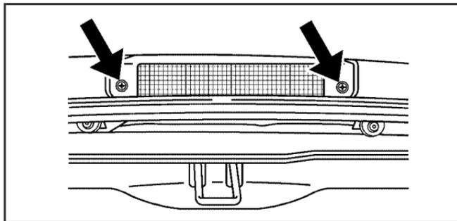
1. Remove the two screws from the CHMSL assembly.
