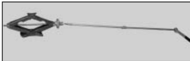
4. Attach the jack handle/jack handle extension to the jack. With the UP mark facing you, slide the ratchet onto the end of the jack handle extension. The set-up should look like the picture above.
