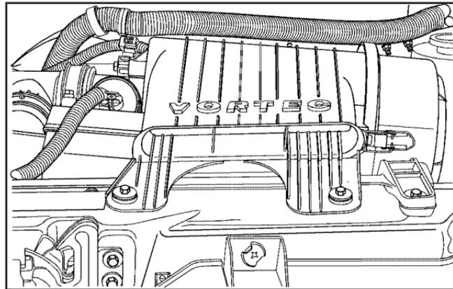
The engine air cleaner/filter is located near the center of the engine compartment. See *Engine Compartment Overview* on page 5-12 for more information on location.
