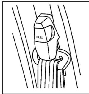
To move it down, pull on the center adjuster control labeled PULL. You can move the height adjuster up just by pushing up on the shoulder belt guide.
