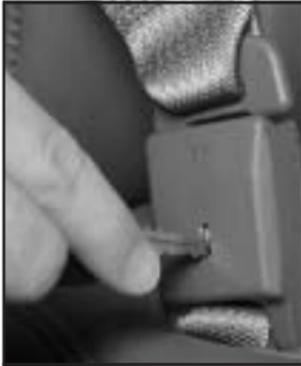
1. Disconnect the quick release latch plates for the lap shoulder belts on the bench seat to be removed. To do this, press the tip of a key into the release hole of the safety belt buckle while pulling up on the safety belt.
