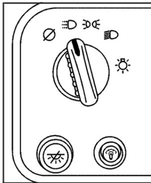
The control on the driver's side of your instrument panel operates the exterior lamps.
