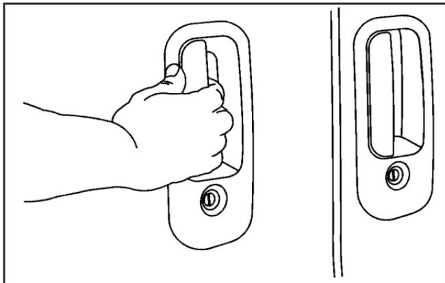
To open the sliding side door from the outside, pull the handle toward the rear of the vehicle and slide the door open.
