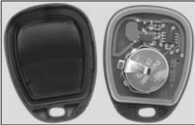
1. Use an object like a coin to pry open the transmitter.
