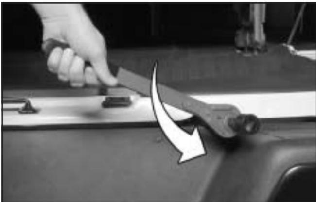
3. Turn the ratchet counterclockwise to lower the spare tire to the ground. If the spare tire does not lower to the ground, the secondary latch is engaged causing the tire not to lower. See *Secondary Latch System* on page 5-79.
