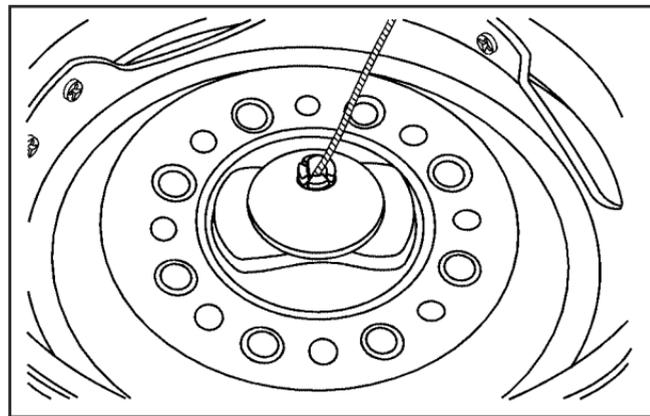
1. Put the tire on the ground at the rear of the vehicle with the valve stem pointed down.
