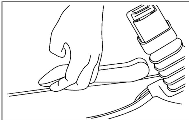
To adjust the seatback, lift the front of the lever located on the inboard side of the seat cushion.
