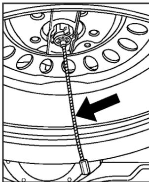
1. Check under the vehicle to see if the cable end is visible.
