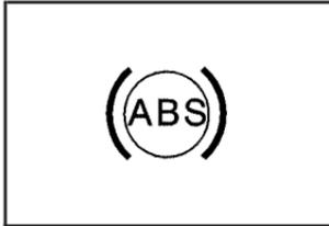
If there is a problem with the anti-lock brake system, this warning light will stay on. See *Anti-Lock Brake System Warning Light* on page 3-34.
