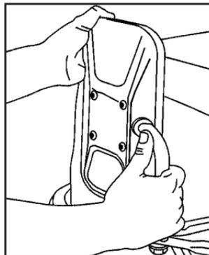
1. To adjust the mirrors when towing a trailer, turn the mirror by pushing the mirror head toward the front of the vehicle.
