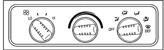
Turn the right knob clockwise or counterclockwise to direct the airflow inside of your vehicle.
