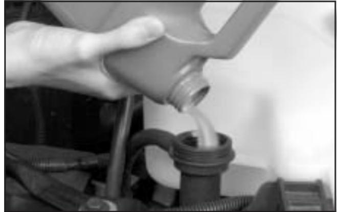
3. Fill the radiator with the proper DEX-COOL<sup>®</sup> coolant mixture, up to the base of the filler neck. See *Engine Coolant* on page 5-21 for more information about the proper coolant mixture.
