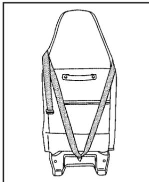
If the position you are using has an integrated headrest and you are using a dual tether, route the tether around the headrest.
