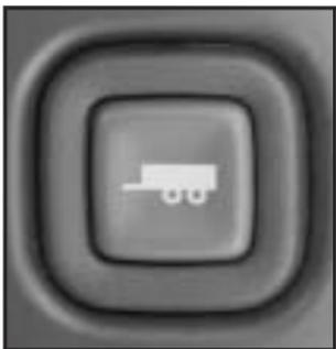
Press this button located to the right of the steering wheel on the instrument panel to turn tow/haul mode on and off.
