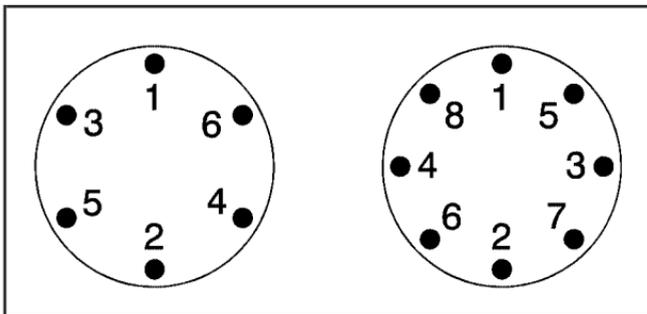
10. Use the wheel wrench to tighten the nuts firmly. Turn the wheel wrench clockwise and in a crisscross sequence as shown.
