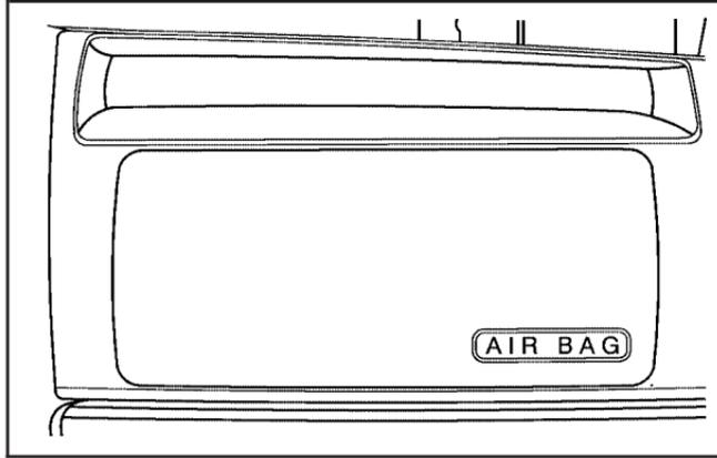
If it says AIR BAG on the middle part of the steering wheel and AIR BAG on the instrument panel in front of the right front passenger's seat, your vehicle has an airbag for the driver and an airbag for the right front passenger.
