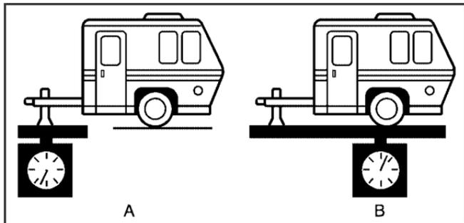
The trailer tongue weight (A) should be 10 percent to 15 percent of the total loaded trailer weight (B), up to a maximum of 400 lbs (181 kg) with a weight carrying hitch.
