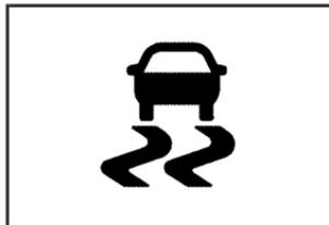
If you have the StabiliTrak<sup>®</sup> system, this light will be on or flashing, according to the description table for the StabiliTrak<sup>®</sup> system.
