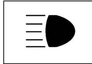
This light will come on when the high-beam headlamps are in use.
