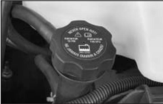
1. You can remove the radiator pressure cap when the cooling system, including the radiator pressure cap and upper radiator hose, is no longer hot. Turn the pressure cap slowly counterclockwise until it first stops. Do not press down while turning the pressure cap.
