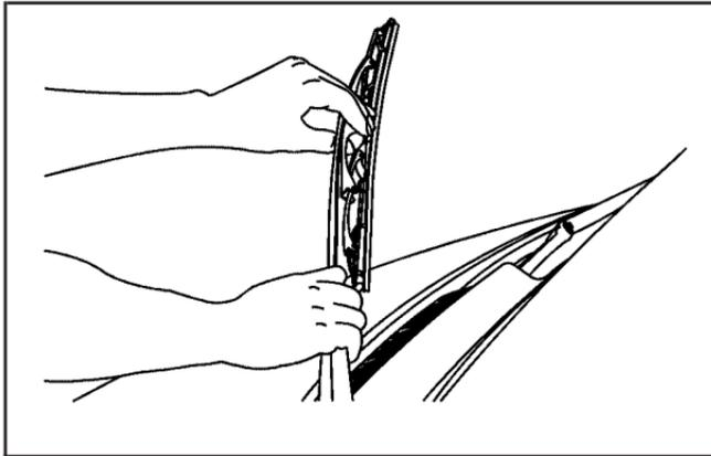
2. Press down on the blade assembly pivot locking tab. Pull down on the blade assembly to release it from the wiper arm hook.
