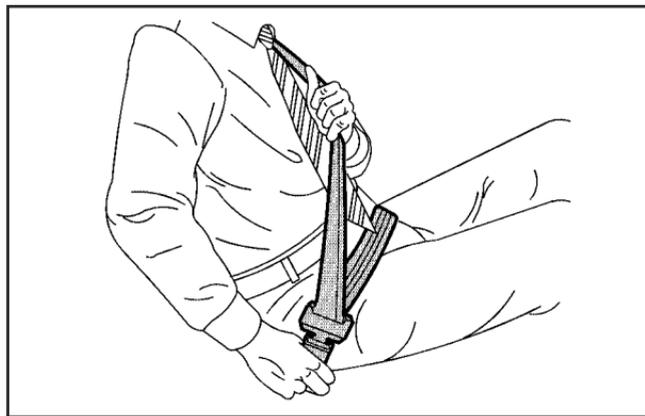
3. To make the lap part tight, pull down on the buckle end of the belt as you pull up on the shoulder part.
