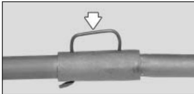
3. Connect the jack handle (C) and jack handle extension (B) together and press the retention clip (arrow) so it engages.
