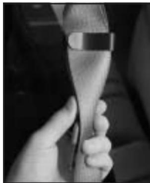
7. For the first row rear seat, stow the safety belt latch by attaching the clip on the safety belt latch to the trim just inside the side door. For the remaining rear seats, stow the safety belt latch plate on the clip at the window trim.
