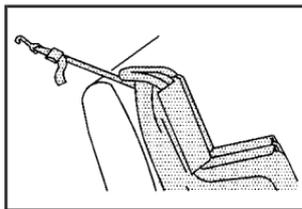
If the position you are using does not have a head restraint and you are using a single tether, route the tether over the seatback.
