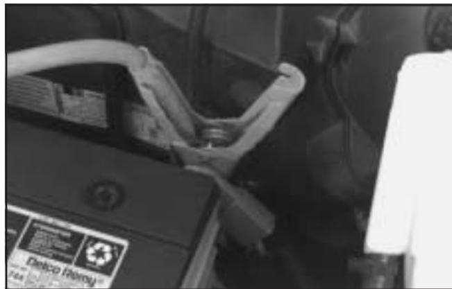
6. Connect the red positive (+) cable to the positive (+) terminal of the dead battery. Use a remote positive (+) terminal if the vehicle has one.
