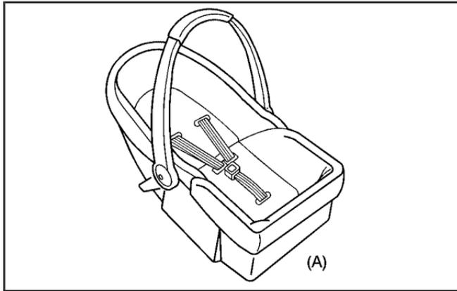
An infant car bed (A), a special bed made for use in a motor vehicle, is an infant restraint system designed to restrain or position a child on a continuous flat surface. Make sure that the infant's head rests toward the center of the vehicle.
