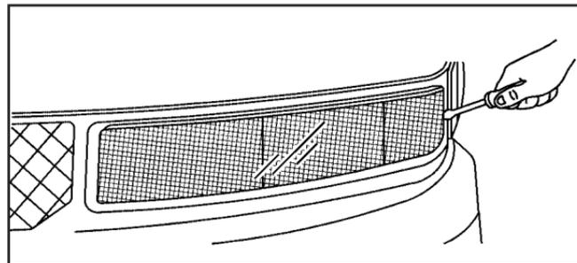
1. Use a small tool to unlatch the outboard clip on the lamp.
