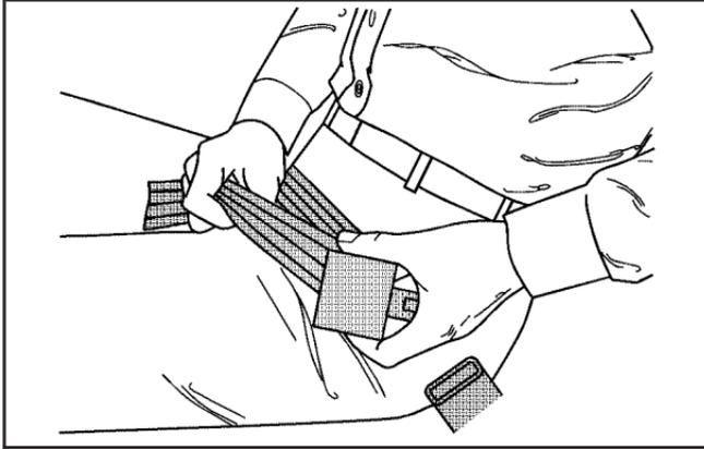
When you sit in a center seating position in the third, fourth or fifth row, you have a lap safety belt, which has no retractor. To make the belt longer, tilt the latch plate and pull it along the belt.
