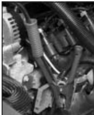
7. Connect the red positive (+) cable to the positive (+) terminal of the vehicle with the dead battery. Use a remote positive (+) terminal if the vehicle has one.
