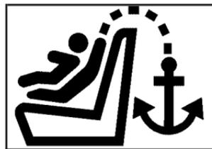
For regular and crew cab models, there is an anchor symbol on the trim covers to assist you in locating the top tether anchors.
