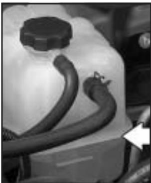
The coolant level should be at or above the FULL COLD mark. If it is not, you may have a leak at the pressure cap or in the radiator hoses, heater hoses, radiator, water pump, or somewhere else in the cooling system.
