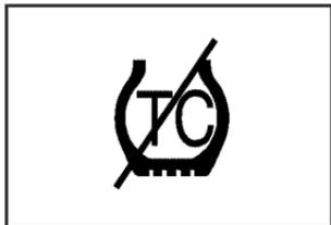
When the traction off light is on, the TAS is off and will not limit wheel spin. Adjust your driving accordingly.
