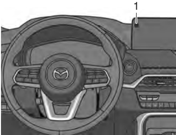
1. Driver monitoring camera
