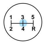
You can shift into R (Reverse) only by moving the gearshift from left of 3 (Third) and 4 (Fourth) gears before you shift into R (Reverse). This is a special lockout feature which prevents you from shifting
