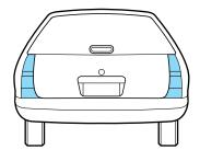
1. Open trunk to expose the tail lamp assembly. Remove the two screws from the front of the lamp.
