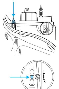
3. The "UP" and "DN" on the bubble indicate the directional change (up or down) of the vertical aim.
