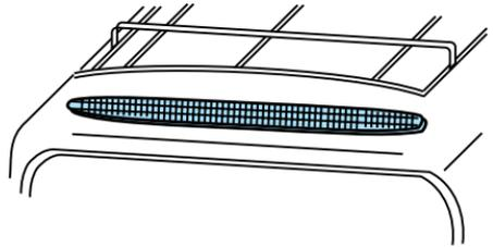
2. Carefully pull the lamp assembly away from the vehicle to access the bulbs.
