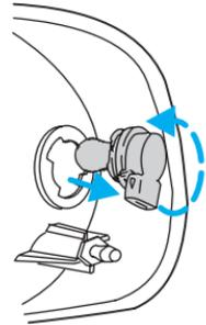
4. Install the bulb socket into the lamp assembly and rotate clockwise.
