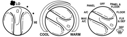
When the auxiliary A/C-heater control is set to FLOOR, airflow only occurs from the third row seat floor vent located in the driver's side rear quarter trim panel.
