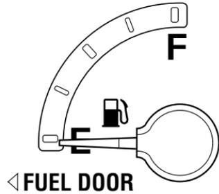
A minimum of six gallons must be added or removed from the fuel tank in order for the gauge to instantaneously update. If less than six gallons is the change, the gauge will take between five to ten minutes to update.
