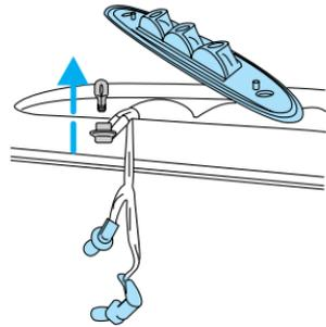
4. Pull the bulb straight out of the socket and push in the new bulb.
