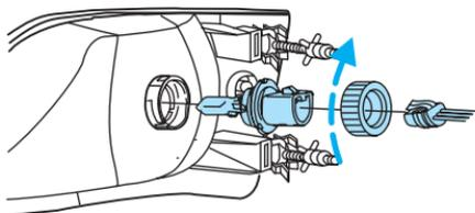
7. Without turning, carefully pull bulb assembly out of headlamp assembly.
