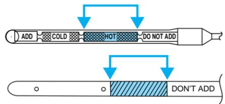
The transmission fluid should be in this range if at ambient temperature (10°C-35°C [50°F-95°F]).
