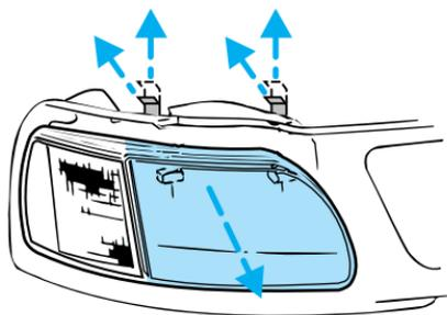
5. Release clip and disconnect the electrical connector from the bulb.
