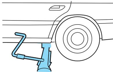
7. Position the jack according to the following guides and turn the jack handle clockwise until the wheel is completely off the ground.
