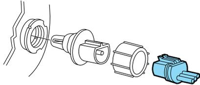
4. Remove the bulb retaining ring by rotating it counterclockwise (when viewed from the rear) to free it from the bulb socket, and slide the ring off the plastic base. Keep the ring to retain the new bulb.
