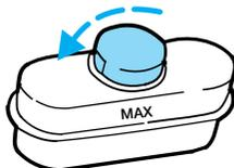
4. Use only brake fluids certified to meet Ford specifications. Refer to *Lubricant specifications* in the *Capacities and specifications* chapter. DOT 3 fluid is recommended. However, if DOT 3 is not available, DOT 4 fluid can be used.
