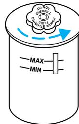
5. If the fluid is low, add fluid in small amounts, continuously checking the level until it reaches the range between the MIN and MAX lines. Be sure to put the cap back on the reservoir.
