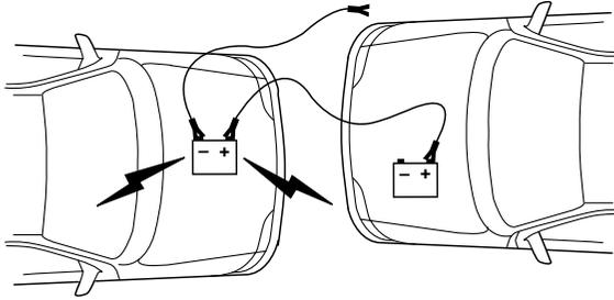
3. Connect the negative (-) cable to the negative (-) terminal of the assisting battery.
