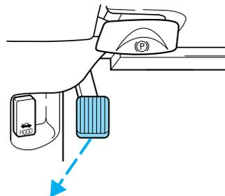
The BRAKE warning lamp in the instrument cluster illuminates and remains illuminated (when the ignition is turned ON) until the parking brake is fully released.
