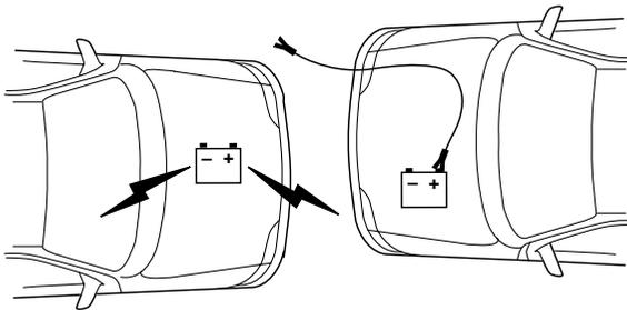
4. Remove the jumper cable from the positive (+) terminal of the disabled vehicle's battery.
