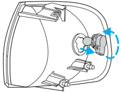
6. Align top and bottom ribs of parking lamp assembly with corresponding slots on front of vehicle.
