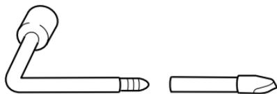
2. Insert the jack handle into the rear bumper opening.
