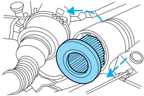
4. Install a new air filter element, ensuring the arrow on the top half of the air filter housing lines up with the notch on the bottom half of air filter housing. Be careful not to crimp the filter element edges between the air filter housing. This could cause filter damage and allow unmetered air to enter the engine if not properly seated.
