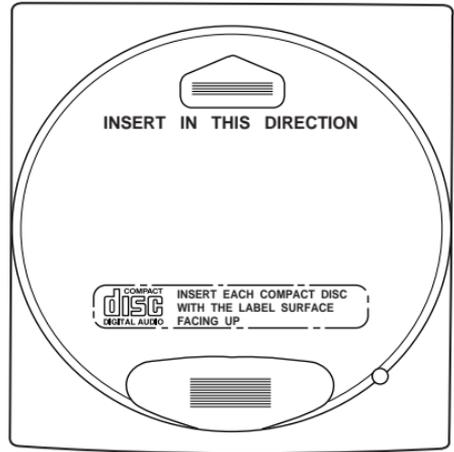
The CD magazine may be inserted or ejected with the radio power off.
