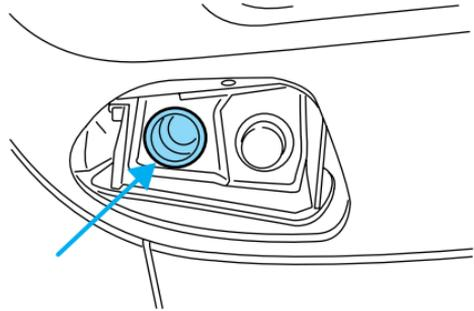
The auxiliary power point is located on the instrument panel.
