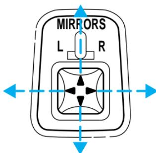
3. Return to the center position to lock mirrors in place.
