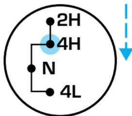
**Do not shift into 4H (4WD High) with the rear wheels slipping.**
