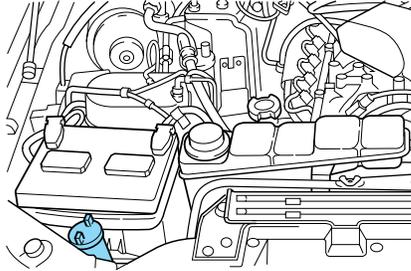
Only use a washer fluid that meets Ford specifications. Refer to *Lubricant specifications* in the *Capacities and specifications* chapter.
