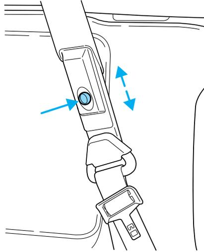
To lower the shoulder belt height, push the button and slide the height adjuster down. To raise the height of the shoulder belt, slide the height adjuster up. Pull down on the height adjuster to make sure it is locked in place.
