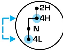
5. If the transfer case **does not** engage into 4L (4WD Low), repeat steps 1 through 4.
