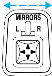
2. Move the control in the direction you wish to tilt the mirror.
