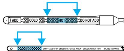
The transmission fluid should be in this range if at ambient temperature (10°C-35°C [50°F-95°F]).
