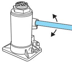
**Hydraulic jacks are equipped with a pressure release valve that prevents lifting loads which exceed the jack's rated capacity.**
