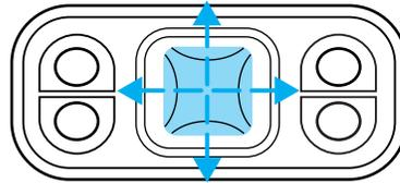
Turn the lumbar support control toward the front of vehicle to move the lumbar support forward for more direct support.
