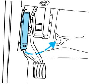
2. Go to the front of the vehicle and release the auxiliary latch located under the right center of the hood. Slide the handle to release the auxiliary latch.
