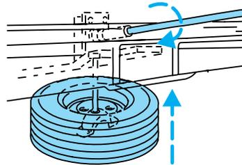
4. Check that the tire lies flat to the frame assembly. Push against the tire to make sure it is tightly seated under the vehicle. Loosen or retighten if necessary.
