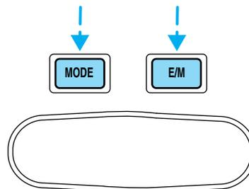
5. Release both controls. Subsequent pressing of either control will increment the zone. Press the control repeatedly until the correct zone setting for your geographic location is displayed on the trip computer.
