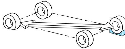
2. Turn engine OFF and block the diagonally opposite wheel (block not provided).
