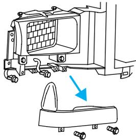
5. Remove the four bolts and headlamp bezel.
