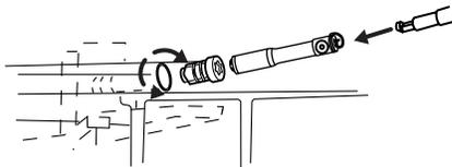
3. If equipped, unlock and remove the spare tire lock from the rear bumper drive tube using the the spare tire lock key and the jack handle.
