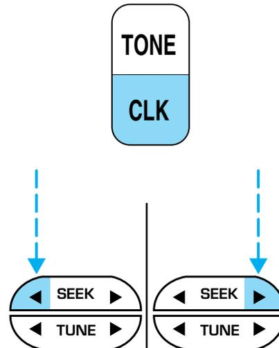
To set the minute, press and hold the CLK control until CLOCK SET appears in the display and press the TUNE control:
