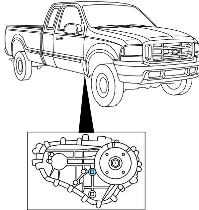
3. Add only enough fluid through the filler opening so that the fluid level is at the bottom of the opening.
