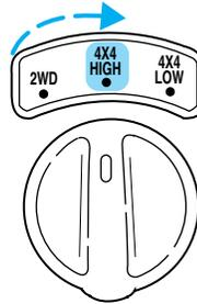
**Do not shift into 4x4 HIGH with the rear wheels slipping.**
