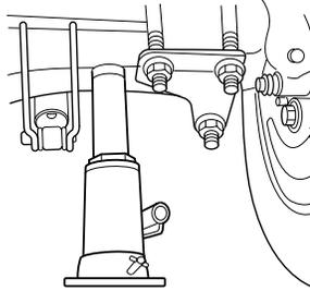
14. Insert the jack handle into the pump linkage.
