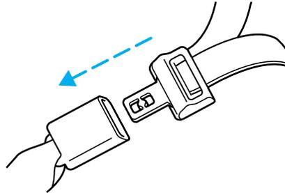
2. To unfasten, push the release button and remove the tongue from the buckle.
