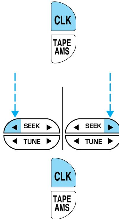
To set the minute, press and hold the CLK control and press the TUNE control:
