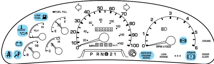
Make sure the corresponding lights illuminate briefly. If a light fails to illuminate, have the vehicle serviced.
