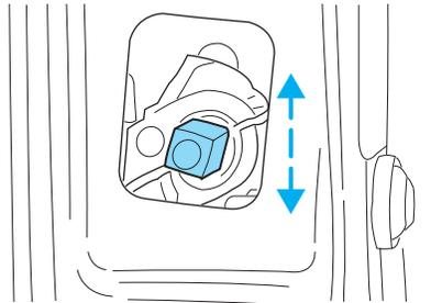
Move lock control up to engage the childproof lock. Move control down to disengage childproof locks.
