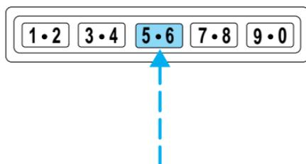
After the factory-set code or personal code has been entered, you can unlock all doors (press 3/4) and release the trunk (press 5/6) as long as the controls are pressed within 5 seconds of each other.
