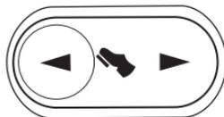
Press and hold the rocker control to adjust accelerator and brake pedal.
