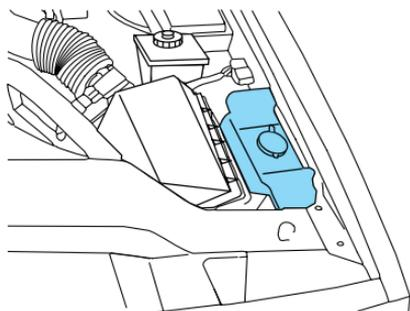
Only use a washer fluid that meets Ford specification . Refer to *Lubricant specifications* in the *Capacities and specifications* chapter.
