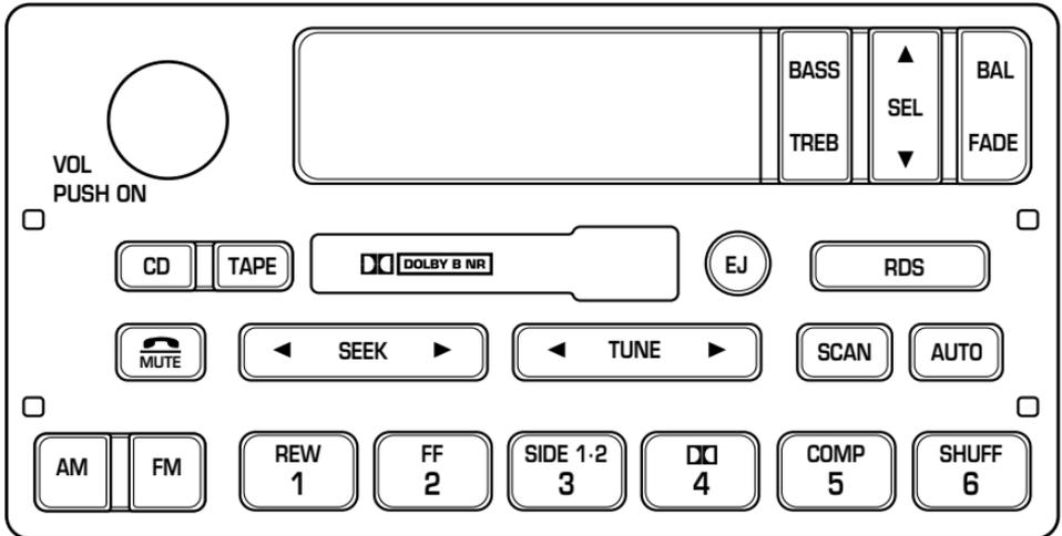
Your audio system is equipped with selective lighting, a unique lighting strategy. This lighting feature is operable when the headlamps are illuminated. During the operation of any selected mode, lighting for the individual function controls will either illuminate or turn off. Those controls which have a function for the specific mode of operation selected will be lit, while the controls which have no function for that mode will be turned off.
