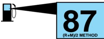
Do not be concerned if your engine sometimes knocks lightly. However, if it knocks heavily under most driving conditions while you are using fuel with the recommended octane rating, see your dealer or a qualified service technician to prevent any engine damage.
