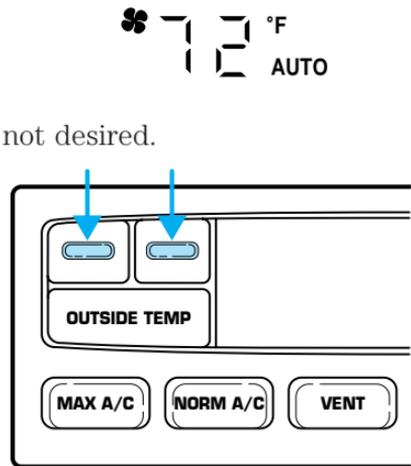
For continuous maximum cooling, push the blue button until 16°C (60°F) is shown in the display window. The EATC will continue maximum cooling (disregarding the displayed temperature) until a warmer temperature is selected by pressing the red button.
