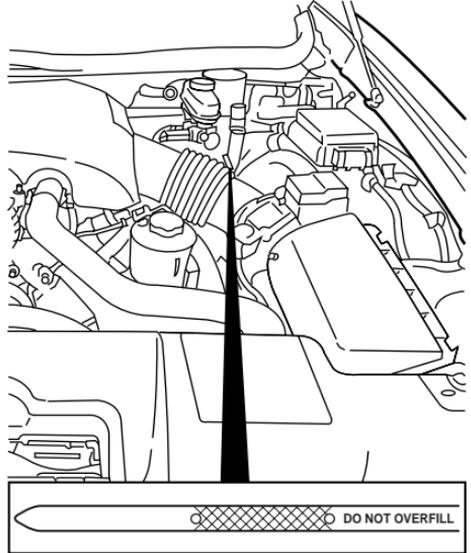
6. Wipe the indicator clean. Insert the indicator fully, then remove it again.
