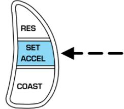
You can accelerate with the accelerator pedal at any time during speed control usage. Releasing the accelerator pedal will return your vehicle to the previously programmed set speed.
