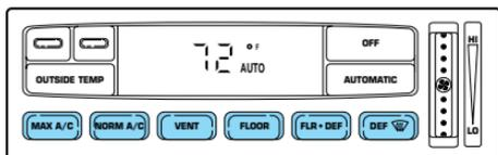
The air conditioning compressor can operate in all modes except FLOOR and VENT. It will also operate only when required when AUTOMATIC has been selected. However, the air conditioning will only function if the outside temperature is about 6°C (43°F) or higher.
