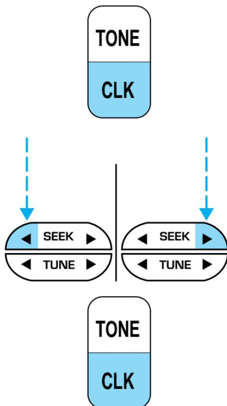
To set the minute, press and hold the CLK control until CLOCK SET appears in the display and press the TUNE control:
