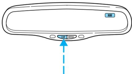
3. Release the COMP side of the control, then press it down again.
