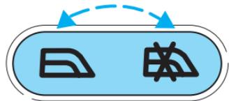
**NOTE:** The window switches will not illuminate when the window control is in the LOCKED position.
