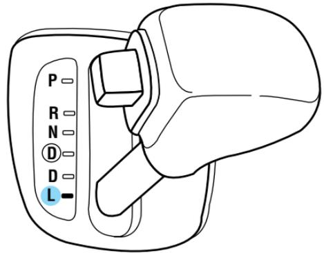
The automatic transaxle will shift into the proper gear to ascend any grade without any need to shift to L (Low).
