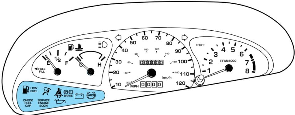
Make sure the corresponding lights illuminate or illuminate briefly. If a light fails to illuminate, have the vehicle serviced.
