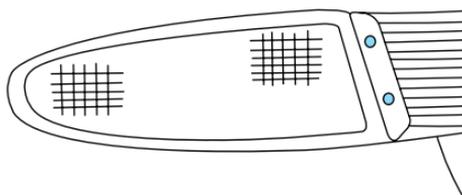
1. Open trunk to expose the tail lamp assembly screws. Remove the two screws from the front of the lamp.
