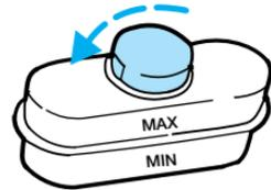
4. Use only a DOT 3 brake fluid certified to meet Ford specification ESA-M6C25-A. Refer to *Lubricant specifications* in the *Capacities and specifications* chapter.
