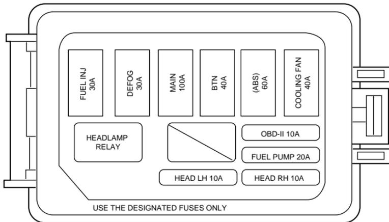
The high-current fuses are coded as follows.
