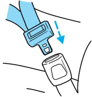
5. To put the retractor in the automatic locking mode, grasp the shoulder portion of the belt and pull downward until all of the belt is extracted and a click is heard.
