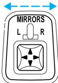
2. Move the control in the direction you wish to tilt the mirror.
