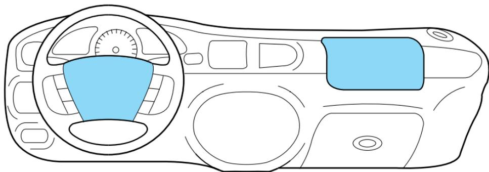
Your vehicle is equipped with a crash sensing and diagnostic module which records information about the air bag and sensor systems. In the event of a collision this module may save information related to the collision including information about the air bag system and impact severity. This information will assist Ford in the servicing of your vehicle and may help Ford better understand real world collisions and further improve the safety of future vehicles.
