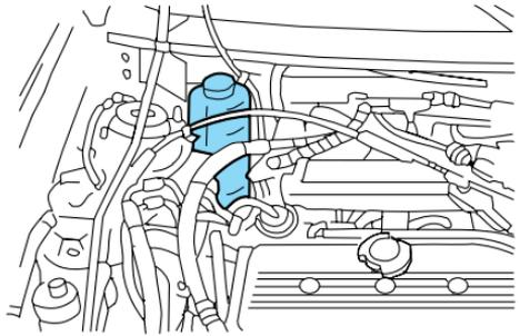
Check the washer fluid whenever you stop for fuel. The reservoir is highlighted with a
