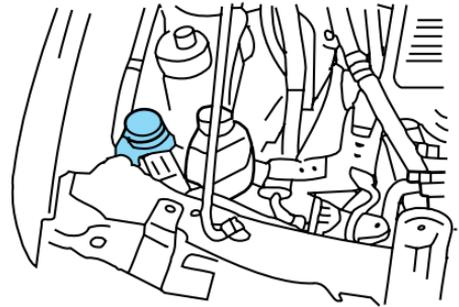
When the engine is cold, check the level of the engine coolant in the reservoir.
