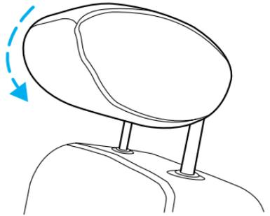
To lower the head restraints, push the release control while pushing down on the head restraint.
