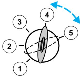
3. If the temperature is below  $-12^{\circ}\text{C}$  ( $10^{\circ}\text{F}$ ) and the engine does not start in 15 seconds on the first try, turn the key OFF and wait 10 seconds and try again. If the engine does not start in two attempts, press the accelerator pedal all the way to floor and hold. Turn the key to START position.
