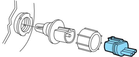
4. Remove the bulb retaining ring by rotating it counterclockwise (when viewed from the rear) to free it from the bulb socket, and slide the ring off the plastic base. Keep the ring to retain the new bulb.
