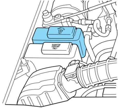
Only use a washer fluid that meets Ford specification . Refer to *Lubricant specifications* in the *Capacities and specifications* chapter.
