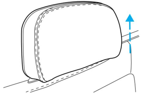
2. Flip the bottom of the head restraint up, toward the front seat.
