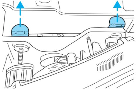
3. Disconnect the electrical connector from the bulb by pulling rearward.
