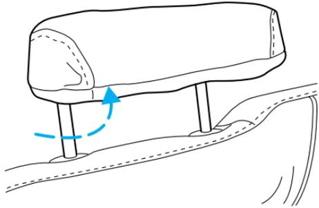
3. While holding the head restraint in “flat” position, lower the head restraint to the seat back.
