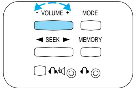
From the rear seat controls, volume control can be set no higher than the current radio setting unless the speakers are turned off. Refer to *Turning speakers on and off*.
