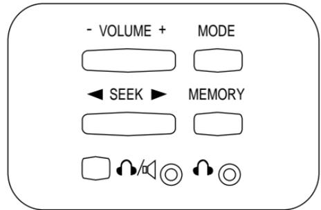
To turn on the rear seat controls, press the memory preset controls 3 and 5 at the same time. The 🎧 will appear in the display.
