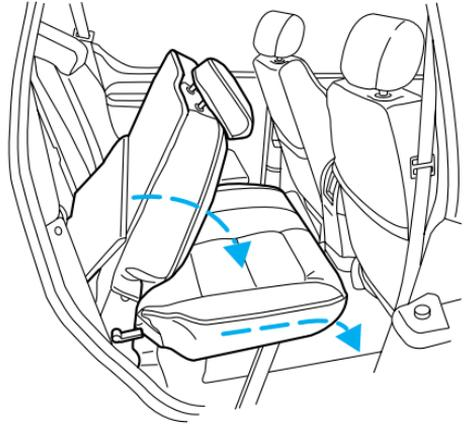
A carpeted panel will flip down from the back panel to complete the load floor.
