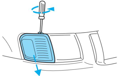
5. Install bulb socket in lamp assembly by turning clockwise.
