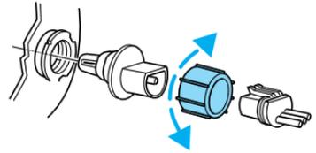
5. Without turning, remove the old bulb from the lamp assembly by gently pulling it straight back out of the lamp assembly.
