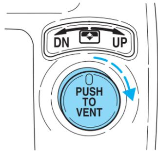
Push control once to move window (up or down) to the vent position (open approximately 2.00 inches for cab ventilation). If the window is already in the vent position and the control is pressed, no movement will occur.
