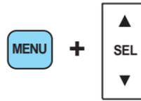
When in FM mode and RDS is activated, press the MENU until TRAFFIC OFF displays. Press the SEL control to engage the feature. The display will read TRAFFIC ON.
