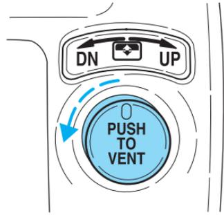
Turn control clockwise and release to raise the window all the way to the full closed position.
