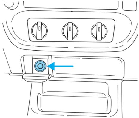
**Power outlets are designed for accessory plugs only. Do not hang any type of accessory or accessory bracket from the plug. Improper use of the power outlet can cause damage not covered by your warranty.**
