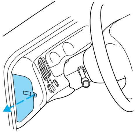
To remove a fuse use the fuse puller tool provided on the fuse panel cover.
