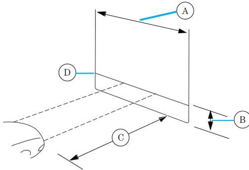
1. Measure the height from the center of your headlamp to the ground and mark a 2.4 meter (8 foot) horizontal reference line on the vertical wall or screen at this height (a piece of masking tape works well). The center of the lamp is marked by a 3.0 mm circle on the headlamp lens.
