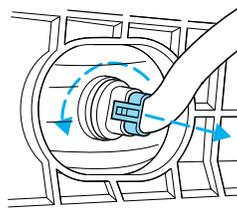
2. Disconnect the electrical connector from the foglamp bulb.
