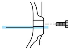
5. Install and tighten the fill plug securely.
