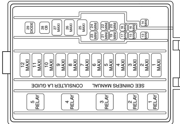
The high-current fuses are coded as follows.
