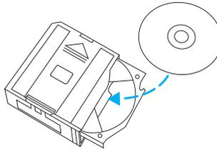
If you pull too hard on the disc holder, the disc holder may come completely out of the magazine. If this happens, reinsert the disc holder back into the magazine.
