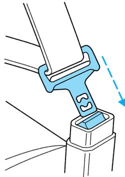
5. To put the retractor in the automatic locking mode, grasp the shoulder portion of the belt and pull downward until all of the belt is extracted and a click is heard.
