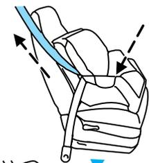
8. Allow the safety belt to retract to remove any slack in the belt.
