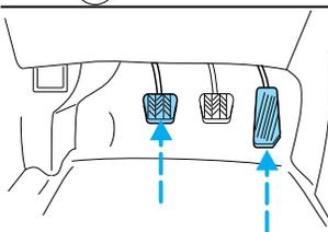
9. Slowly release the clutch pedal while slowly pressing down on the accelerator pedal.
