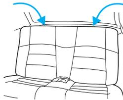
4. Access tether anchors located behind the seatback and pull away vinyl cover to expose anchors.
