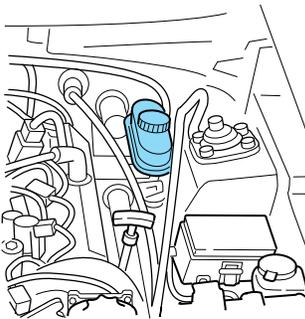
1. Clean the reservoir cap before removal to prevent dirt or water from entering the reservoir.
