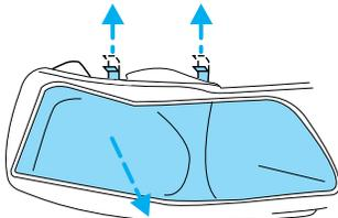
4. Pull headlamp assembly forward disengaging the lamp from the rear snap retainers to expose the back of the bulb.
