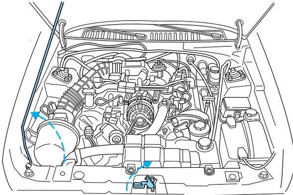
3. Lift the hood and secure it with the prop rod.
