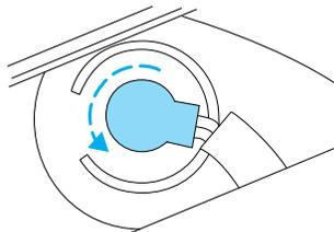
2. Pull the bulb straight out of the socket and push in the new bulb.
