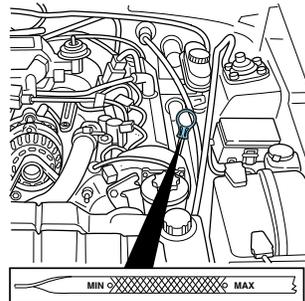
6. Wipe the indicator clean. Insert the indicator fully, then remove it again.
