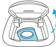
5. Clip the tether strap to the anchor as shown.
