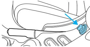
The power point is an additional power source for electrical accessories.
