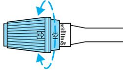
The bars of varying length are for intermittent wipers. When in this position rotate the control upward for fast intervals and downward for slow intervals.
