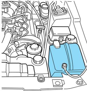
However, for severe usage or in high temperature climates, check the battery electrolyte level. Refer to the scheduled maintenance guide for the service interval schedules.
