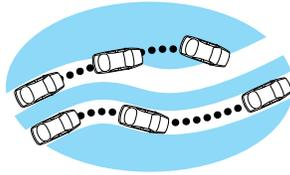
locking even when the brakes are firmly applied. The accompanying illustration depicts the advantage of an ABS equipped vehicle (on bottom) to a non-ABS equipped vehicle (on top) during hard braking with loss of front braking traction.
