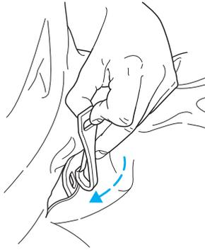
**If the tether strap is clipped incorrectly, the child safety seat may not be retained properly in the event of a collision.**
