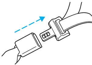
The front and rear outboard safety restraints in the vehicle are combination lap and shoulder belts. The front passenger and rear seat outboard safety belts have two types of locking modes described below:
