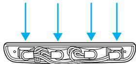
3. Remove the bulb socket by rotating it 45 degrees and pulling it out of the lamp assembly.
