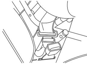
Ford recommends the use of a child safety seat having a top tether strap. Install the child safety seat in a seating position which is capable of providing a tether anchorage. For more information on top tether straps, refer to *Attaching safety seats with tether straps*.
