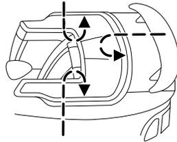
9. Fasten snap on boot to quarter trim panel on both sides of the vehicle.
