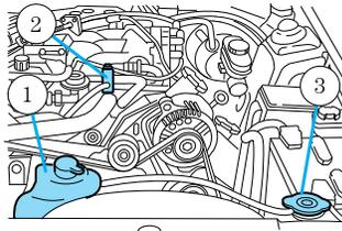
4. Add a **50/50 mixture** of engine coolant and distilled water to the radiator until full.
