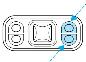
Press the control to move the seat forward, backward, up or down.
