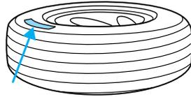
applicable on the tire sidewall between tread shoulder and maximum section width. For example:
