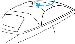
6. Push the convertible top switch on the console in front of the armrest and hold until the top is completely stored.
