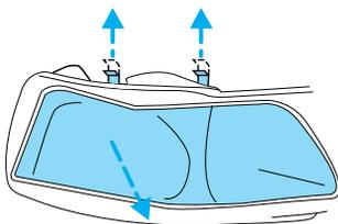
3. Pull headlamp assembly forward disengaging the lamp from the rear hidden snap retainers to expose the back of the bulb.
