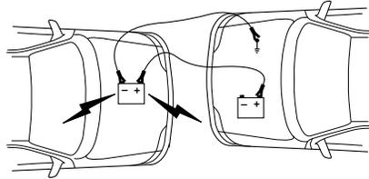
**Remove the jumper cables in the reverse order that they were connected.**
