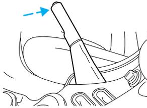
Push the button on the end of the parking brake handle and push the handle down as far as possible. Driving with the parking brake applied will cause the brakes to wear out quickly and reduce fuel economy.
