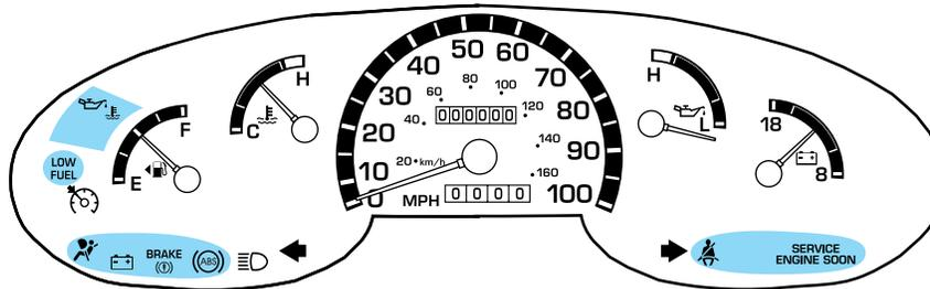
Make sure the corresponding lights illuminate or illuminate briefly. If a light fails to illuminate, have the vehicle serviced.
