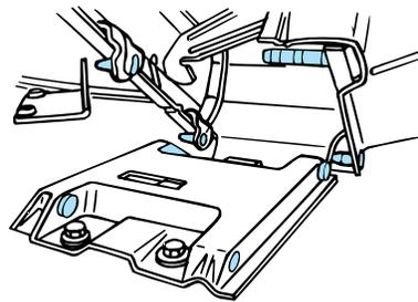
3. Pull the seat latch handle downward to lock the seat in position.
