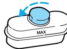
4. Use only a DOT 3 brake fluid certified to meet Ford specification ESA-M6C25-A. Refer to *Lubricant specifications* in this chapter.
