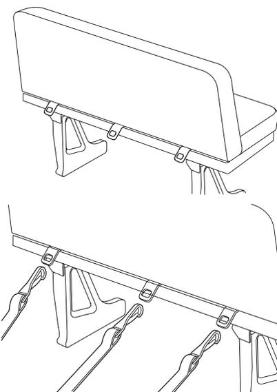
3. Clip the tether strap hook to the tether bracket mounted hook to the tether bracket mounted under rear rail of seat cushion frame.
