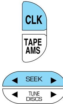
To set the minute, press and hold the CLK control and press the TUNE control:
