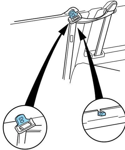
To make access to the 4th and 5th row seats easier, attach the 3rd and 4th row passenger side seat belts to the trim panel by using the snaps attached to the seat belt webbing and the trim panel.
