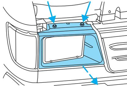
4. Remove the four headlamp bulb retaining screws and the retaining ring.
