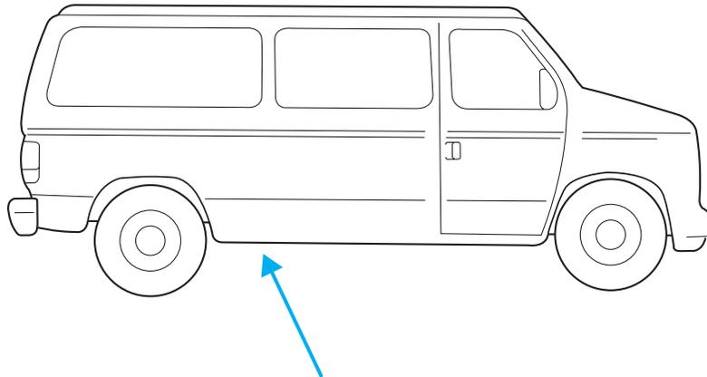
The auxiliary battery is located on the passenger side frame rail.
