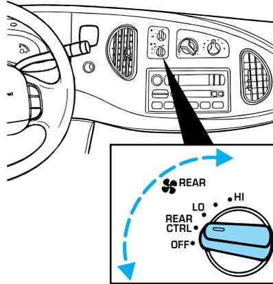
The fan speed of the auxiliary unit can be controlled either by the front seat using the front auxiliary control or by the rear seat passengers using the rear auxiliary control, but not both. To control the auxiliary unit using the rear control, the front control must be in the REAR position.
