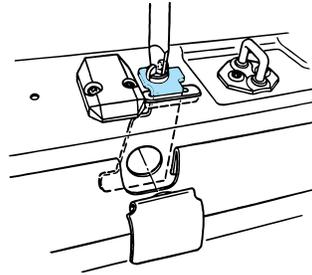
3. Remove the jack handle from the right side compartment and insert the tip of the jack handle through the access hole and into the tube.
