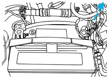
2. Wrap the secondary positive cable with a non-conductive material to insulate.
