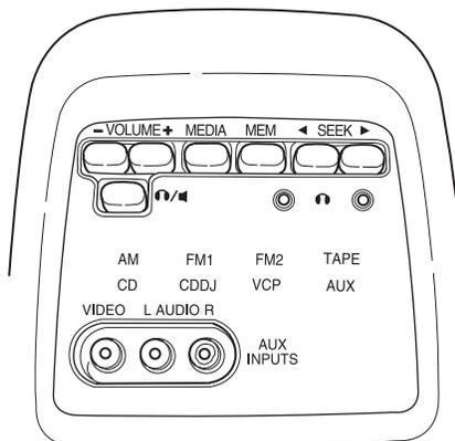
The AutoVision® controls allow the rear seat passengers to operate the radio, tape, CD or CD DJ(if equipped).
