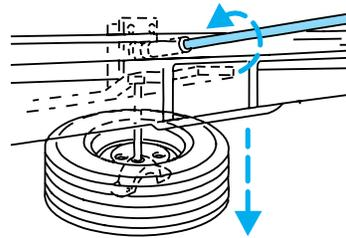
5. Remove the retainer from the spare tire.
