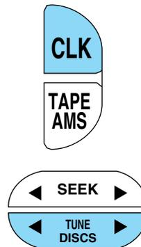
The CLK control will allow you to switch between media display mode (radio station, stereo information, etc.) and clock display mode (time).
