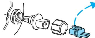
6. Remove the bulb retaining ring by rotating it counterclockwise (when viewed from the rear) to free it from the bulb socket, and slide the ring off the plastic base. Keep the ring to retain the new bulb.
