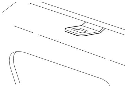
3. Route the child safety seat tether strap over the back of the front right-hand passenger seat as shown.
