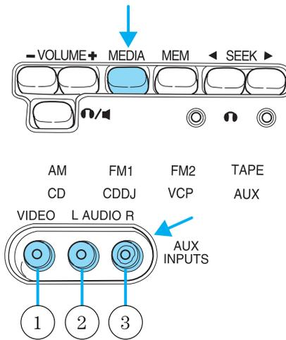
Press the MEDIA control until AUX is illuminated in the control panel. This will allow you to view the video and listen to the audio from the auxiliary input.
