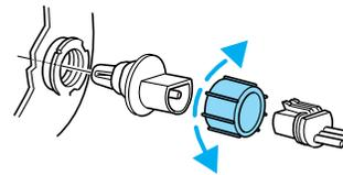
7. Without turning, remove the old bulb from lamp assembly by gently pulling it straight back out of the lamp assembly and replace.
