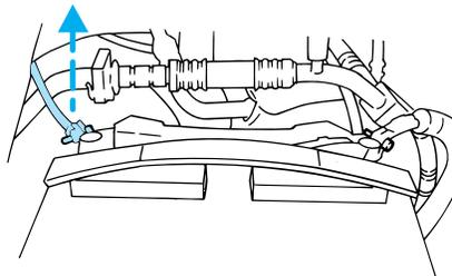
2. Disconnect the auxiliary battery frame ground.
