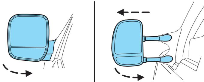
The telescoping feature (if equipped) allows the mirror to extend approximately 76 mm (3 inches).
