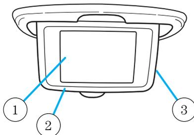
1. 6.4" (diagonal) color liquid crystal display (LCD) screen.
