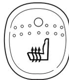
The heated seats will activate when the ignition is in the RUN position. When activated, they will turn off automatically after 10 minutes or when the ignition is turned to the OFF position.
