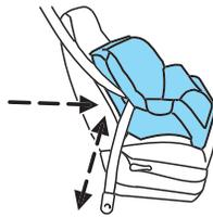
10. Try to pull the belt out of the retractor to make sure the retractor is in the automatic locking mode (you should not be able to pull more belt out). If the retractor is not locked, unbuckle the belt and repeat steps two through nine.
