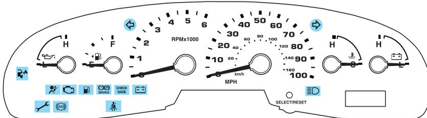
Warning lights and gauges can alert you to a vehicle condition that may become serious enough to cause expensive repairs. A warning light may illuminate when a problem exists with one of your vehicle's functions. Many lights will illuminate when you start your vehicle to make sure the bulb works. If any light remains on after starting the vehicle, have the respective system inspected immediately.
