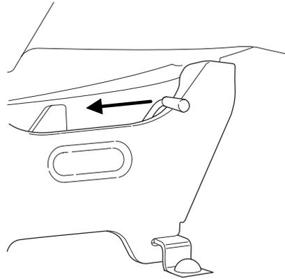
3. Move the seat rearward and lift the seats rear hooks away from the rear strikers prior to lifting the front hooks out from the front strikers.
