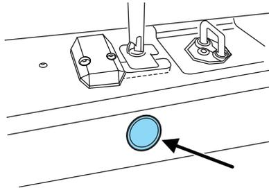
3. Remove the jack handle from the right side compartment and insert the tip of the jack handle through the access hole and into the tube.
