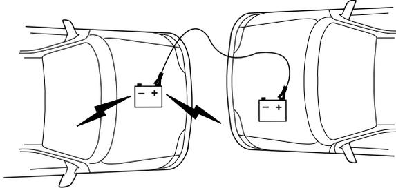
2. Connect the other end of the positive (+) cable to the positive (+) terminal of the assisting battery.
