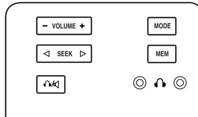
This feature allows front and middle seat passengers to listen to different media sources (radio, cassette, CD or DVD) simultaneously. (However, the front and middle-seat passengers cannot listen to two different radio stations at the same time.)
