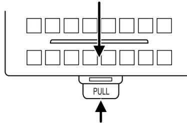
To reinstall the fuse box cover, place the top part of the cover on the fuse panel, then push the bottom part of the cover until you hear it click shut. Gently pull on the cover to make sure it is seated properly.
