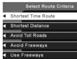
1. **Shortest time route** — Creates a driving route which minimizes driving time taking into consideration things such as speed limits, number of turns, etc.
