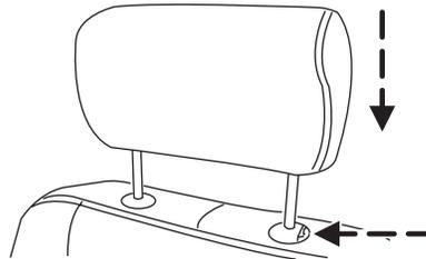
If the head restraint becomes detached, replace the notched bar into the bezel while holding the release button.
