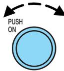
12. **Phone (if equipped):** If the phone button is pressed, the display will read NO PHONE. This button is non-functional (the radio will not mute). Cellular connectivity is not currently available for this radio.
