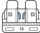
**Note:** Always replace a fuse with one that has the specified amperage rating. Using a fuse with a higher amperage rating can cause severe wire damage and could start a fire.
