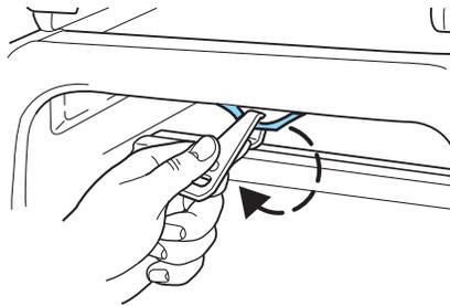
7. Tighten the child safety seat tether strap according to the manufacturer's instructions.
