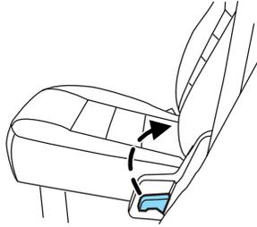
3. Locate the latch strap at the front of the seat and pull to release the seat into a kneel down load floor position. A moderate force may be required to move the seat forward and down.
