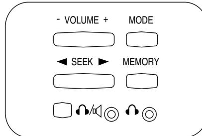
If your vehicle is equipped with the Vehicle Navigation Radio, then it may also be equipped with rear seat radio controls.
