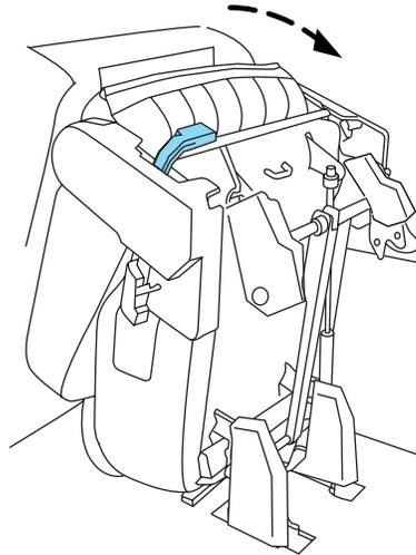
4. With the seat in the flat back position, lift up on the lever located on the side of the seat cushion. This will allow the seat back to be lifted to the upright locked position.
