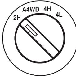
**Note:** If your vehicle is equipped with AdvanceTrac® with RSC, the AdvanceTrac® with RSC system will automatically turn off the stability enhancement feature when you shift the Control Trac A4WD system into 4L (4X4 LOW). The brake traction enhancement feature will still be enabled.
