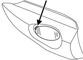
3. While holding the clip in the release position, pull the approach light module down.
