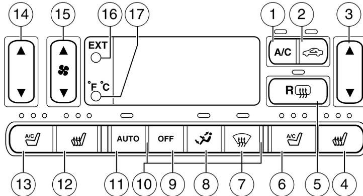
1. **A/C control:** Press to engage/disengage the air conditioning in all modes except defrost and floor/defrost. Uses outside air to cool the vehicle.
