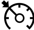
**O/D off:** Illuminates when the overdrive function of the transmission has been turned off, refer to the *Driving* chapter. If the light flashes steadily or does not illuminate, have the transmission serviced soon, or damage may occur.
