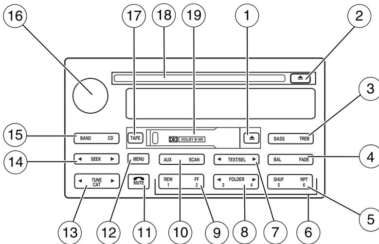
1. **EJ (Eject):** Press to stop and eject a tape.
