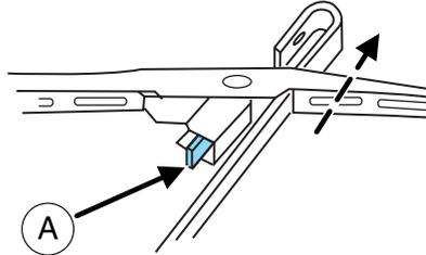
3. Install the new wiper blade on the arm and press it into place until a click is heard.
