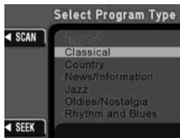
Use the cursor control to select the desired program type. The system will search for and begin playing that program type if available. During a seek or scan and for 10 seconds after a station is found, pressing the seek up/down or scan will initiate another search. If the desired type cannot be found, 'Not Found' appears in the display and the audio system returns to the original station.
