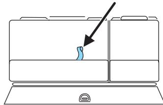
3. Locate the anchor webbing loop for the seating position.
