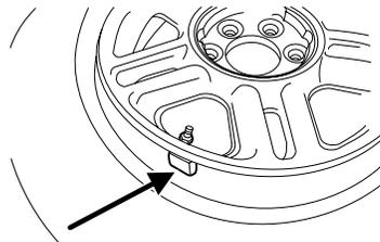
The tire pressure should be checked periodically (at least monthly) using an accurate tire gauge, refer to *Inspecting and inflating your tires* in this chapter.
