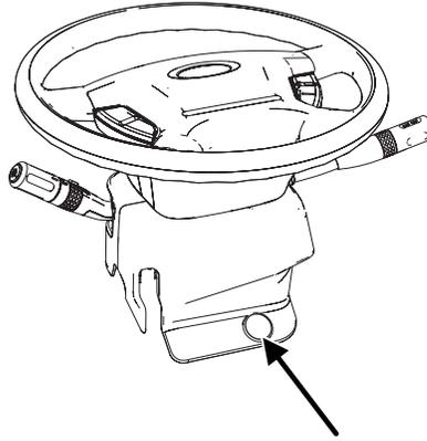
4. Remove the access plug using a flat-head screwdriver, then insert your finger and pull the override button toward you. With the button pulled toward you, apply the brake pedal and shift the transmission into N (Neutral).
