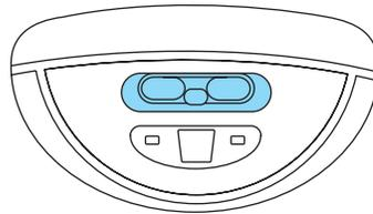
With the ignition key in the ACC or ON position, the rear dome lamp can be turned ON or OFF by sliding the control.
