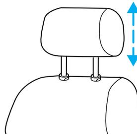
Push control to lower head restraint.
