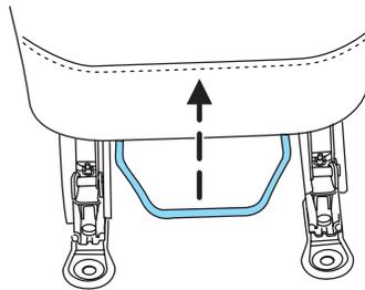
**Note: This seat can be moved forward to keep a child in a child restraint close to the front seat occupants. The seat should be moved to the full rearward position when it is occupied by older children or adults.**
