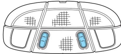
The map lamps are activated by pressing the controls on either side of the lens.
