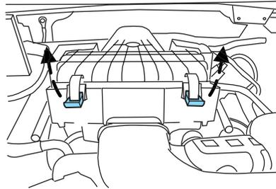
2. Pull air filter tray assembly out toward front of vehicle and lift air filter element up and out of housing.
