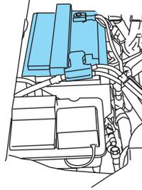
However, for severe usage or in high temperature climates, check the battery electrolyte level. Refer to the *scheduled maintenance information* for the service interval schedules.
