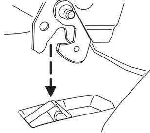
2. With the seat in the flat back position, lift up on the lever located on the side of the seat cushion. This will allow the seat back to be lifted to the upright locked position.
