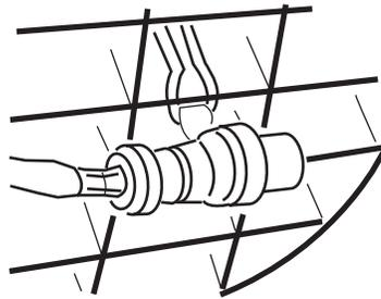
Use of an engine block heater is strongly recommended if you live in a region where temperatures reach  $-10^{\circ}\text{F}$  ( $-23^{\circ}\text{C}$ ) or below. For best results, plug the heater in at least three hours before starting the vehicle (the heater can be plugged in the night before starting the vehicle). To plug the heater in, remove the cap from the plug and insert the plug into a 110 volt grounded outlet. Be sure to re-attach the cap onto the plug when the heater is not in use.
