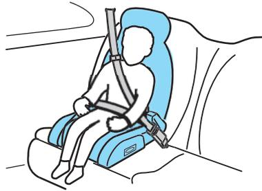
Both can be used in any vehicle in a seating position equipped with lap/shoulder belts if your child is over 40 lb. (18 kg).
