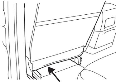
To remove climate controlled seat air filter:
