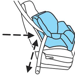
10. Try to pull the belt out of the retractor to make sure the retractor is in the automatic locking mode (you should not be able to pull more belt out). If the retractor is not locked, unbuckle the belt and repeat Steps 2 through 9.
