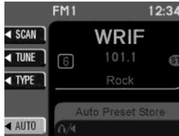
Any preset stored via the presets directly (pressing and holding) in this mode are temporary.
