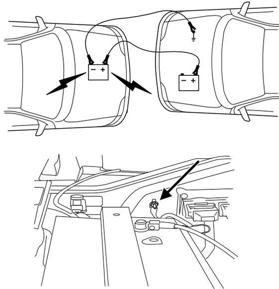
4. Make the final connection of the negative (-) cable to the jump starting stud located in the rear of the engine compartment, near the battery. **Do not** use fuel lines, engine rocker covers or the intake manifold as *grounding* points.
