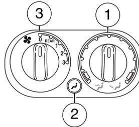
2. **Mode selector:** Press to select air flow direction to
