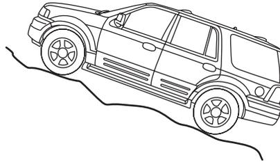
Apply just enough power to the wheels to climb the hill. Too much power will cause the tires to slip, spin or lose traction, resulting in loss of vehicle control.
