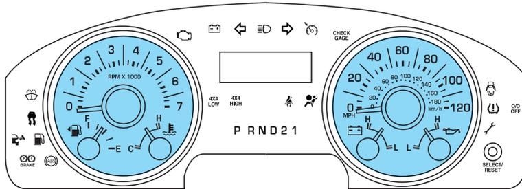
**Speedometer:** Indicates the current vehicle speed.
