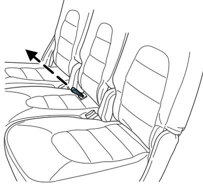
**To prevent possible damage to the seat or safety belts, ensure that the safety belts are not buckled when moving the seat to the load floor position.**
