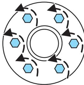
5. Position the jack according to the jack locator arrows found on the frame and turn the jack handle and extension tool assembly clockwise.
