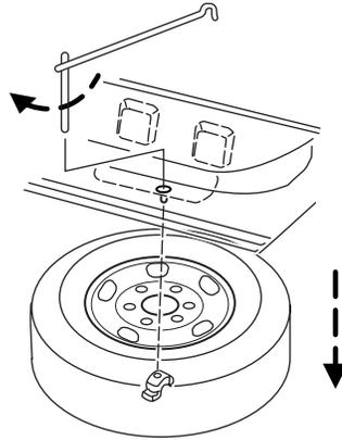
4. Turn the jack handle clockwise until the tire is raised to its stowed position underneath the vehicle. The wrench will become harder to turn and the spare tire winch will ratchet or slip when the tire is raised to maximum tightness. A clicking sound will be heard from the winch indicating that the tire is properly stowed.
