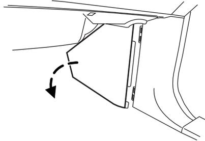
To remove the fuse box cover, place a finger behind the PULL tab and your thumb above the PULL tab as shown in the illustration, then pull the cover off.
