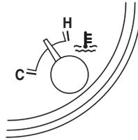
If the engine reaches a preset over-temperature condition, the engine will automatically switch to alternating cylinder operation. Each disabled cylinder acts as an air pump and cools the engine.
