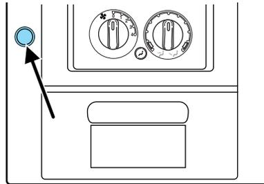
The rear auxiliary power point is located on the right rear quarter panel. The power point is accessible from the liftgate or the third row seat.
