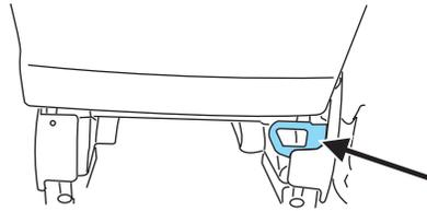
3. Route the child safety seat tether strap under the head restraint (outboard seats) and over the back of the seat.
