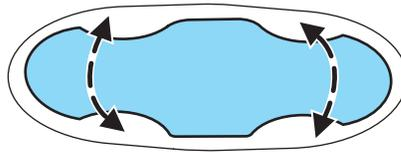
Press the control to move the seat forward, backward, up or down.
