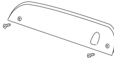
2. Pull the lamp assembly straight out.
