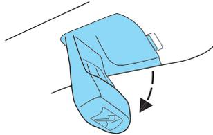
The conversation mirror on the cover allows the driver to view the rear seating area.
