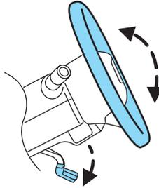
While holding the steering wheel, pull the lever up to its original position to lock the steering column.
