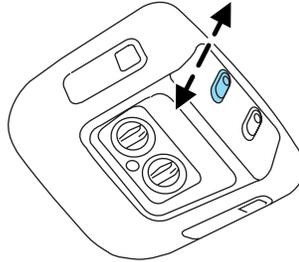
**To close the moon roof:** Press and hold the ▼ control until the glass panel stops at the “comfort” position. Press and hold the control again until the glass stops moving. When fully closed, the rear portion of the glass panel will appear higher than the front portion.
