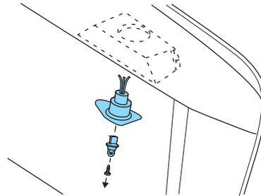
5. Install the bulb socket in the lamp assembly by turning it clockwise.
