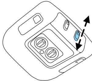
Press the ▲ portion of the VENT control to open the power rear quarter windows.
