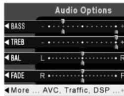
5. Use the cursor control to increase or decrease the levels. The higher the level selected, the greater the compensation. The levels will be shown in the display. Decrease all the way to the left to turn AVC off.
