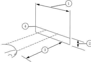
2. Measure the height from the center of your headlamp (indicated by a 3.0 mm circle on the lens) to the ground and mark an 8 foot (2.4 meter) horizontal reference line on the vertical wall or screen at this height (a piece of masking tape works well).
