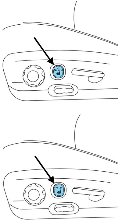
The heated seat icon in the Dual Automatic Temperature Control (DATC) will illuminate when activated.
