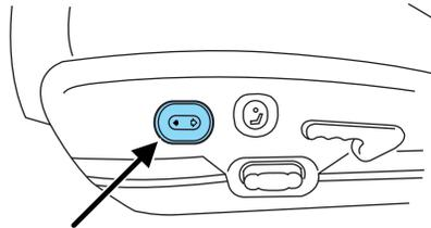
The power lumbar control is located on the outboard side of the seat.
