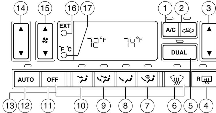
1. **A/C control:** Uses outside air to cool the vehicle. Press to turn on/off in all modes except
