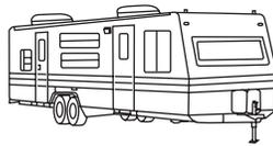
**GCW (Gross Combined Weight)** – is the weight of the loaded vehicle (GVW) plus the weight of the fully loaded trailer.
