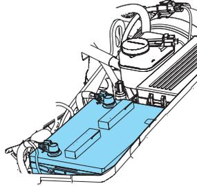
However, for severe usage or in high temperature climates, check the battery electrolyte level. Refer to *scheduled maintenance information* for the service interval schedules.
