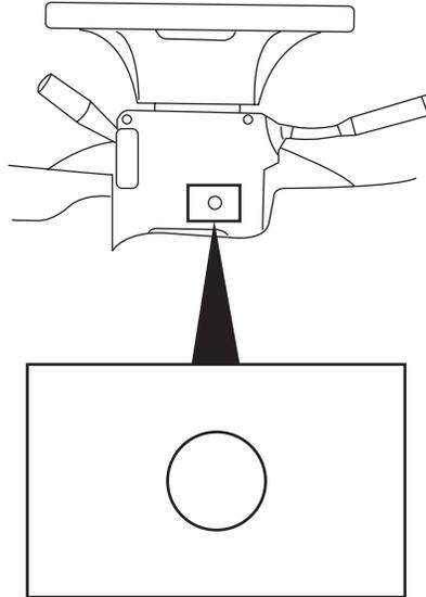
4. Insert a tool (or screwdriver) into the access hole to override the brake-shift interlock. Apply the brake and shift into Neutral.
