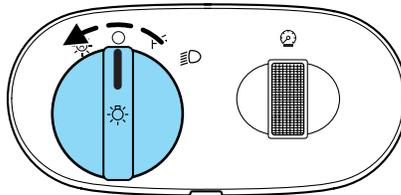
To turn the autolamps on, rotate the control counterclockwise to
