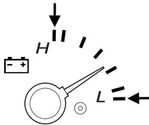
**Engine oil pressure gauge:** Indicates engine oil pressure. The needle should stay in the normal operating range (between "L" and "H"). If the needle falls below the normal range, stop the vehicle, turn off the engine and check the engine oil level. Add oil if needed. If the oil level is correct, have your vehicle checked at your dealership or by a qualified technician.
