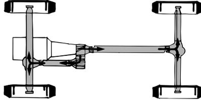
On some 4WD models, the initial shift from two-wheel drive to 4WD while the vehicle is moving can cause a momentary clunk and ratcheting sound. These sounds are normal as the front drivetrain comes up to speed and is not cause for concern.
