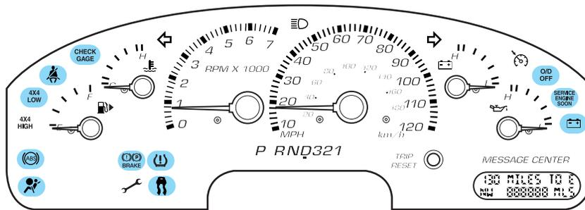
Make sure the corresponding lights illuminate or illuminate briefly. If a light fails to illuminate, have the vehicle serviced.
