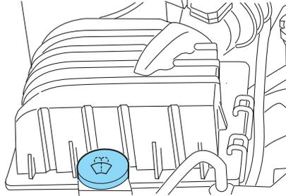
Only use a washer fluid that meets Ford specification WSB-M8B16-A2. Refer to *Lubricant specifications* later in this chapter.
