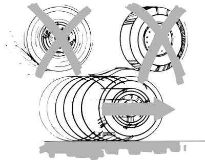
If your vehicle has anti-lock brakes, apply the brakes steadily. Do not “pump” the brakes.
