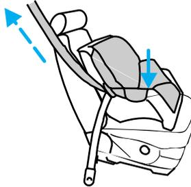
8. Allow the safety belt to retract to remove any slack in the belt.
