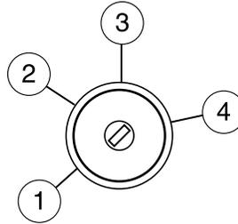
**Note:** If the engine does not start within five seconds on the first try, turn the key to OFF, wait 10 seconds and try again. If the engine still fails to start, press the accelerator to the floor and try again; this will allow the engine to crank with the fuel shut off in case the engine is flooded with fuel.
