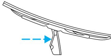
2. Attach the new wiper to the wiper arm and press it into place until a click is heard.
