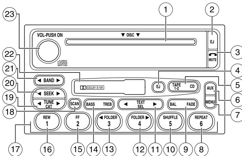
1. **CD slot:** Insert a CD with the label side up.
