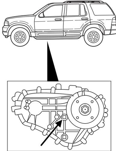
3. Add only enough fluid through the filler opening so that the fluid level is at the bottom of the opening.
