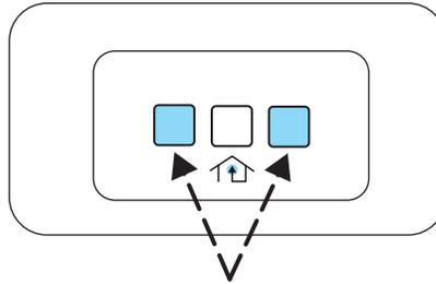
2. Position the end of your hand-held transmitter 1-3 inches (2-8 cm) away from the HomeLink® button you wish to program (located on your overhead console) while keeping the indicator light in view.
