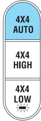
**4X4 AUTO** - Power to all four wheels; used for normal street and highway driving.
