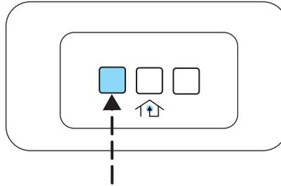
4. The indicator light will flash slowly and then rapidly. Release both buttons when the indicator light flashes rapidly. (The rapid flashing light indicates acceptance of the hand-held transmitters' radio frequency signals.)
