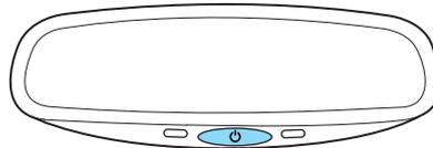
When the auto-dimming mirror is turned on, it will automatically return to the normal, high reflective, state whenever the vehicle is placed in R (Reverse) to ensure a clear view while backing up.
