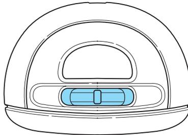
With the ignition in the ACC or ON position, the rear dome lamp can be turned ON or OFF by sliding the control.
