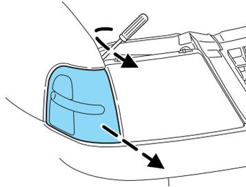
4. Rotate the bulb socket counterclockwise and remove it from the lamp assembly.
