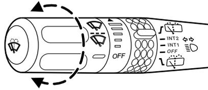
**Speed dependent wipers:** When the wiper control is on, the speed of the wipers will automatically adjust with the vehicle speed. The faster your vehicle is travelling the faster the wipers will go.
