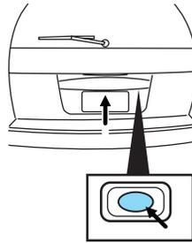
To lock the liftgate and the liftgate window, use the power door locks or press the door lock switch on the left side of the cargo area. To manually lock or unlock the liftgate, move the button located below the window down or up.
