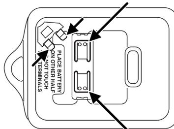
3. Remove the old battery. **Note:** Please refer to local regulations when disposing of transmitter batteries.
