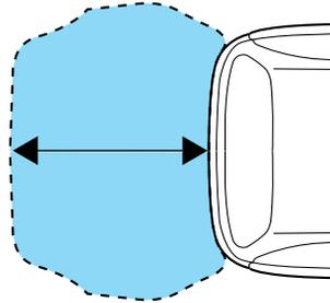
The RSS automatically turns on when the gear selector is placed in R (Reverse) and the ignition is ON. An RSS control on the instrument panel allows the driver to turn the RSS on and off. To turn the RSS off, the ignition must be ON, and the gear selector in R (Reverse). An indicator light on the control will illuminate when the system is turned off. If the indicator light illuminates when the RSS is not turned off, it may indicate a failure in the RSS.
