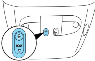
**To close the moon roof:** Press and hold the ▼ control until the glass panel stops at the “comfort” position. Press and hold the control again until the glass stops moving. When fully closed, the rear portion of the glass panel will appear higher than the front portion.
