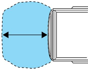
The RSS may have reduced performance or an increased chance of false detection if the tailgate is not locked and in the upright position. If the tailgate is down, the RSS tone may be heard intermittently or continuously. The tone may also be heard if items in the truck bed protrude rearward outside the bed.
