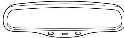
The mirror will automatically return to the normal state whenever the vehicle is placed in R (Reverse) to ensure a bright clear view when backing up.
