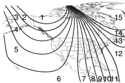
4. Press the ODO reset button in the cluster, hold for six seconds and release. You will see that ZONE appears in the instrument cluster display.
