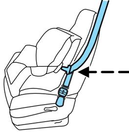
5. Insert the belt tongue into the proper buckle for that seating positions until you hear a snap and feel it latch. Make sure the tongue is securely latched to the buckle by pulling on the tongue.
