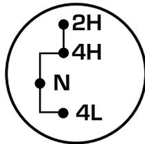
**2H (2WD High)** - Power to the rear wheels only; used for street and highway driving. Provides optimal smoothness and fuel economy at high speeds.
