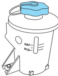
5. If the fluid is low, add fluid in small amounts, continuously checking the level until it reaches the range between the MIN and MAX lines. Be sure to put the cap back on the reservoir.
