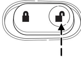
1. Turn the ignition to the 3 (ON) position, then press the
