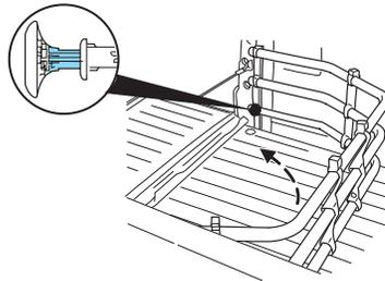
4. Evenly push down on the extender and push the round knobs in on each side locking it in place.
