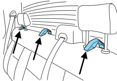
Many tether straps cannot be tightened if the tether strap is hooked to the loop directly behind the child seat. To provide a tight tether strap:
