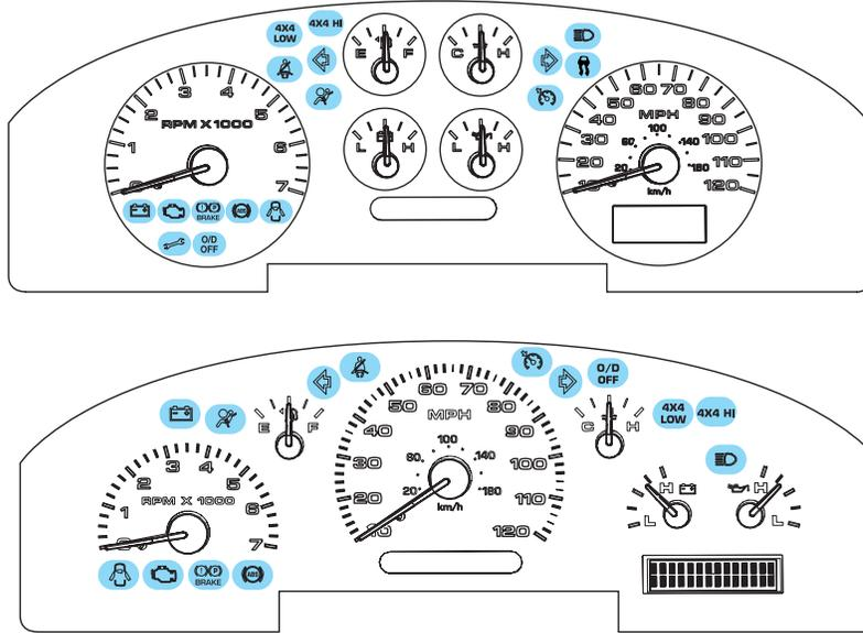
Make sure the corresponding lights illuminate or illuminate briefly. If a light fails to illuminate, have the vehicle serviced.
