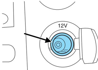
The auxiliary power point is located on the instrument panel.
