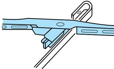
2. Attach the new wiper to the wiper arm and press it into place until a click is heard.
