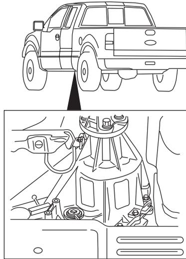
3. Add only enough fluid through the filler opening so that the fluid level is at the bottom of the opening.
