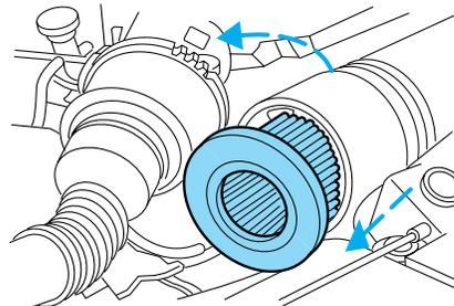
4. Install a new air filter element.
