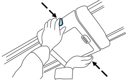
With pressure applied with palms and side latches squeezed down, pull downward on the entire storage bin and remove.
