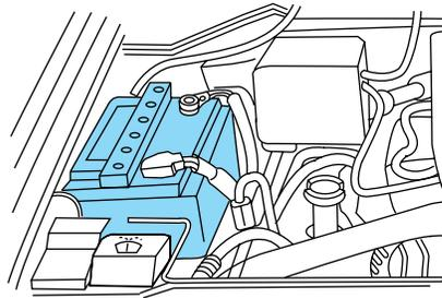
However, for severe usage or in high temperature climates, check the battery electrolyte level. Refer to the *scheduled maintenance information* for the service interval schedules.
