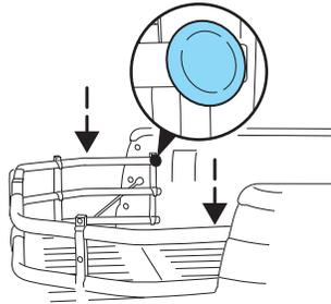
**Note: If the red marking on the shaft is visible, the bed extender is not locked or properly secured.**
