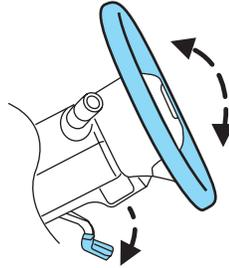
While holding the steering column, pull the lever up to its original position to lock the steering column.
