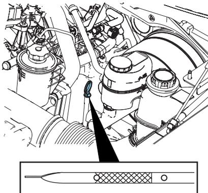
5. Locate and carefully remove the engine oil level indicator (dipstick).
