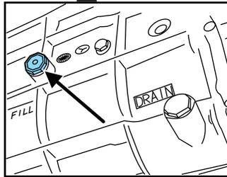
2. Remove the filler plug and inspect the fluid level.
