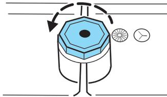
3. Fluid level should be at bottom of the opening.
