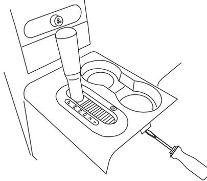
4. Press and hold the white button located along side the shifter housing assembly (as shown in the illustration). Press the gearshift lever release on the shifter knob and move the gearshift lever back to N (Neutral) (two places rearward from P [Park]).
