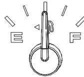
The arrow next to the fuel pump icon indicates which side of the vehicle the fuel filler door is located.
