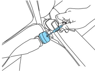
2. Insert the belt into the clip on the back panel. Protect the stowed belt if you carry cargo this may damage or soil the belt.
