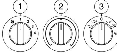
2. **Temperature selection:** Controls the temperature of the airflow in the vehicle.
