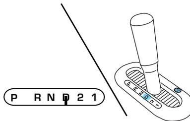
Overdrive can be deactivated by pressing the transmission control switch on the end of the gearshift lever (column-shift transmission) or on the gearshift bezel (floor-shift transmission).
