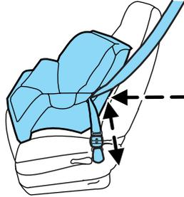
9. Check from time to time to be sure that there is no slack in the lap/shoulder belt. The shoulder belt must be snug to keep the lap belt tight during a collision.
