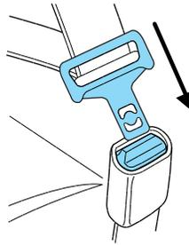
2. Grasp the shoulder portion and pull downward until the entire belt is extracted.
