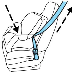
7. Allow the safety belt to retract and remove any slack in the belt to securely tighten the child safety seat in the vehicle.
