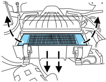
The air filter box needs to be free of any debris before installing a new air filter.
