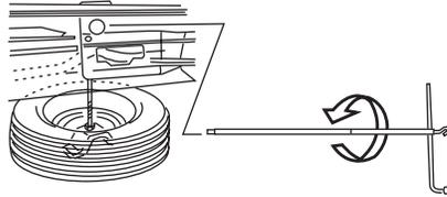
3. Turn the handle counterclockwise until tire is lowered to the ground, the tire can be slid rearward and the cable is slightly slack.
