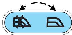
**Note:** The rear window switches will not illuminate when the window control is in the LOCKED position.
