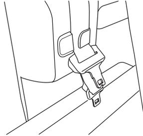
2. Buckle the small tongue on the end of the belt into the mini-buckle on the driver's side. The belt is now ready for use. This mini-buckle should stay buckled at all times unless cargo-carrying makes it necessary to detach the belt.
