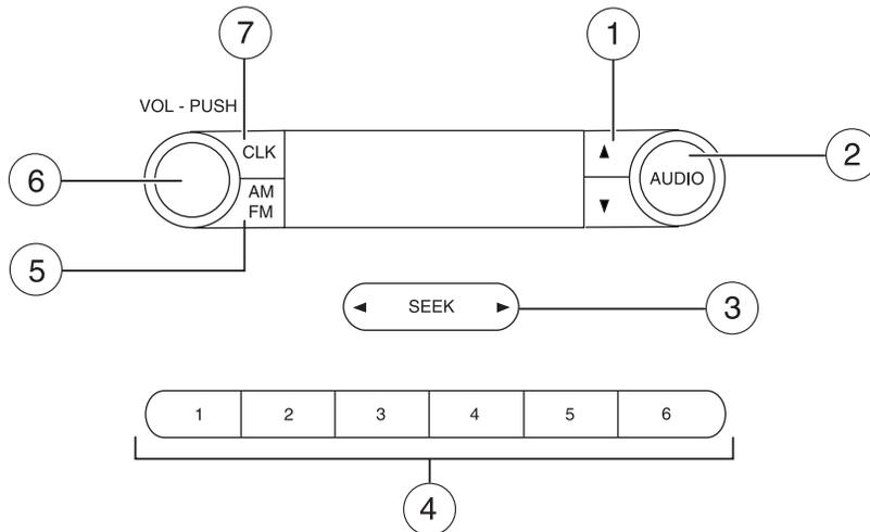
1. **▲ / ▼ Tuner:** Press to manually go up or down the radio frequency. Also use in menu mode to select various settings.
