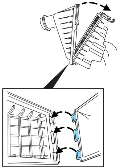
9. Reinstall the air cleaner assembly into the vehicle. Ensure the tabs on the inlet tube are secure in the sheet metal.
