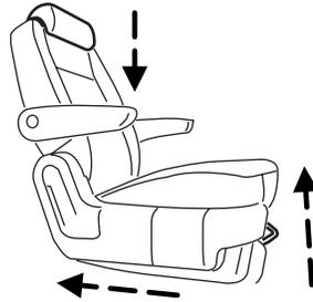
**Note:** Place the front row seat in a forward position to allow the 2nd row to be fully upright.
