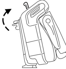
After entering the 3rd row seat, return the seat from the tumbled position and latch it to the floor.
