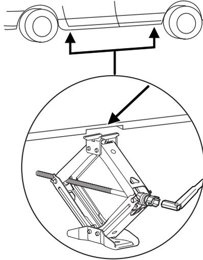
7. Turn the jack handle clockwise until the wheel is completely off the ground.
