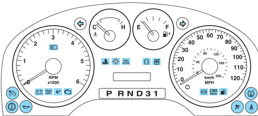
Make sure the corresponding lights illuminate or illuminate briefly. If a light fails to illuminate, have the vehicle serviced.
