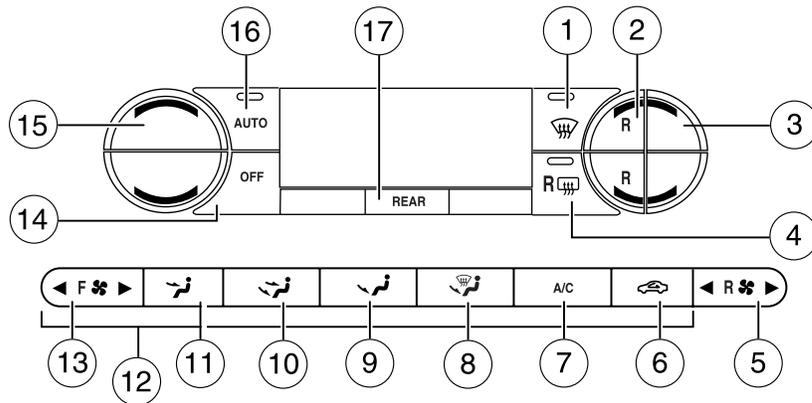
1. **Defrost:** Distributes outside air through the windshield defroster vents. Can be used to clear thin ice or fog from the windshield.
