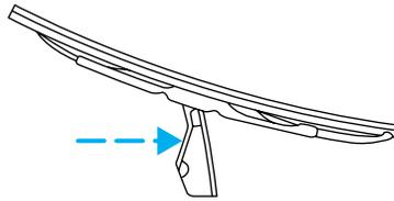
2. Attach the new wiper to the wiper arm and press it into place until a click is heard.
