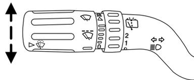
The cornering lamps feature (if equipped) automatically illuminates the left or right cornering lamps, located at the front corners of the vehicle, when the left or right turn signal, is activated. Cornering lamps are to provide better visibility of the area where the driver intends to turn.
