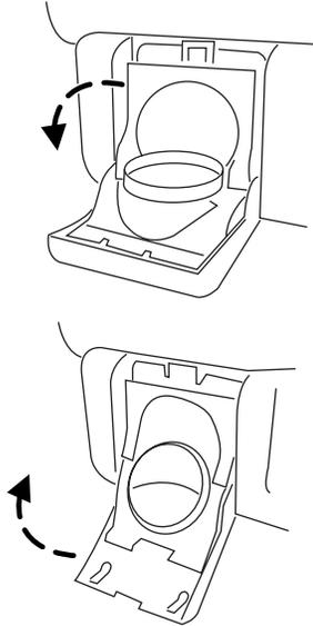
The cupholder is designed to detach from the seat when subjected to heavy load. The cupholder can be reinstalled by returning to the closed position.
