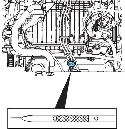
6. Wipe the indicator clean. Insert the indicator fully, then remove it again.
