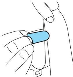
The end of the shoulder belt **must** be clipped in order to keep it from striking anything during vehicle operation.
