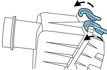
5. Remove the air filter element from the air filter housing.
