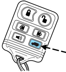
Press the control another two times within three seconds to close the power liftgate and turn off the interior lights.
