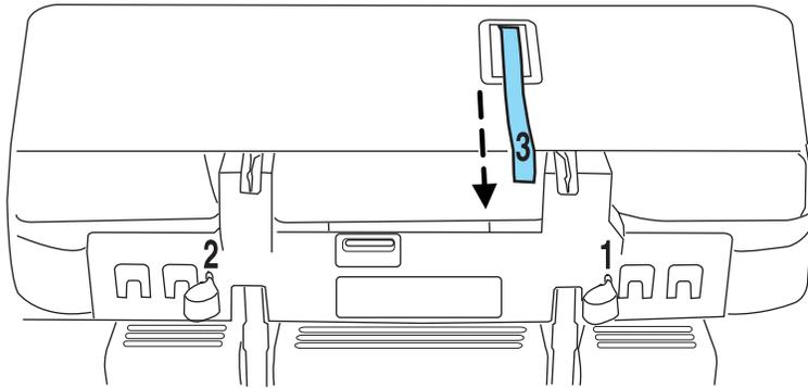
8. Pull the number 3 strap on the seat back to tumble seat all the way in to the tub in the floor.
