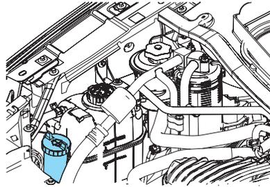
State or local regulations on volatile organic compounds may restrict the use of methanol, a common windshield washer antifreeze additive. Washer fluids containing non-methanol antifreeze agents should be used only if they provide cold weather protection without damaging the vehicle's paint finish, wiper blades or washer system.
