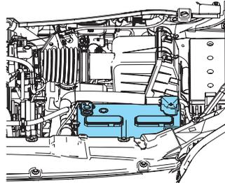
However, for severe usage or in high temperature climates, check the battery electrolyte level. Refer to *scheduled maintenance information* for the service interval schedules.
