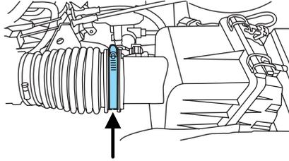
3. Remove the air cleaner assembly from the vehicle.
