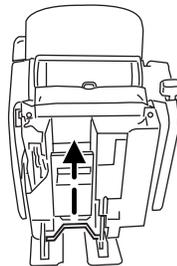
5. Rotate the seat rearward at a 30 to 45 degree angle.
