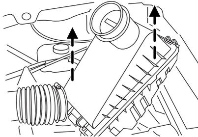
4. Release the two clamps that secure the cover to the air filter housing and place the cover aside.
