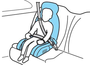
Both can be used in any vehicle in a seating position equipped with lap/shoulder belts if your child is over 40 lb. (18 kg).
