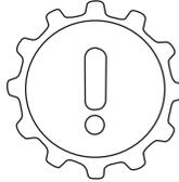
**Charging system:** Illuminates when the battery is not charging properly.
