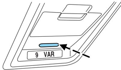
4. Press the button to increment the VAR number to the desired VAR number. Wait 5 seconds without button activity and the compass will return to the heading mode.
