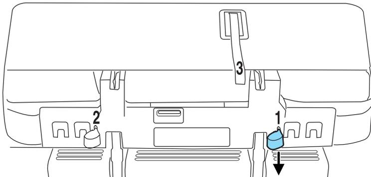
6. From the rear of the vehicle, fold seat back by **pulling and releasing** the number 1 strap.
