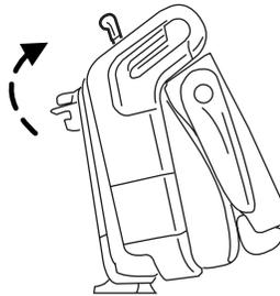
4. Rotate seat rearward until the back of the seat latches onto the floor.
