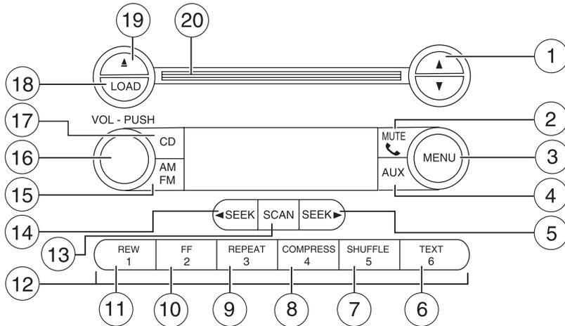
1. **▲ / ▼ Tuner:** Press to manually go up or down the radio frequency. Also use in menu mode to select various settings.
