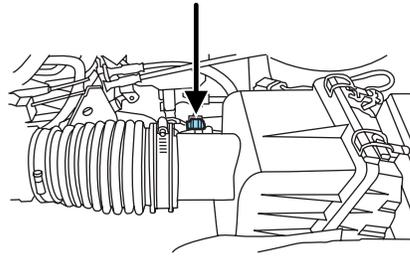
Reposition the locking clip (on the connector) and squeeze connector to remove.
