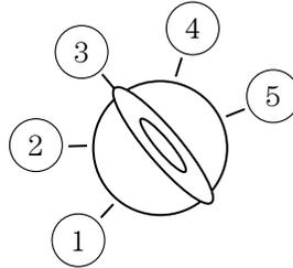
2. Turn ignition from the 4 (ON) position back to the 3 (OFF) position in order to remove the first **coded key** from the ignition.
