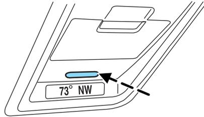
If the outside temperature falls below 3°C (38°F), the display will alternate from “ICE” to the outside temperature at a two second rate for one minute.
