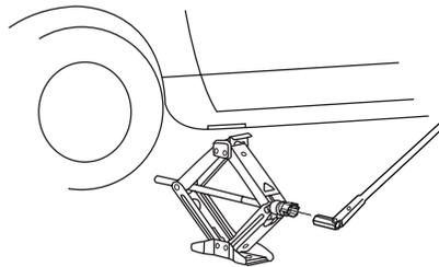
8. Remove the lug nuts with the lug wrench.
