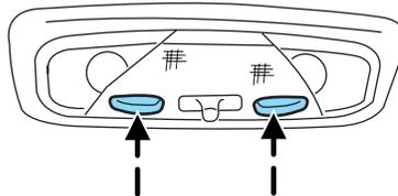
The dome lamp will illuminate whenever a front door is opened. If either front door has been opened from the outside, the lamp will remain on for 20 seconds after the door is shut. If any other door has been opened from the inside, the lamp will shut off immediately after the door is closed.
