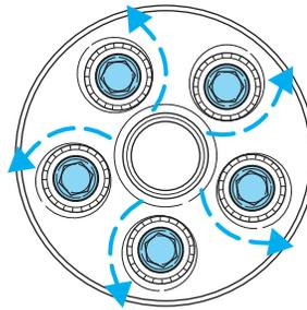
5. Loosen each wheel lug nut one-half turn counterclockwise but do not remove them until the wheel is raised off the ground.
