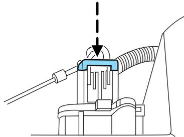
**Note:** If hose clamp is not secured properly or Mass Air Flow Sensor electrical connector is not properly installed the Check Engine light will illuminate when vehicle is operated.
