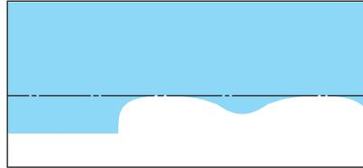
5. Locate the vertical adjuster on each headlamp, then use a # 2 Phillips screwdriver to turn the adjuster either counterclockwise (to adjust up) or clockwise (to adjust down) positioning the horizontal edge of the high intensity light on the horizontal reference line.
