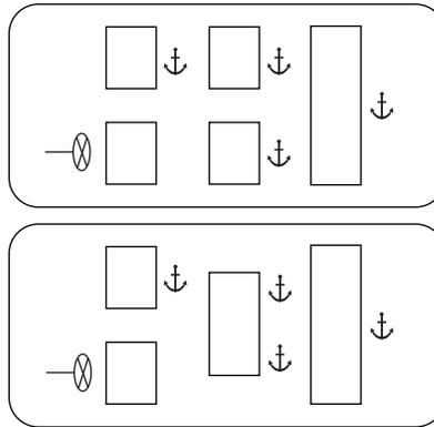
**The front passenger seat with power adjustment does not have a tether anchor.** The two tether anchors on the back of the second row bench seat can be used either for child safety seats at the two seating positions, or either anchor can be used for a single LATCH child seat installed at the center of the bench seat.
