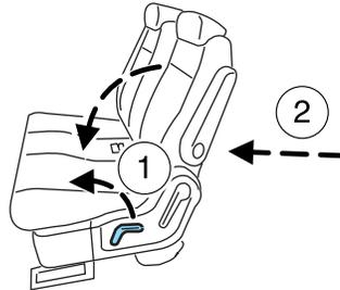
After entering the 3rd row, pull back the seatback until it latches. This will latch and lock the seatback and the seat track. The seatback and seat will not return to their original position.
