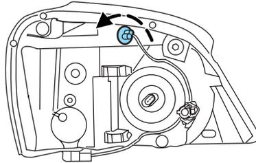
4. To remove the *parking/turn* bulb, turn the socket on the bottom of the headlamp assembly counterclockwise and pull the bulb straight out of the socket.
