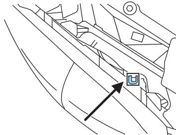
6. HORIZONTAL AIM IS NOT REQUIRED FOR THIS VEHICLE AND IS NON-ADJUSTABLE.
