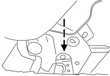
3. Rotate the seat forward until it latches onto the front pin.
