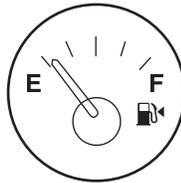
The arrow near the fuel pump icon indicates which side of the vehicle the fuel filler door is located.
