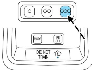
5. Press and hold the just-trained HomeLink® button and observe the HomeLink® house icon on the display. If the indicator light(s) underneath the house icon are constant, programming is complete and your device should activate when the HomeLink® button is pressed and released. **Note:** To program the remaining two HomeLink® buttons, begin with step 2 in the “Programming” section — **do not** repeat step 1.
