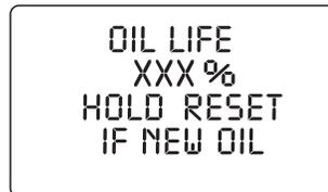
2. Press and hold the RESET control for 3 seconds and release. Oil life is set to 100% and “OIL LIFE START VALUE SET TO XXX%” is displayed.
