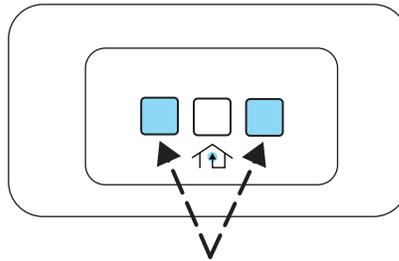
2. Position the end of your hand-held transmitter 1–3 inches (2–8 cm) away from the HomeLink® button you wish to program (located on your overhead console) while keeping the indicator light in view.
