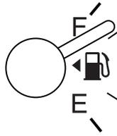
The arrow near the fuel pump icon indicates which side of the vehicle the fuel filler door is located.
