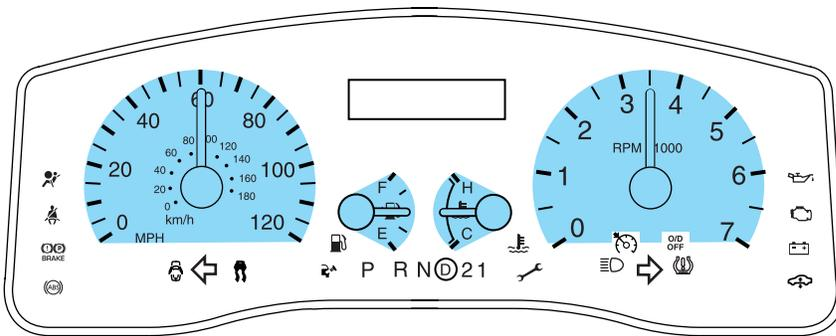
**Speedometer:** Indicates the current vehicle speed.
