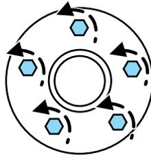
3. If equipped with a full wheelcover, remove the wheelcover center ornament then loosen the five black plastic nuts which retain the wheelcover using the lug wrench.
