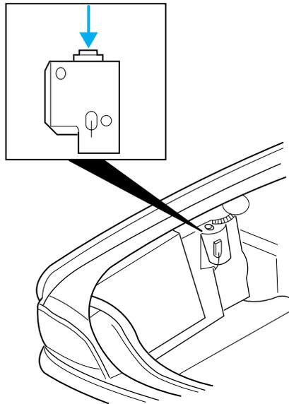
Use the following procedure to reset the fuel pump shut-off switch.
