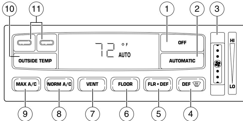
1. **OFF:** Outside air is shut out and the fan will not operate.
