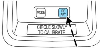
5. Drive the vehicle in a tight circle in a magnetically clean area such as an open parking lot.
