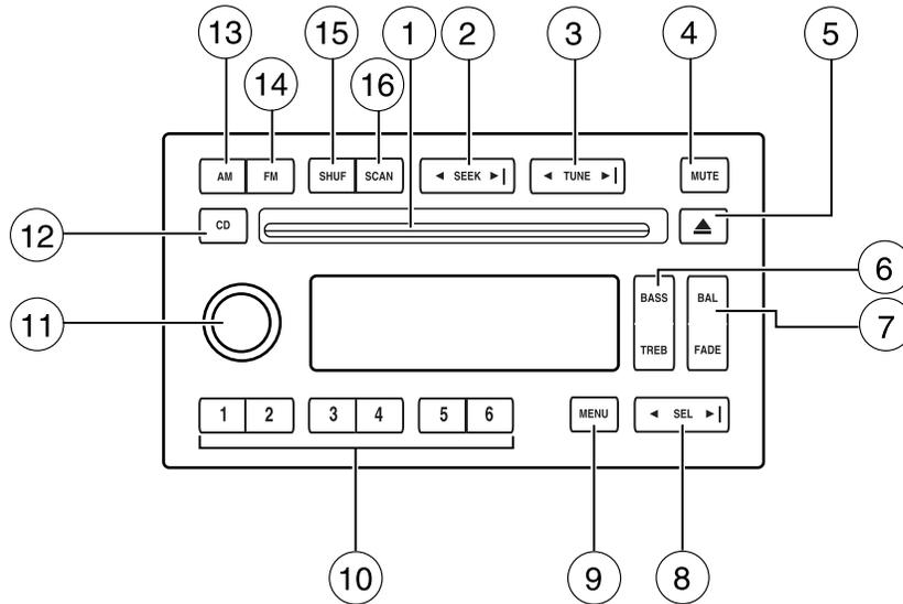
1. **CD slot:** Insert a CD, label side up. With the ignition on, the radio will begin play when a CD is inserted. If the ignition is off, press CD prior to inserting a disc. Do not force a disc into the system as damage could result.
