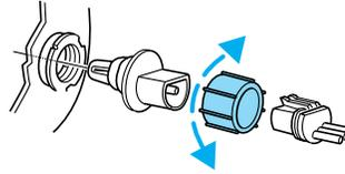
6. Without turning, remove the old bulb from the lamp assembly by gently pulling it straight back out of the lamp assembly.
