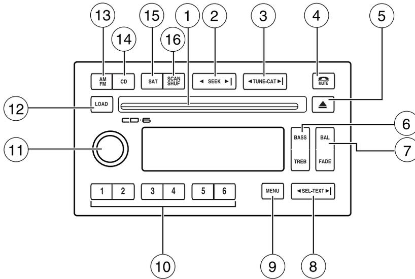
1. **CD slot:** To insert a CD, press LOAD. When the system is ready, insert a CD, label side up.
