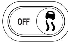
The traction control indicator flashes during a Traction Control™ system event.
