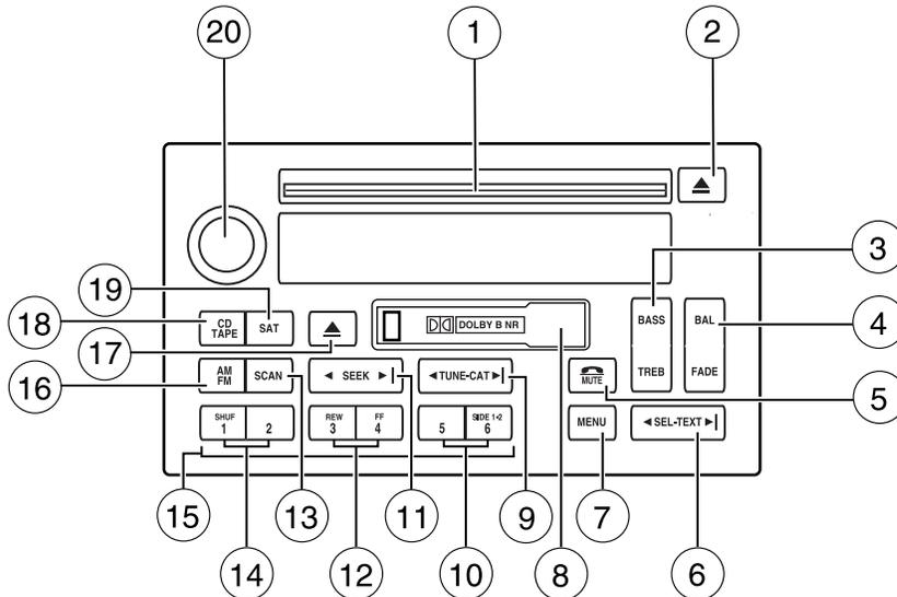
1. **CD slot:** Insert a CD, label side up. With the ignition on, the radio will begin to play a CD once inserted. With the ignition off, the CD control must be pressed before inserting the disc. Failure may result in damage to the CD and/or audio system.
