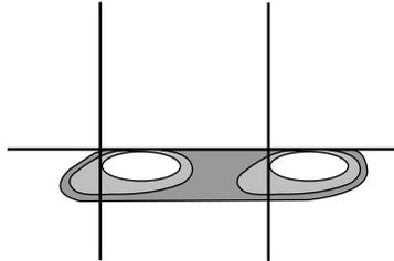
5. Locate the vertical adjuster for each headlamp. Adjust the aim by turning the adjuster control either clockwise (to adjust down) or counterclockwise (to adjust up).
