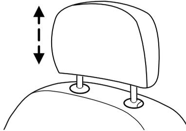
Push control to lower head restraint.
