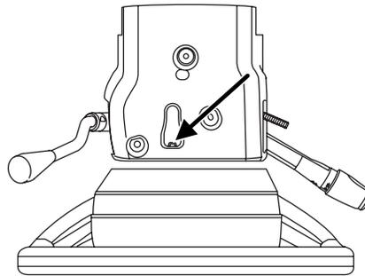
3. Remove the access plug using a flat head screwdriver. Insert the screwdriver into the access hole nearest the steering wheel. Then push and hold the override button using a flat head screwdriver. Apply the brake pedal and shift the transmission into N (Neutral) while continuing to depress the override button.
