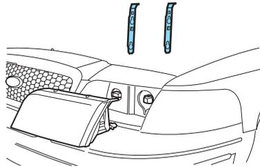
4. Disconnect the electrical connector from the bulb by pulling rearward.
