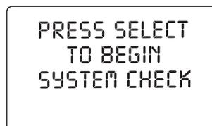
Pressing the SELECT control cycles the message center through each of the systems being monitored.
