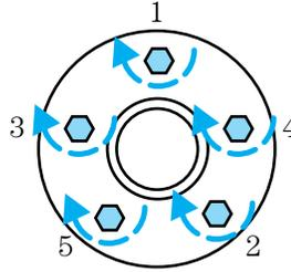
9. For full size spare aluminum wheel, firmly install the center ornament. If equipped with a full size spare tire/wheel assembly and lug nut retained full wheelcover, install the wheelcover by tightening the five black plastic nuts in the order shown on the wheelcover using the lug wrench with about 80 lb. in. (9 N•m) torque. Then firmly install the wheelcover center ornament.
