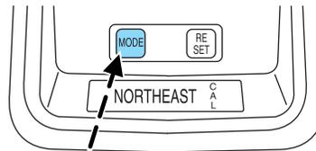
2. Hold down the MODE button for 10 seconds to enter the calibration mode. The display will read PRESS RESET TO DECAL.
