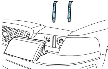
5. Remove the bulb retaining ring by rotating it counterclockwise (when viewed from the rear) to free it from the bulb socket, and slide the ring off the plastic base. Keep the ring to retain the new bulb.
