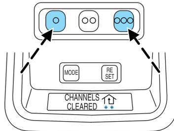
**Do not** repeat step one to program additional hand-held transmitters to the remaining two HomeLink® buttons. This will erase previously programmed hand-held transmitter signals into HomeLink®.
