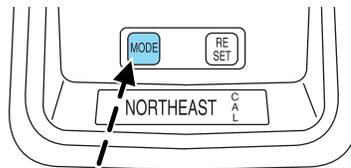
2. Hold down the MODE button for 5 seconds to enter zone mode. The display will read PRESS RESET TO SET ZONE XX where XX is the current zone.
