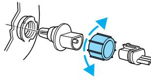
6. Remove the old bulb from the lamp assembly by gently pulling it straight back out of the lamp assembly.
