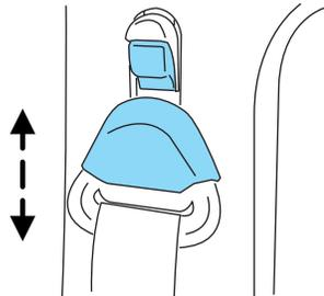
Pull down on the height adjuster to make sure it is locked in place.
