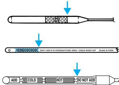
Fluid levels above the safe range may result in transmission failure.
