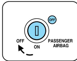
**WARNING:** If the light fails to illuminate when the passenger air bag switch is in the OFF position and the ignition switch is in ON, have the passenger air bag switch serviced at your Ford or Lincoln-Mercury dealer immediately.
