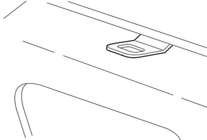
3. Route the child safety seat tether strap over the back of the front right-hand passenger seat as shown.
