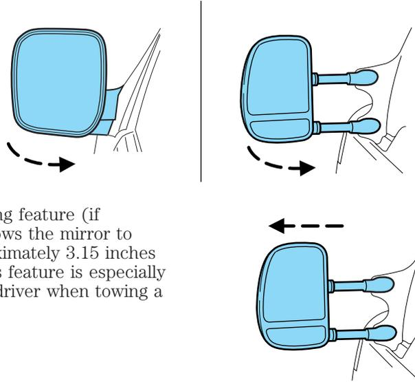
The telescoping feature (if equipped) allows the mirror to extend approximately 3.15 inches (80 mm). This feature is especially useful to the driver when towing a trailer.
