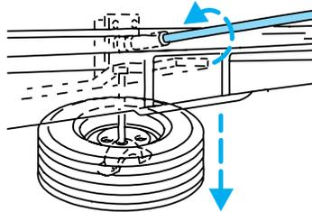
5. Remove the retainer from the spare tire.
