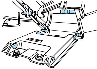
2. Pull the seat latch handle downward to lock the seat in position.
