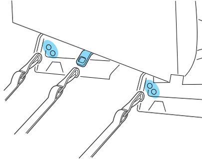
4. Install the child safety seat tightly using the LATCH anchors or safety belts. Follow the instructions in this chapter.
