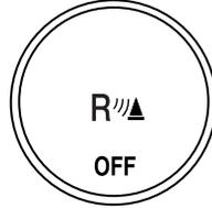
(Reverse). An indicator light on the control will illuminate when the system is turned off. If the indicator light illuminates when the RSS is not turned off, it may indicate a failure in the RSS. The RSS will remain off until either the RSS control is pushed again or the ignition switch is recycled.
