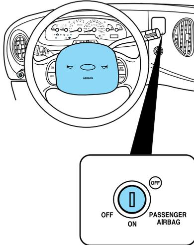
**WARNING:** An airbag ON/OFF switch (if equipped) may have been installed in this vehicle. Before driving, *always* look at the face of the switch to be sure the switch is in the proper position in accordance with these instructions and warnings. Failure to put the switch in a proper position can increase the risk of serious injury or death in a collision.
