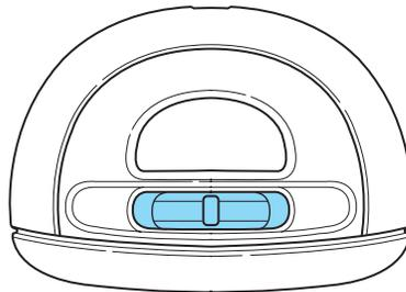
With the ignition key in the accessory or on position, the rear dome lamp can be turned on or off by sliding the control.
