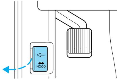
2. Go to the front of the vehicle and push the auxiliary latch, located in the center top of the grill, to the left to release the hood.
