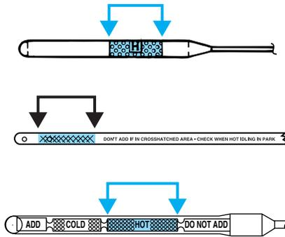
The transmission fluid should be in this range if at normal operating temperature (150°F-170°F [66°C-77°C]).
