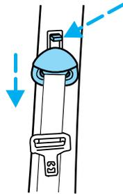
To adjust the belt upward, slide the adjuster up. Pull down on the height adjuster to make sure it is locked in place.
