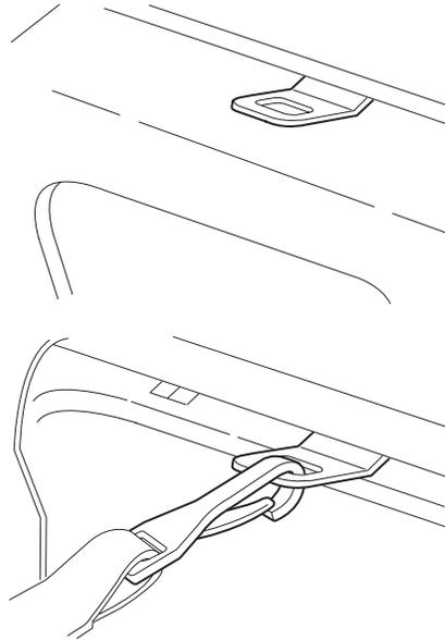
4. Install the child safety seat tightly using the LATCH anchors or safety belts. Follow the instructions in this chapter.
