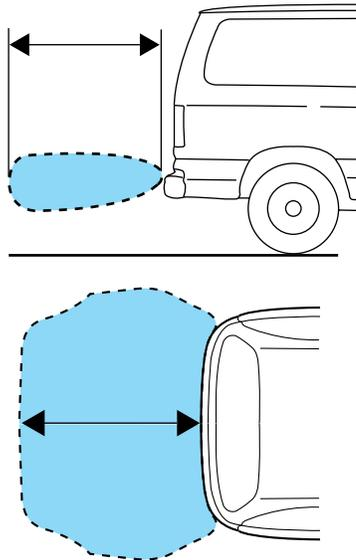
The RSS automatically turns on when the gearshift lever is placed in R (Reverse) and the ignition is on. An RSS control allows the driver to turn the RSS on and off. To turn the RSS off, the ignition must be ON, and the gear selector in R
