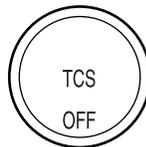
If you should become stuck in snow or ice or on a very slippery road surface, try switching the Traction Control™ system off. This may allow excess wheel spin to “dig” the vehicle out and enable a successful “rocking” maneuver. Remember to switch the Traction Control™ system back on once the vehicle is no longer stuck.
