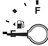
The FUEL icon and arrow indicates which side of the vehicle the fuel filler door is located.
