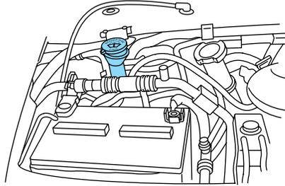
State or local regulations on volatile organic compounds may restrict the use of methanol, a common windshield washer antifreeze additive. Washer fluids containing non-methanol antifreeze agents should be used only if they provide cold weather protection without damaging the vehicle's paint finish, wiper blades or washer system.
