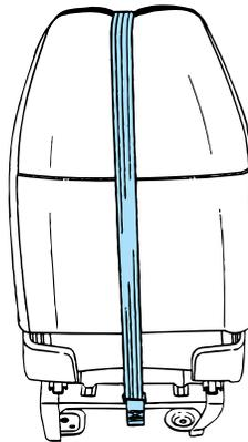
4. Clip the tether strap hook to the seat pedestal to the location shown.
