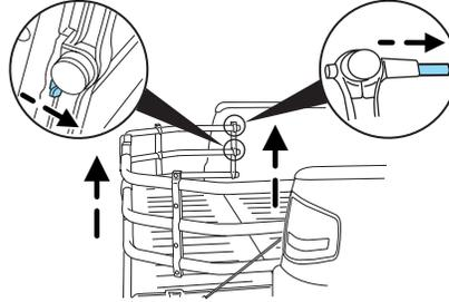
To install the cargo cage, follow the removal procedure in reverse order.
