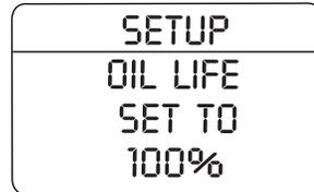
3. Once “OIL LIFE SET TO XXX%” is displayed, release and press the RESET control switch to change the Oil Life Start Value. Each release and press will reduce the value by 10 percent.
