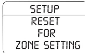
6. Press the RESET control repeatedly until the correct zone setting for your geographic location is displayed on the message center. The range of zone values are from 01 to 15 and “wraps” back to 01.
