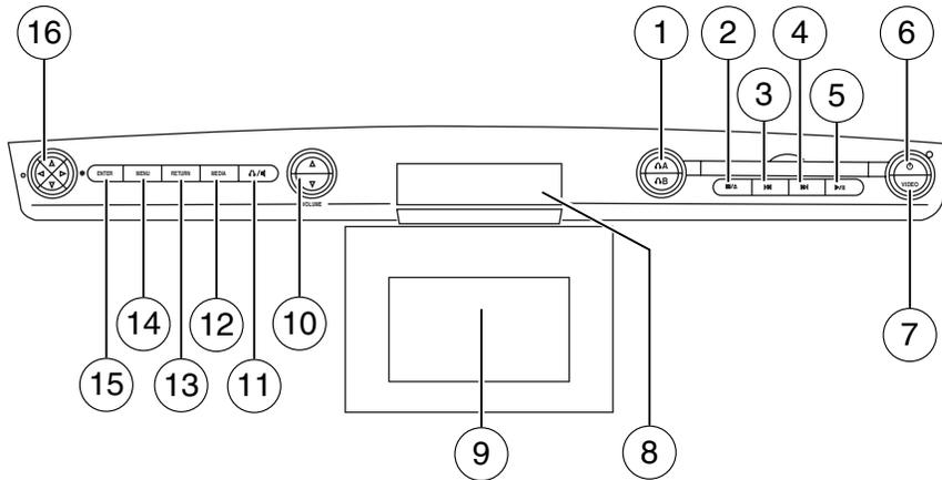
1. **Headphone control A/B:** Press to select either the A or B headphone source. Then press MEDIA to select the desired playing media for that headset. When a headphone channel has been selected (A or B), selections will affect the source on that channel only.
