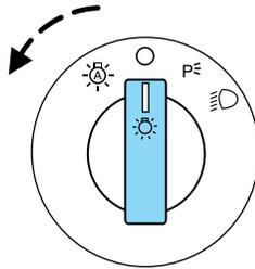
To turn the autolamps on, rotate the control counterclockwise to
