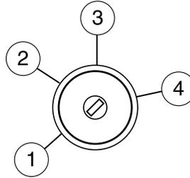
2. Turn the ignition from the 1 (OFF/LOCK) position to the 3 (ON) position. Keep the ignition in the 3 (ON) position for at least three seconds, but no more than 10 seconds.
