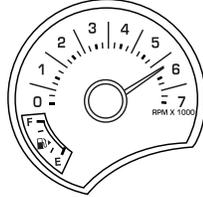
**Fuel gauge:** Indicates approximately how much fuel is left in the fuel tank (when the ignition is in the ON position). The fuel gauge may vary slightly when the vehicle is in motion or on a grade.
