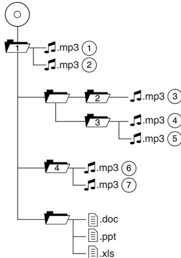
In track mode, the system will display and play the structure as if it were only one level deep (all .mp3 files will be played, regardless of being in a specific folder). In folder mode, the system will only play the .mp3 files in the current folder.
