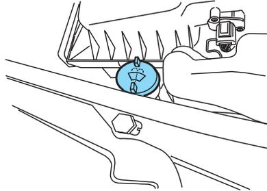
Only use a washer fluid that meets Ford specification WSB-M8B16-A2. Do not use any special washer fluid such as windshield water repellent type fluid or bug wash. They may cause squeaking, chatter noise, streaking and smearing. Refer to the *Maintenance product specifications and capacities* section in this chapter.
