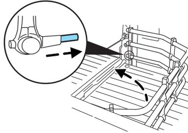
4. Evenly push down on the cargo cage and push the lever in on each side locking it in place.
