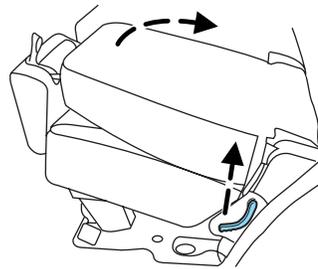
2. Lift up on the head restraint until it locks into its original position.
