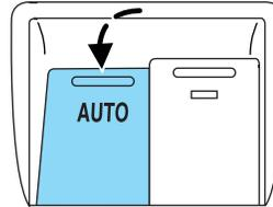
If the switch is pressed and held to the normal close or ONE TOUCH UP position during a ONE TOUCH DOWN event, the window will stop. If, after 1/2 second the switch is still held, the window will perform a normal close or ONE TOUCH UP.
