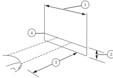
3. Turn on the low beam headlamps. The brightest part of the light should be below the horizontal line (4). If it is above the line the headlamp will need to be adjusted.
