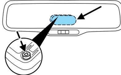
4. Press and hold the reset button on the compass module for approximately 4 seconds until COMPASS ZONE XX appears in the message center display.
