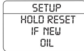
2. Press and hold the RESET control for more than 2 seconds. Oil life is set to 100% and “OIL CHANGE SET TO 100%” is displayed.
