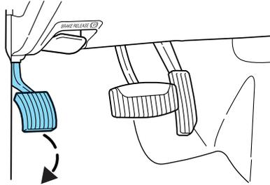
The BRAKE warning lamp in the instrument cluster illuminates and remains illuminated (when the ignition is turned ON) until the parking brake is released.
