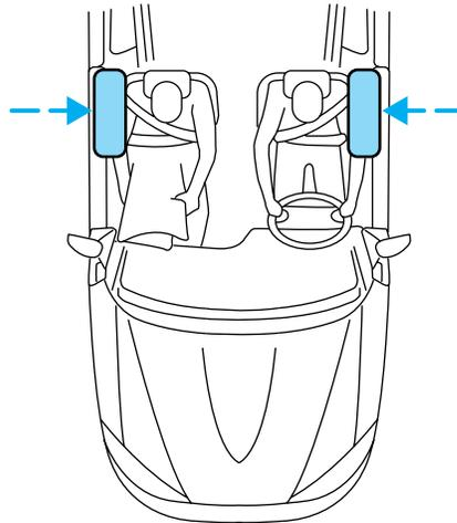
Side airbags, in combination with safety belts, can help reduce the risk of severe injuries in the event of a significant side impact collision.
