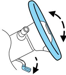
Lift the lever back to its original position to lock the steering column.
