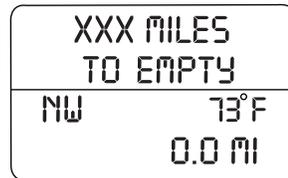
The DTE function will display LOW FUEL LEVEL and sound a tone for one second when you have approximately 50 miles (80 km) to empty. If you RESET this warning message, this display and tone will return within 10 minutes.
