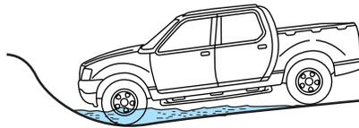
Once through water, always try the brakes. Wet brakes do not stop the vehicle as effectively as dry brakes. Drying can be improved by moving your vehicle slowly while applying light pressure on the brake pedal.
