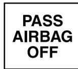
**Note:** The indicator lamp will illuminate for a short period of time when the ignition is turned to the ON position to confirm it is functional.
