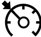
**Upshift (if equipped):** To maximize fuel economy, this light illuminates when the manual transmission should be shifted to the next highest gear. Refer to the *Driving* chapter for more information.
