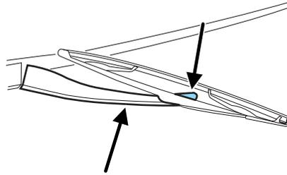
2. Grab the primary structure of the blade with the other hand close to the arm/blade joint.
