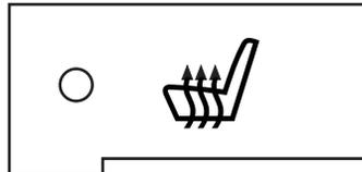
The heated seats will activate when the ignition is in the on position.
