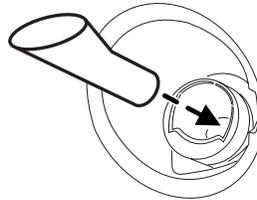
3. Fill the vehicle with fuel from the portable fuel container.
