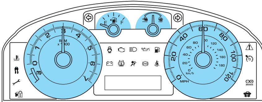
**Speedometer:** Indicates the current vehicle speed.
