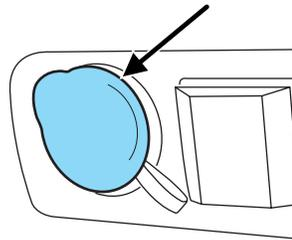
To prevent the fuse from being blown, do not use the power point(s) over the vehicle capacity of 12 VDC/180W. If the power point or cigar lighter socket is not working, a fuse may have blown. Refer to *Fuses and relays* in the *Roadside Emergencies* chapter for information on checking and replacing fuses.
