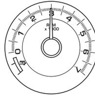
The pointer will indicate engine RPMs when the engine is running and point at the EV symbol when the engine is off and the vehicle is running on pure electrical power.
