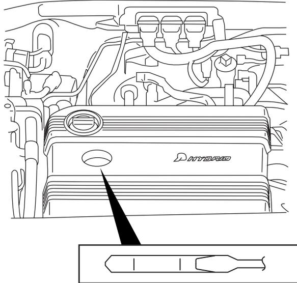
5. Locate and carefully remove the engine oil level dipstick.
