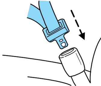
5. To put the retractor in the automatic locking mode, grasp the shoulder portion of the belt and pull downward until all of the belt is pulled out.
