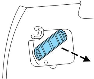
3. Install new filter and filter cover (note arrows indicating top side). The arrow on the filter cover and the arrow on the filter both point in the same direction (upward).
