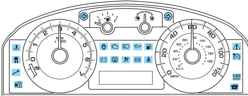
Warning lights and gauges can alert you to a vehicle condition that may become serious enough to cause extensive repairs. A warning light may illuminate when a problem exists with one of your vehicle's functions. Many lights will illuminate when you start your vehicle to make sure the bulbs work. If any light remains on after starting the vehicle, refer to the respective system warning light for additional information.
