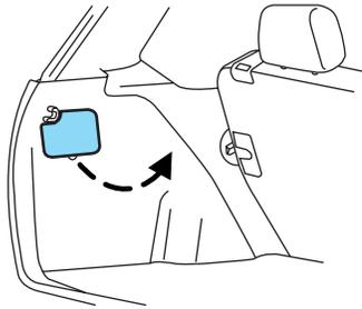
2. Push the tabs (located on each side of filter cover) while pulling gently to remove filter cover. Remove the old filter.
