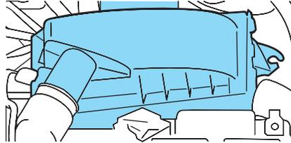
3. Remove the air filter element from the air filter housing.
