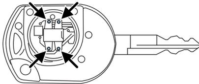
4. Insert the new battery. Refer to the instructions inside the IKT for the correct orientation of the battery. Press the battery down to ensure that the battery is fully seated in the battery housing cavity.
