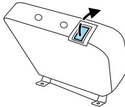
6. Rotate seatback down into load floor position.
