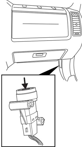
The high voltage shut-off switch is located in the cargo area on the passenger side of the vehicle in the jack compartment, behind the jack access door. The switch is located behind the jack.
