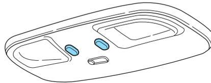
For models equipped with a moon roof, the map lamps are located on the moon roof control panel. Press the button on either side of each map lamp to illuminate the lamps. Push the button again to turn off the lamps.
