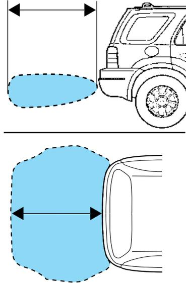
The RSS automatically turns on when the gear selector is placed in R (Reverse) and the ignition is on. An RSS control located on the instrument panel allows the driver to turn the RSS on and off. To turn the RSS off, the ignition must be on.
