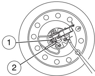
5. Use the lug wrench to remove the lug nut from the spare tire tether.
