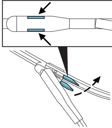
3. Attach the new blade to the arm and snap it into place.
