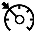
**O/D off:** Illuminates when the overdrive function of the transmission has been turned off; refer to the *Driving* chapter.
