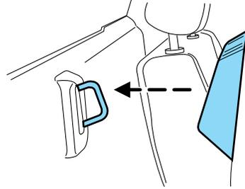
2. Lift up on the head restraint until it locks into its original position.
