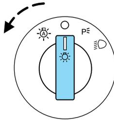
To turn the autolamps on, rotate the control counterclockwise to ☀.
