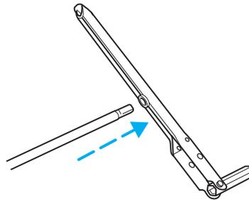
2. Insert the square end of the jack handle extension into the rear access hole located just above the rear bumper and below the tailgate. Forward motion will stop and resistance to turning will be felt when properly engaged.
