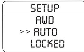
**Note:** When the AWD system is in the LOCKED mode, the 4X4 indicator will be illuminated.
