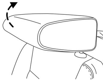
**WARNING:** Before returning the seatback to its original position, make sure that cargo or any objects are not trapped behind the seatback. After returning the seatback to its original position, pull on the seatback to ensure that it has fully latched. An unlatched seat may become dangerous in the event of a sudden stop or collision.
