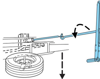
3. Connect the jack handle to the jack handle extension. Turn the handle counterclockwise until the tire is lowered to the ground and the cable is slightly slack.
