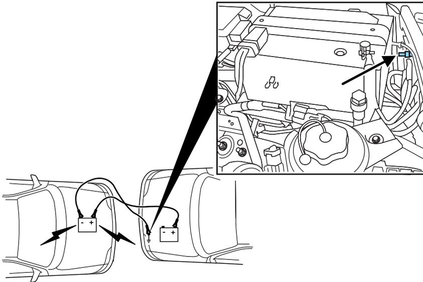
4. Make the final connection of the negative (-) cable to the ground stud located toward the front of the vehicle (forward of the battery) on the radiator support. Keep the negative (-) cable away from the battery and the carburetor/fuel injection system. **Do not** use fuel lines, engine rocker covers or the intake manifold as *grounding* points.
