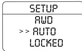
**Note:** When the AWD system is in the LOCKED mode, the 4X4 indicator will be illuminated.
