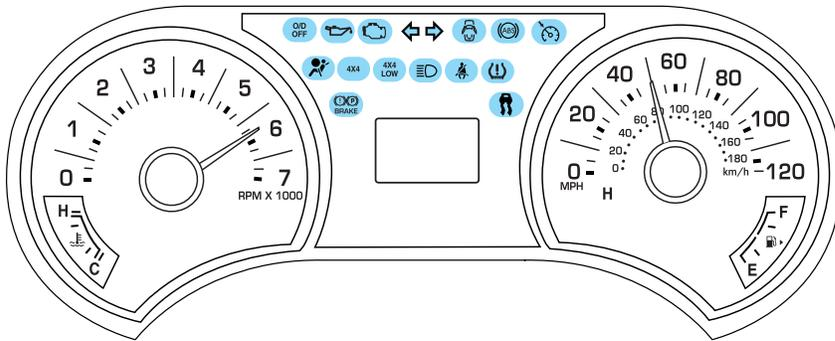
Warning lights and gauges can alert you to a vehicle condition that may become serious enough to cause expensive repairs. A warning light may illuminate when a problem exists with one of your vehicle's functions. Many lights will illuminate when you start your vehicle to make sure the bulb works. If any light remains on after starting the vehicle, refer to the respective system warning light for additional information.
