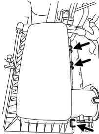
1. Release the clamps that secure the air filter housing cover.
