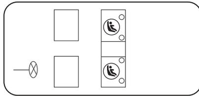
The LATCH anchors are located at the rear section of the rear seat between the cushion and seatback. Follow the child seat manufacturer's instructions to properly install a child seat with LATCH attachments.
